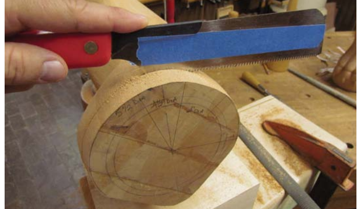
11 Use a hand saw with a piece of tape stuck to the side of the saw to cut into the foot 12mm deep
