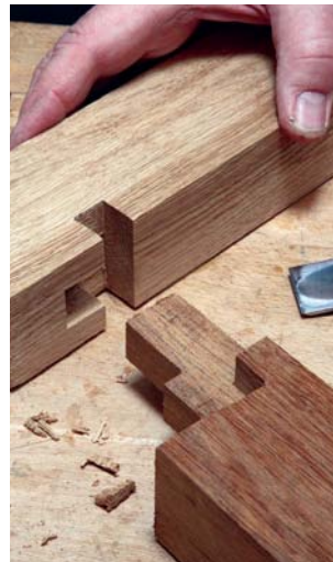
Ready to assemble the eriwa kone hozosashi has a two narrow stage tenon and a full width collar
