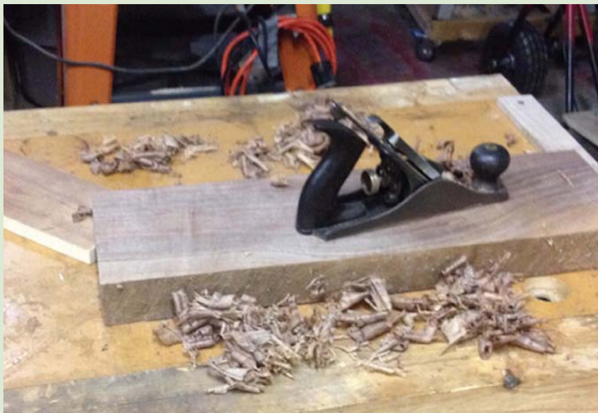
A plane stop used with a batten is as good as any vice
