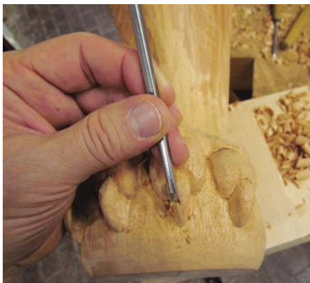
23 Use a No.2, 5mm gouge to shape the tip of each claw
