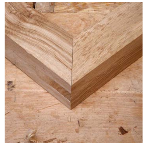
The tomekata sanmai hozo joint is particularly suitable for making strong small-scale mitre joints
