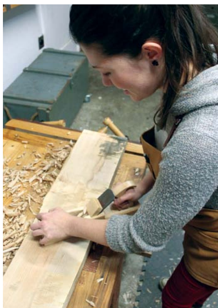
1 Traversing a board at 45° with the Jack plane to identify and remove high spots
