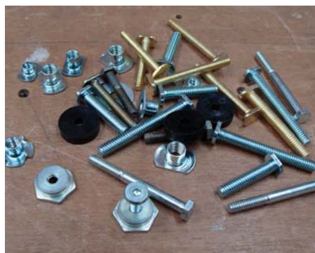
Typical contents of jig kits available from the major tool retailers
