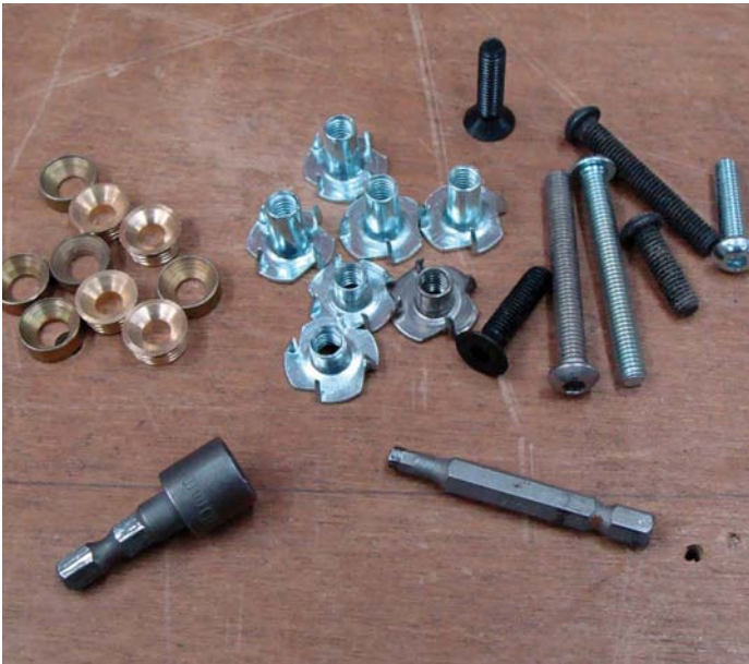
An assortment of M6 clamping fixtures and tightening tools referred to in the text. Using the bits with a torque controlled cordless screwdriver or drill can save a great deal of wear and tear on the arm muscles!
