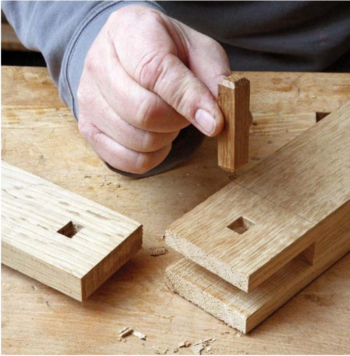
The wanagi-komi joint is an open slot mortise with a full section tenon
