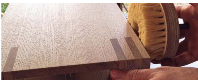
The matte surface left behind can be buffed up a bit with a dry cloth, as well as a natural bristle brush. This removes the pith and creates nice texture
