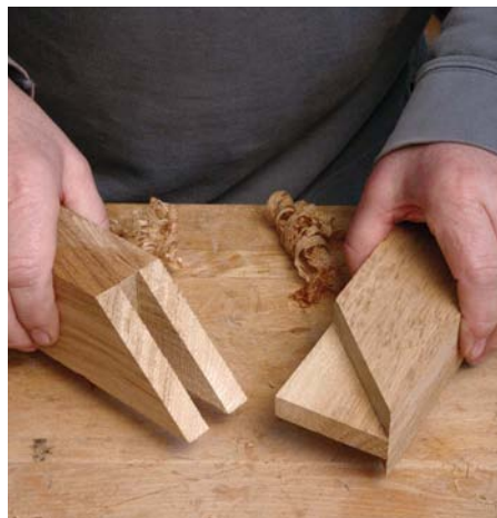
The tomekata sanmai hozo is a full width open slot mitre
