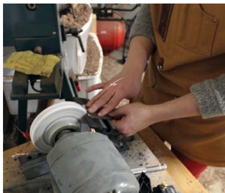
Grinding the camber
