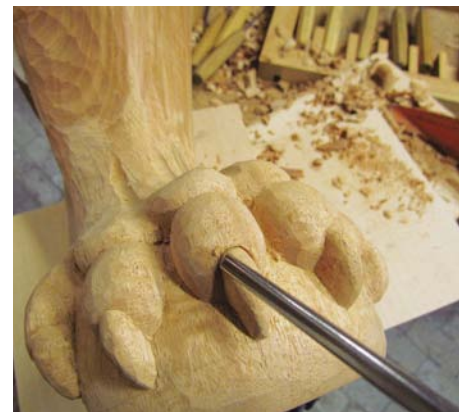
25 Stab cut into each toe at the upper radius of the claw
