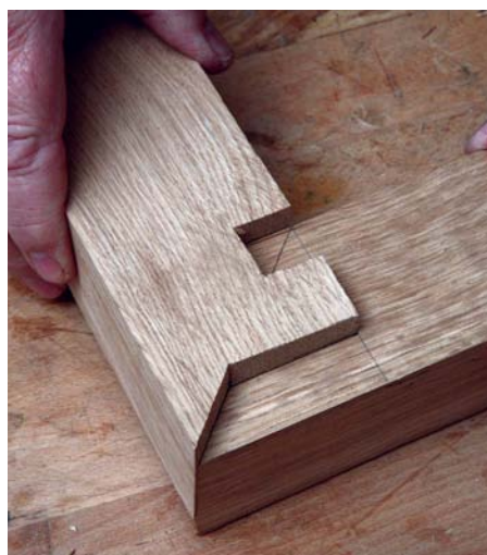
The hako dome is assembled by sliding the two halves together either sideways to progressively test the fit, or endways to finally glue up the joint
