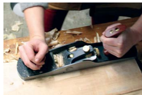
2 Slightly skew the plane and work in the direction of the grain
