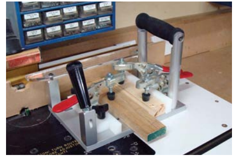
A quality ready-made sledge that came complete with three toggle clamps
