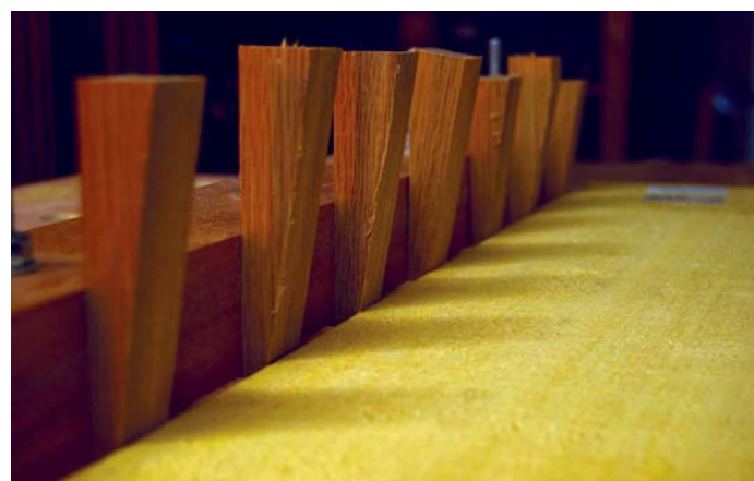
Here, oak wedges provide clamping pressure for gluing these bookmatched yellow cedar panels
