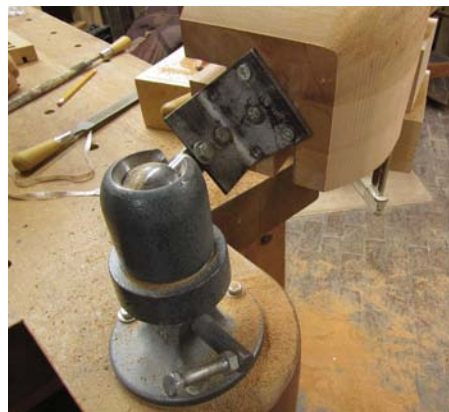
8 Mount the leg to your carving bench using a carver's vice and screw to the top of the leg
