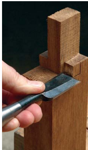
Shaping the tenon sides for a eriwa kone hozosashi or collared haunch mortise and tenon joint
