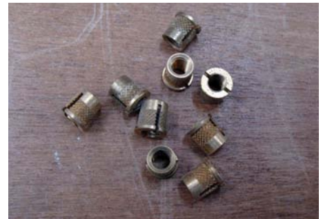
Another type of threaded fixing, this time for plastic and Tufnol
