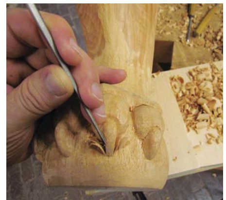
22 When carving the claw, keep in mind that the shape is wider at the top and thinner towards the tip
