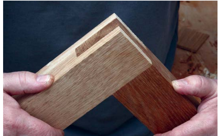
The strength of a kanegata sanmai hozo joint comes from the large area of the glued long-grain faces, which must be a good fit
