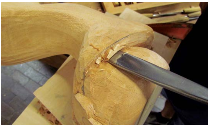
18 On the side of the foot, draw in the arch of the thumb approximately 12mm higher than the heel
