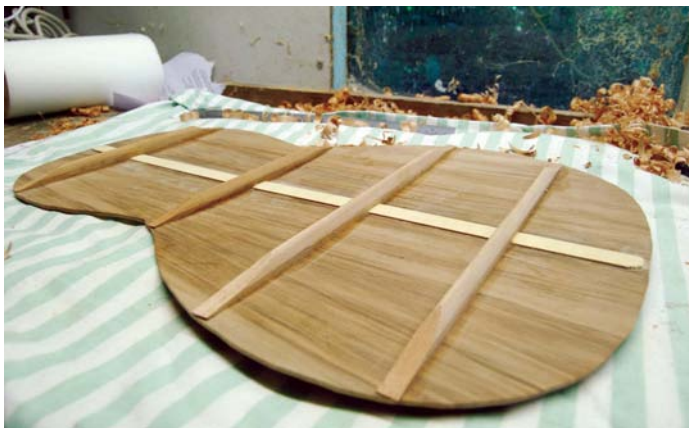
Cedrela braces on red gum back for a 19th-century parlour guitar build, glued with go bars
