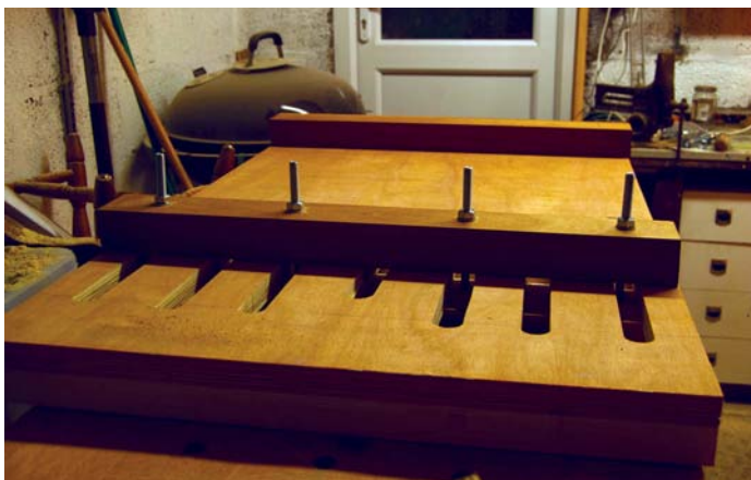
A simply made jig makes gluing thin panels straightforward
