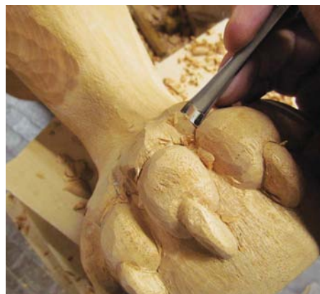
21 You can then round and shape the radius corners of each knuckle
