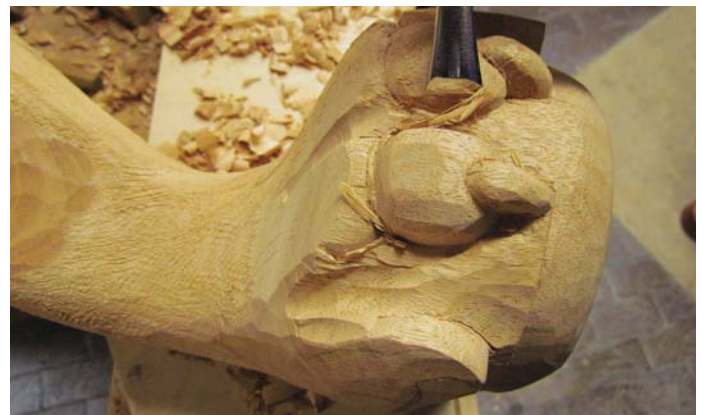
19 To carve the toes and claws of the lion's foot, keep stab cutting into the ball around each toe, knuckle and claw
