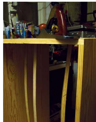
Go bars prevent the carcass side from deflecting under the weight of the plane
