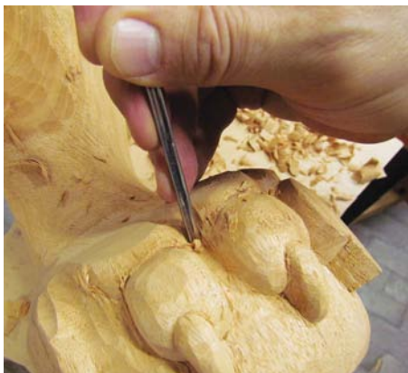
20 Begin shaping the knuckles and carve a small radius between each knuckle down into the ball
