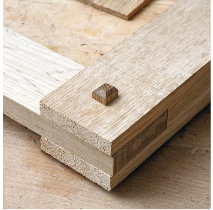
With a well-fitted peg driven in the wanagi-komi is locked solid
