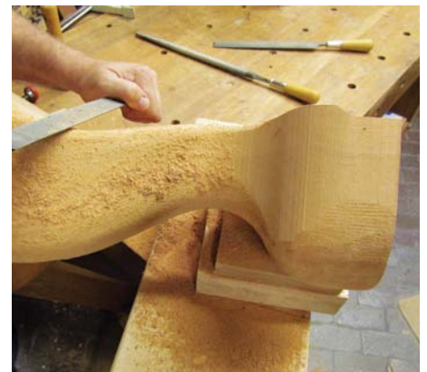
9 To shape the leg, use a medium wood rasp to round the front corner and blend it into the sides
