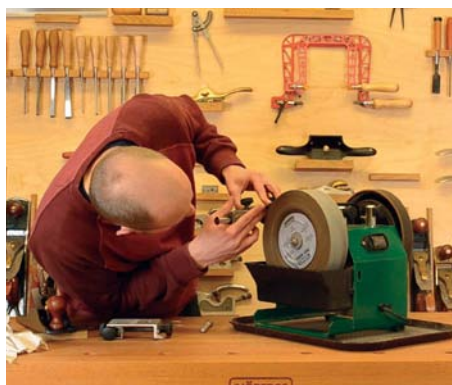
Accurate positioning of the primary bevel against the wheel
