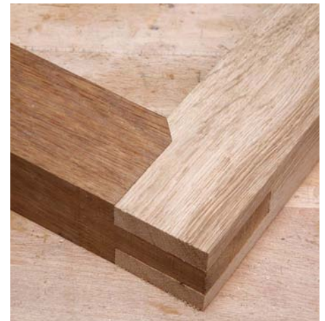
As with any mitred joint, accurate alignment of the angles is essential for a good fit
