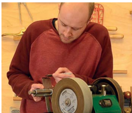
Felt-tip pen is used to aid inspection of the blade positioning
