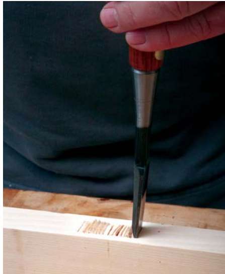
Each end of the mortise is chopped with the straight back of the chisel. Note the chisel is tilted away from the centre so the mortise ends slope inwards
