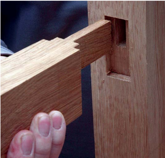
The two-stage tenon is trial inserted in the two-stage mortise
