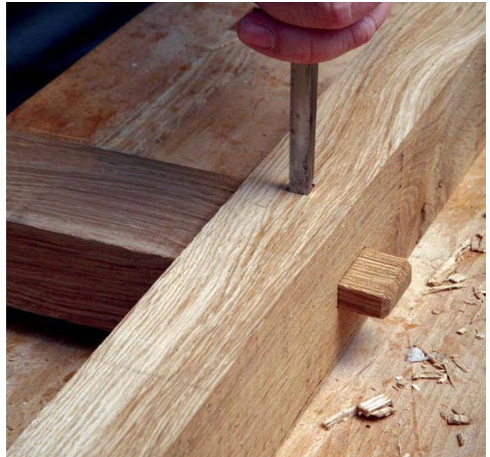
A socket is chopped through the side of the mortise to take a locking peg
