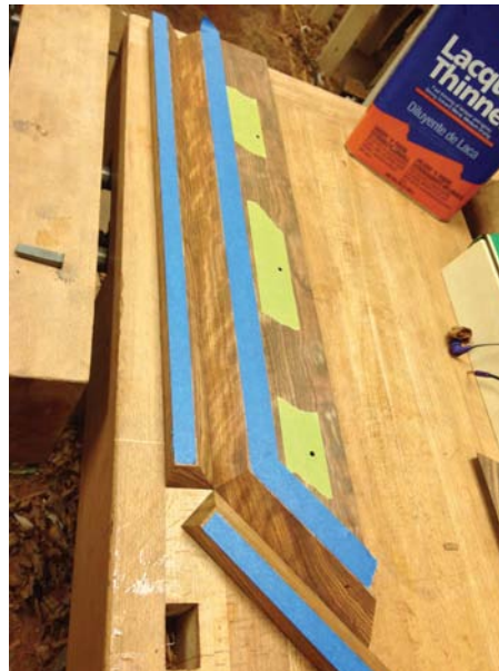
Preparing the breadboard mitre fold
