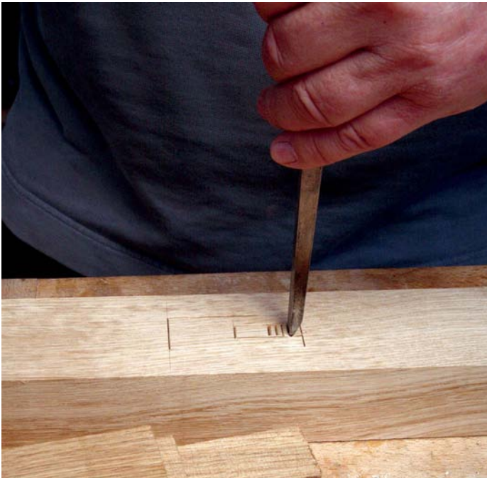
The deep, narrow inner mortise is chopped through from both the entry and exit face
