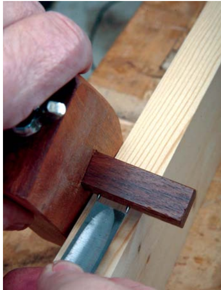
The width of the chisel matches the spacing between the two pins of the kebiki dai mortise gauge
