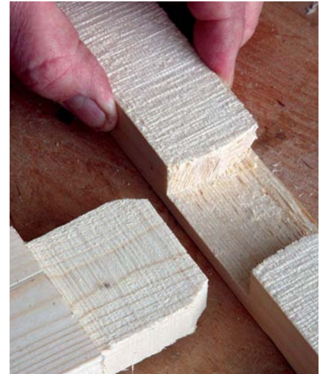
This through-mortise has been sawn open to reveal its inner shape. It narrows towards the middle while the tenon has a chamfered end to ease it into the mortise
