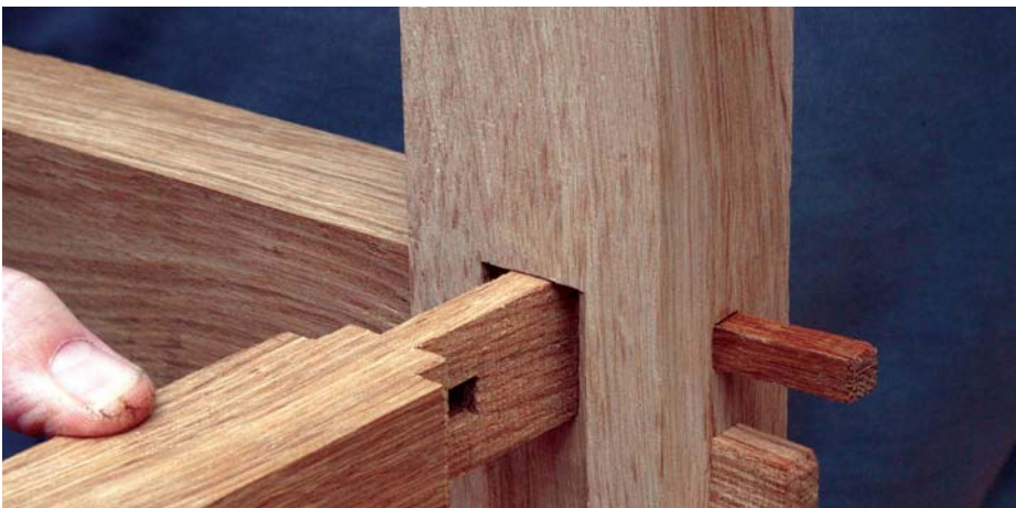
A pair of haunched tenons are inserted in their mortises and locked in place with pegs
