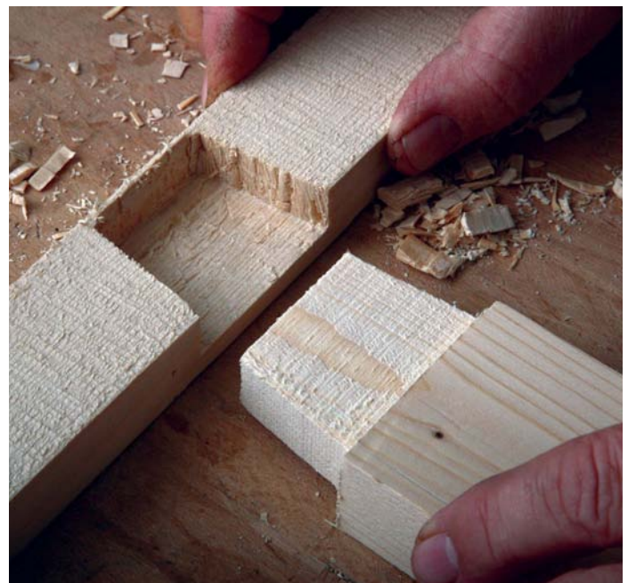
The tapered tenon will be wedged tightly into the tapered mortise – cut away for clarity
