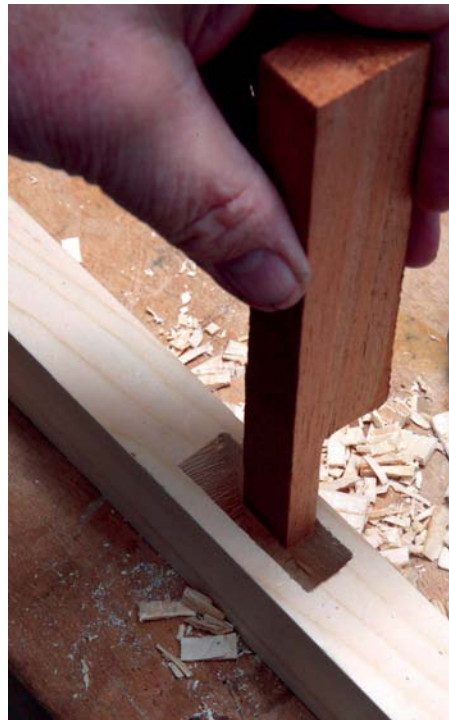
A simple depth gauge is used for checking progress of the blind mortise
