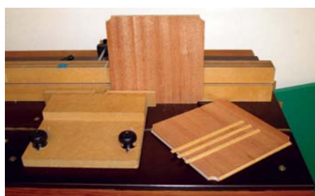
7 The bottoms, once the quarter-round corners had been completed
