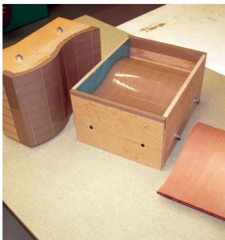
9 I made a two-part mould to press the laminations
