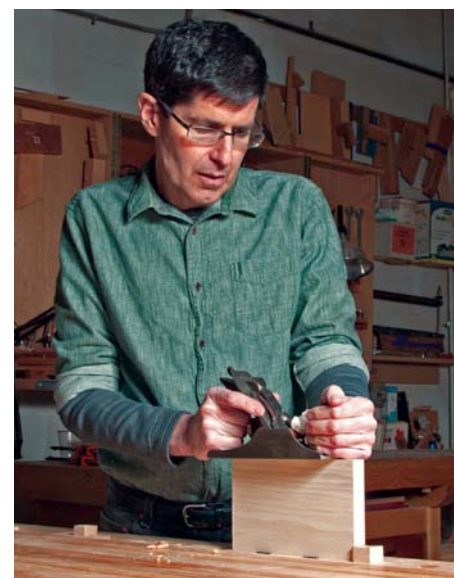
Planing a short board upright against a single bench dog is a good way to learn about balance and pressure when planing
