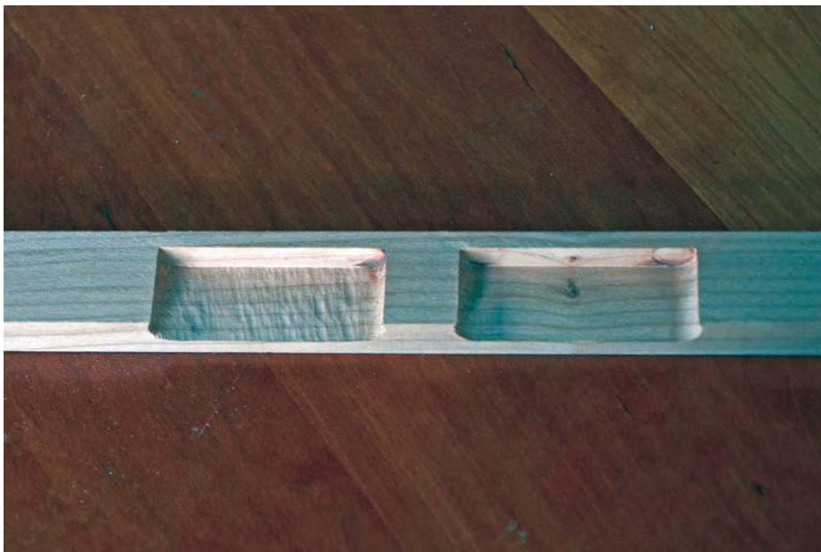
Cutting too aggressively with the router caused problems both visible – note the rough surface – and invisible – it is measurably wider – in the mortise on the left – sliced in half lengthwise. The otherwise-identical mortise at the right was routed at an appropriate speed
