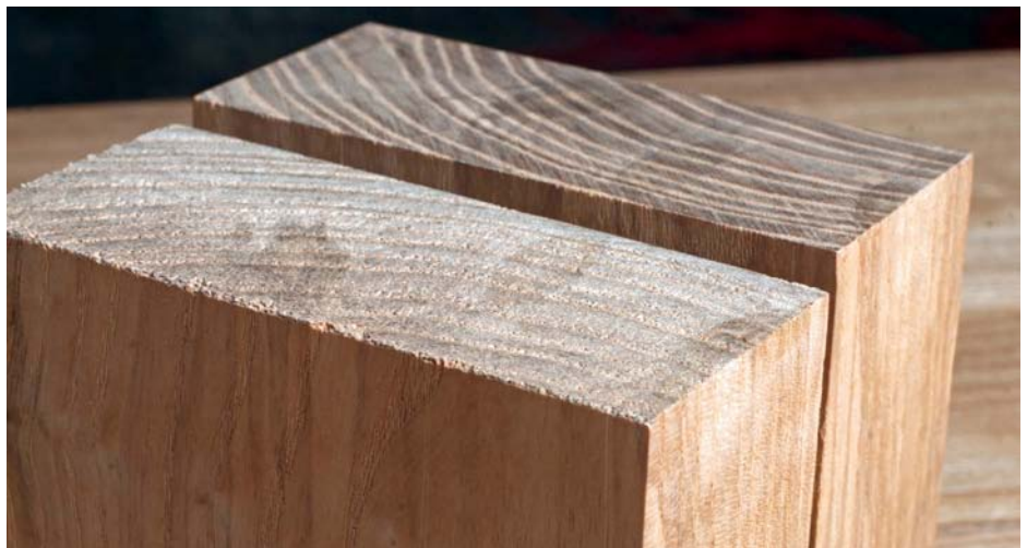
Cutting too hard – or fast – with a machine makes a mess of the cut. I cut the block in front too quickly on the tablesaw. I fed the back piece through the saw at the proper speed
