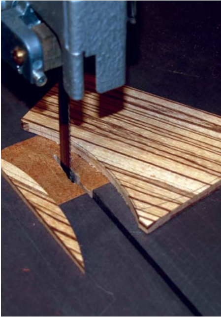
20 The inner curve sawn on the bandsaw
