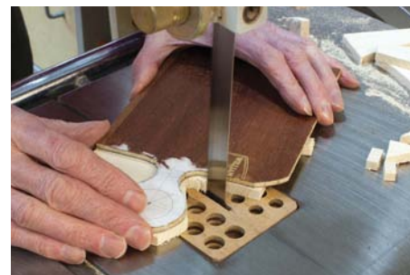
8 An over-length template keeps fingers well away from the blade. If, like me, you don't have a narrow blade that will make curves this tight, it's easy to make several straight cuts into the curve and then nibble away the remaining waste
