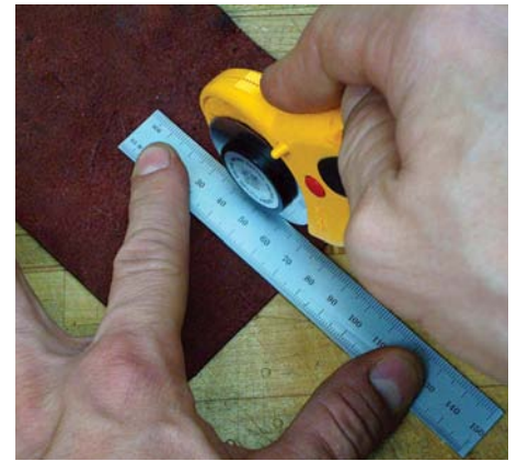
Using a standard rotary cutter and metal rule to cut out the pieces from this vegetable tanned leather scrap
