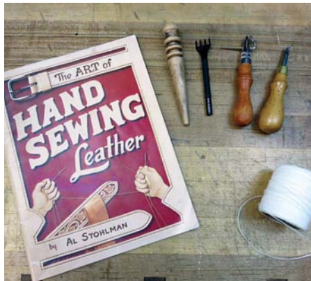
Specific leather tools that will be needed. Pictured from left to right, The Art of Hand Sewing Leather , hand burnisher, diamond chisel, adjustable stitching groover, No.2 keen edge beveller, needles and waxed thread
