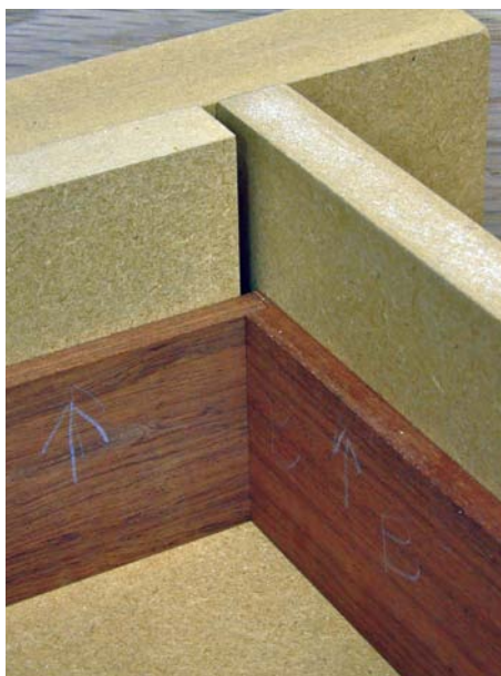
The 'T' section is secured to the base with a number of Miller dowels and the two 'T' elements are similarly dowelled
