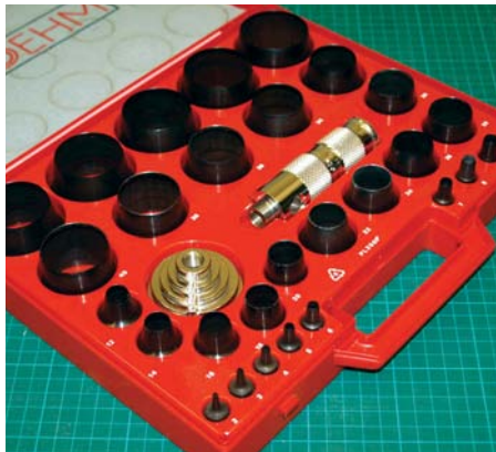
32 I have a set of disc punches which can be used to punch single discs or in combination to punch washers
