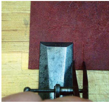
A set of dividers are the perfect tool for marking the layout of the chisel cover directly on to the leather's surface
