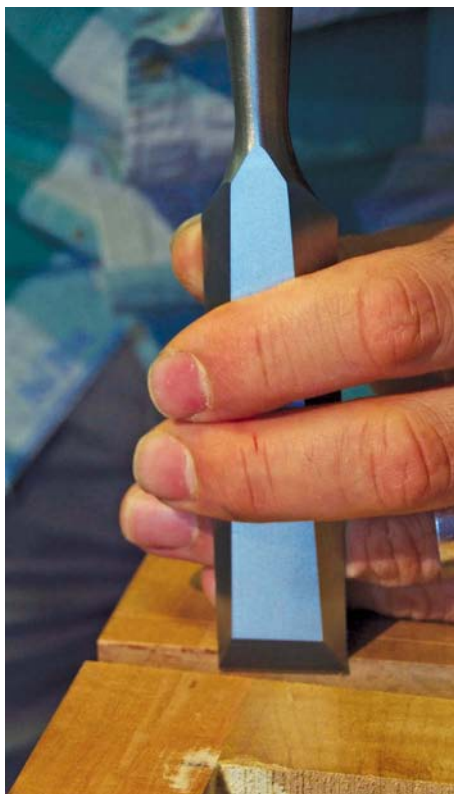
Paring the joint for the slipper heel, on an acoustic guitar neck in steamed pear
