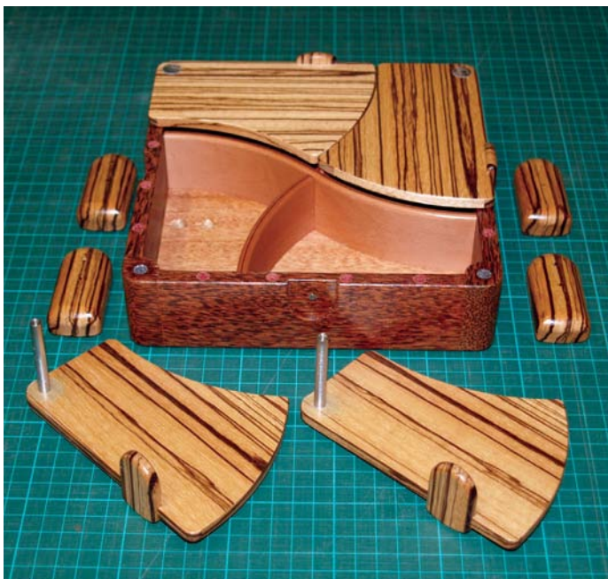
34 I sprayed a basecoat and two top coats of Morrells pre-cat 10% sheen lacquer for the finish
