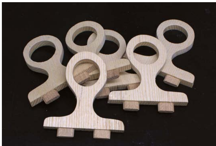
10 The completed bulb holder plates. The narrow sections minimise light obstruction
