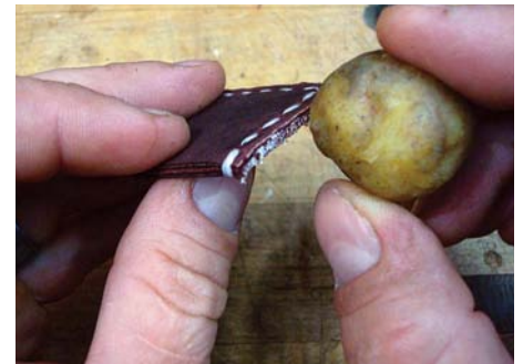
Lightly rubbing a block of beeswax along the edge of the leather prior to burnishing. The warmth created here melts the wax, allowing it to penetrate the leather
