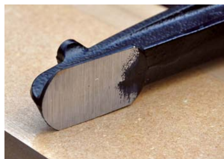
The Bahco 'F' cramp end jaw ground to ensure it is at 90° to the cramp rail and applies even pressure. The plastic shoe still fits securely
