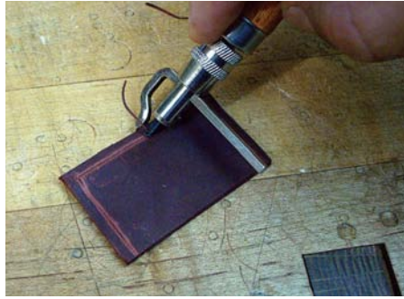
The stitching groover cuts a channel for the thread to sit in; this keeps the stitches below the leather's surface, reducing abrasion and wear
