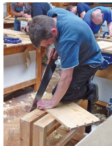
Ed Sutton cuts the slope on his Dutch tool chest by hand using his 'shop made saw bench
