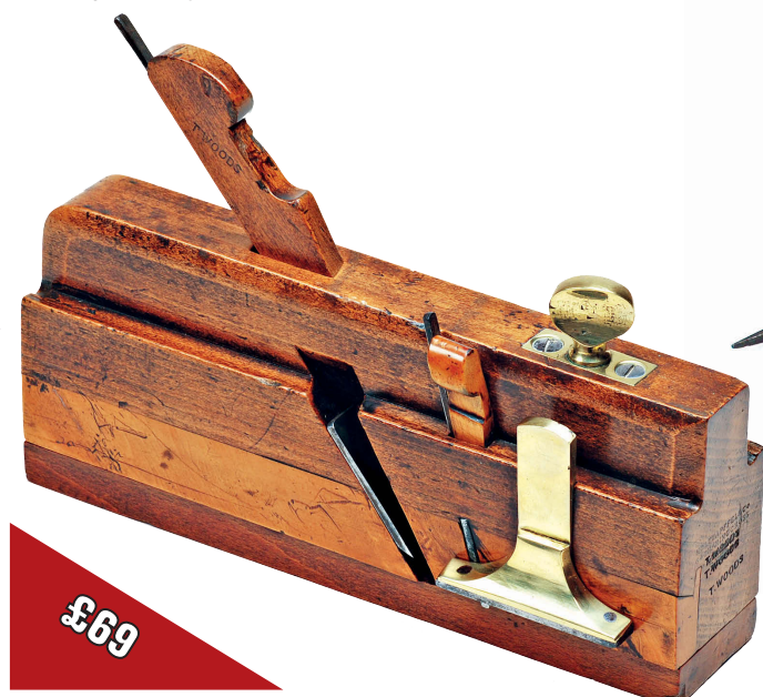
Lot 908. The fillister “is intended to plane both with and across the grain, as in planing a rebate around the margin of a panel,” wrote Charles Holtzapffel in his book Turning & Mechanical Manipulation . This 9 \frac{1}{2} in example in beech and boxwood with brass screw stop bears the mark of Holtzapffel & Co., 64 Charing Cross, London
