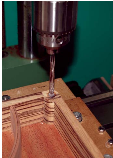
26 After the resin had cured I drilled and reamed the holes to get the smooth fit for the rotation of the lids
