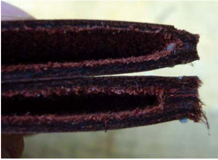
In these cross-sections, you can see the exposed thread where no welting is used – top – and the added protection when welting is used – bottom
