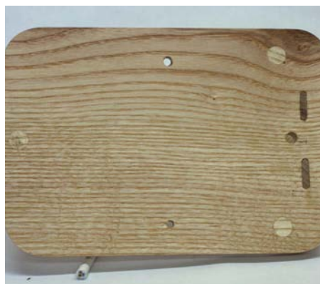
13 The magnets need to be recessed as far as possible into the backplate; you don't have to plug the recesses after fitting the magnets but it makes a neater job. This is an early plate with three magnets but I subsequently fitted four for a firmer grip between frame and backplate
