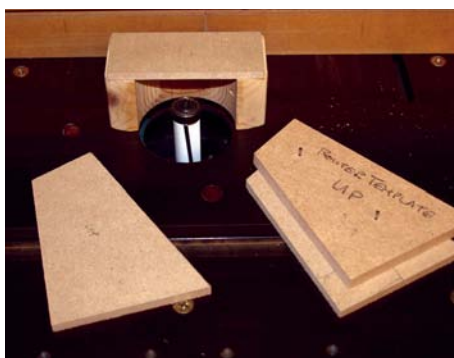
17 The shape was cut with a ball-race router cutter on my router table
