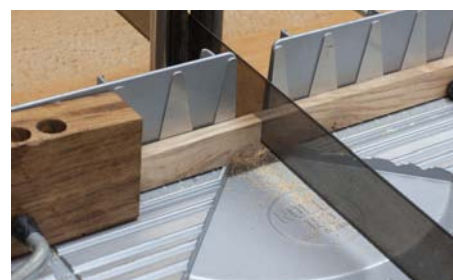
1 My Nobex mitre saw with clamped-on stops made a good clean job of cutting to length
