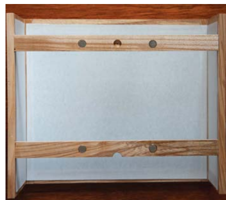
14 Magnets are glued using CA adhesive into and flush with the back of the frame cross rails
