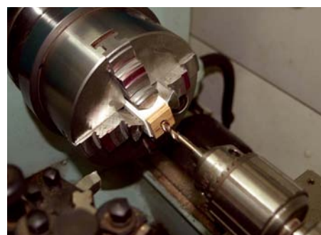
4 An engineering lathe is used to drill the pivot holes in the corner blocks
