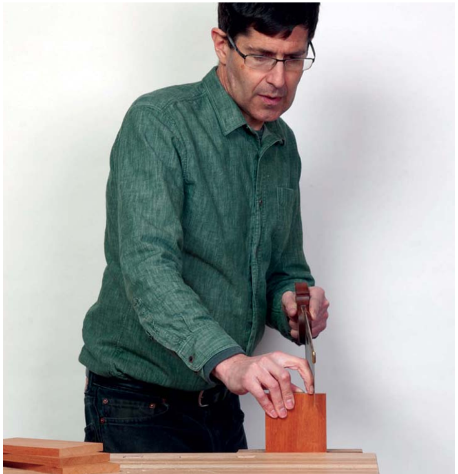
Here, the saw and my forearm line up correctly. I'm a little further off to the side in order to accomplish this
