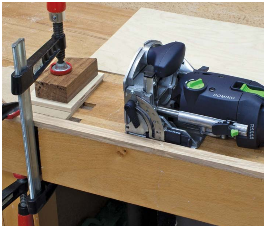
6 Cutting the mortises in the lamp holder plate – best done before shaping. It's easy to create a simple jig by clamping fence pieces to the bench. The Domino jointer runs against the left-hand fence for one mortise and the right-hand fence for the other. A piece of MDF acts as a front fence and raises the workpiece to the correct height
