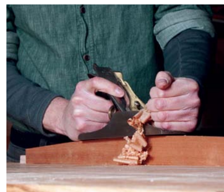
To keep the cutting edge on the wood when you plane a convex curve with a straight plane, you have to learn to balance the pressure between your hands
