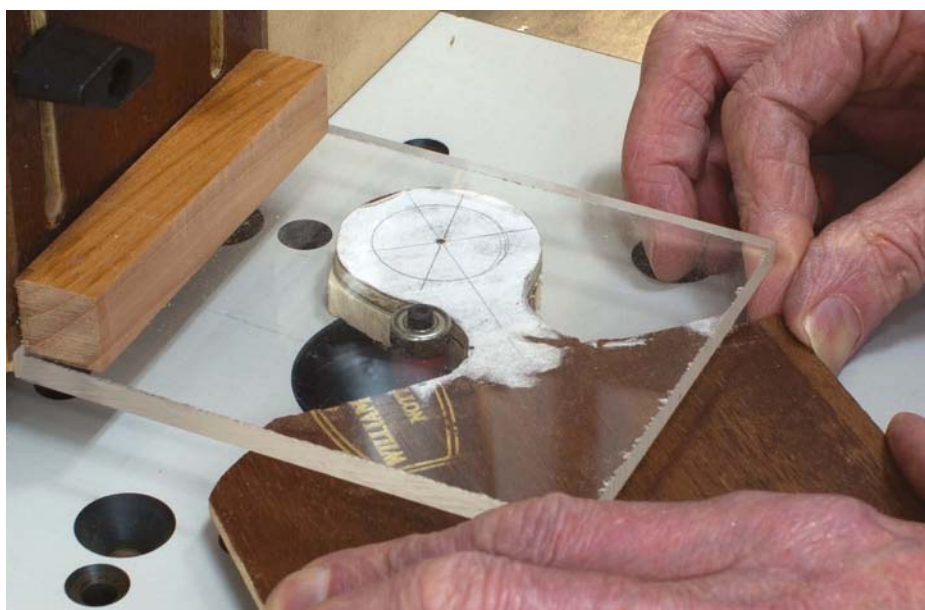
9 Cutting with rather than against the rotation of the cutter can be scary but can give a much better finish. A firm grip and a clear acrylic guard set close to the work enables it to be done safely
