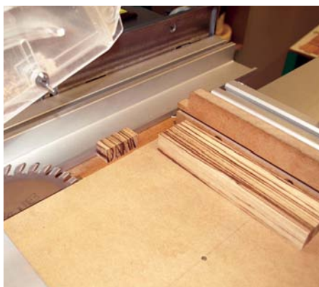
2 Dimensioning the pieces using the sliding table in conjunction with the rip fence
