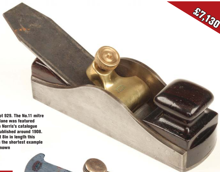
Lot 947. This little-used steel-soled gun-metal 4in Norris A28 chariot plane with ebony wedge and full original 1½in Norris iron brought the highest bid of the sale
