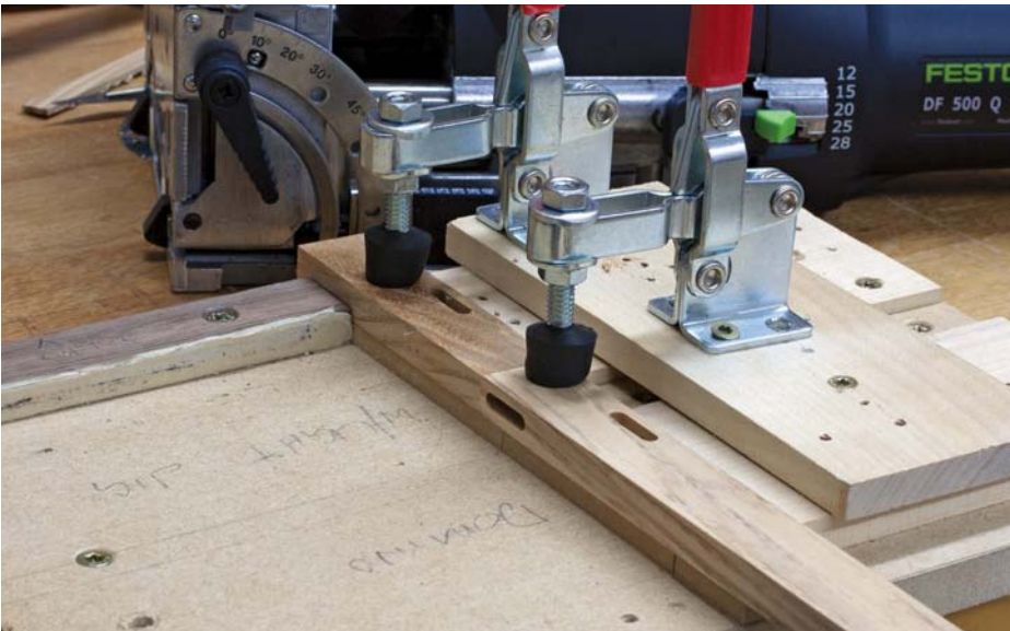
3 Clamped-on stops position the cross grain mortises. Left and right should be done separately so that the cut is always referenced off the face side and edge
