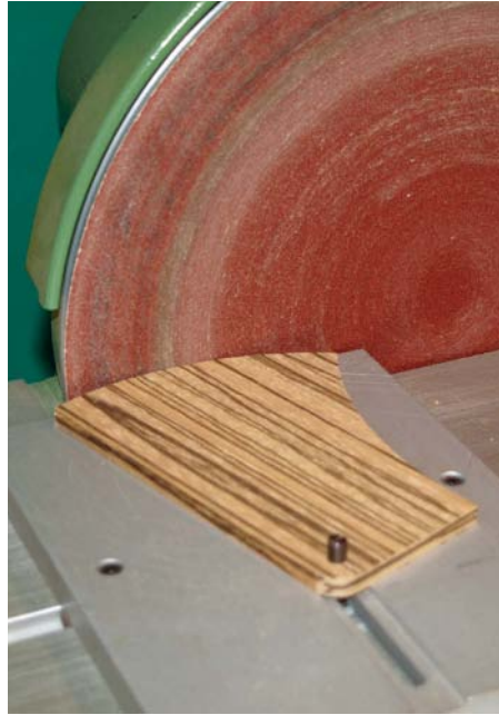
21 Outer curve formed on disc sander using a pivot pin
