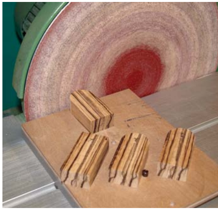
30 Inner profile of feet formed on the disc sander
