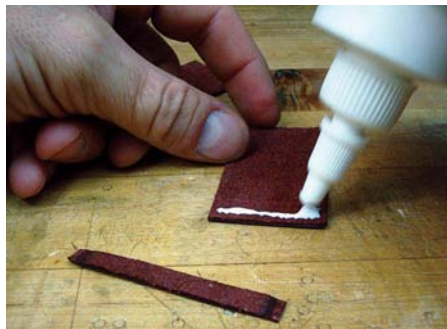
Apply leather cement to all edges being stitched; this will help hold the leather together as you pierce holes and stitch. I prefer using a water-based leather cement from Tandy Leather. Here you can see the skived ends of the welting
