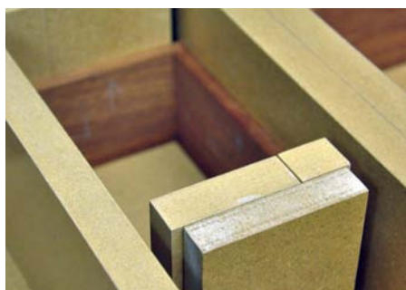
If you use two spacers for an odd size, ensure you have a further block behind to apply even pressure from your cramp
