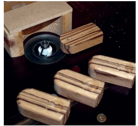
31 Rounding over of feet in stages on the router table
