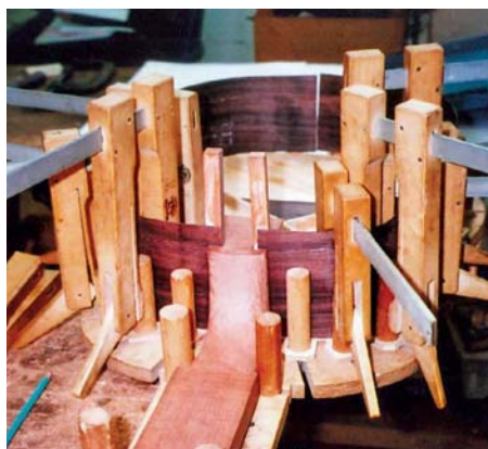
Gluing an acoustic guitar in a solera. Once the glue is dry the mahogany wedges will be trimmed to length and the back glued on
