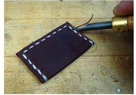
Using the edge beveller tool to round over all of the edges prior to burnishing
