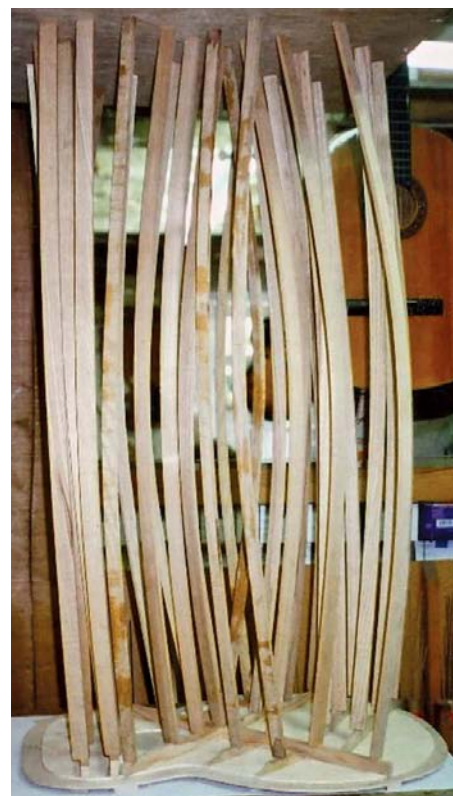
Using go bars to glue braces to an acoustic guitar soundboard
