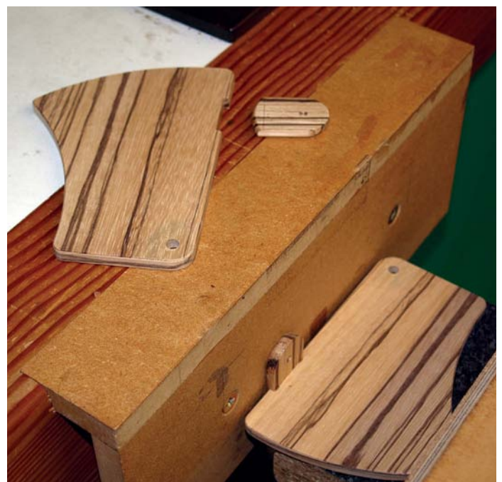
24 The handles were then glued into the slot in the lid being held in place and cramped in a bench vice
