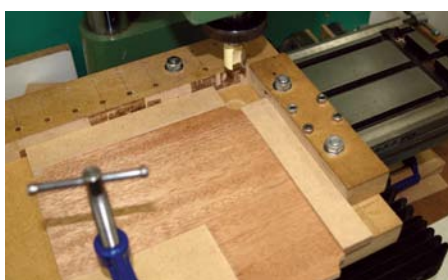
6 The bottom of the box is made from 6mm-thick MDF veneered with khaya
