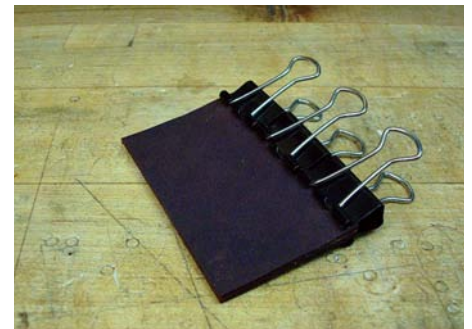
Small binder clips are the perfect clamping accessory. If you feel that they may mark the leather, a piece of paper can be placed between the clips and leather while clamped
