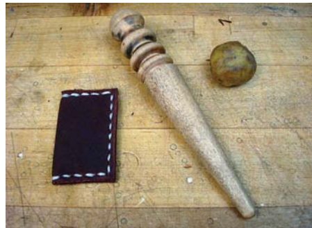
After bevelling the edges, it's time to clean them up with some beeswax and this wooden burnisher
