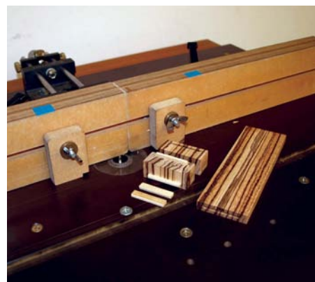
3 The corner blocks are joined to the sides with loose tongues
