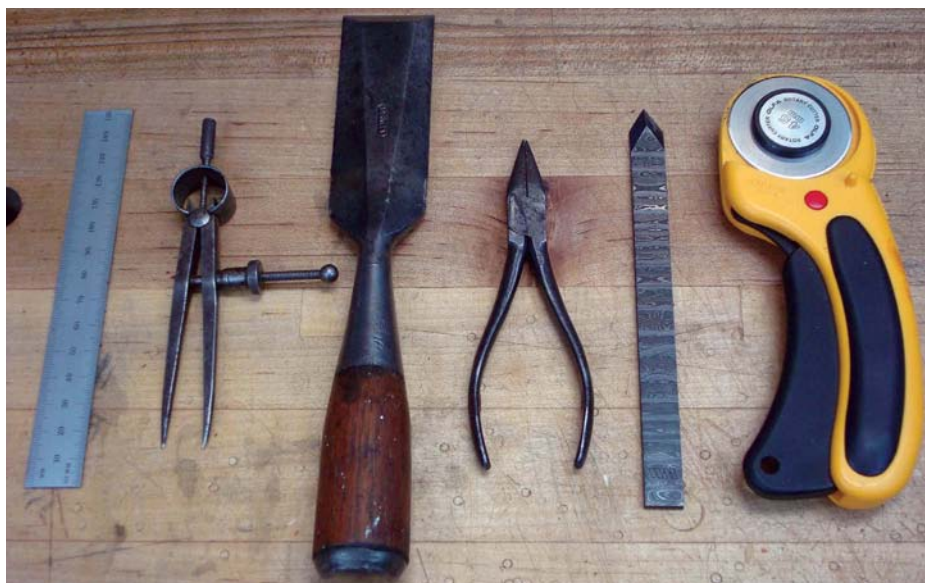
Other everyday tools and woodworking tools that will be used. Pictured from left to right: 150mm metal rule, small dividers, chisel, small needle nose pliers, marking knife or utility knife and rotary knife
