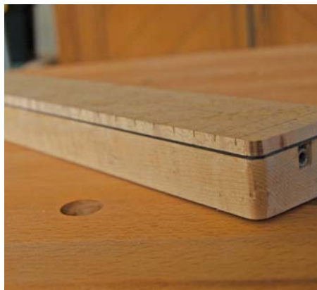
Dyed sycamore veneer between a birds-eye maple neck and fretboard, on an electric guitar build
