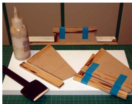
18 The glue was applied to the edge of the MDF with a comb spreader
