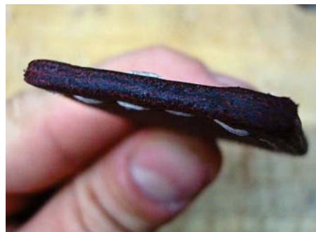
Here you can see the edge of the leather after burnishing. The warmth created during the process melts the wax, allowing it to penetrate and adhere to the leather. This provides protection for the leather and looks aesthetically pleasing
