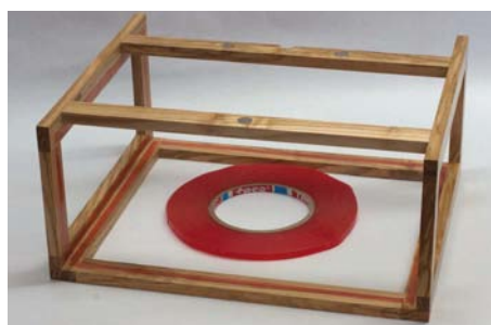
15 Fitting shade parchment is easy with 6mm-wide double-sided tape and...
