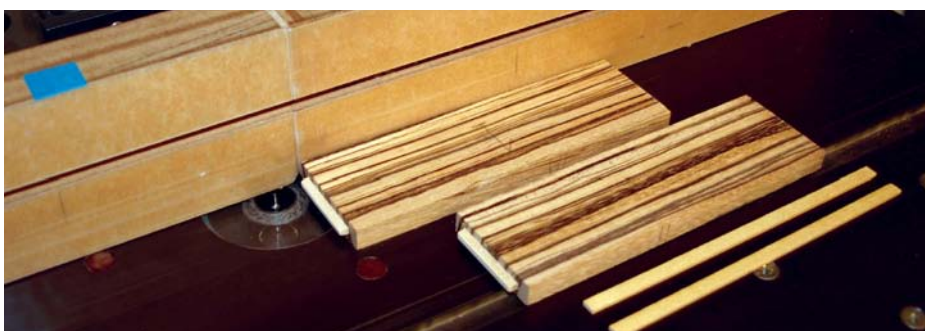
8 The pressure block was then removed to use the fence setting for the grooves on the inside faces of the box sides
