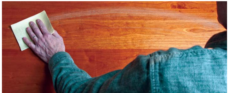
The natural pivoting motions of the shoulder naturally lead to a curved stroke with the sandpaper
