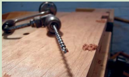
Drill the holes for the removable fence
