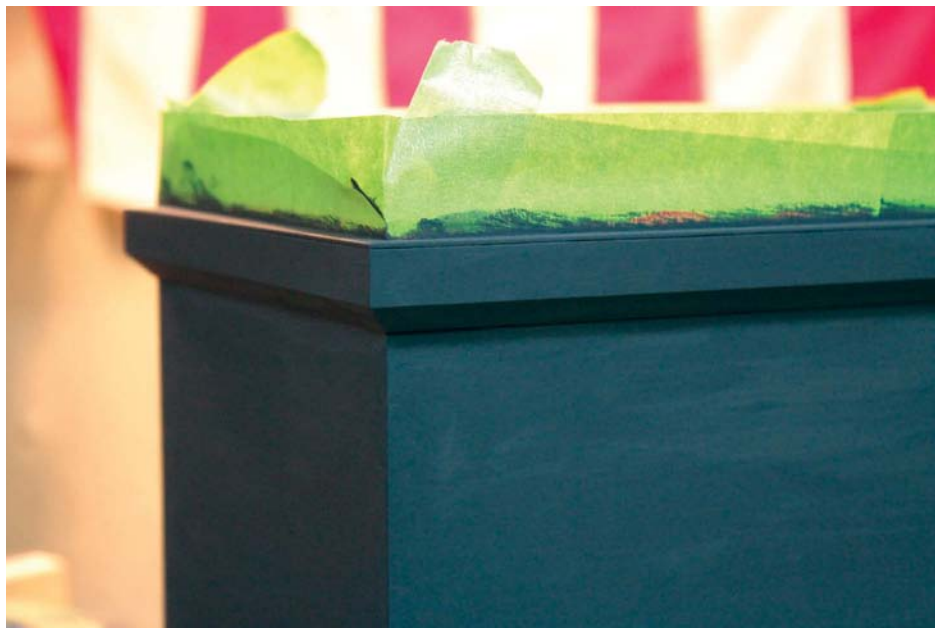
Keep sharp edges and corners crisp and don't load up any fine details with paint
