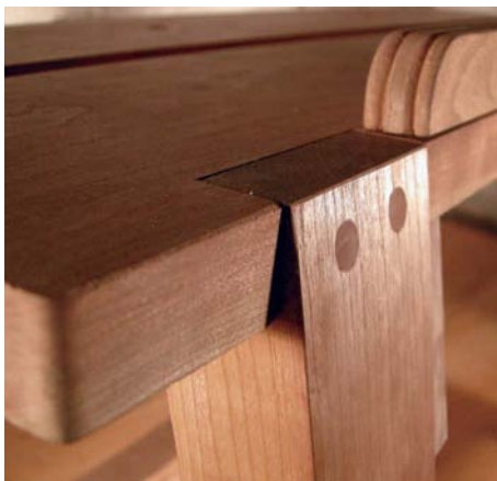
19 Two dowels through each leg's top joint
