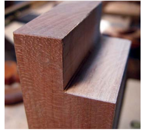
7 Saw the square notches in the top of the legs and clean up the joinery with a sharp chisel
