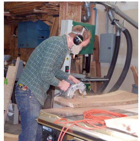
5 Using a circular saw to cut away the waste so I can achieve my 25mm thickness for the top
