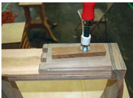
23 Once the knuckle joints are cut and drilled, the part that attaches to the skirt is glued in place
