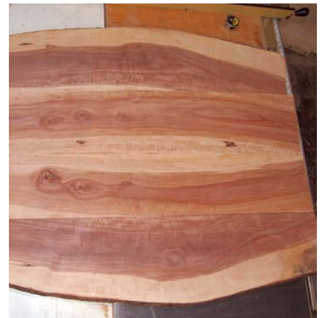
7 Milled and jointed, the top is now ready for the joinery
