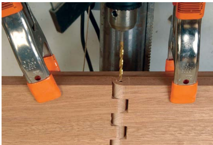
Check your drill for accuracy and drill both parts of the hinge at the same time
