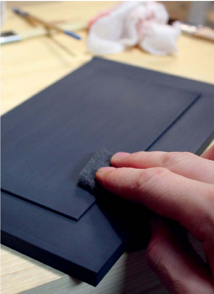
Abrasive pads are gentle on sharp edges and less likely to break through the paint layers and expose the bare timber
