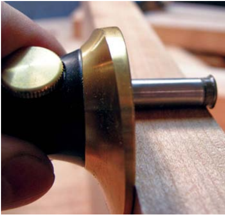
5 Set the marking gauge using the top board as reference for the lap-joint depth
