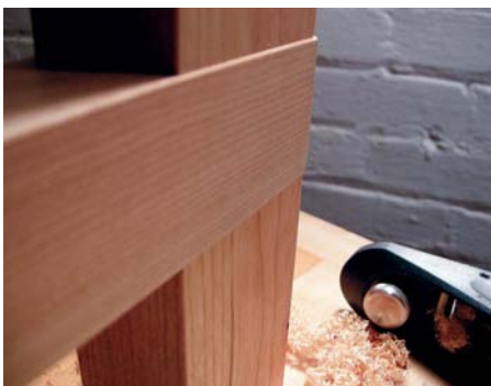
9 Dry-fit the legs and stretchers
