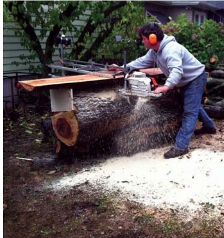
2 Using an Alaska mill to slab up the base. Note that the trunk is so wide the first cut is being made while standing up
