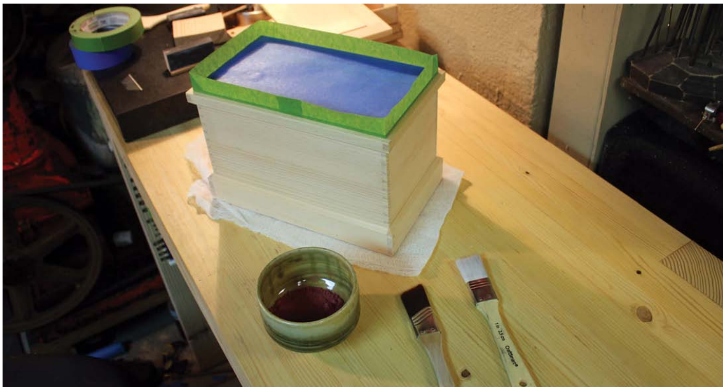
The inside of the chest is left bare so mask it off to avoid dust contamination and any accidental flicks of paint
