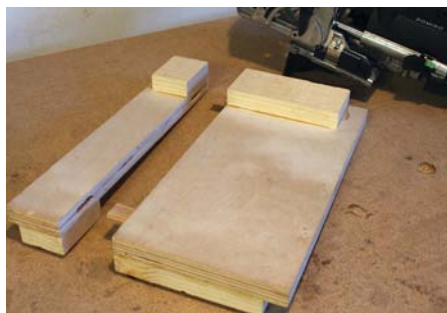
Make sure the dowels or tenons don't fit into the holes or mortise slots too tightly
