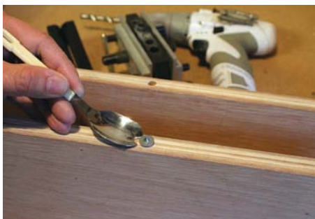
A teaspoon with a 'V'-notch cut in it makes a great dowel centre extractor
