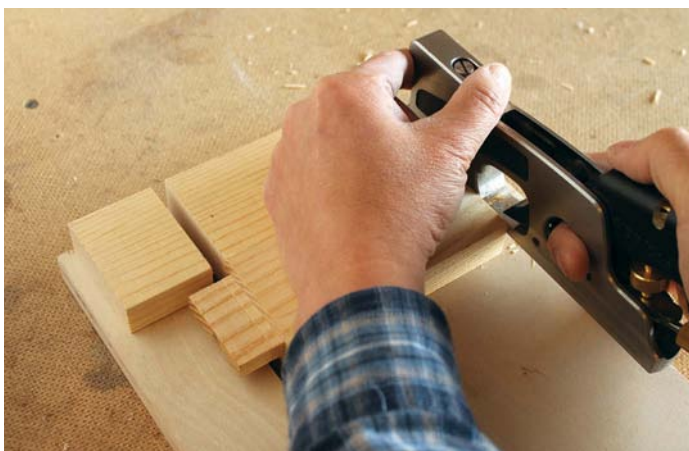
My off-hand holds the stock against the stop as well as pressing the plane down on the cheek
