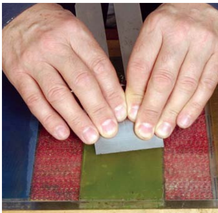
The finer micro films can rupture easily if you apply pressure on both the forward and back stroke
