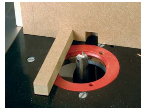
Use the dimensions of the cutter to determine the size of the locating pin and space
