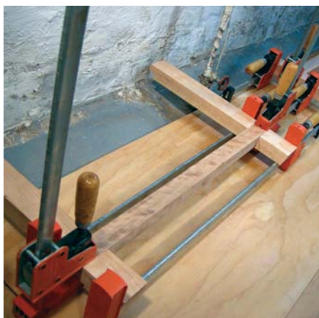
14 Assemble the legs and stretchers first; clamp and leave to cure overnight
