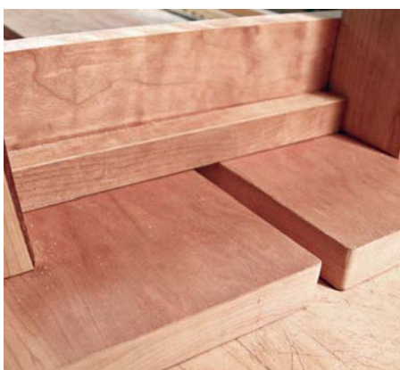
17 Drill and countersink the apron and attach it to the inside of the legs with three No.8 x 38mm wood screws
