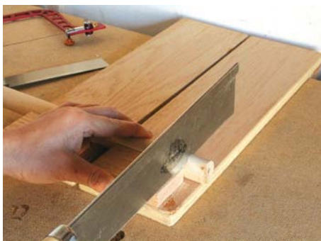
Flip the bench hook over and use the hook for sawing in pull strokes
