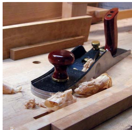
15 Once the glue is dry, you can plane the aprons and cleats flush
