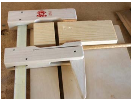
My wooden cam clamp makes a handy stop block when I cut a batch of identical dowels
