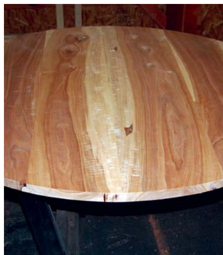
12 The top with the rule joints cut
