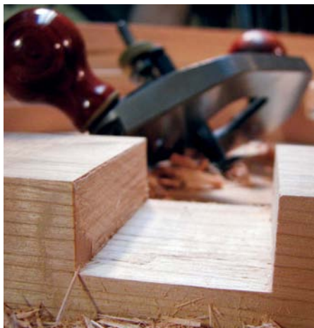
4 Use a router plane to fine-tune the depth
