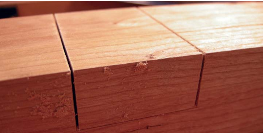
2 The first two saw cuts establish the width of the lap joint
