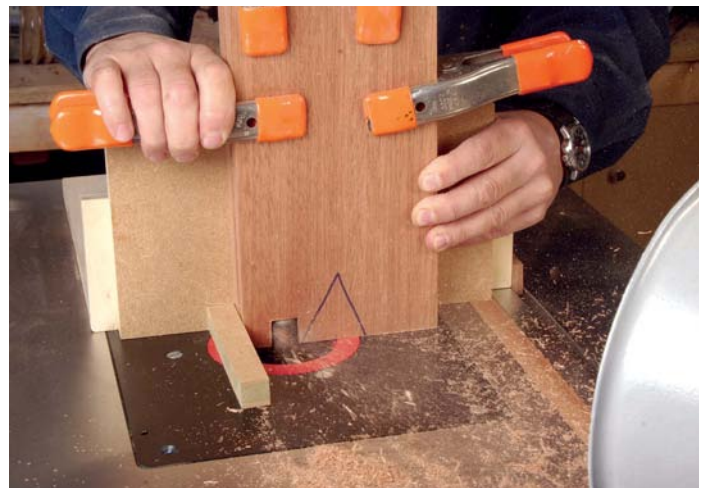
The first pass is made with the hinge parts tight up against the pin
