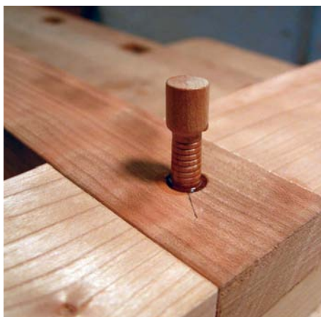
13 Drive wooden dowels through the lap joints for added insurance
