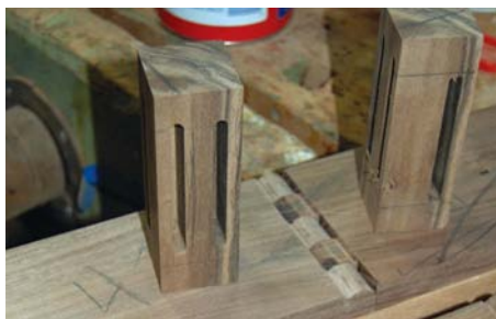
21 The double mortise and tenon joinery for the skirt. Note how the bracket parts are all numbered and have arrows for orientation
