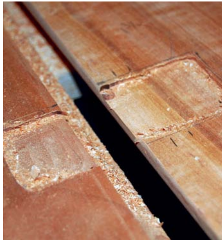
15 I used the router freehand to rough out most of the waste before squaring up the sides and corners with a chisel
