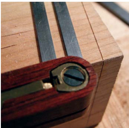
8 Set a sliding bevel gauge for the top and bottom of the splayed legs
