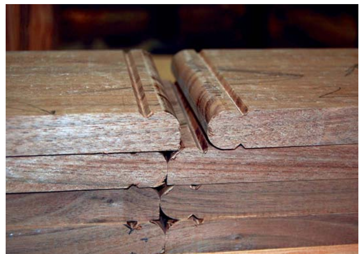
20 The brackets after passing through the roundover and V-groove bit. Next, I used a chisel to round over one side of the V-groove to match the radius on the other side
