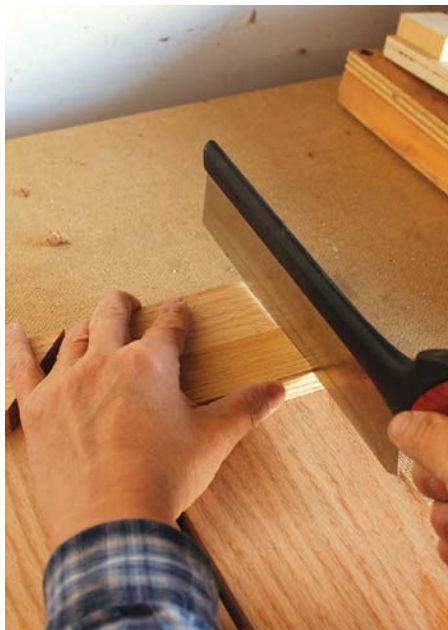
The pencil line on the stock and the stop's edge together give a longer line to align the starting cuts
