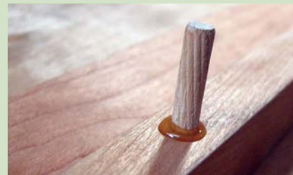
Glue the dowels in the bottom of the fence
