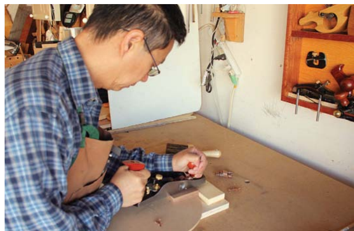
A scrap board raises the thin stock above the bench hook's stop
