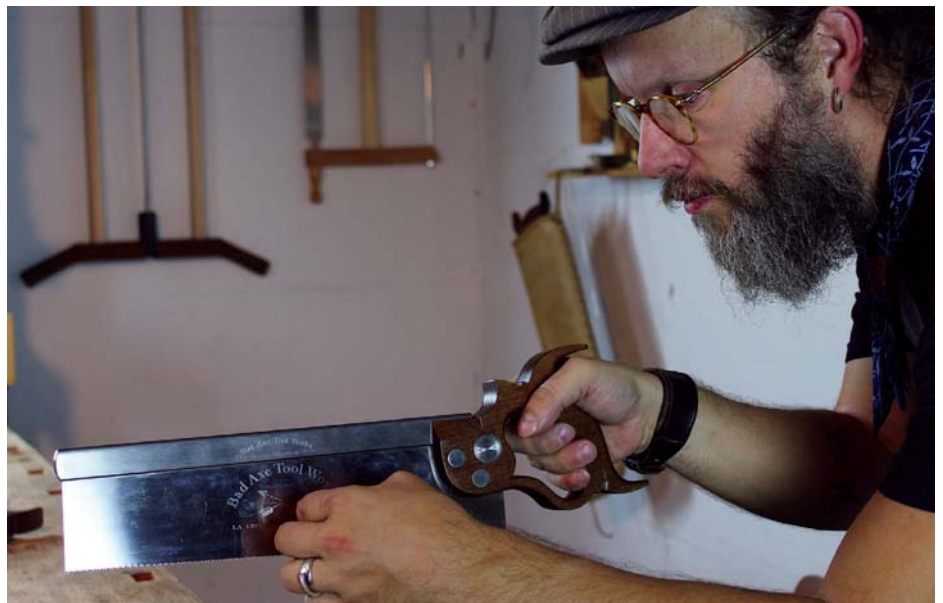
My 305mm small tenon saw filed at 14ppi rip is also great for cutting dovetails
