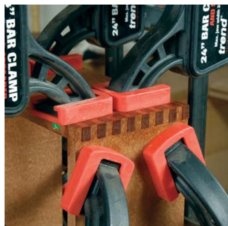
Clamp together gently with the clamps behind the pins
