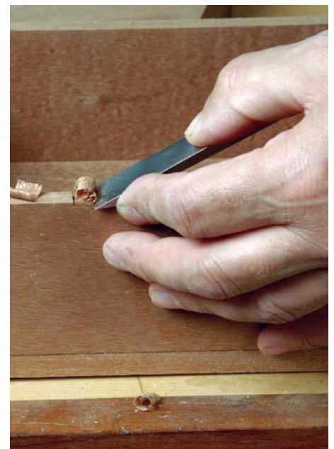
Use a chisel with the bevel facing down to pare the waste down to just above the depth line
