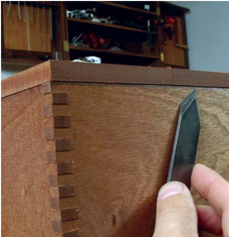
Mark the tops and bottoms and trim to size
