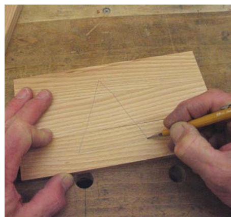
Mark the rails together with the mid-rail, if there is one. Again, this gives positive orientation and positioning for each component
