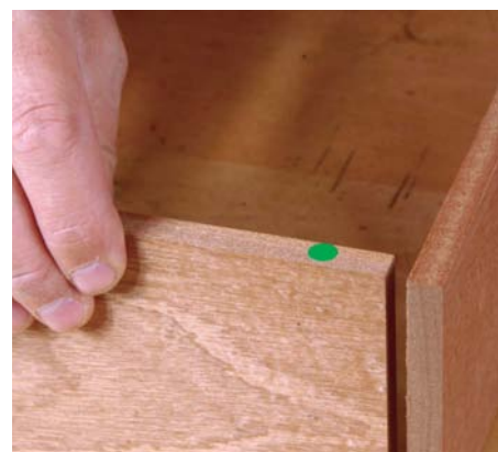
Mark the components to identify the orientation for machining
