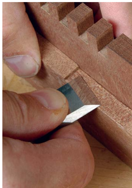
Use a block of wood to prevent the chisel from slipping off the back of the mortise
