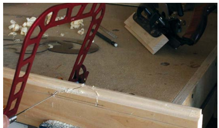
Cut out the desired profile for the pull with a fretsaw or coping saw
