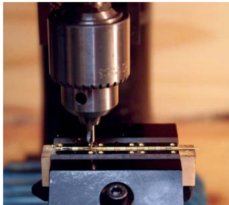
A centre drill is used to position the holes
