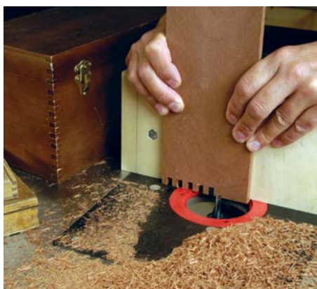
The classic box construction method
