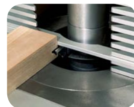
Variable multi-functional moulding fence for extra safety, working on smaller work pieces.
