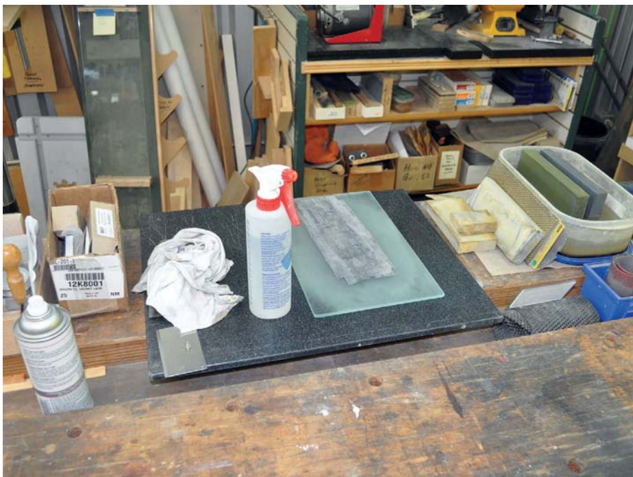
My sharpening station in the shop at work spreads across half a workbench. Laid out for efficiency because I do a lot of sharpening. Stone pond to the right and the Corian work surface in the middle also serves as a flat reference surface for lapping, miscellaneous tools to the left. Behind on a separate bench are a couple of grinders and storage. Out of the photo on the rest of the bench I would take apart planes and stack up blades. A lamp is situated to the right
