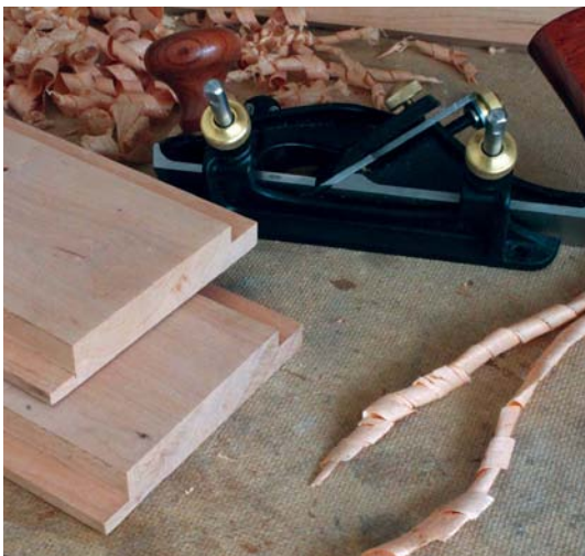
I cut out the rebates on the front edges before changing the blade setting for the rear rebates
