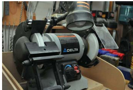
Variable speed 150mm grinder with cool wheels and a Veritas toolrest
