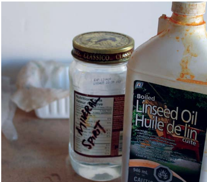
Mix the boiled linseed oil with mineral spirit in equal parts. Dispose of any oil soaked rags carefully as heat can build up and cause them to ignite
