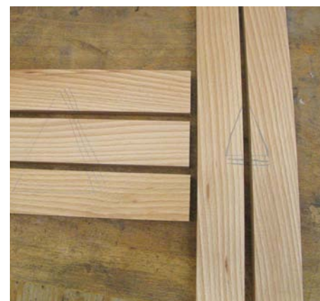
If there are several doors, drawers, etc. then number them by adding lines to the base or the side of the triangles – this is No.2
