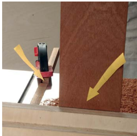
Keep an eye on the stop at the far end of the table and the line on the back of the board
