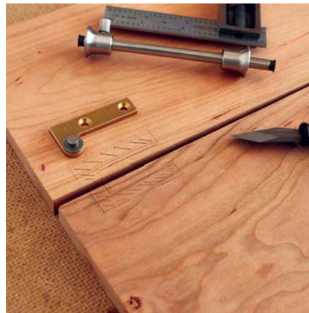
I transferred the scribed lines to the top piece using a marking knife and combination square
