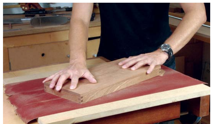
Use a sanding board to level the lid and base and don't stay in one place too long
