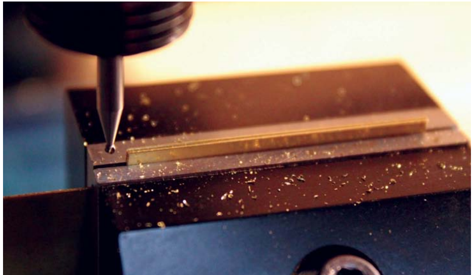
A curved profile was machined along one edge of each leaf to mate with the knuckle
