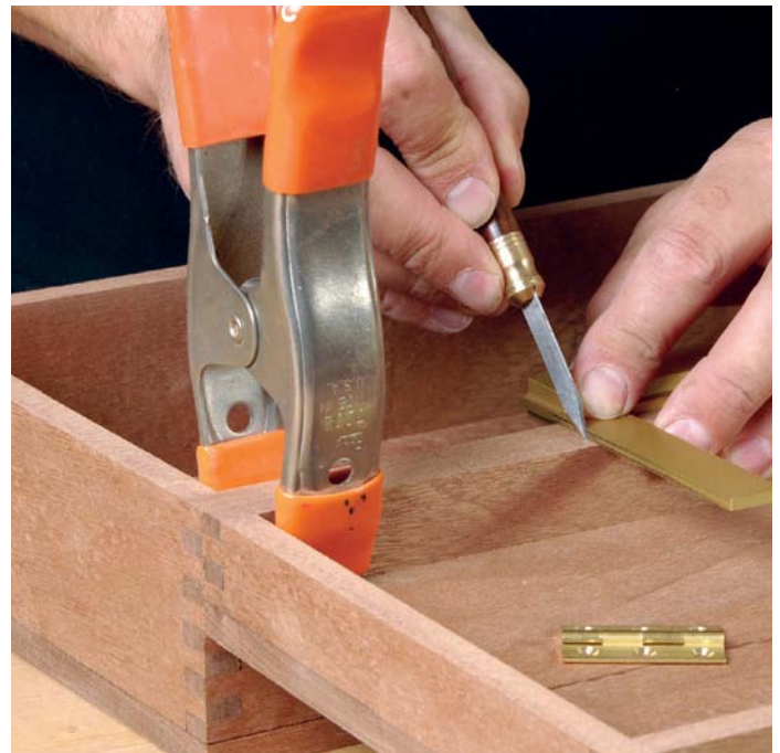
Mark out the walls of the hinge mortise
