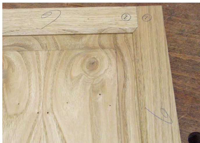
Numbering joints is a thing of the past with the triangle system
