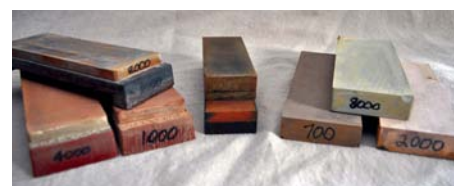
Quite a collection. The King 1,000, 4,000 and 8,000 that I used for many years on the left; a couple of oilstones in the middle that I've never used; my current favourites on the right, Bester/Imanishi ceramic waterstones in 700, 2,000 and 8,000 grits. The numbering will be explained in a future issue!
