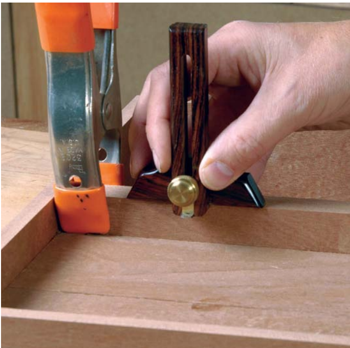
Mark a depth setting on the lid and base for the hinges
