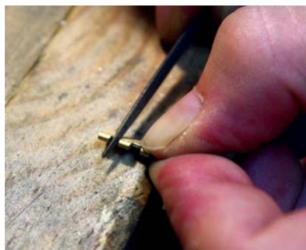
Some careful filing was required to finish the components
