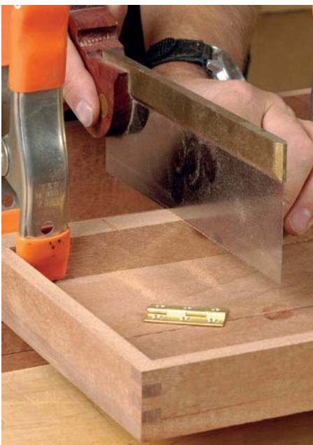
Gang cut the mortises
