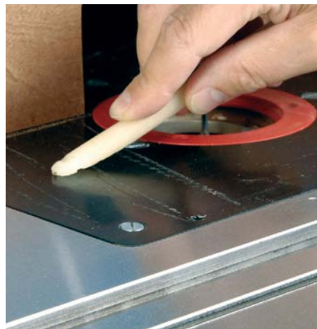
Waxing the table and the fence will make the box easier to manoeuvre over the cutter
