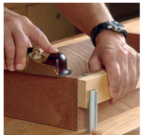
Trim the top and bottom edges of the box
