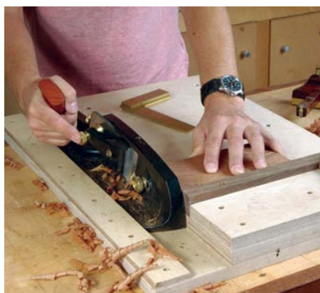
Shoot all four sides of the box to length and width plus a little extra
