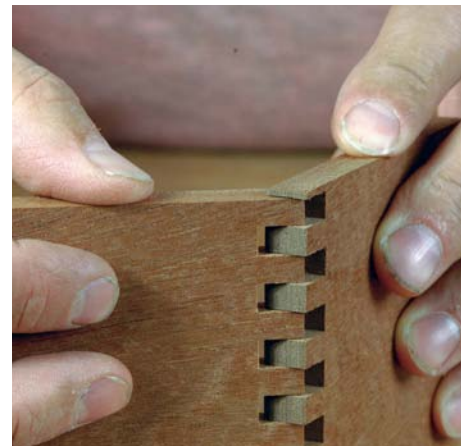
When you did your width calculation the extra material will combine into a half peg or thereabouts at the top and bottom of opposing sets of corners
