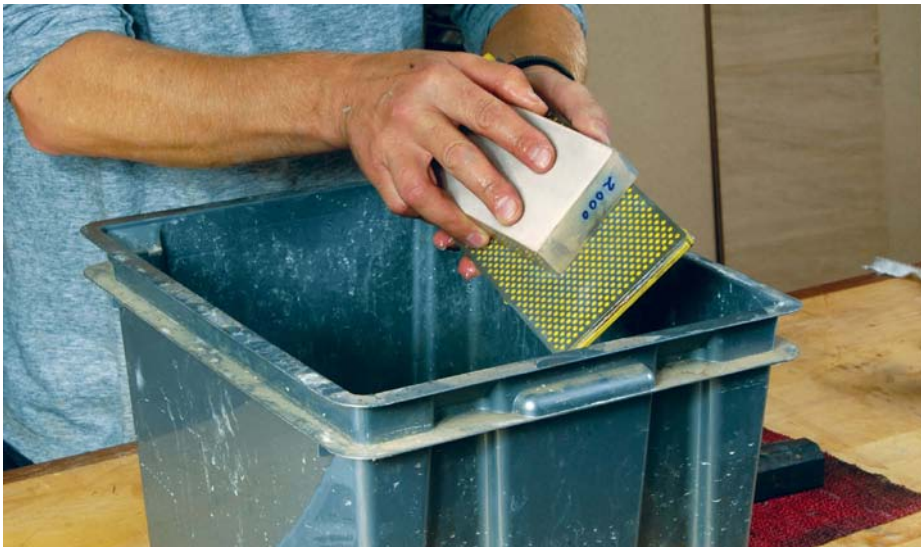
Use a coarse diamond plate to flatten your waterstones after every sharpening session
