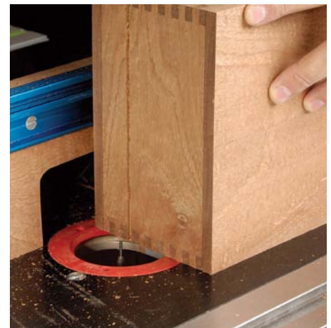
For a thin cutter make several passes
