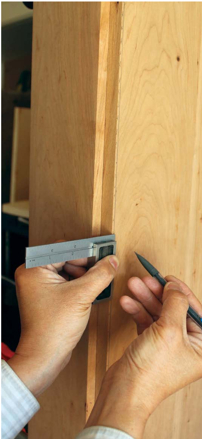
You need to assemble the cabinet with the oversized door in place and mark out the waste to be removed
