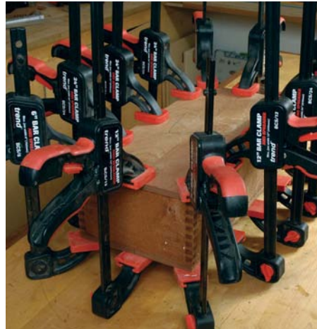
Use as many clamps as you can to create equal pressure around the box
