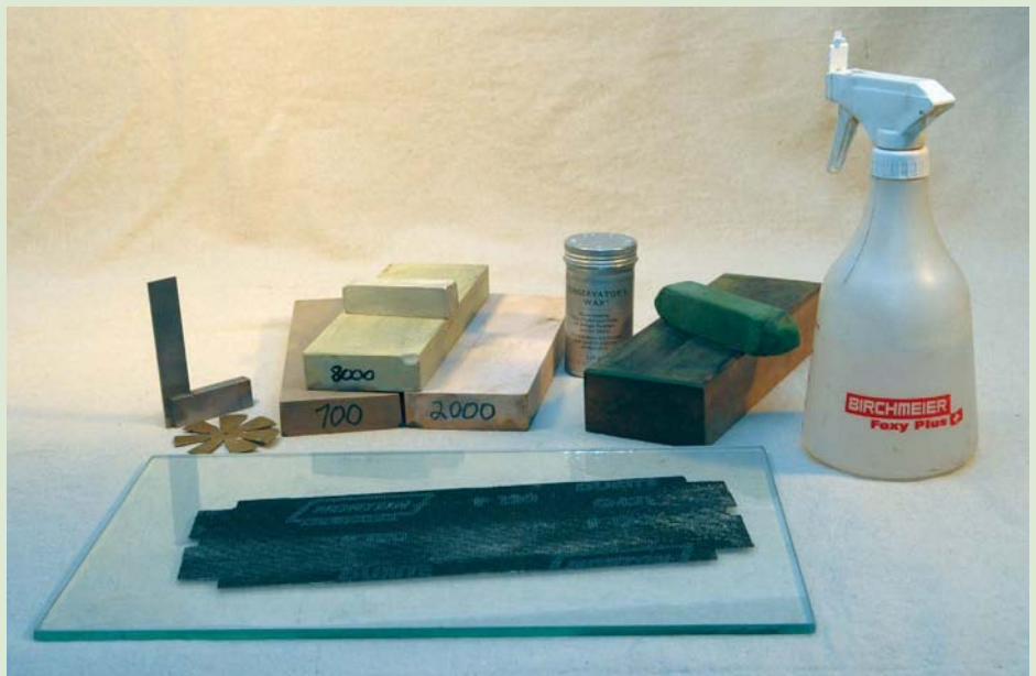
Add something for water and this is all you really need. In the front is a glass plate with drywall sanding mesh for lapping. A diamond plate is a versatile and more compact substitute. In the back is a small square and bevel angle gauge. My Bester stones with a small chunk of Nagura on top. Wax for lubricating and waterproofing. My maple strop with a bar of honing compound – chromium and aluminium oxide – and a spray bottle
