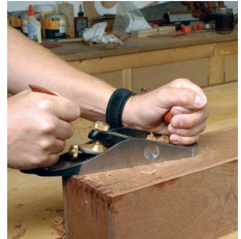
The extra depth of the finger slots will result in some material to plane off to square the box
