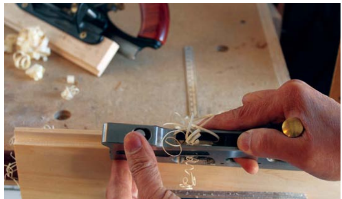
Round off both the tongue and the base with a shoulder plane or sandpaper
