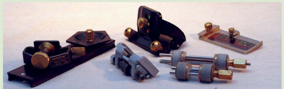
A meeting of honing guides. On the left is my venerable early Veritas model that I haven't used in years. Centre back is the Veritas MkII with its projection setting jig. These are both top clamping guides. Front centre is an eclipse-style side clamp guide that excels at narrow blades. At the front right is a pair of guides by Richard Kell
