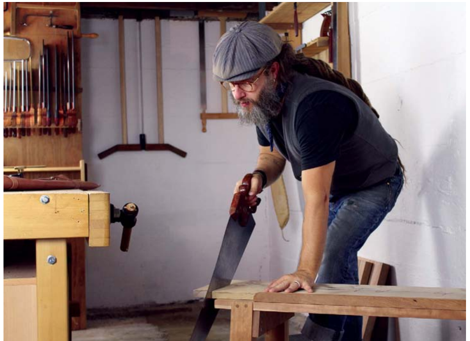
Breaking large stock down into manageable furniture parts. If you plan on using handsaws, you owe it to yourself to make a dedicated saw bench
