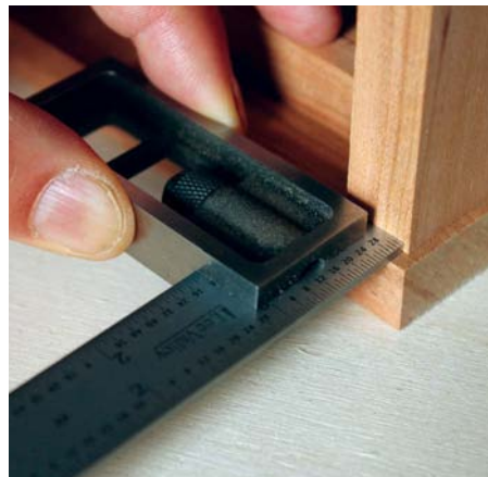
Measure the set-back distance and adjust the face of the marking gauge away from the wheel by the same amount
