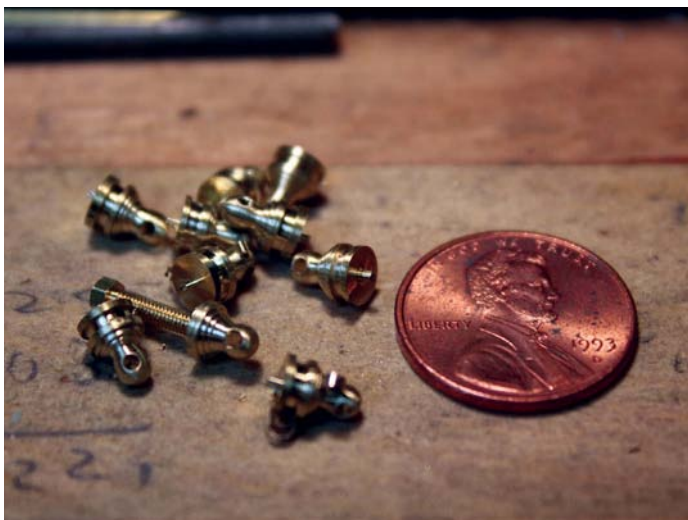
The individual bodies separated from the brass rod
