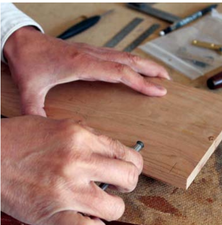
You can then mark the mortise on the bottom with the reset marking gauge
