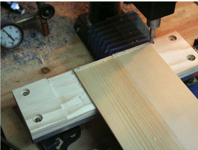
If you use a milling machine, a sacrificial clean carrier will protect the components
