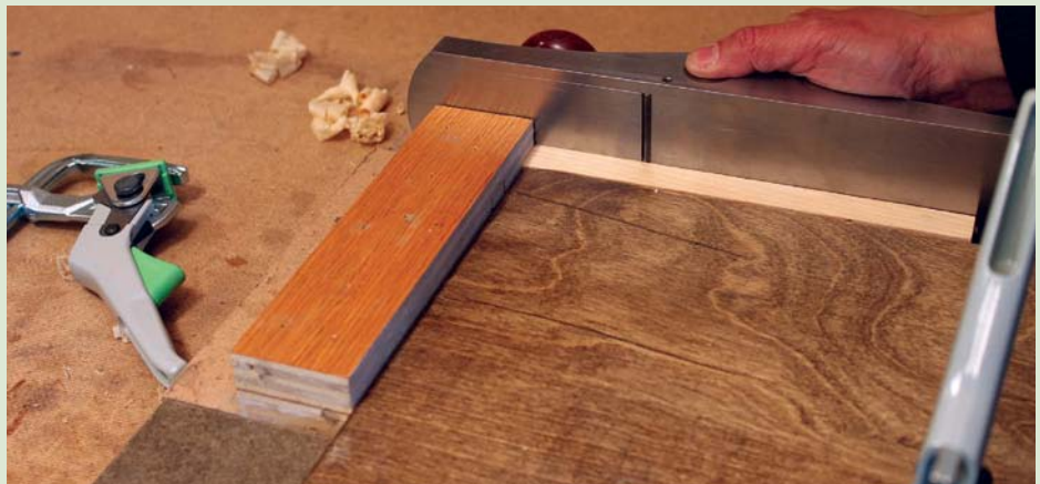
Trimming narrow, long edges with a shooting board
