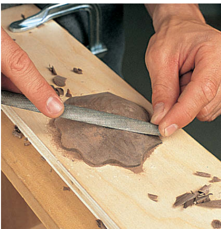
Step 15 after carving the contour, you can remove any remaining facets with a smooth file
