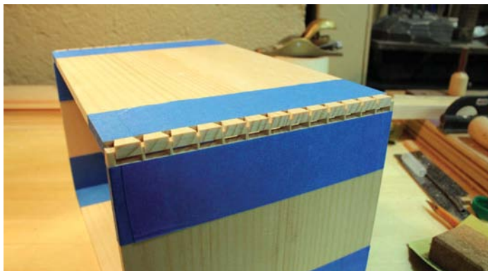
A low-tac masking tape will protect the surfaces from any excess glue
