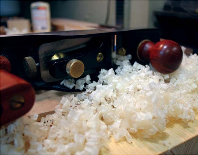
... using a shooting board and suitable shooting plane
