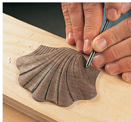
Step 27 use a No. 11, 1.5mm gouge to carve the veins
