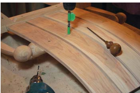
24 The back slats get fixed with a No.6 screw and then capped or plugged with wood
