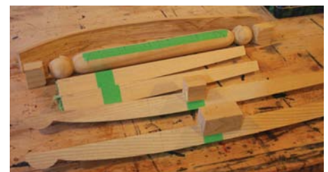
6 The front legs and back legs are a different length in an armless chair
