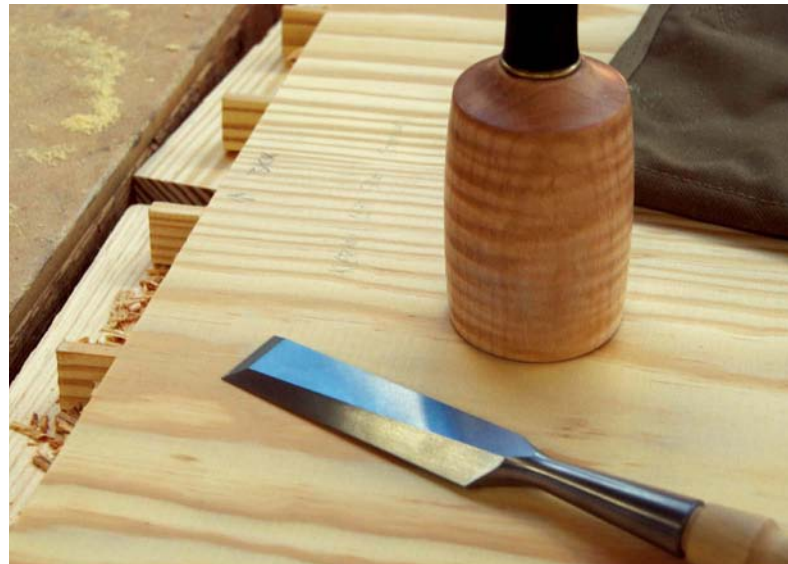
Using hand tools to cut the dovetails
