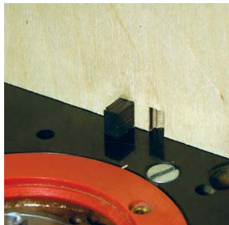
Make a trial pass into the faceplate to half the diameter of the cutter
