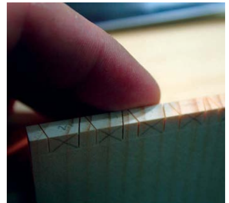
After transferring the outline of the pins, complete the tails and mark the waste
