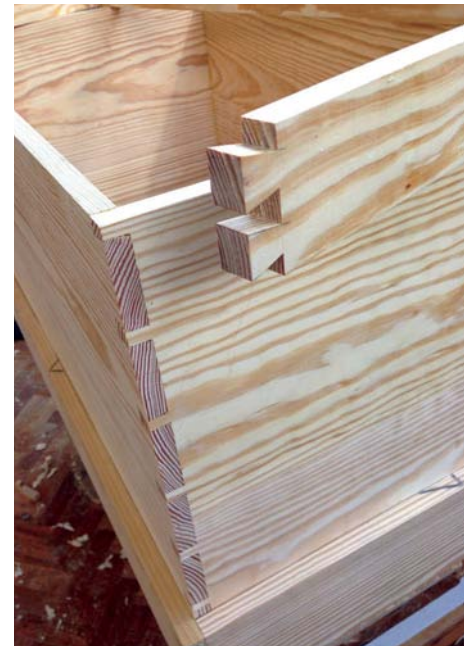
If the first set of dovetails you cut are this good and in yellow pine, everything else will be child's play
