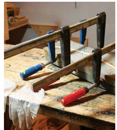
18 The jig is made from spruce or available softwood and two boards are glued and screwed together to get 76mm thickness
