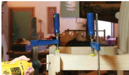
23 The counter-bored screw gets a wood cap or plug
