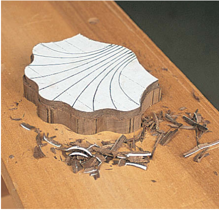
Step 9 the entire outline will later be inverted to become the base of the shell
