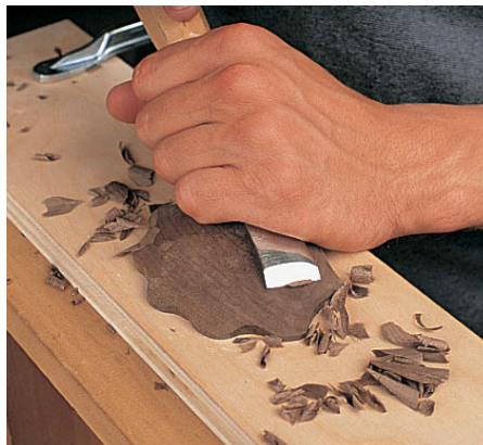
Step 14 use a No. 2, 25mm gouge to shape the contour, producing sweeping curves from left to right
