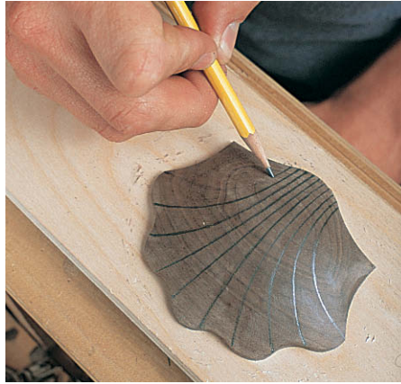
Step 18 connect the points by sketching smooth, flowing curves
