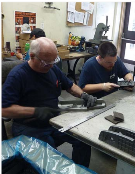
Rough castings of the Veritas shooting plane having the edges knocked off before heading off for machining
