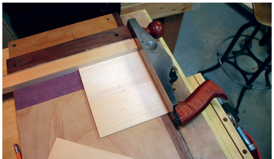
The process for preparing stock for jointing in miniature is similar to that of full scale work...
