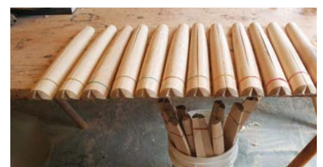
7 Legs are paired in order to match the grain
