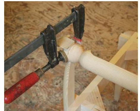
16 I do a dry fit first and make sure the back slat fits flat to the angle of the bandsaw cut
