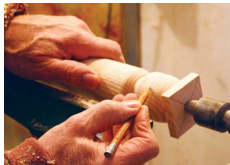
12 The pencil line at the peak of the sphere is retained even after sanding the finished rail
