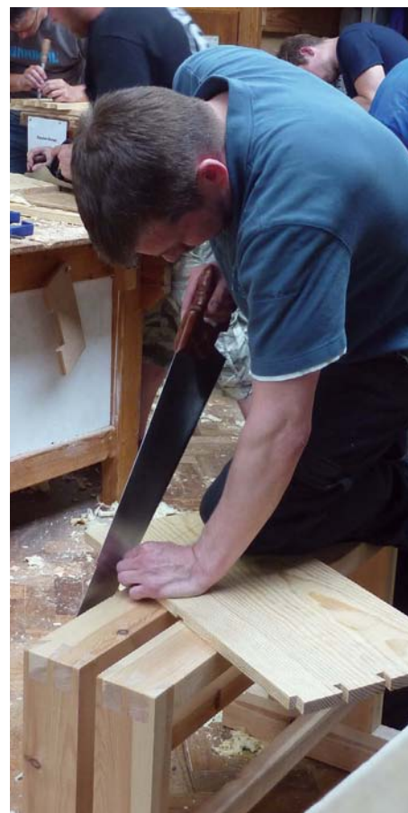
Hand tools only. Ed Sutton cuts the sloping sides for his Dutch chest
