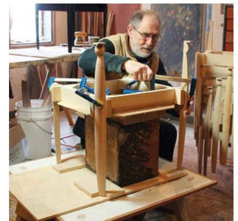
10 The gluing of the legs and seat frame is set up on a baseboard
