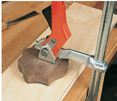
Step 12 clamp the shell to the board and allow the glue to thoroughly dry
