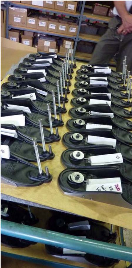
A partly assembled tray of No. 4 1/2 bevel downs with the paperwork that will stay with the tool until it's packaged for distribution
