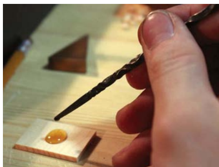
Don't apply glue straight from the pot – you can't control it and it will dispense much more than you need
