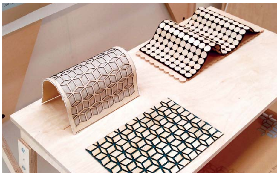
Samples by Laura Krumina of Birmingham City University made using laser cutting and CNC machines
