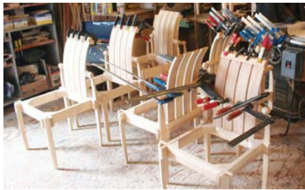
21 The rail at the top of the chair is glued on later to the back of the chair
