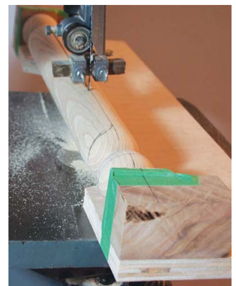
14 Green tape secures the back rail into the jig and this is where I appreciated having the square block on the end of the turning
