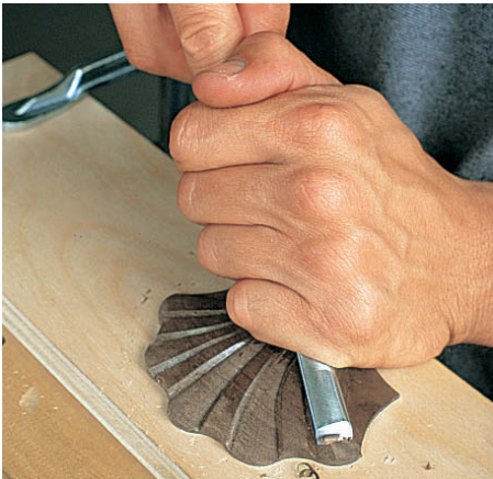
Step 23 to carve the convex lobes, start by contouring the ends of the lobes with a No. 5, 12mm gouge
