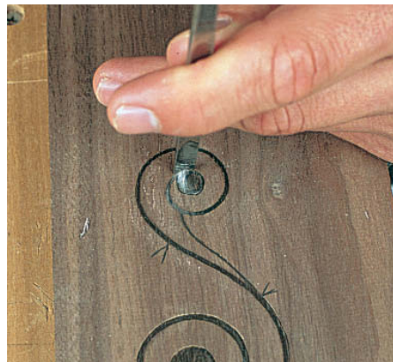
Step 5 beginning with the centre hub, incise the outline of the volute with the same series of gouges that you used to incise the template
