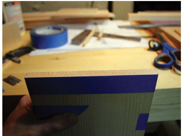
Gang cutting components is a good way of introducing consistency
