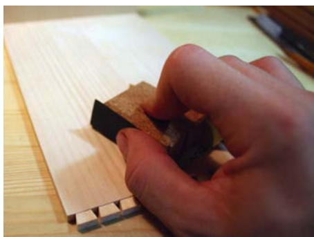
Using fine abrasive stuck to a cork block with double-sided tape will allow you to clean up the interior faces
