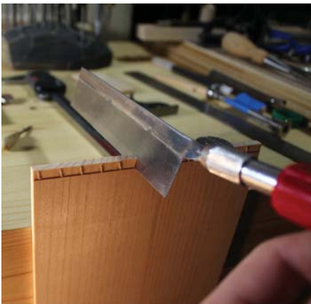
Cut shy of the baseline using a fine-bladed saw
