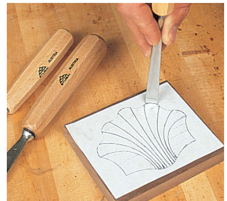
Step 4 for the lobes on this shell, use a No. 7, 14mm gouge
