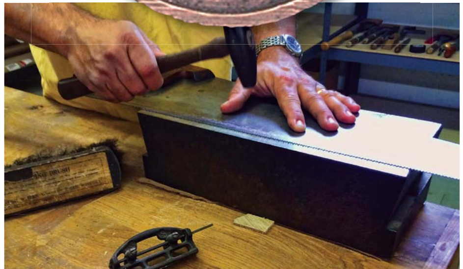
Hammer-smithing a vintage Disston sawplate back into true
