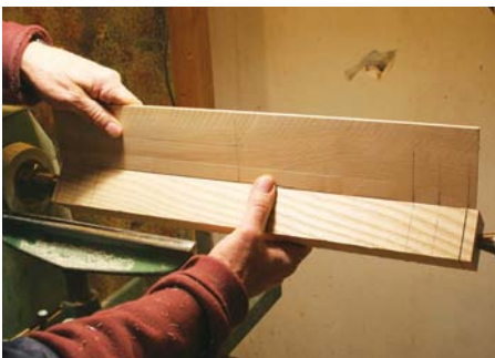
11 I mark out exactly where the sphere will go on the back rail
