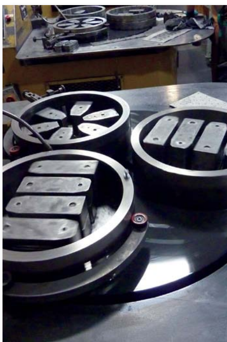
When a Veritas blade is lapped flat, anything you do to that surface afterwards makes this machine a waste of time. Don't do it
