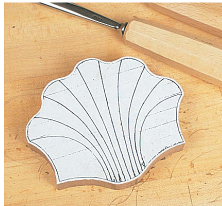
Step 5 saw approximately 1.5mm from the line because the final outline of the shell is created with carving tools
