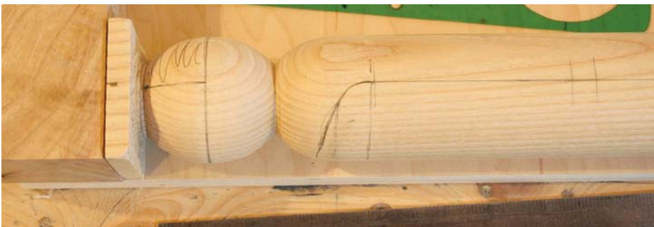
13 I then mark out where the back rail of the chair is cut
