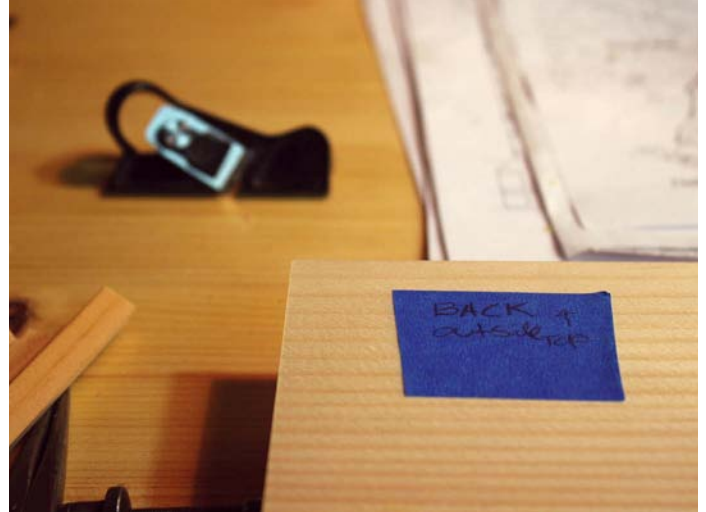
Identifying the components is best done with labels rather than risking damaging the surface of a delicate material, such as white pine
