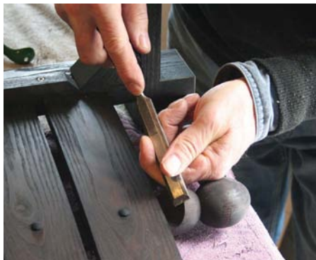
28 The chamfer took off the corners and it also has the benefit of looking good
