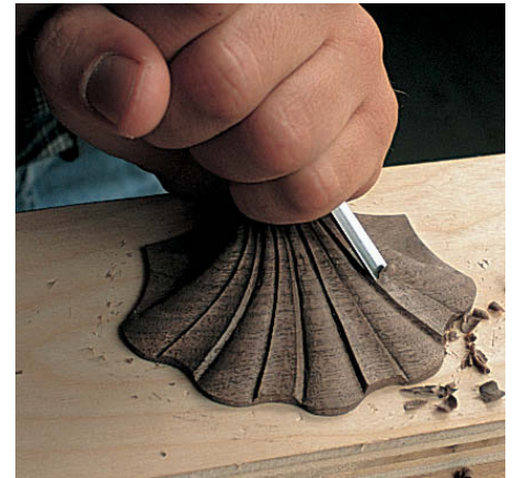
Step 25 ...as you carve the rays and lobes, use the gouges to blend the curves
