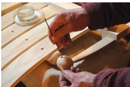
25 Dowelling the super egg is not essential but if the glue should fail the dowel still holds it together
