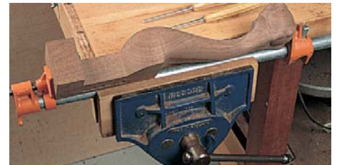
You can use clamps mounted in a vice to hold complex shaped carvings
