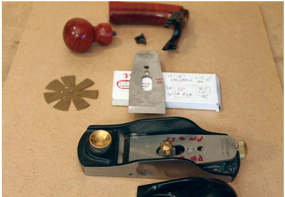
Increase the cutting angle of a low-angle block plane to 45° with a 33° blade
