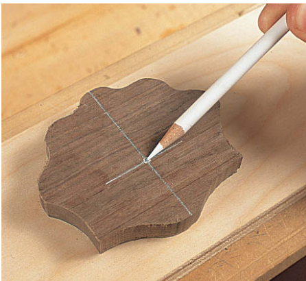
Step 13 mark the high point of the contour before you contour the face of the shell
