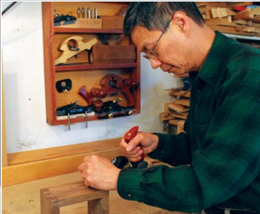
A low-angle block plane used like a No.3 smoothing plane
