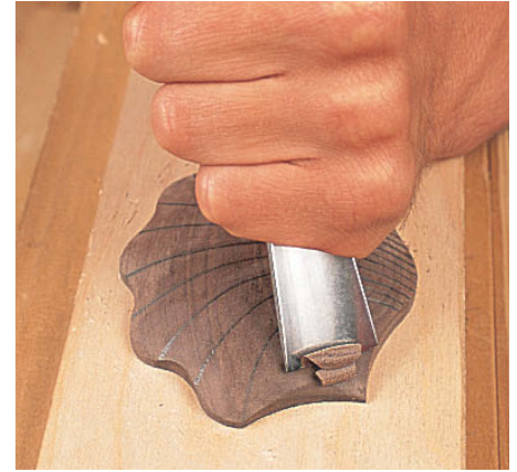
Step 19 to incise the hinge area, hold a No. 5, 25mm gouge nearly vertical to create a steep wall...
