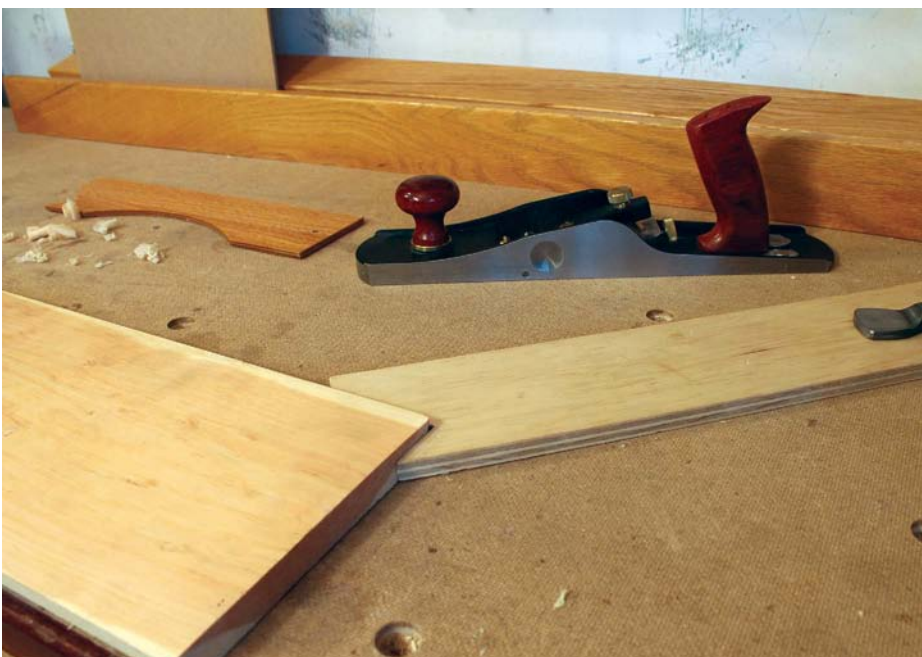
With the stock locked in the notch, you can plane across or towards the front of the stock
