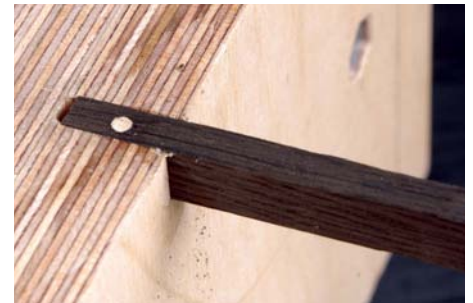
Fix the peg in place with glue, dowel or screw
