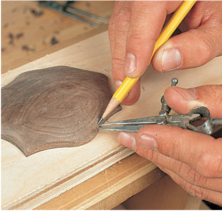
Step 17 ... you can then divide the base of the shell into equal spaces
