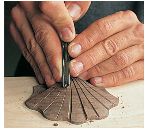
Step 22 as you carve the Vs, watch the spacing and flow of the curves
