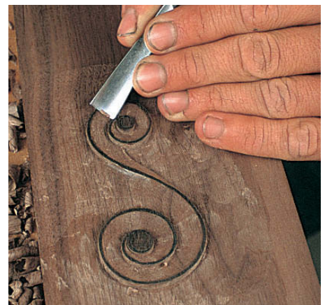
Step 9 use a No.3 gouge and take sweeping cuts around the volute to remove the facets
