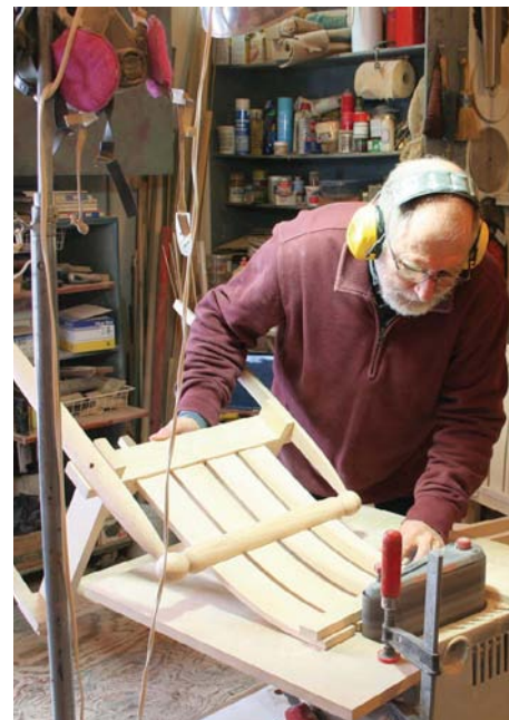
26 The chair is hand sanded, keeping most of the edges square as they will get a chamfer later
