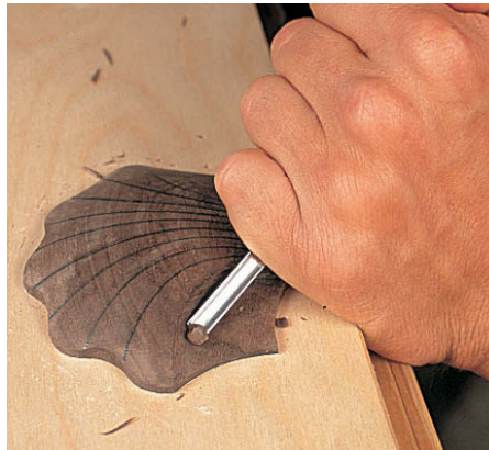
Step 21 take long, sweeping cuts to blend the wall with the hinge area
