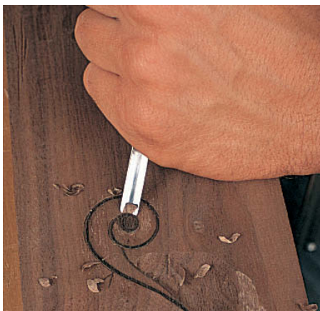
Step 7 make a second series of cuts that intersect the first cut at a shallow angle
