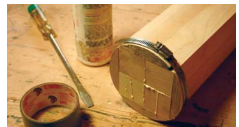
5 The legs are made from four turning blanks which are 38mm square
