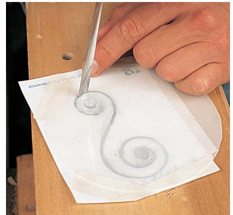
Step 2 draw the design on paper, then position a transparent plastic sheet over the drawing
