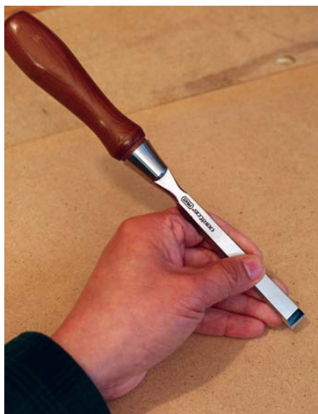
The little finger rests with the palm on the work, steadying both the hand and the chisel
