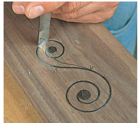
Step 6 as the curves become broader, use wider gouges with less sweep
