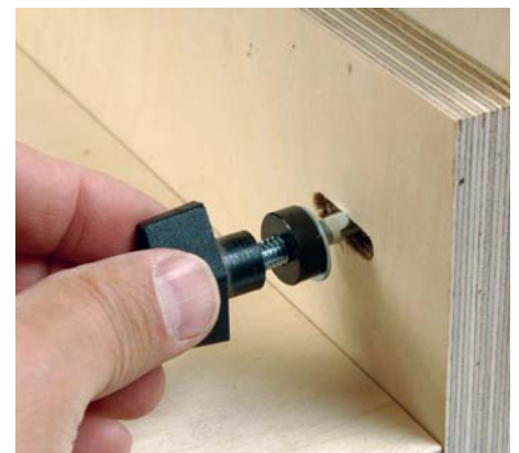
Use easily adjustable nuts to secure the faceplate in place
