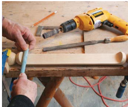
15 Cleaning up the bandsawn surface using files and drum sanding
