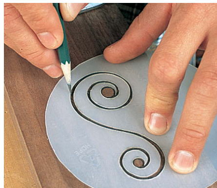
Step 3 trace the template onto the stock...
