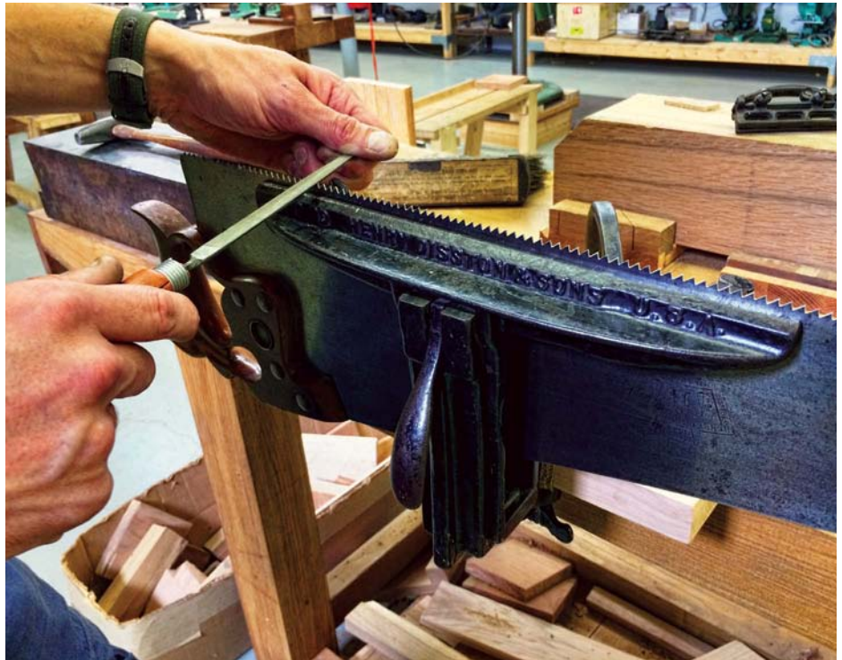
Sharpening a Disston D8 from the 1887-1896 era
