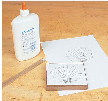
Step 3 glue a copy of the drawing to the stock for the shell
