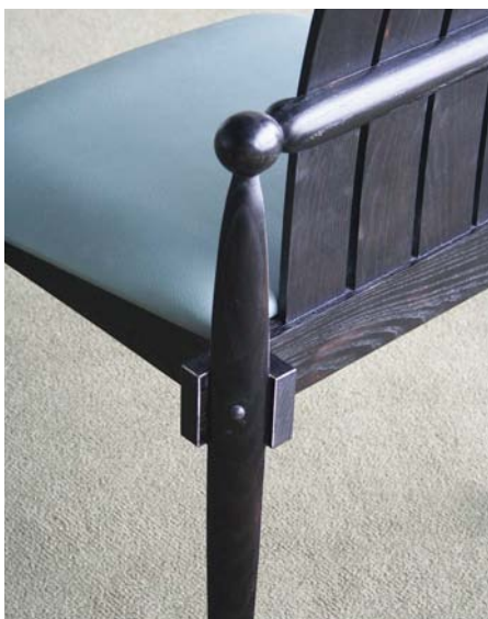
4 Fundamental to the design of the chair is the cross-halving seat
