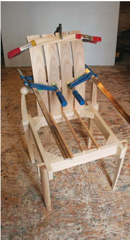
20 The slats are glued on and the clamps left overnight
