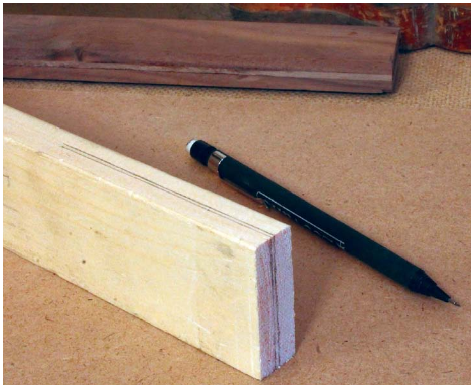
Sawing between two parallel lines gives better results
