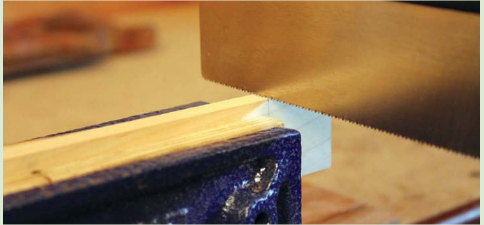
Tilt the saw blade side to side until the edges in the reflection line up straight with the actual edges
