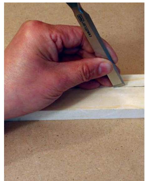
Place the corner of the chisel on the line and then roll the edge down, guillotine-fashion
