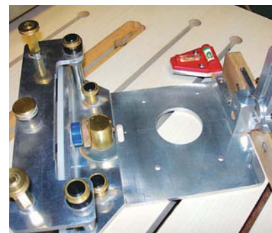
The router baseplate is drilled to match the router fixing holes for a conventional router table
