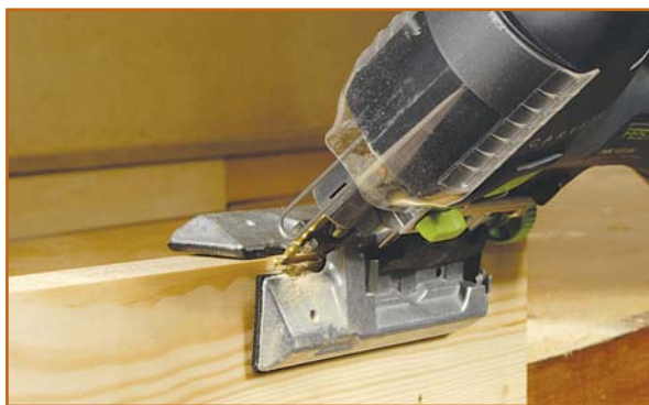
The sole of the bevel cutting baseplate can be adjusted to give support in both planes
