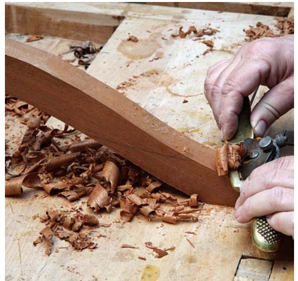
9 After cutting to shape on the bandsaw, curves of the back post or stile are faired smooth with a spokeshave
