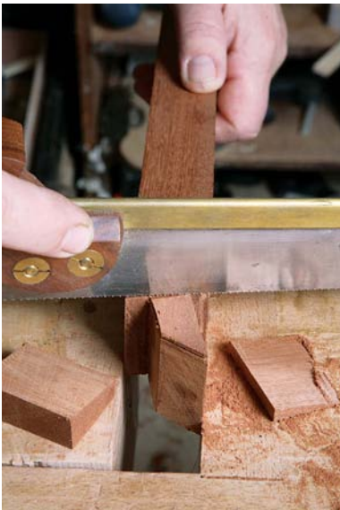
7 The tenon shoulders are similarly hand sawn following the angled lines
