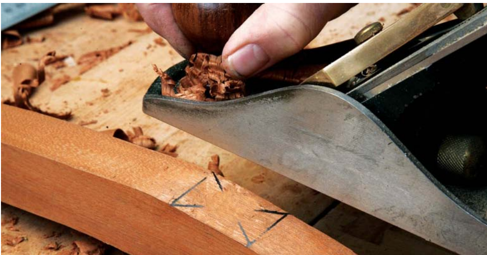
10 The position of the rail joint on the curved post is marked out then planed flat
