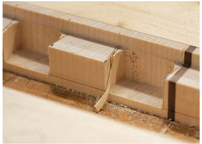
5 Time spent setting up the router depth and backstop is rewarded with waste removed accurately to the line and very little left to chop out by hand
