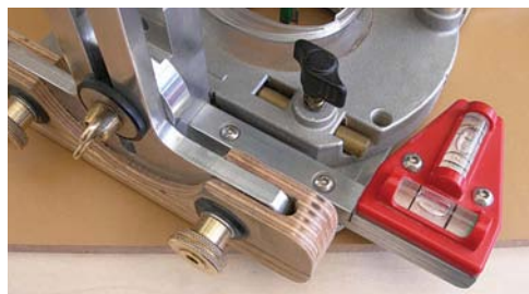
To ensure square cuts the table has to be levelled and the router calibrated similarly. The fine adjuster can be moved laterally by 0-15mm; this allows the router to be adjusted without losing its fixed reference
