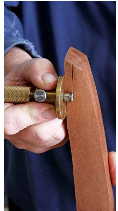
15 The top of the post is marked out with the depth of a sliding dovetail to attach the crest rail
