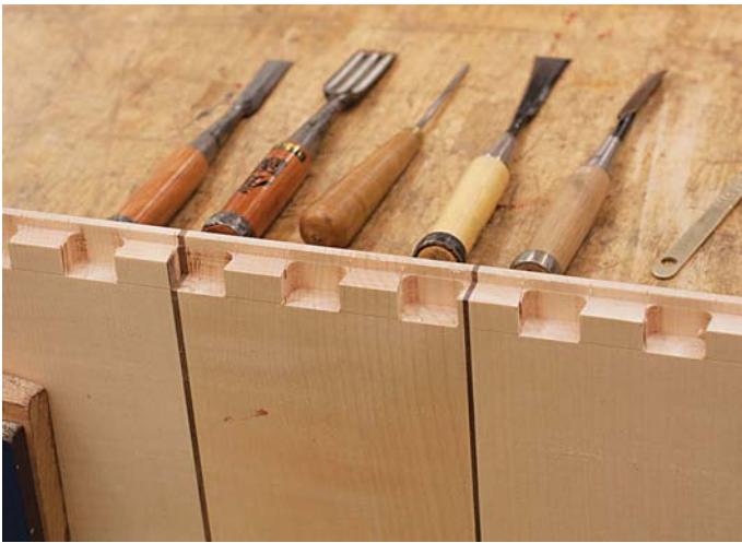
4 Long secret mitred dovetails are a demanding technique. Creation of the vulnerable mitre is left as late as possible to limit the risk of damage
