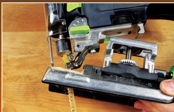
The separate baseplates attach to the body using a quick-lock system
