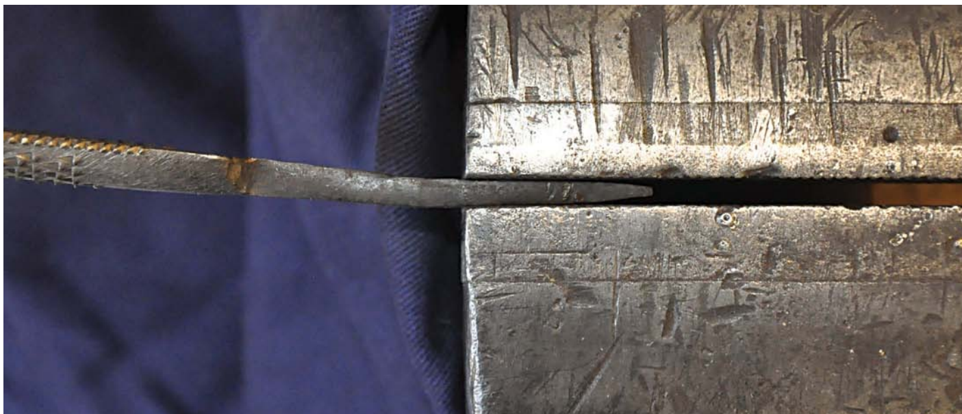
Straightening the tang of a 4in Parkinson's rasp held in an engineer's vice
