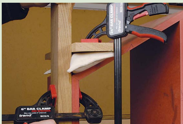
Use a sandbag to fill the void between pressure blocks on angled joints
