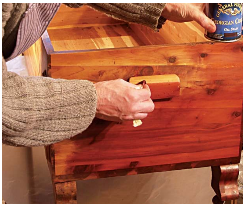
Applying the stain with a rag folded into a brush shape
