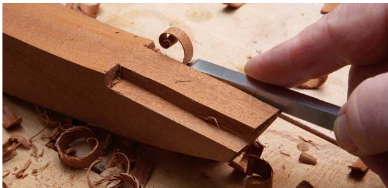
17 The sides of the sliding dovetail are pared out with a bevel edged chisel
