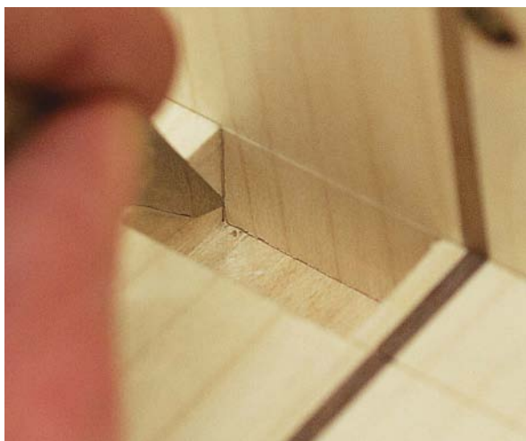
8 Scribing the tails is a little awkward but a sharp, fine scalpel helps
