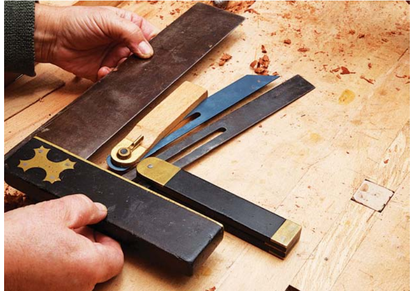
2 Two angles adding up to a right angle are known as complementary angles – shown here by two bevel gauges fitting together between the stock and blade of a try-square
