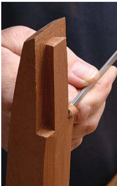
18 The shoulders of the sliding dovetail on the top edge of the post are cleaned with a fine chisel
