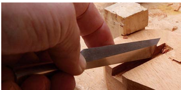
21 Waste is chiselled out from between the two saw cuts so the crest rail housing can receive the sliding dovetail
