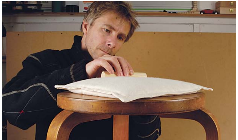
Distribute the sand evenly across the area
