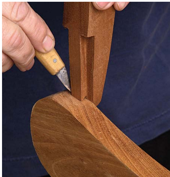
19 The end of the sliding dovetail on the post is used as a template to mark out the housing that will receive it
