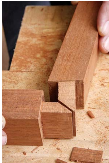
8 A finished angled tenon on the side rail (top) butts up to a straight tenon on the back rail (left) in a mitre which will be hidden in the mortises
