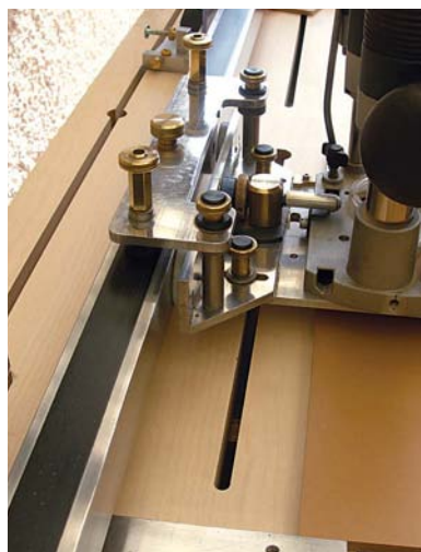
The router is cradled in a baseplate and suspended from a reference fence
