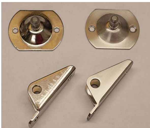
14 Gas strut mounting plates before and after fettling with files and emery paper
