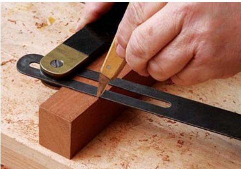
3 Tenon shoulder lines on the chair's side rails are marked at an angle corresponding to the splay of the seat
