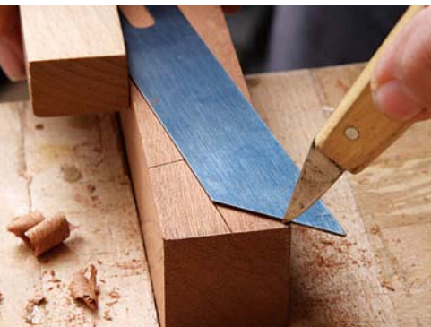
5 This bevel gauge has a 45^\circ end, making it easy to mark the mitre angle on the tenon
