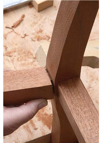
13 Both tenons insert straight into their sockets although the side rail (left) is at an angle to its tenoned end
