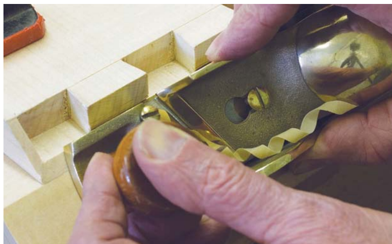
9 An accurately machined 45° block attached with double sided tape and clamped in the vice with the work makes forming the mitre a pleasurable job
