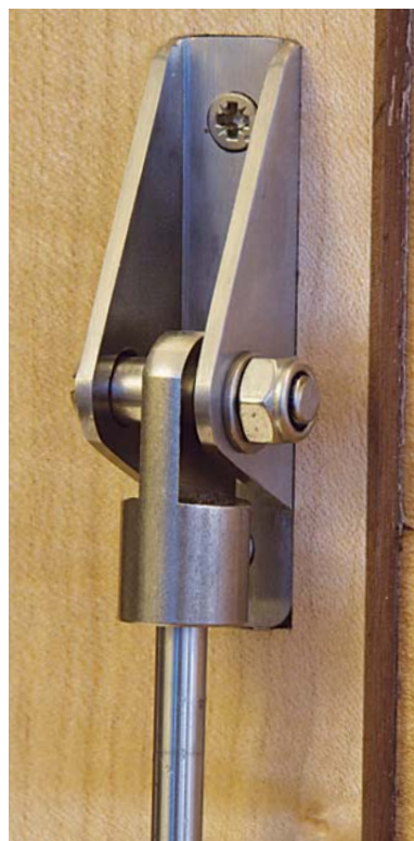
15 Top strut mounting brackets are mortised into the lid frame to reduce their obtrusiveness
