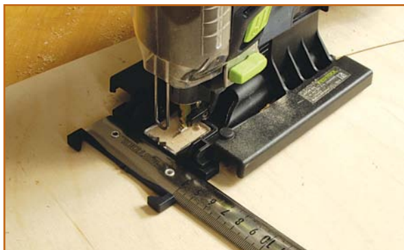
The trammel bar works off a centre point to cut near perfect circles
