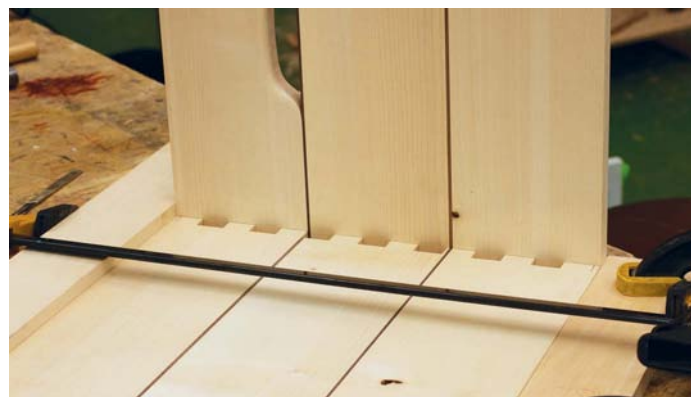
7 The end panel set up for marking the tails from the pins. Clamped-on stops ensure that the string lines are perfectly aligned
