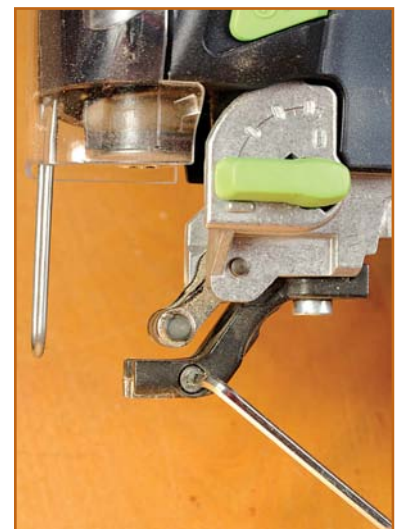
A new support wheel has been placed above the blade guide which needs adjusting to fit each new blade
