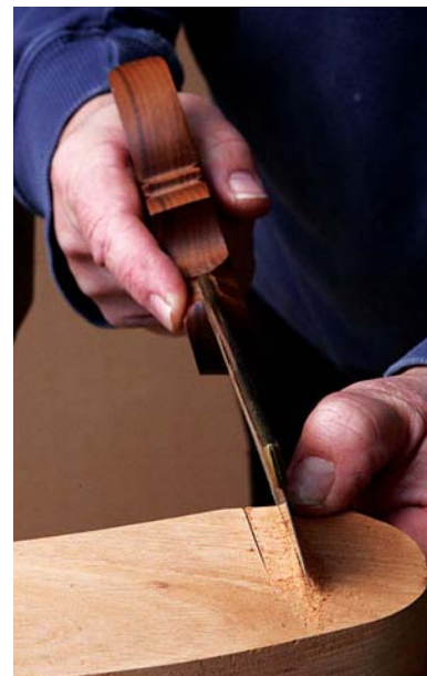
20 A pair of cuts is made in the back of the crest rail with the saw tilted in each direction forming the sides of a housing
