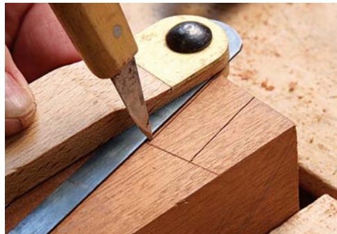
4 The side cheeks of the tenon itself are marked at the complementary angle to the shoulder lines
