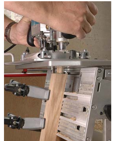
Instead of hand sawing angled tenons they can be machined with a router jig
