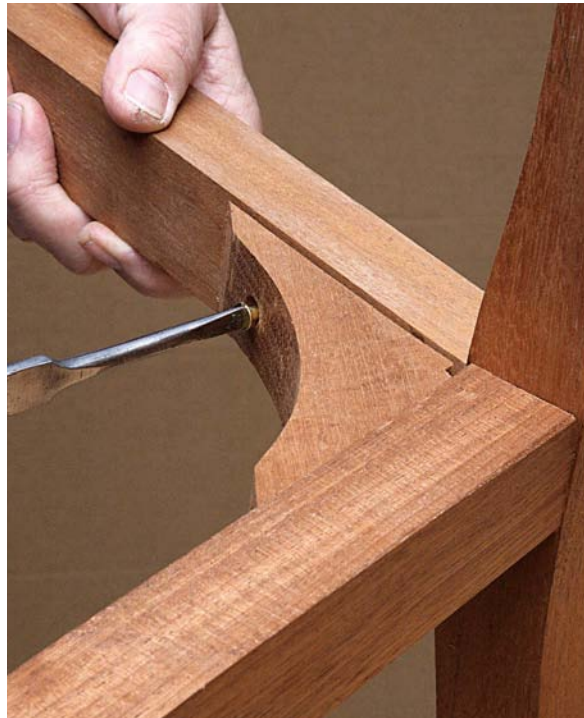
14 A corner block is shaped to match the angle of the splay of the seat
