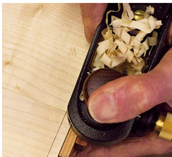
11 Forming the tongue on the divider with the Veritas skew block plane. An extended wooden fence is screwed to the standard fence to give a longer bearing length
