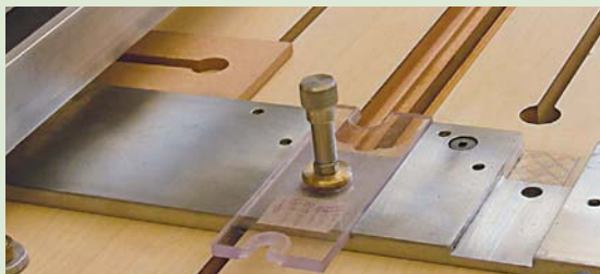
Cutter reference guides are used to identify the outer edge of the tooling. These are housed in a purpose made groove within the squaring fence
