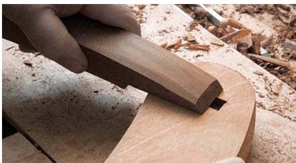
22 The tapered key slides into the matching socket to secure the crest rail
