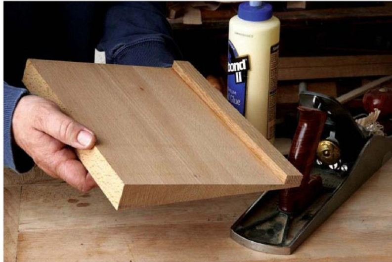
A sloping platform cut to the same angle as the dovetails
