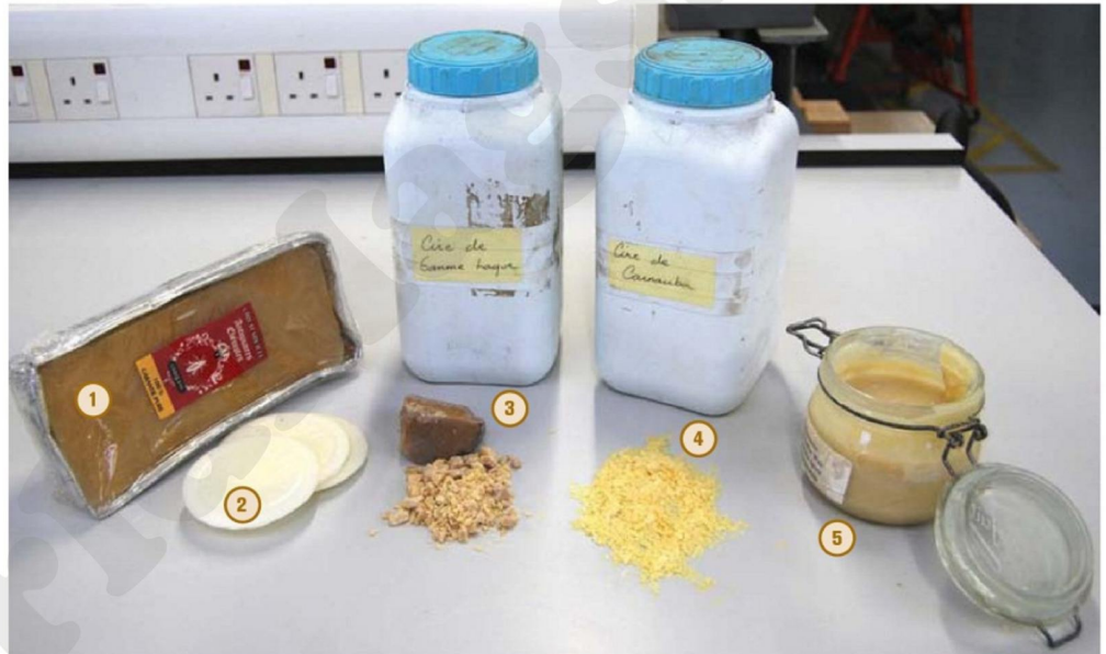
A block of brown beeswax (1); biscuits of high quality white beeswax (2); shellac wax (3); carnauba wax (4); the mix is stored in an airtight container (5)
