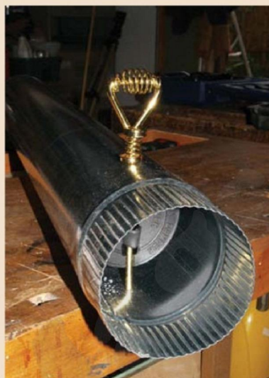
This is the flue damper in position. Drilling holes are easy but wiggling the spindle in is a bit of a fiddle
