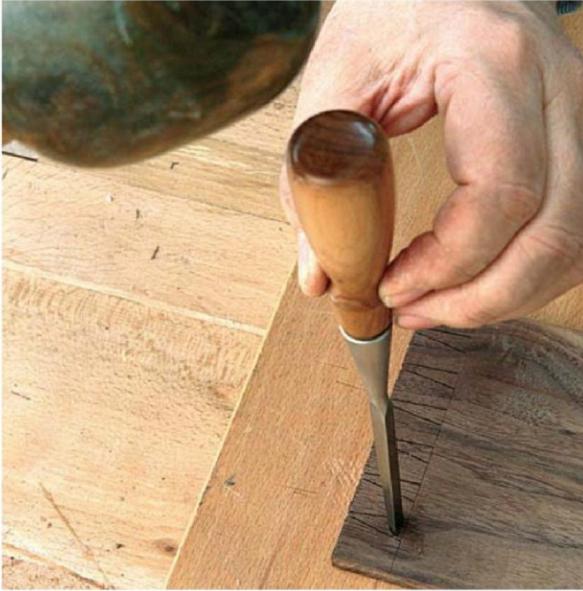
Make an initial cut a millimetre or more away from the shoulder line from both sides
