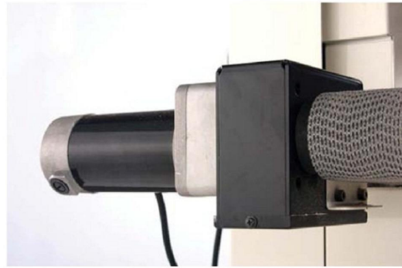
The drive for the belt is in a slightly vulnerable location
