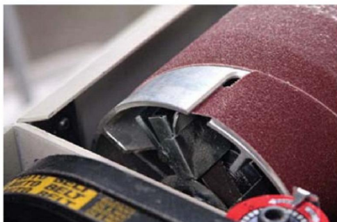
Self tightening clamps hold the abrasive sheet in place on the drum
