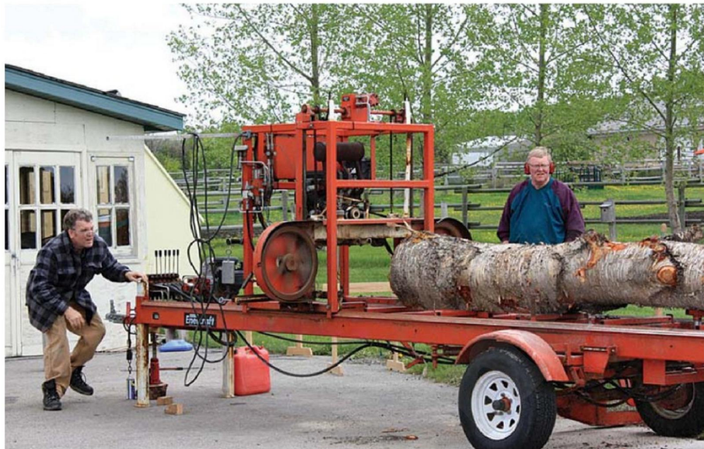
A portable saw mill was used to convert the logs into planks at Andy's workshop
