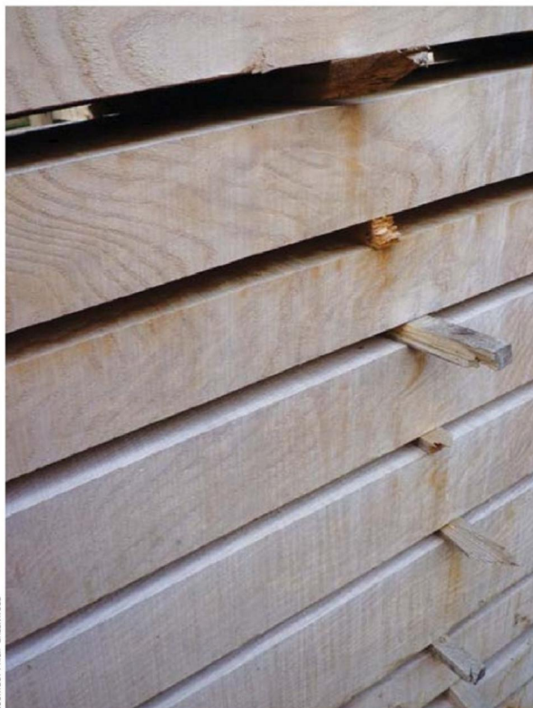
Sticks placed between planks of timber to allow air flow
