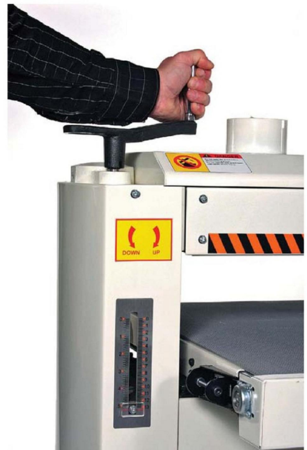
The bed is raised and lowered by a single wheel
