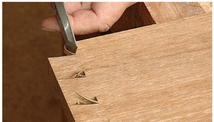
To ease a tight joint create a small chamfer on the edges where the two pieces come together
