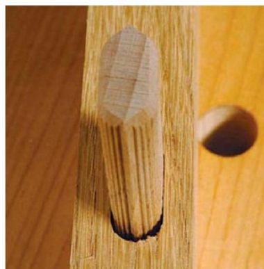
The wide slot setting allows 2mm of play side-to-side
