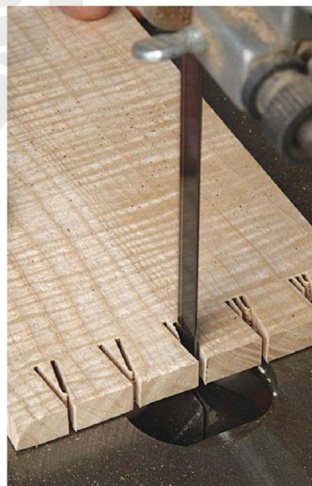
Use the blade to nibble away at the waste
