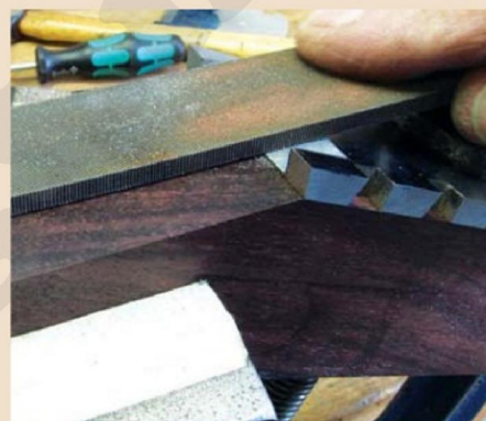
Once again a block of hardwood cut to the right angle makes a great platform from which to gauge progress
