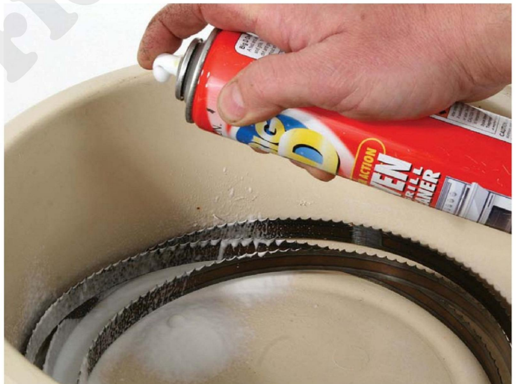
Oven cleaner can be used to soften resin build-up on your blade
