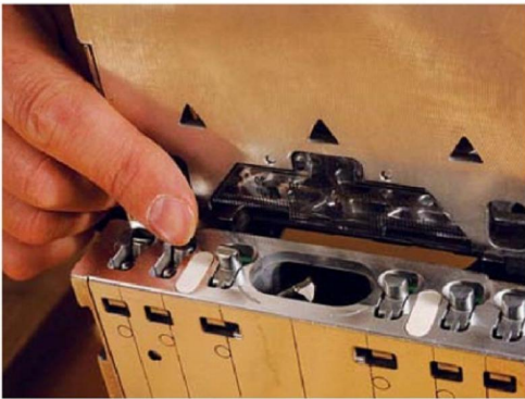
The quick set stops can be pressed into the base plate. A visual guide is etched into the base for quick reference
