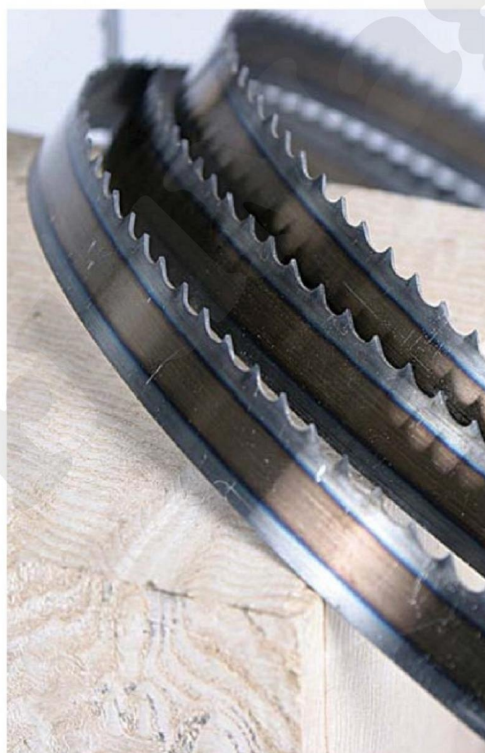
Wide thin gauge blades like these from TuffSaws are easier to tension on smaller machines
