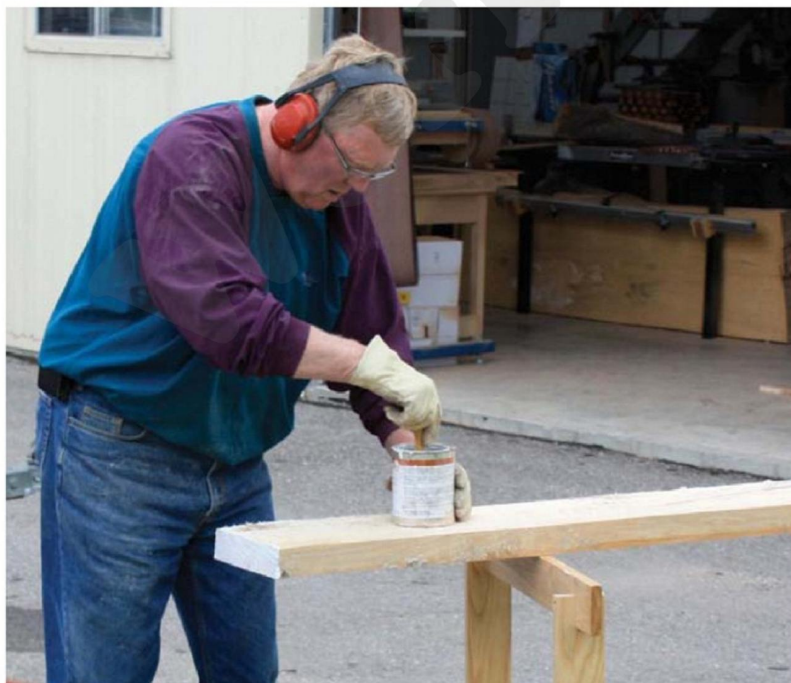
Before loading the planks into the kiln the ends were sealed with an emulsified wax to slow the drying process down
