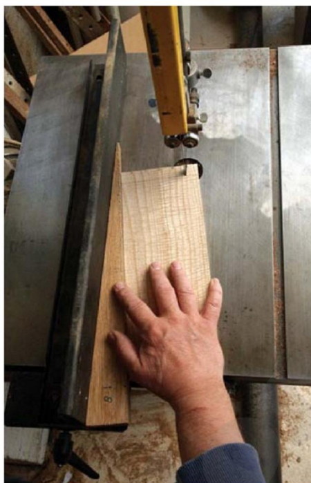
Wax the edge of the wedge that meets the fence
