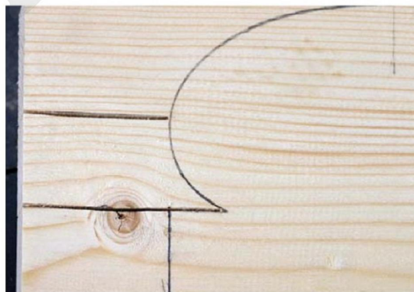
Release cuts are a must for intricate shapes and tight curves
