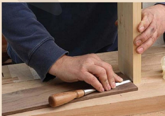
Save time marking shoulders for your dovetails by registering them directly off the material.
