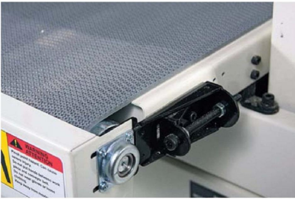
Controls either side of the belt are used to adjust the belt tracking
