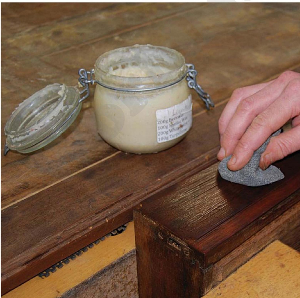
A soft cloth dampened with white spirit makes applying hard wax a little easier
