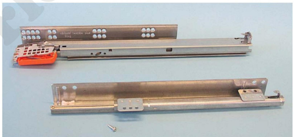
At the rear is the Blum Tandem Plus runner, and at the front is the Quadro Concealed Drawer Runner; it requires a hole in the back of the drawer, and a plate to be screwed on to the bottom of the drawer
