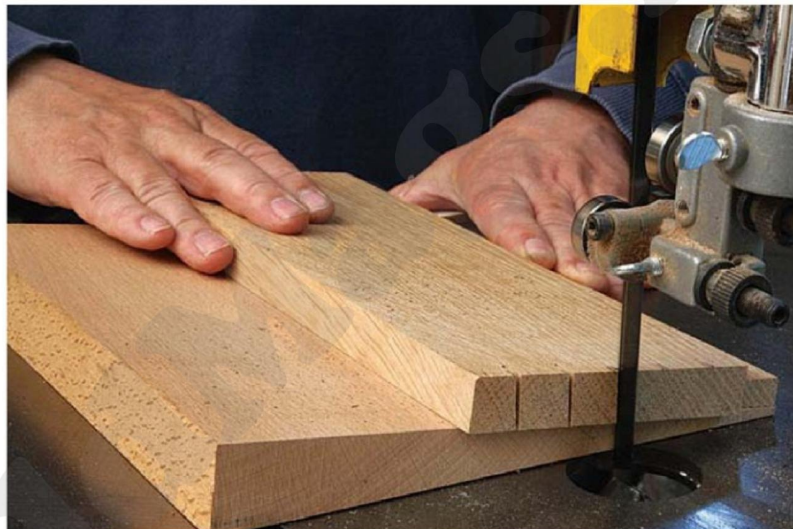
Begin the sequence by cutting all the same sides of the pins
