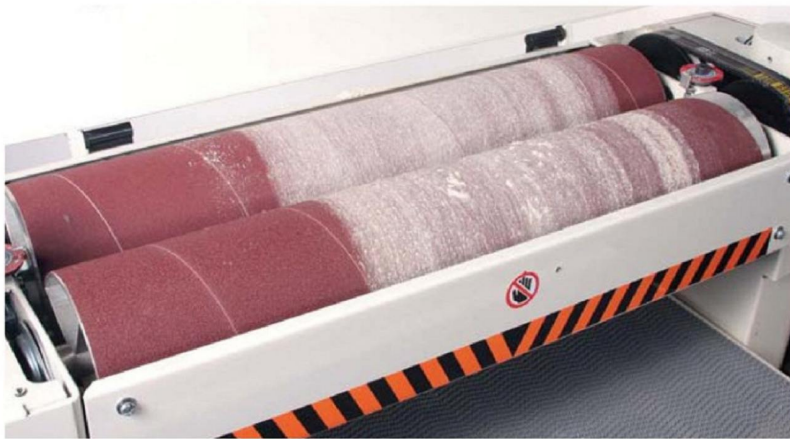
Abrasives are wound round the cast aluminium drums
