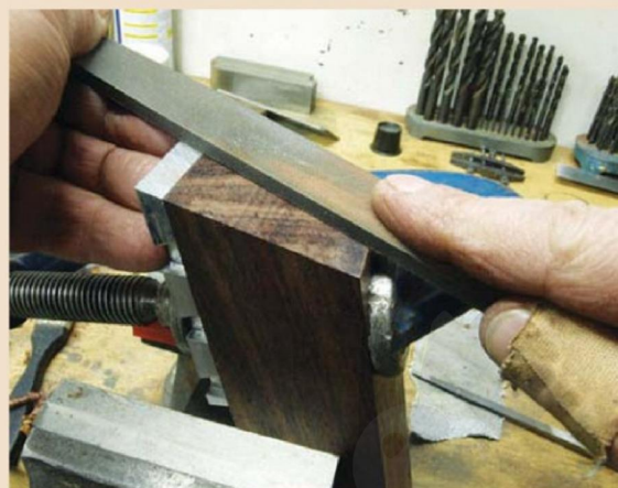
Filing the correct angle of the opening accurately is best done using a hard wood block for reference
