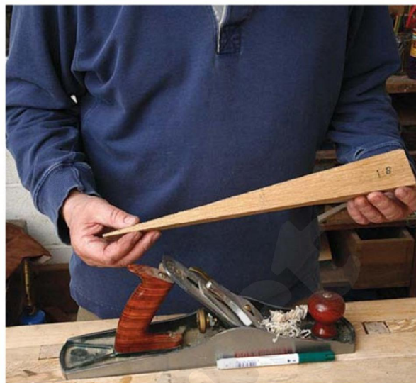
Hardly a jig but a wedge of timber will save you time cutting dovetails on the bandsaw
