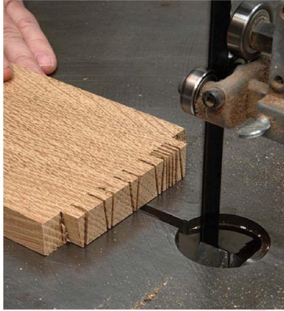
Divide the waste up into thin sections on the bandsaw before continuing to chop out with a bevel edged chisel
