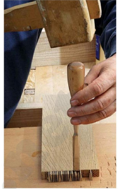
Divide the waste up into thin sections on the bandsaw before continuing to chop out with a bevel edged chisel
