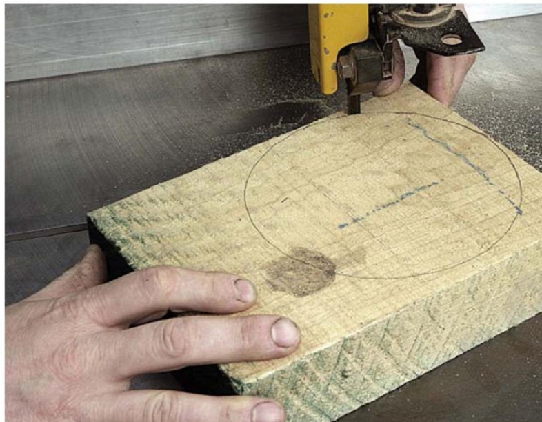
Repeatedly cutting turning blanks will knock the set off one side of your blade
