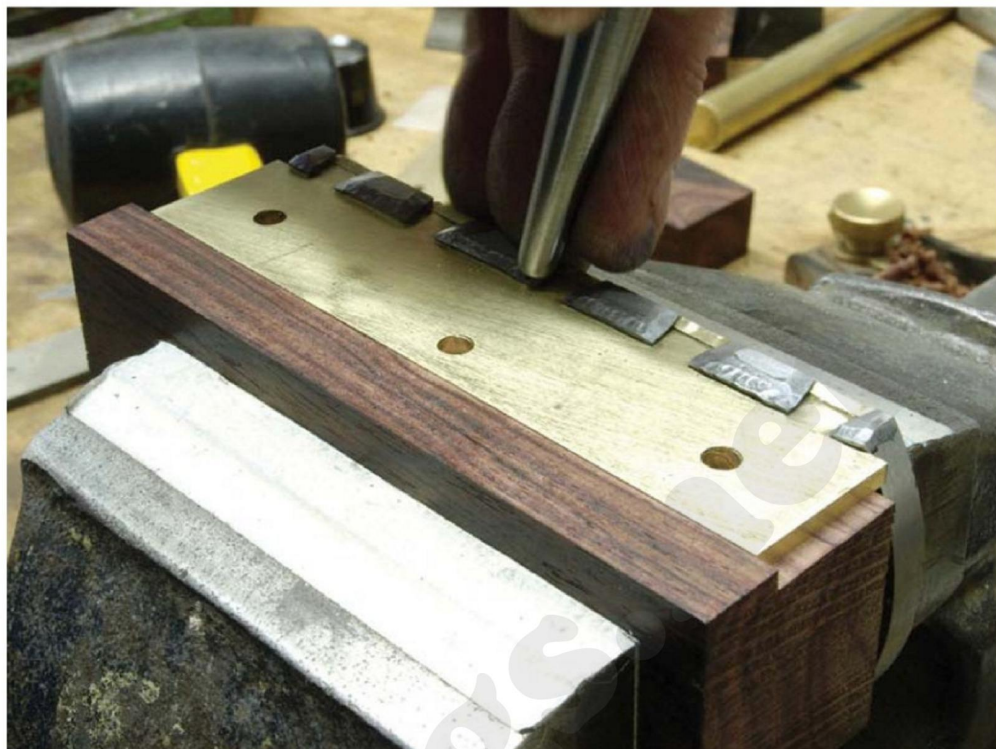
A block of wood prepared to the thickness of the infill is used to support the sides during the peining process
