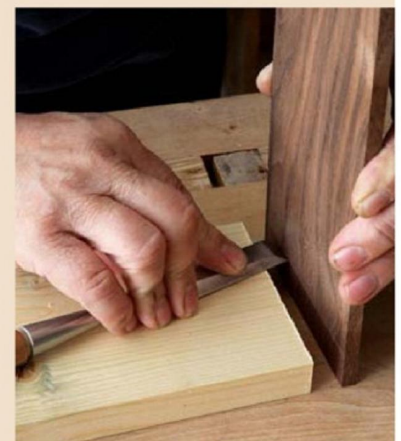
Swap the components over for the corresponding shoulder line
