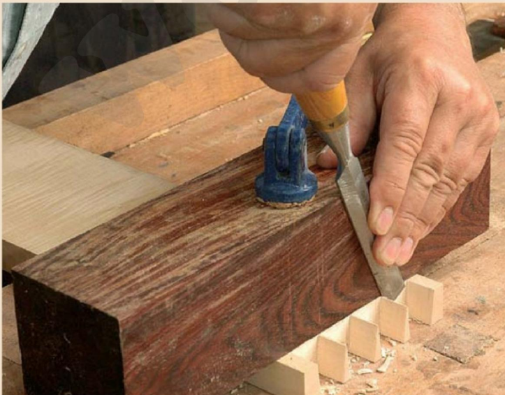
Transfer the dovetail positions from the pins on the mating piece
