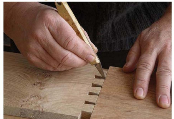
Transfer the dovetail positions from the pins on the mating piece
