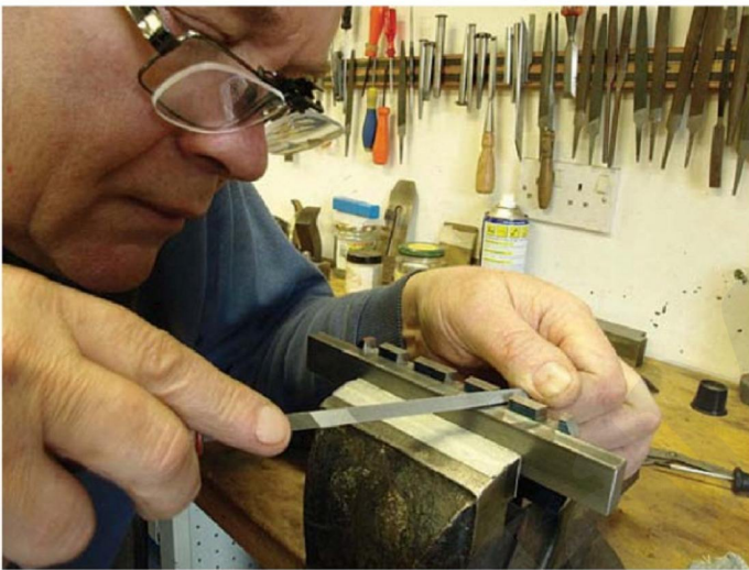
File each dovetail using a straight edge to maintain a flat shoulder line
