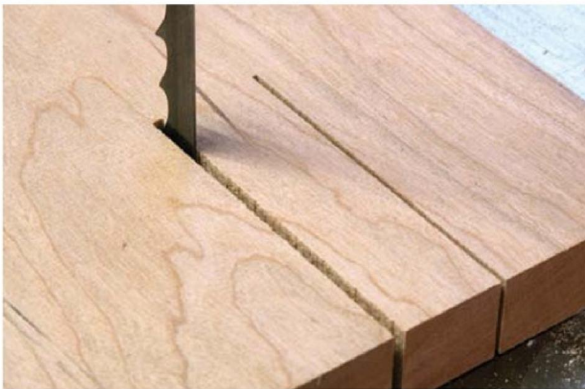
A blade with a wide set (left) will allow you to perform tighter cuts
