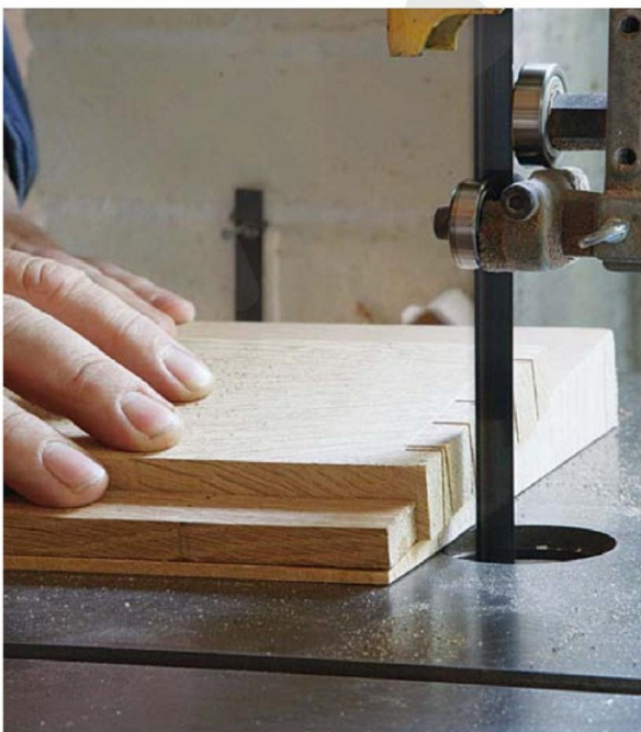
Turn the wedge over and complete the remaining cuts
