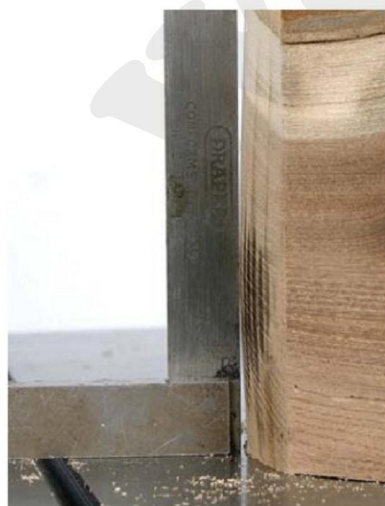
Barrelling is more pronounced on deeper cuts and can be caused by under tension as well as a blunt blade
