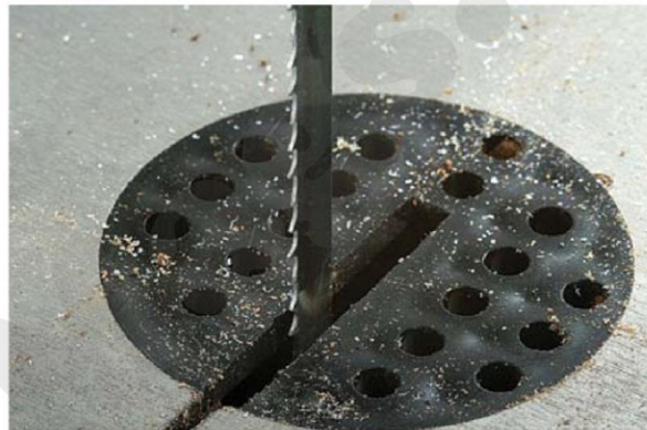
Perforated inserts reduce swarf build-up between the board and the table
