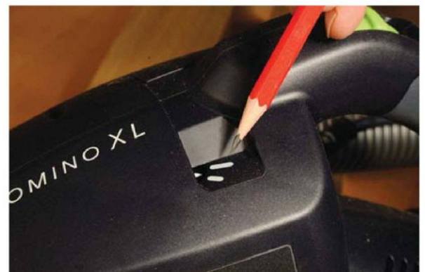
The switch between wide and narrow mortises is clearly indicated on the top of the machine casing
