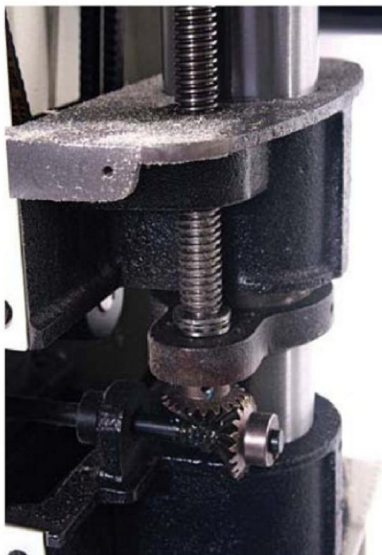
Bevel gears on each side of the bed ensure smooth and accurate raising of the bed
