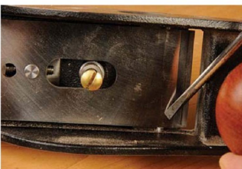
Set screws in the side of the body help to guide the blade and maintain settings
