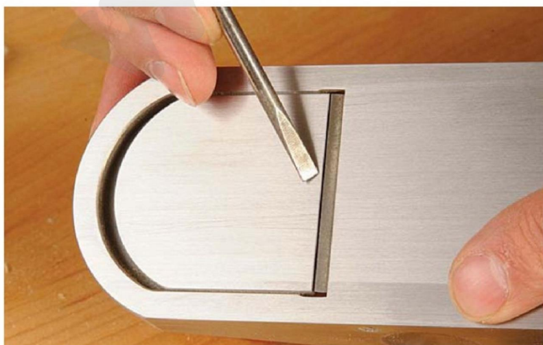
The adjustable mouth closes to a very fine aperture
