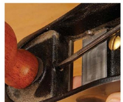
A stop screw prevents the toe sole from colliding with the blade
