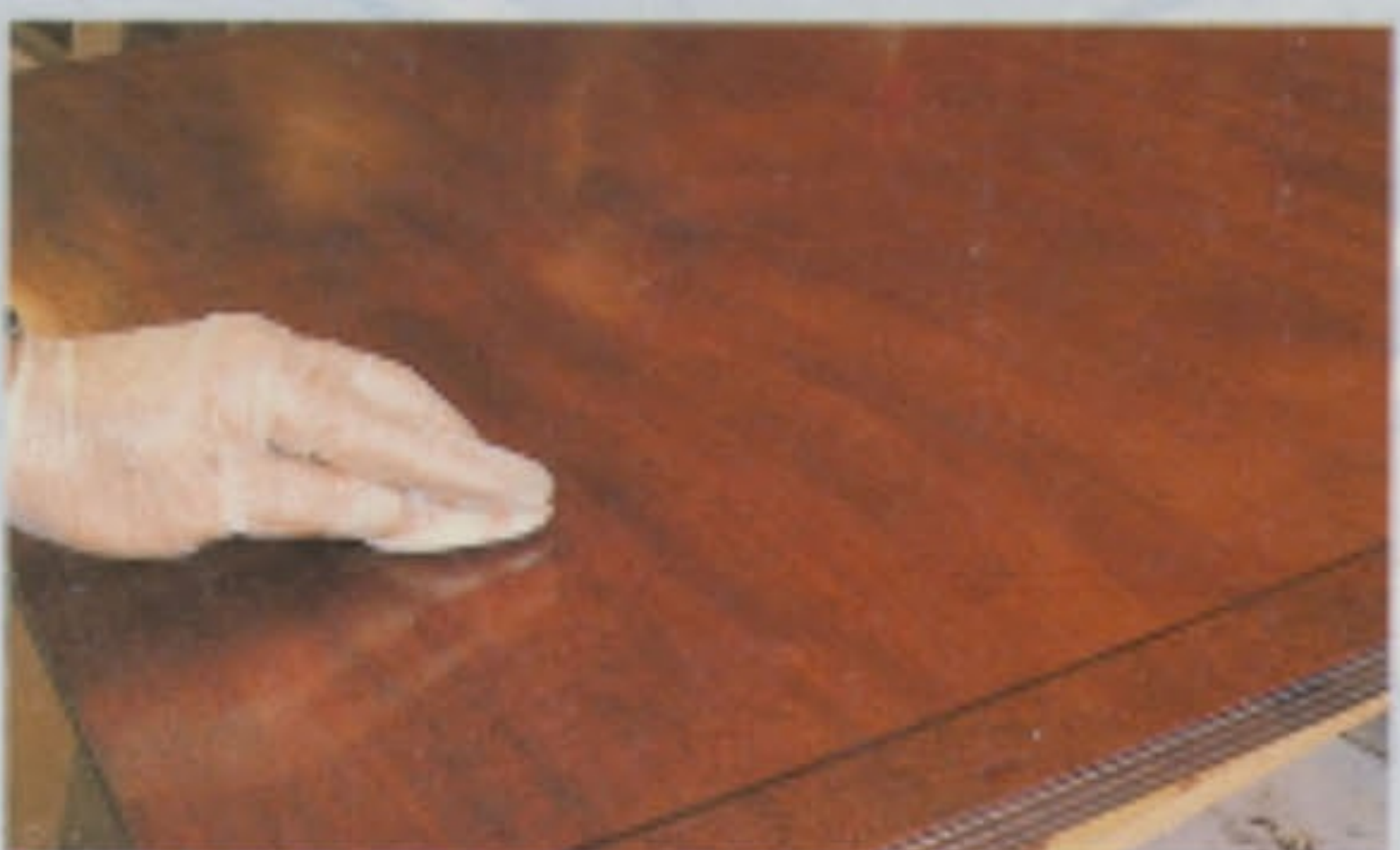
Final pulling over with 'pull over' solution
