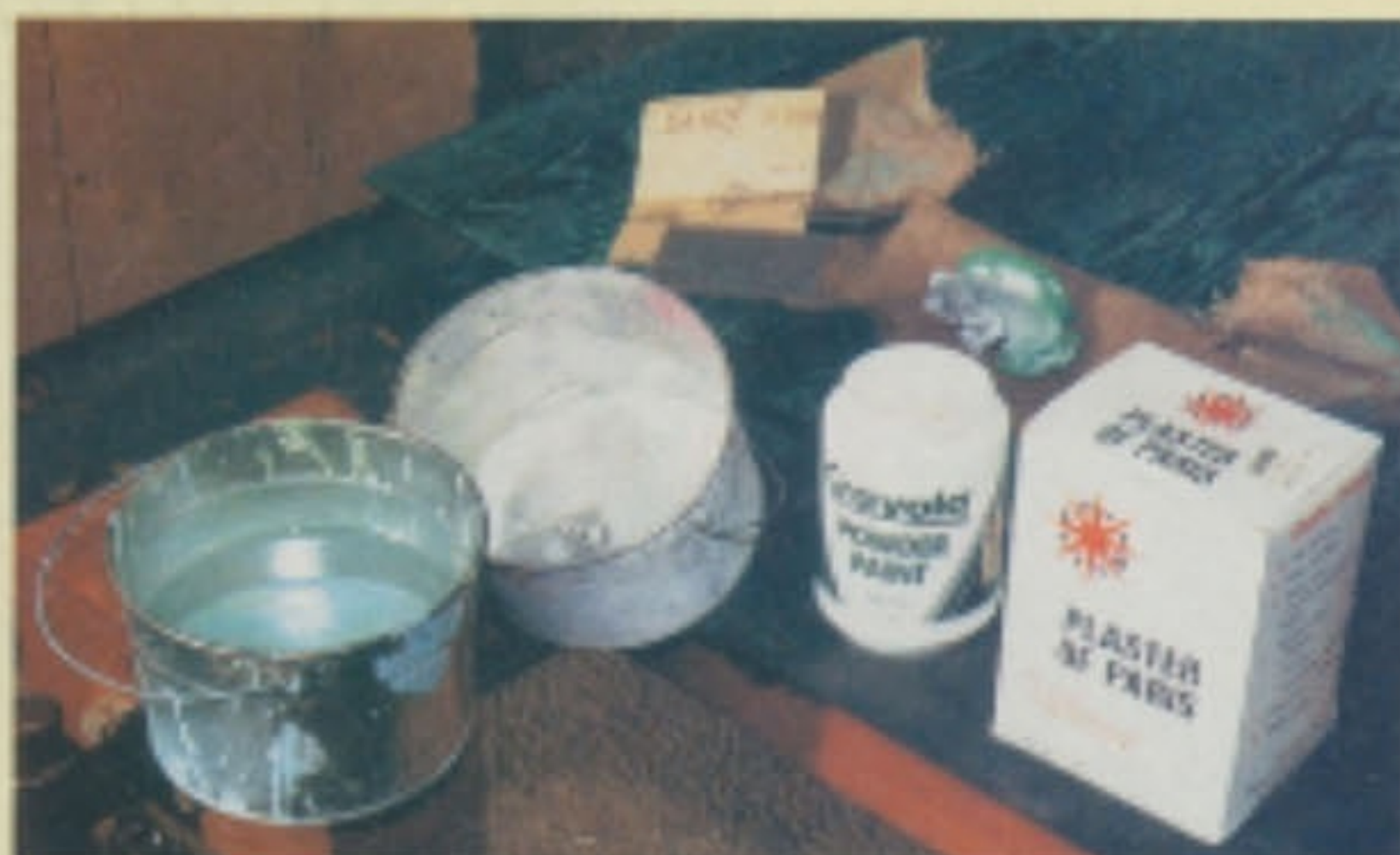
Tools and materials for filling grain
