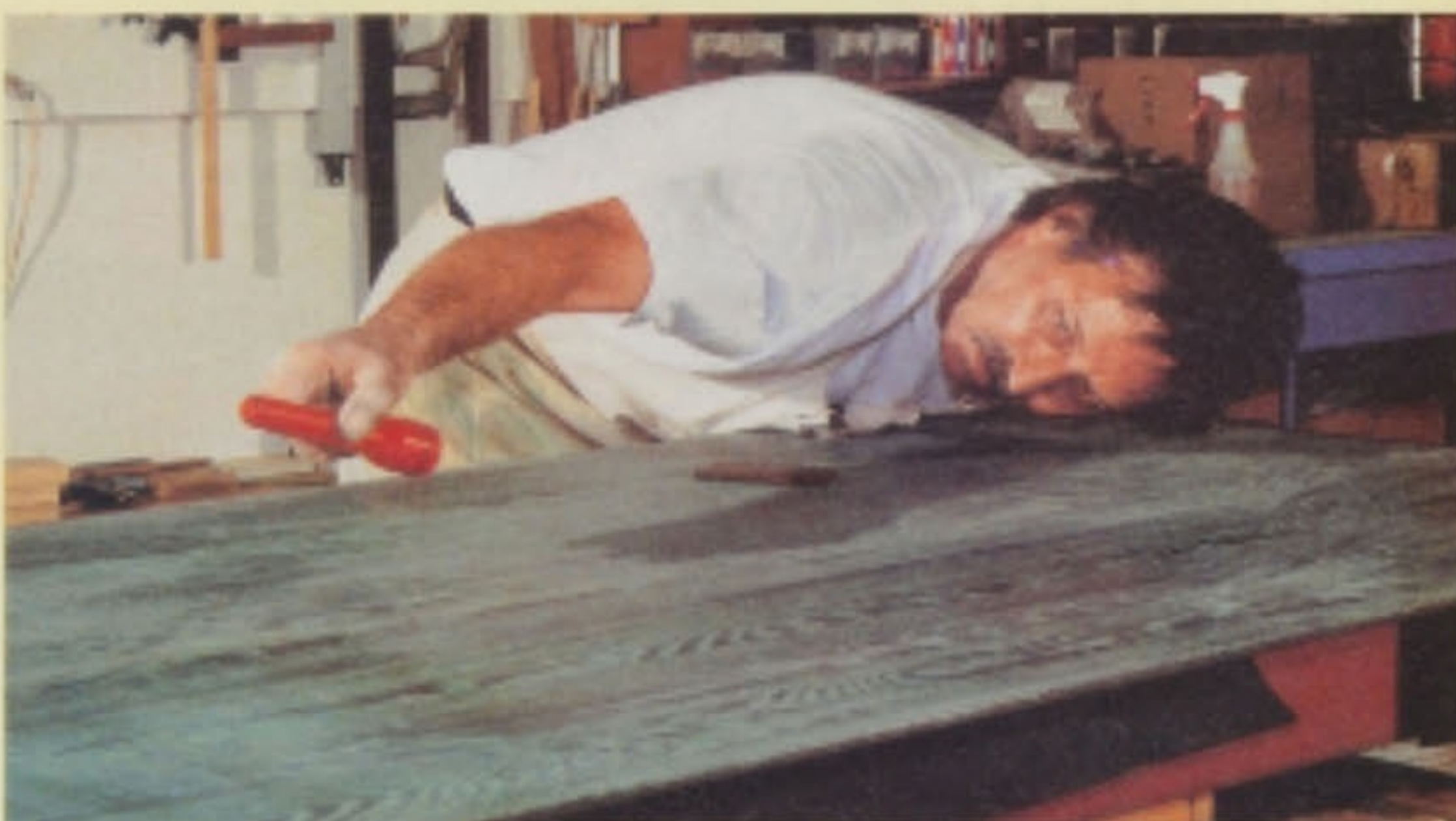
Shine a light from a low angle to reveal unfilled grain and other flaws
