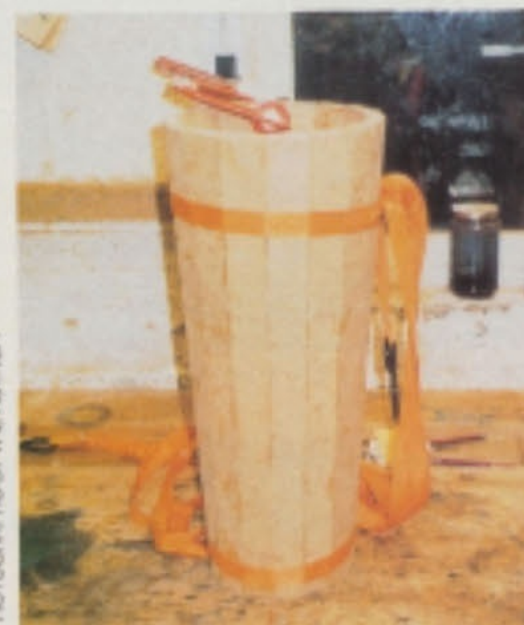
Clamping up the tapered column
