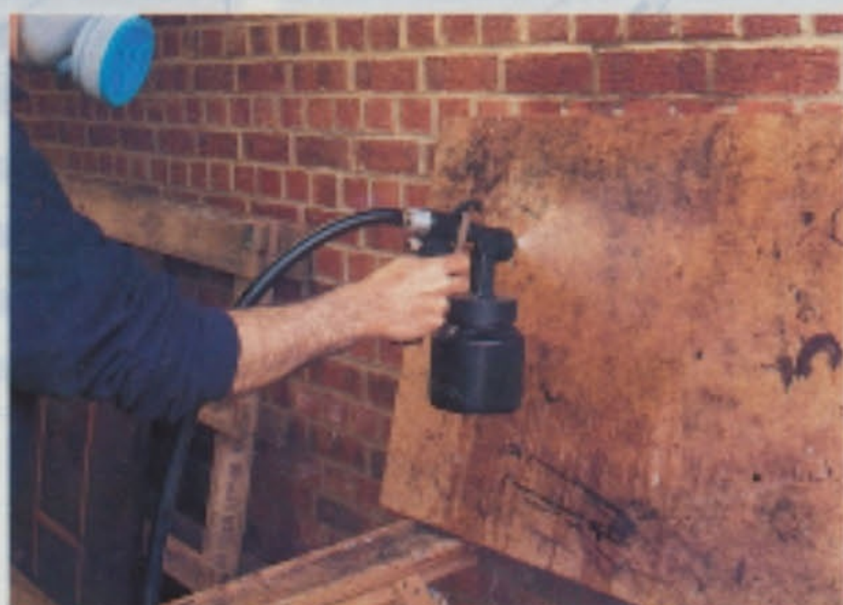
Testing the spray pattern
