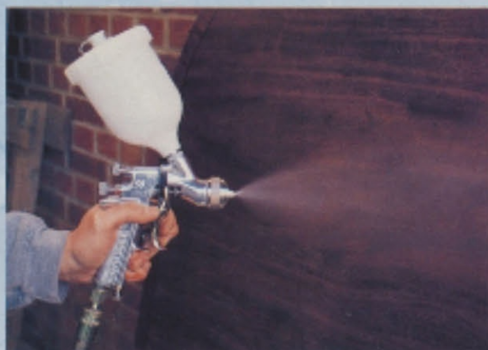
One disadvantage of this set-up is over-spray, caused by the finish bouncing off the surface, due to the higher pressure
