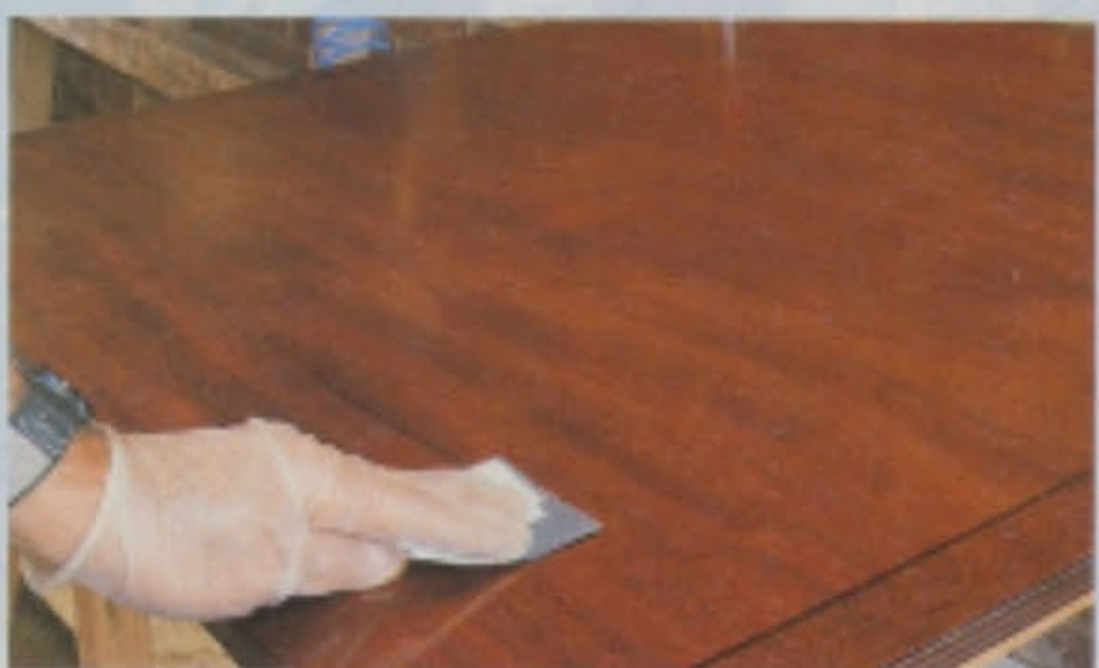
Cutting back with 400 grit Lubrasil paper and white spirit
