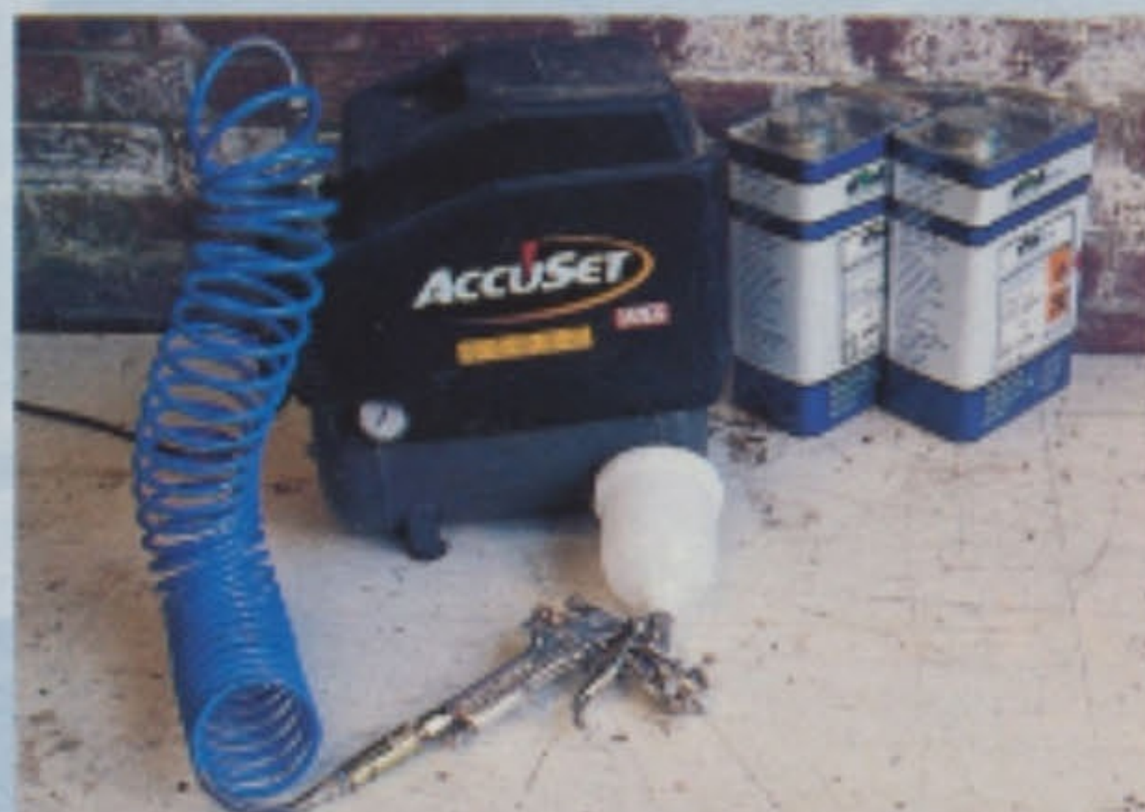
Conventional spray set-up, using a compressor with moderate volume and high pressure
