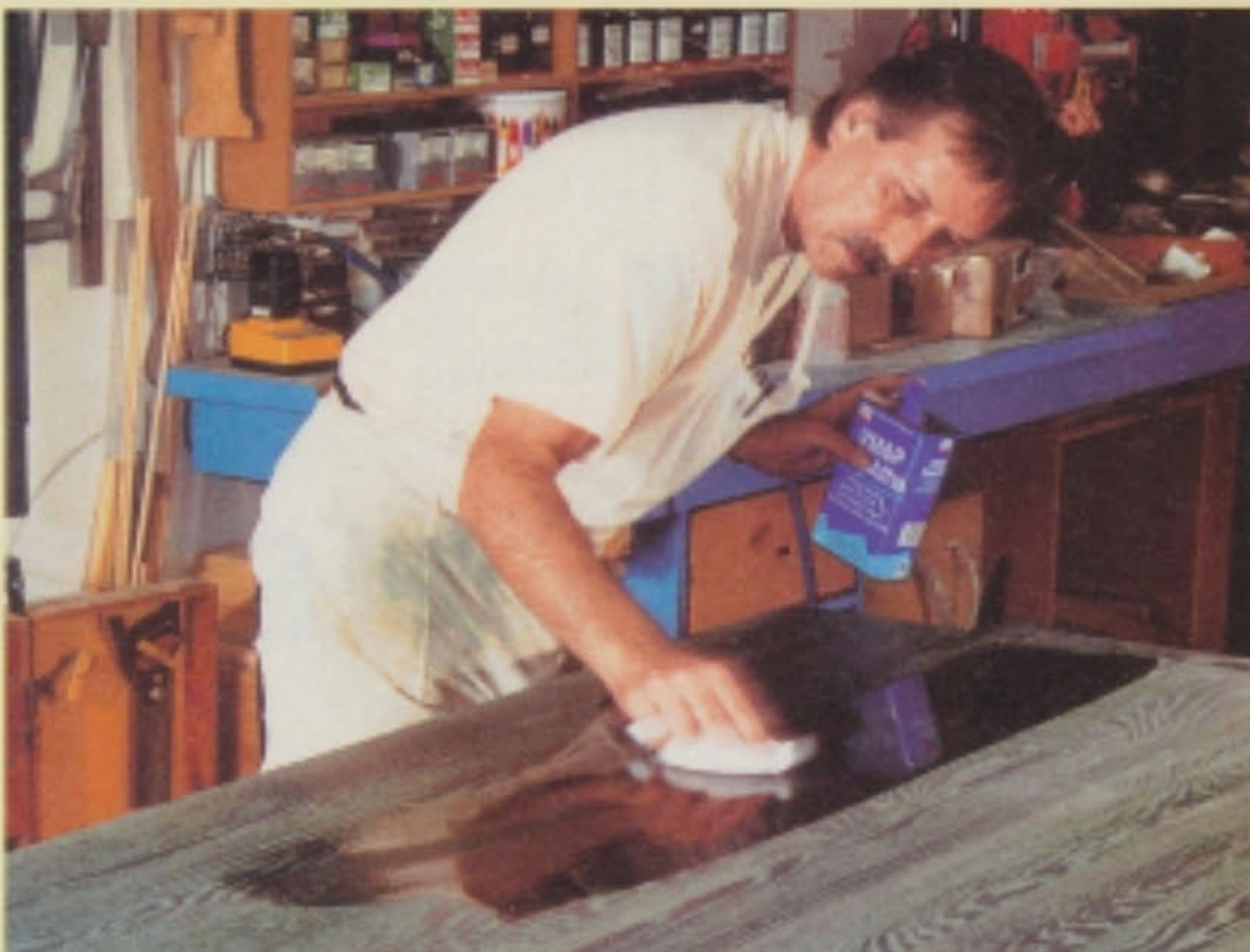
Apply naphtha to the surface to highlight areas not filled properly
