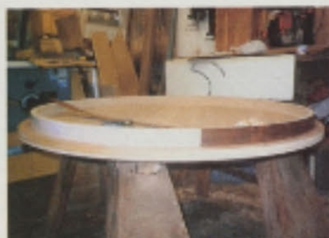
Applying veneer to the apron, with great difficulty, using an iron and PVA
