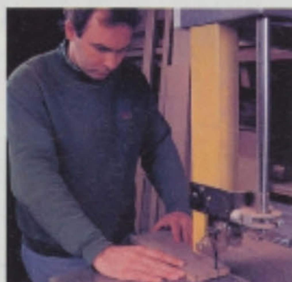
Mark using the 601 for more 'refined' work – cutting dovetails
