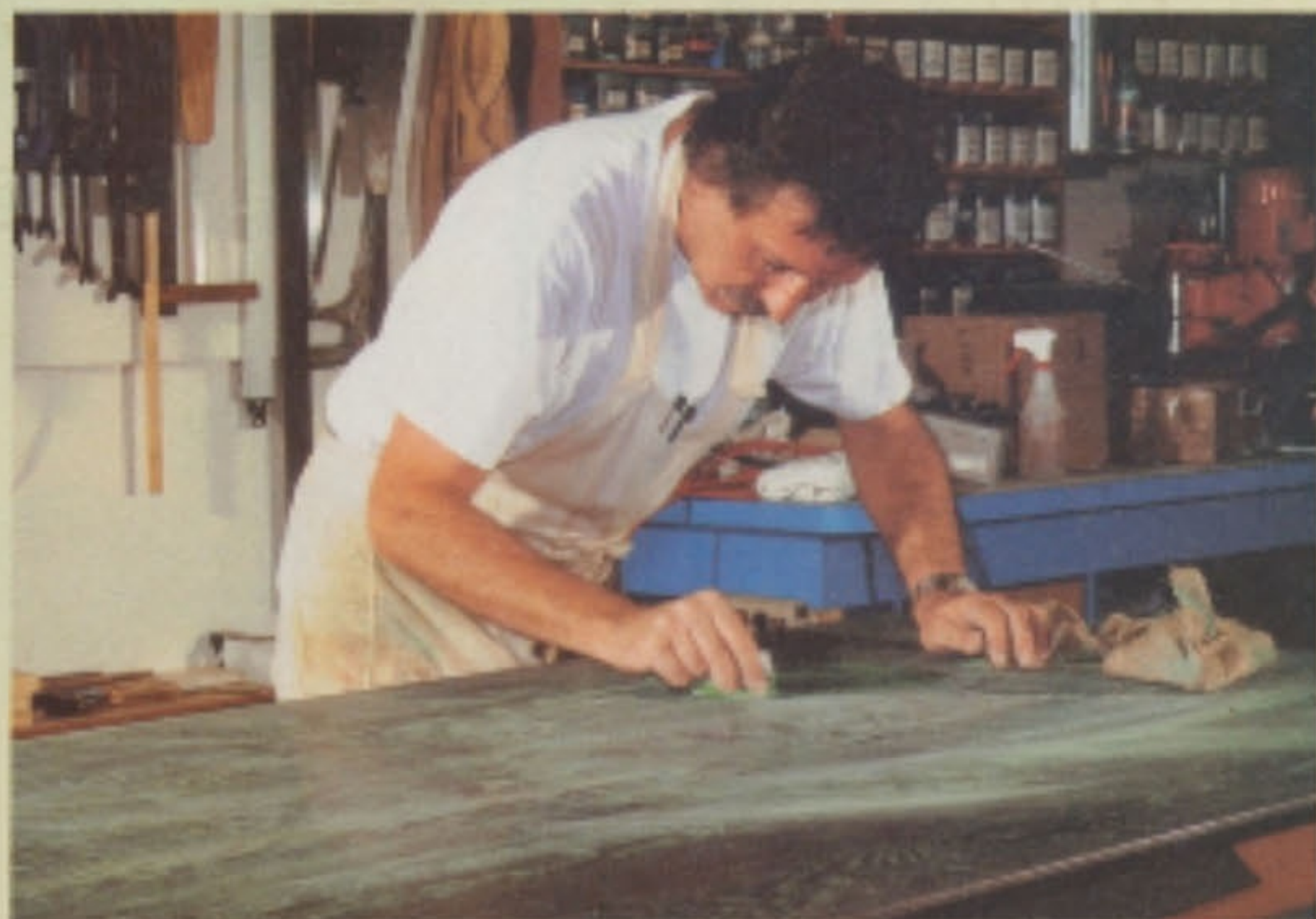
Apply the grain filler using a rag
