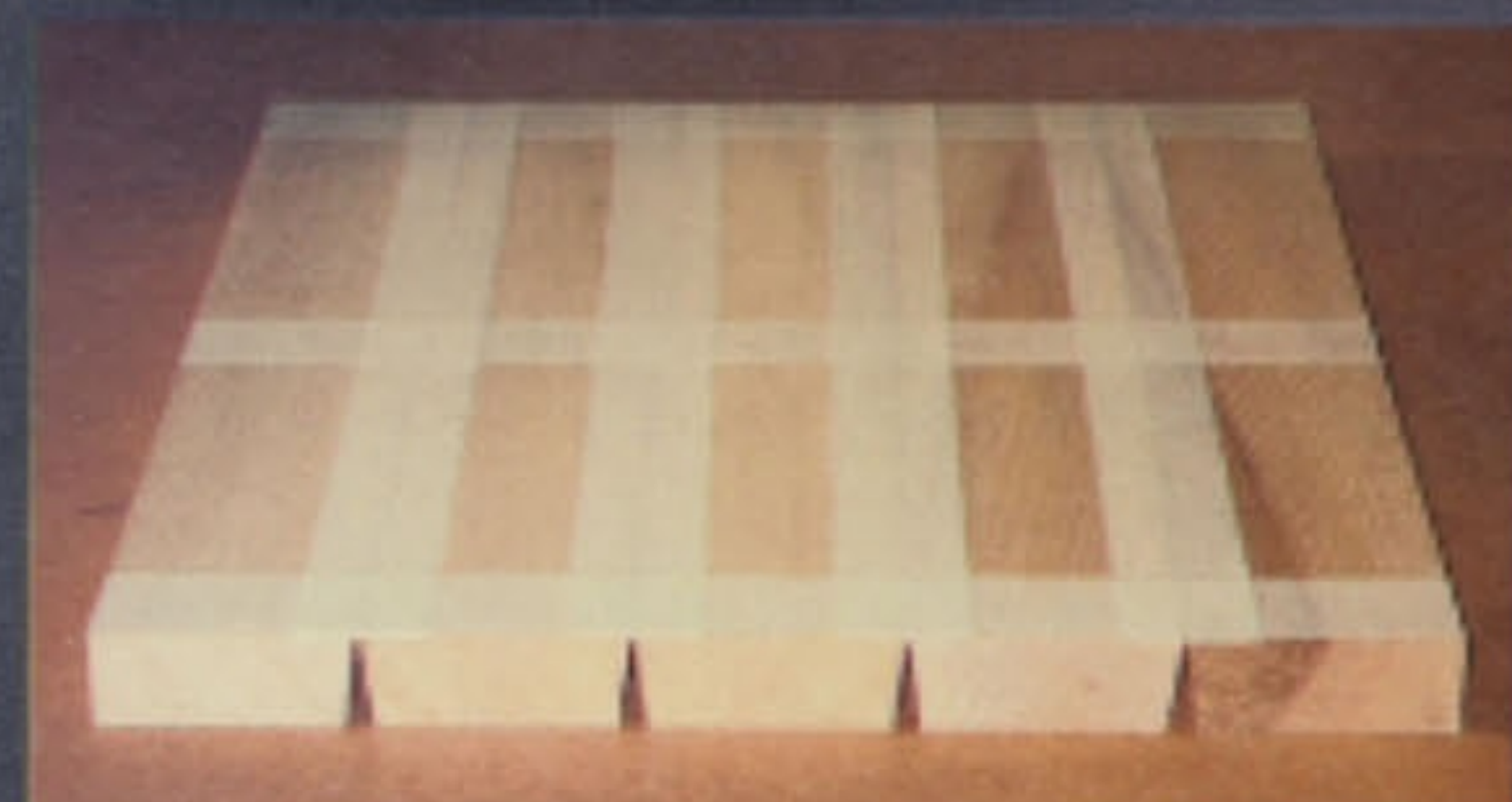
Joints assembled and taped on the outer surface of the curve
