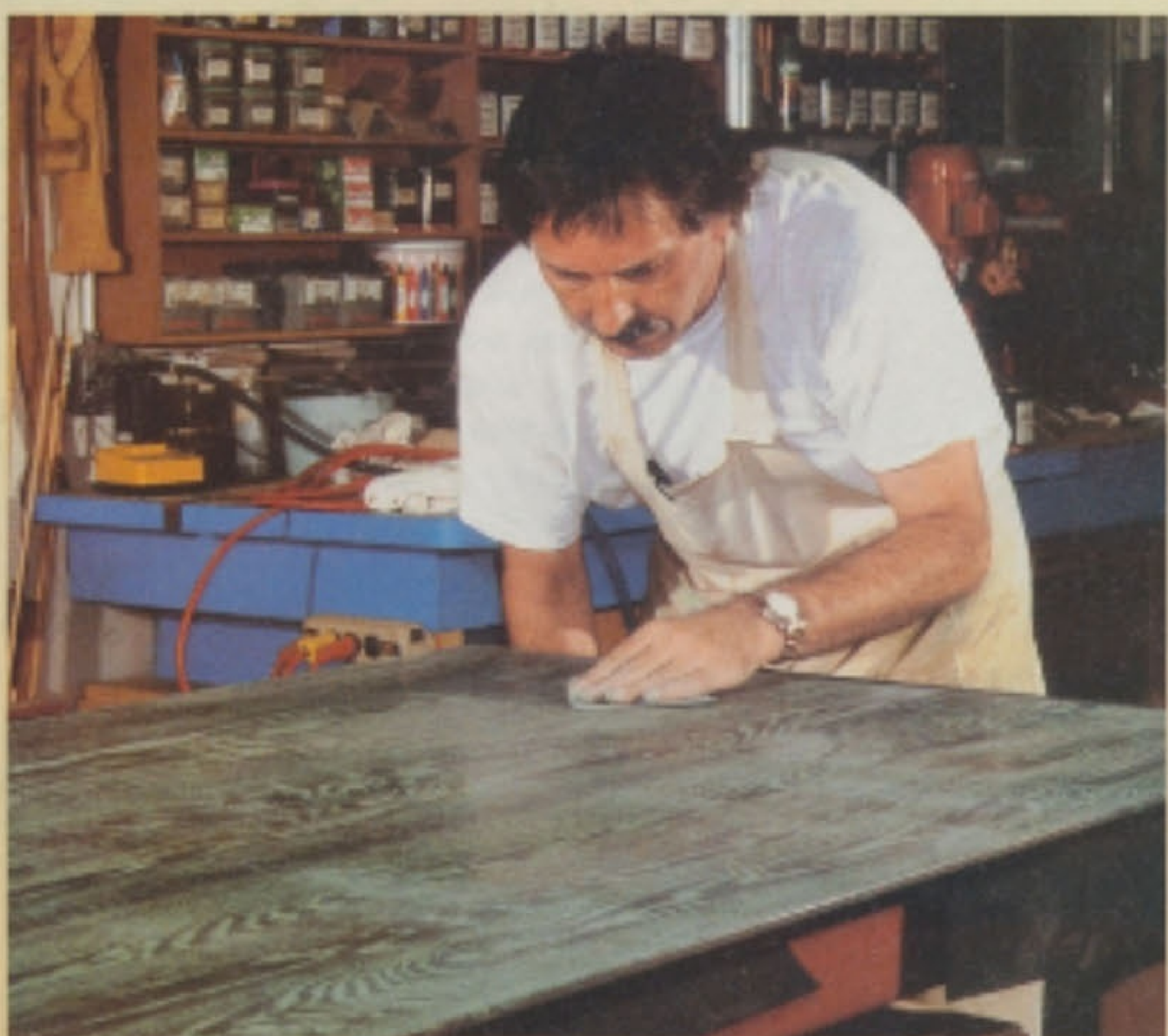
Hand sand dry filler with grain
