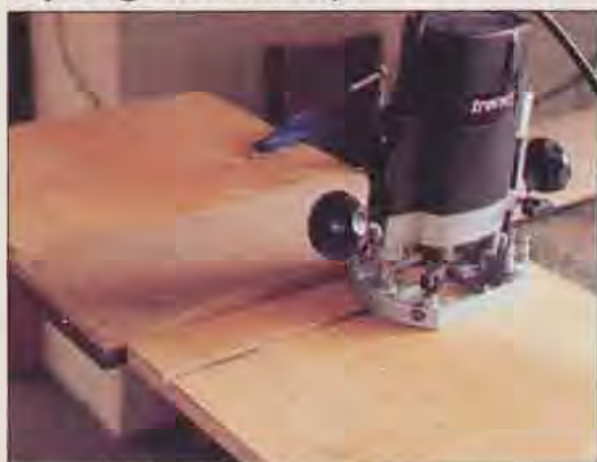
Cutting a housing using a shop-made guide
