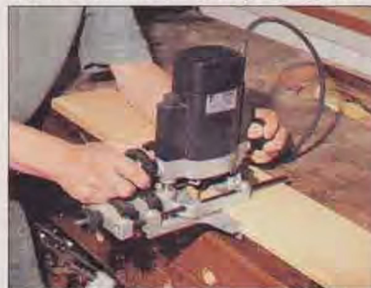
Starting the first cut of a rebate by backfeeding, subsequent cuts are done in the conventional manner
