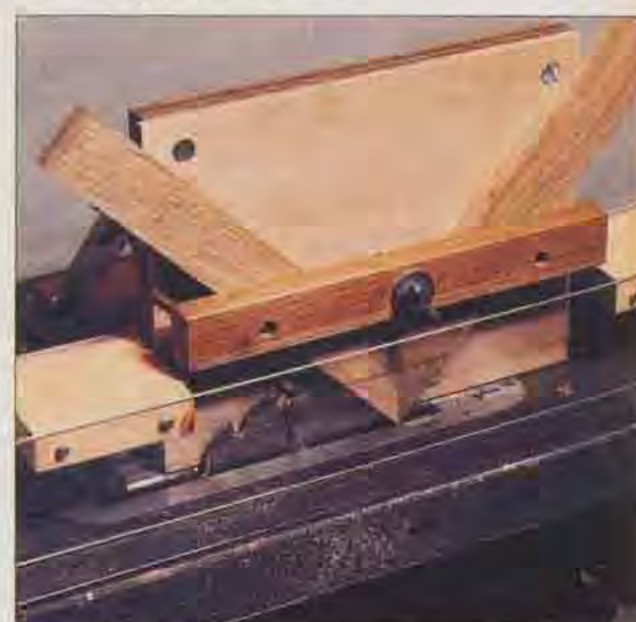
Sawing the slots for a mitred frame
