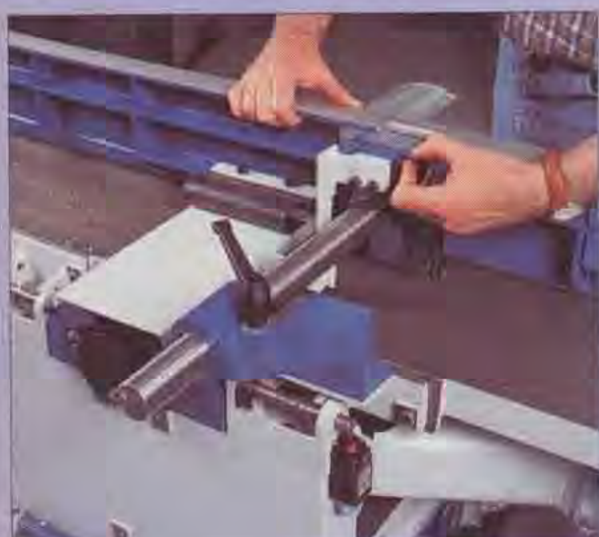
Apart from being a nice solid lump, the fence has a sprung pin to lock it square to the bed
