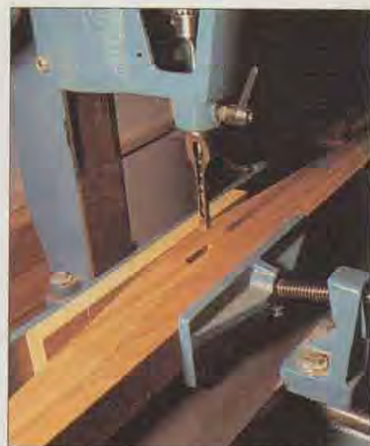
Morticing the rear leg for rear seat rail using an offcut to cramp the leg into the morticer
