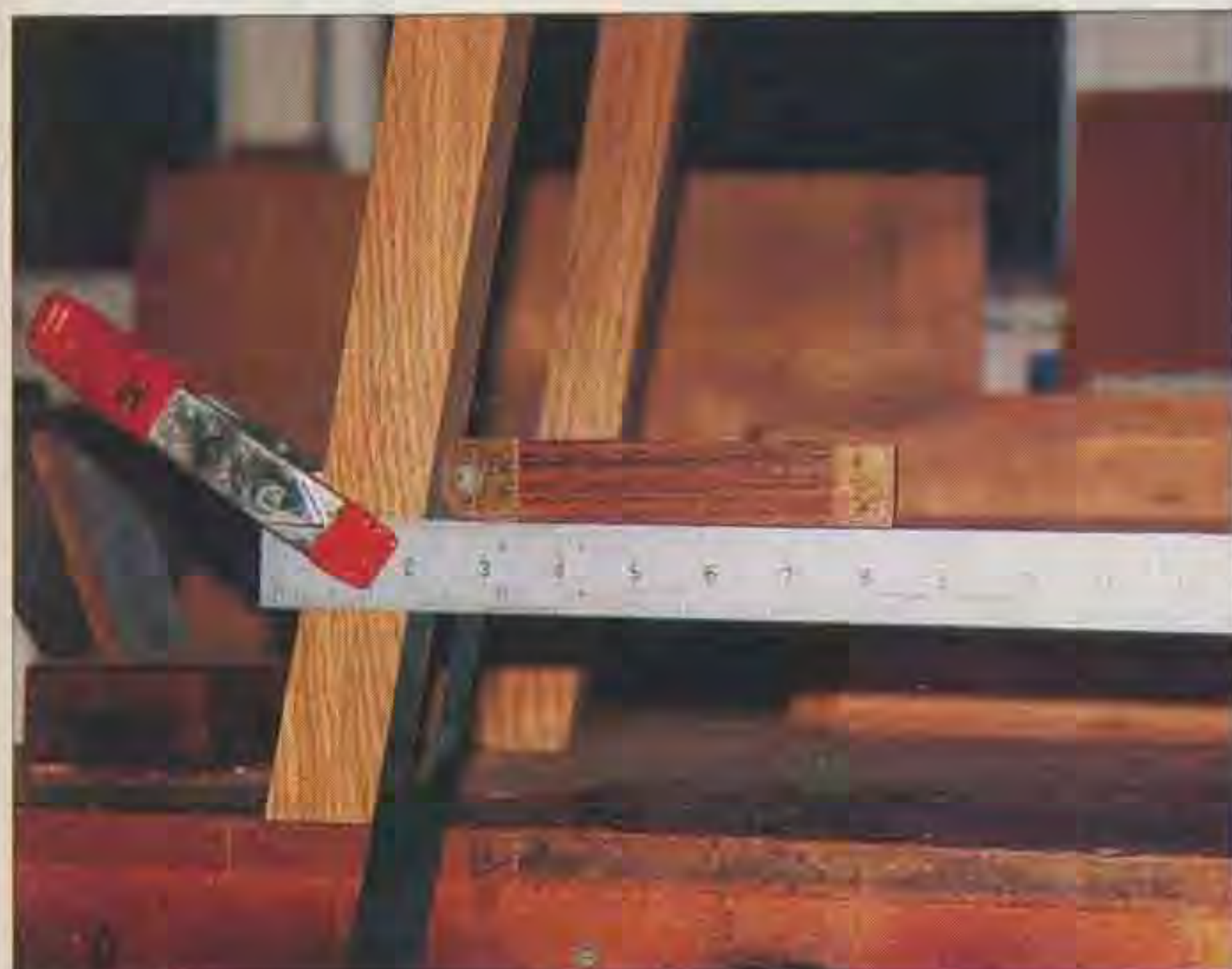
A steel rule and sliding bevel are used to find the shoulder angle for the rear leg/side stretcher joint
