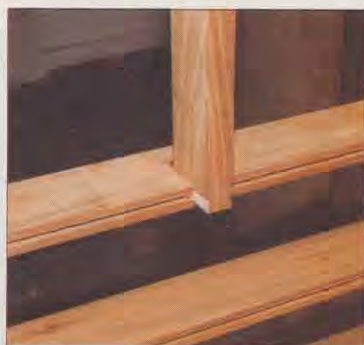
Sliding dovetail on drawer divider
