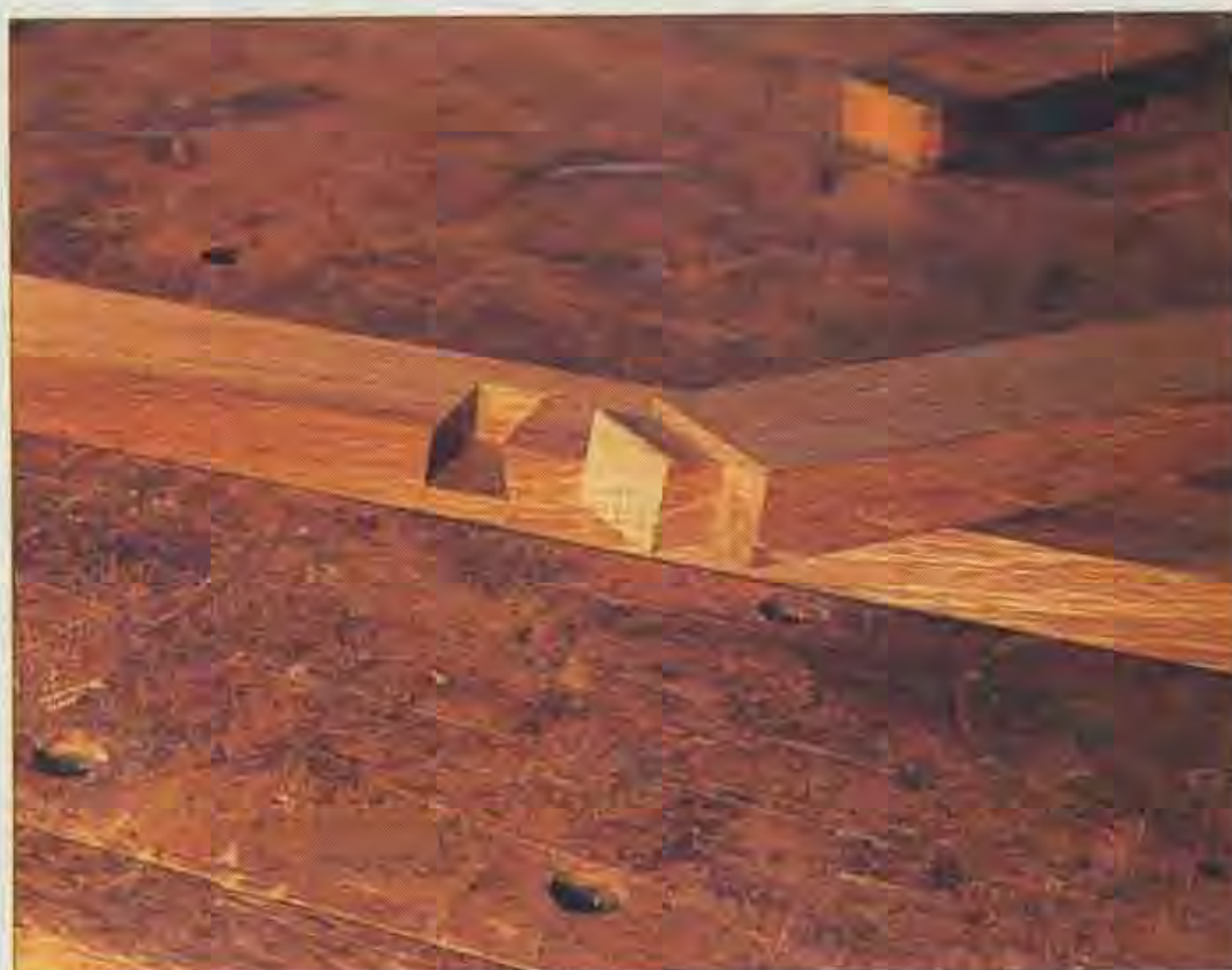
Note the stopped slot dovetail to the 'H' stretcher – joint apart
