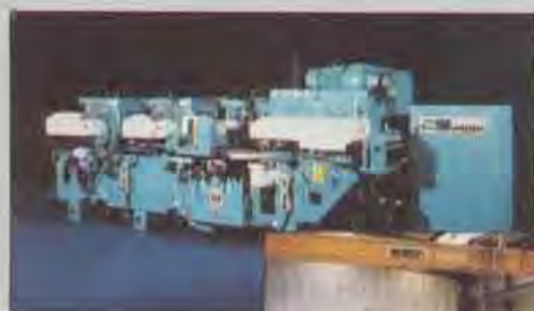
Wadkin XE Planer/Moulder after rebuilding in the Dalton workshops
