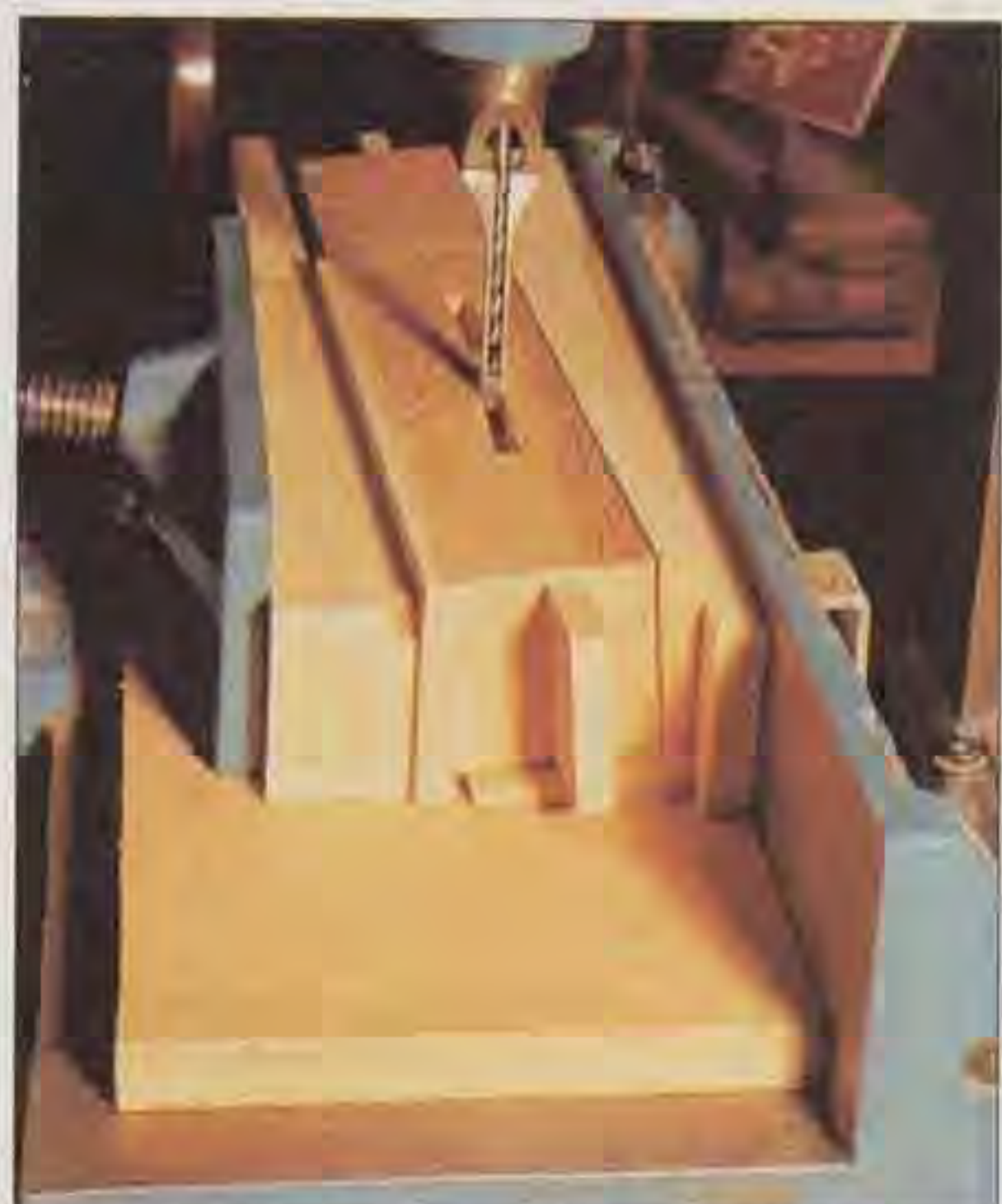
Additional wedges are made for the compound angle
