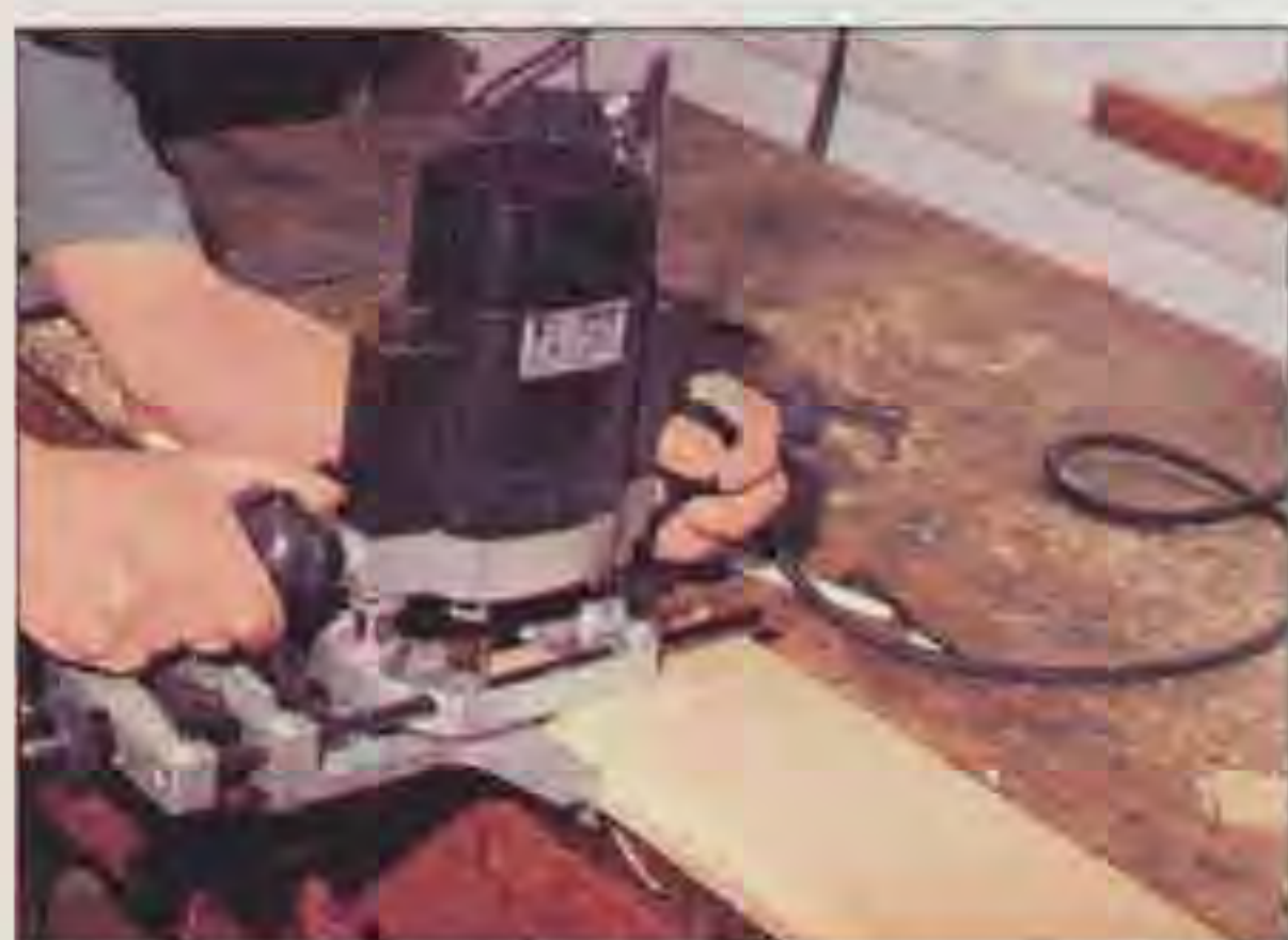
Starting the final cut of a rebate without the use of a run-in board
