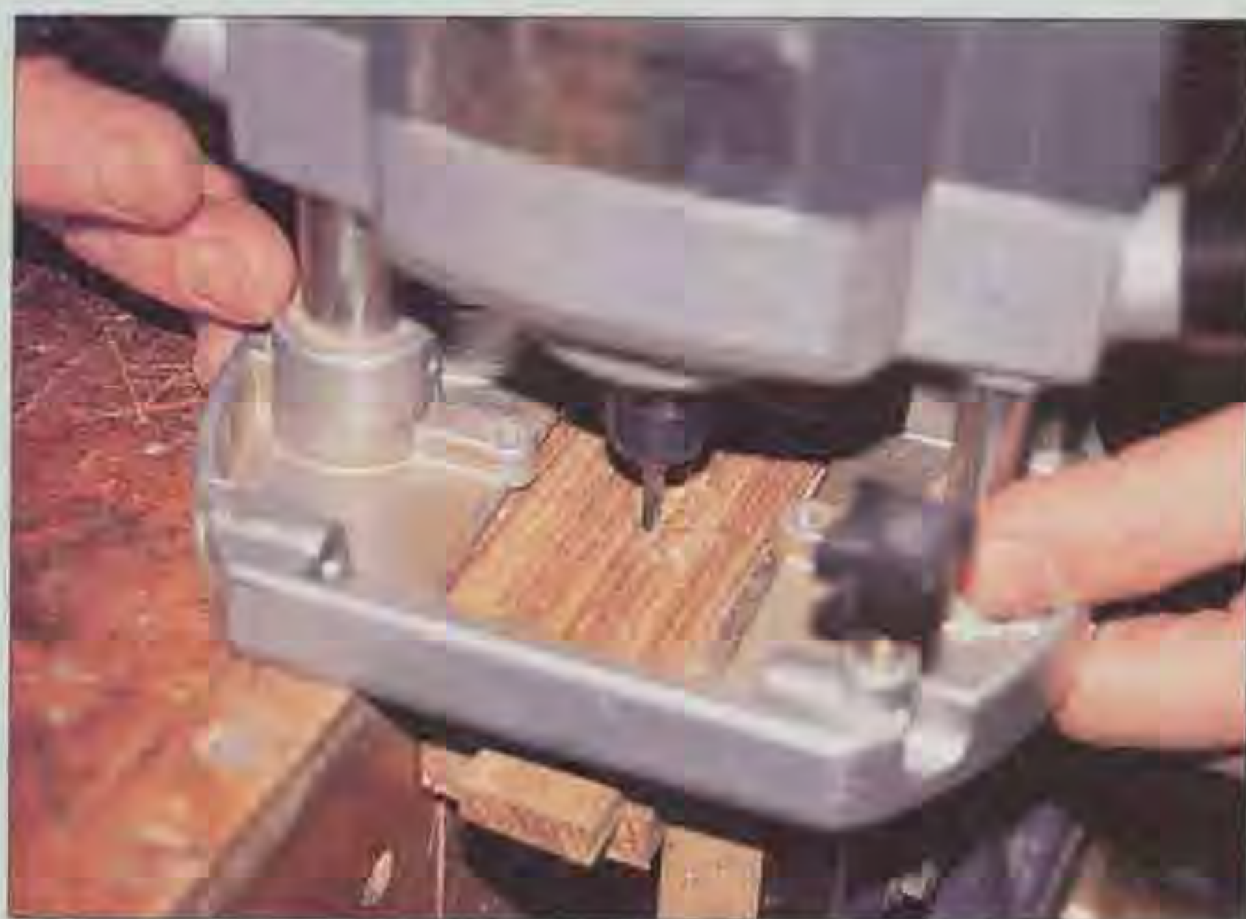
A freehand router with small bit is used for the inlay
