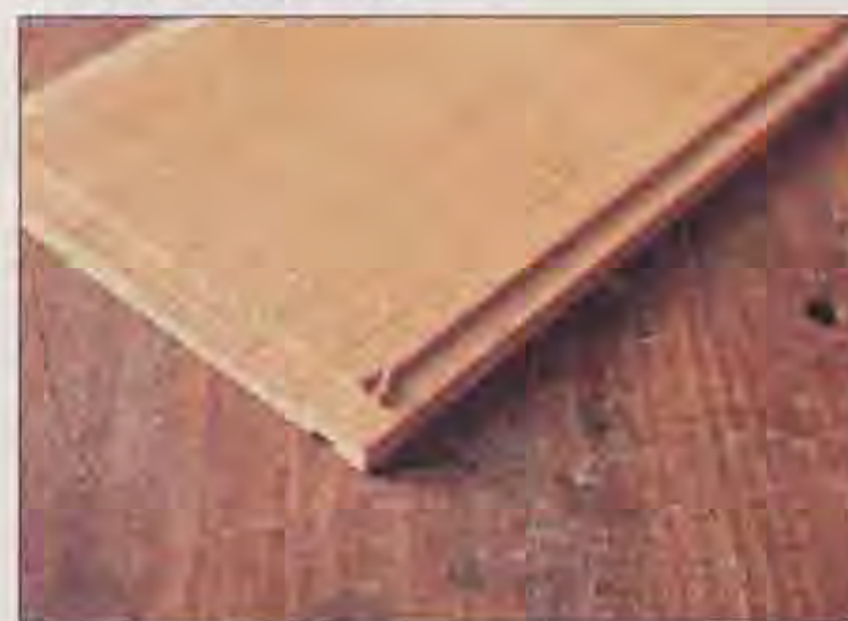
Breakout caused by machining a rebate in the wrong sequence
