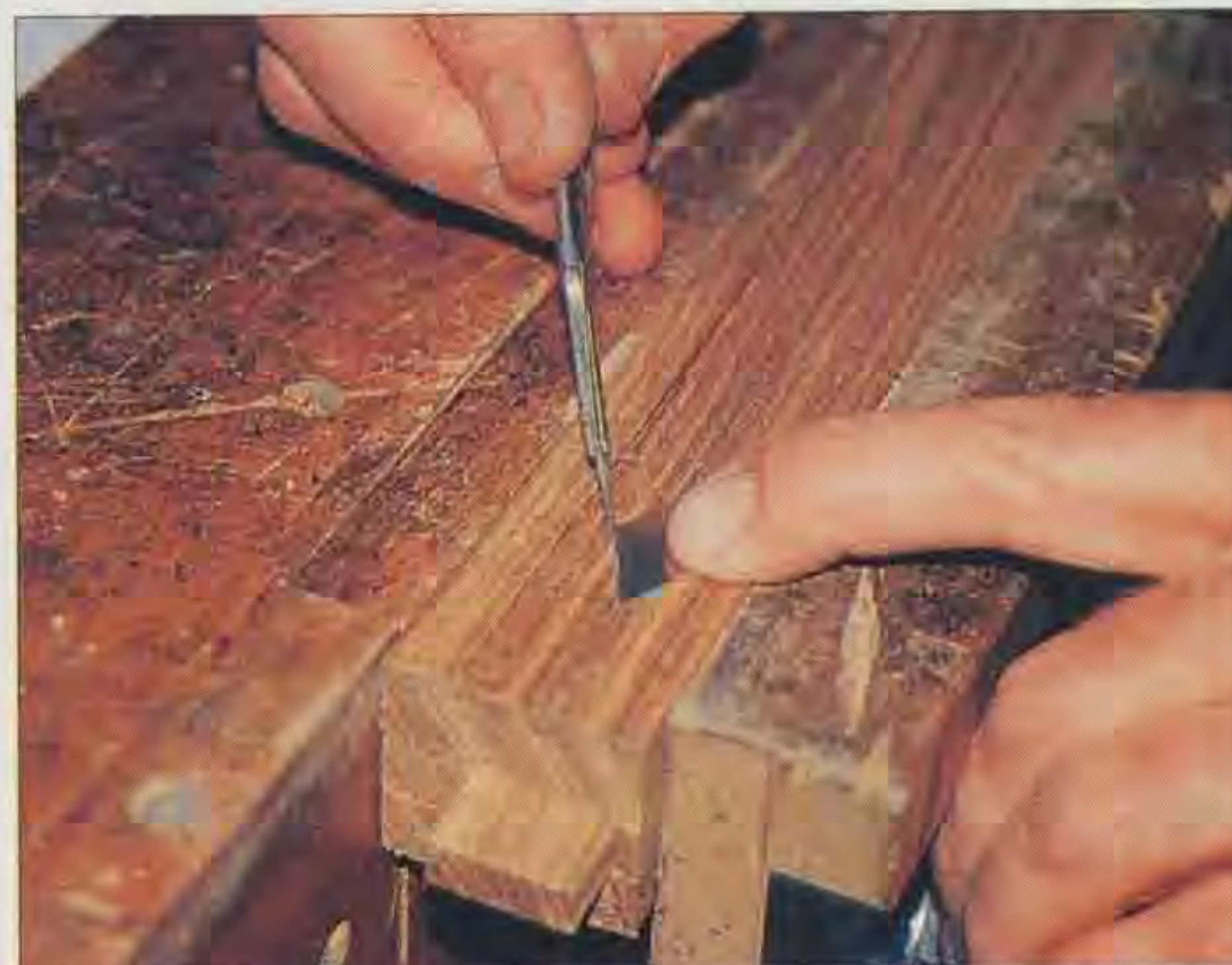
Marking out the diamond inlay with a scalpel
