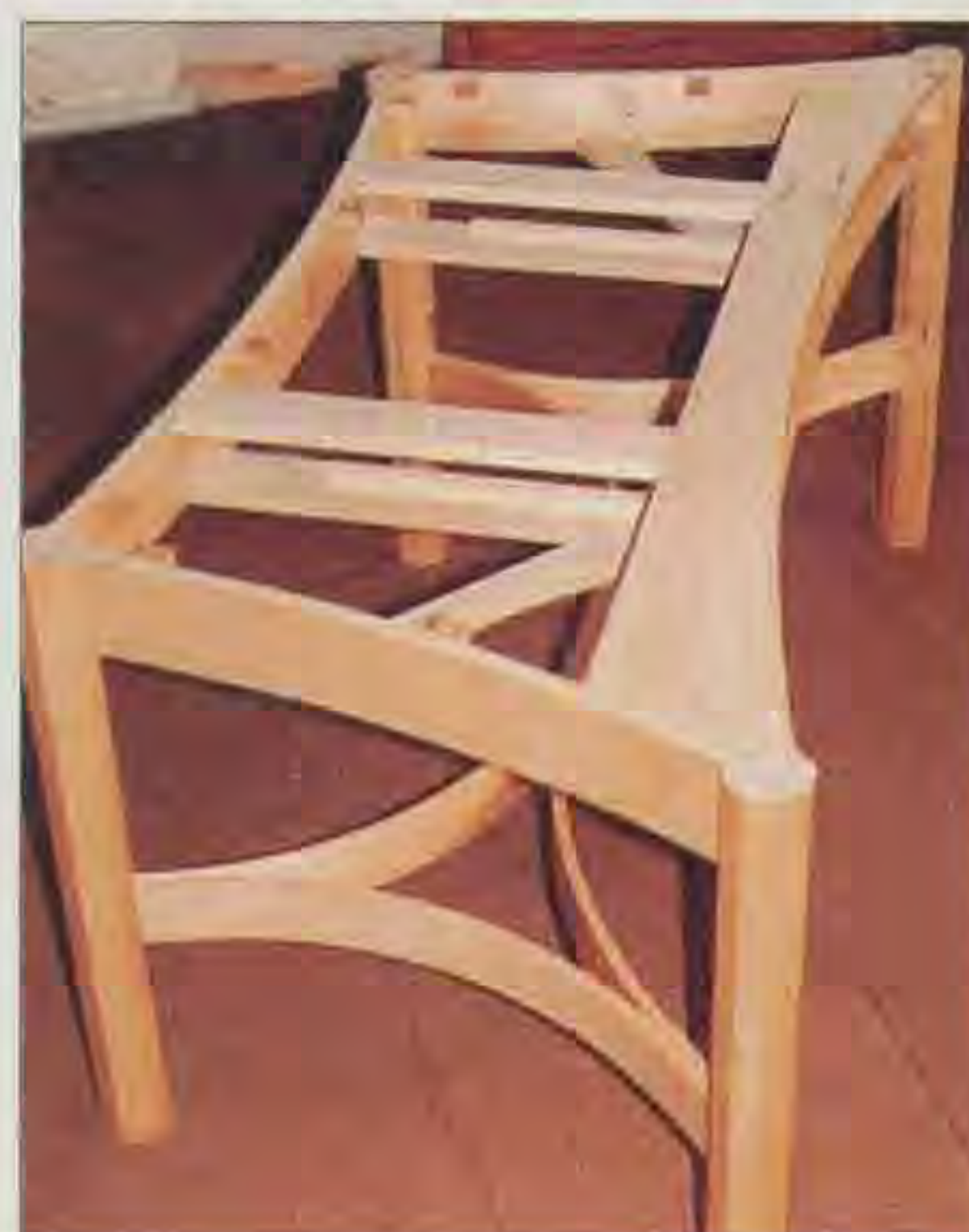
Internal carcass construction, showing runner
