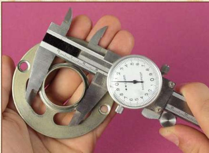
$$\text{Ø grand guide} - \text{Ø petit guide} = 2 \times \text{Ø fraise}$$
