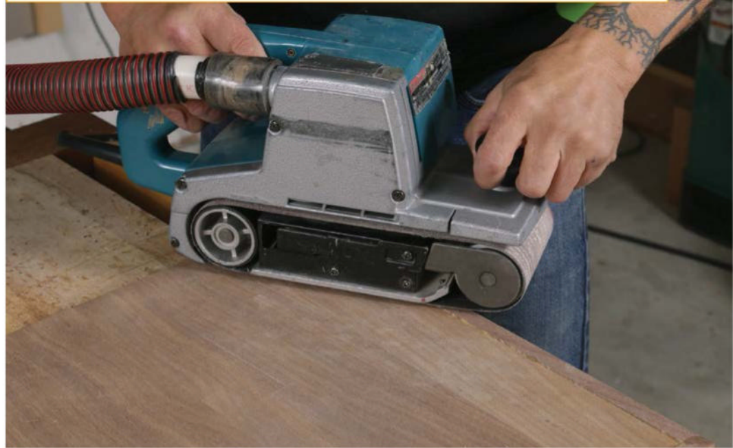
Skew the sander. Because the solid-wood edge is proud, most of the sanding is needed there. A slight skew angle will focus more surface area of the sanding belt over the desired area.
