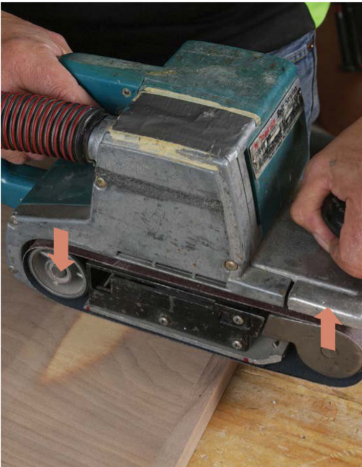
Balance the weight. When sanding the solid-wood banding flush, it's important to keep the weight even over the edge of the workpiece or else the weight will favor the back wheel and you will sand through the veneer.
