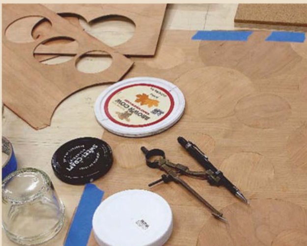
Working in circles. Using veneer he sawed from Jere Osgood's curly cherry planks, Coleman created a marquetry pattern with a quartersawn background inlaid with quartersawn and flatsawn circles. He shifted the orientation of the circles' grain direction to increase the chatoyant effect.
