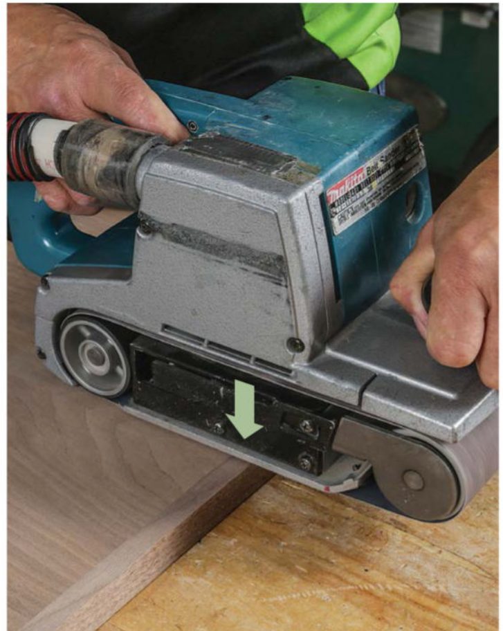
The tipping point. Focusing the weight at the center of the sander, or the “tipping point,” keeps the pressure evenly distributed on the flat platen and yields consistent results.
