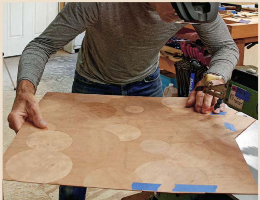
Working in circles. Using veneer he sawed from Jere Osgood's curly cherry planks, Coleman created a marquetry pattern with a quartersawn background inlaid with quartersawn and flatsawn circles. He shifted the orientation of the circles' grain direction to increase the chatoyant effect.
