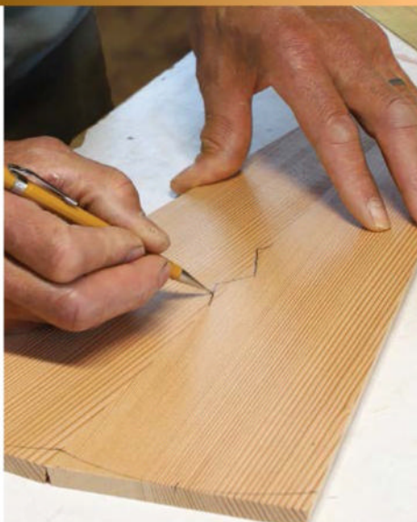
Perforation layout. With adjacent staves pressed together, Rolland lays out the angled cutouts by eye. In various lamps, he has made piercings in a wide range of shapes.
