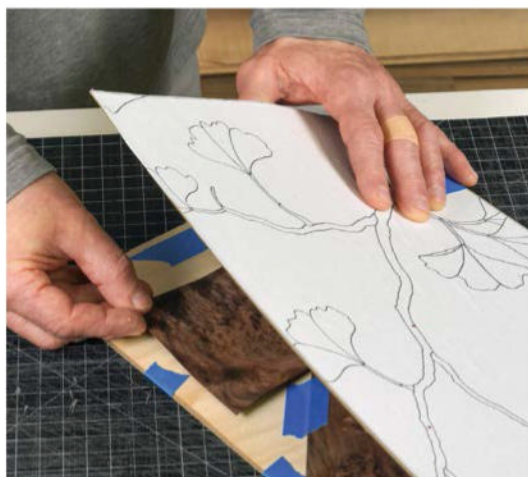
Find its position. Flip the drawing up and down to be sure the piece will lie below all of its corresponding parts in the drawing.
