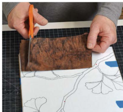
Start adding veneer pieces. Thibodeau often starts with branches when placing these parts. Cut each piece a bit larger than the part it corresponds to.
