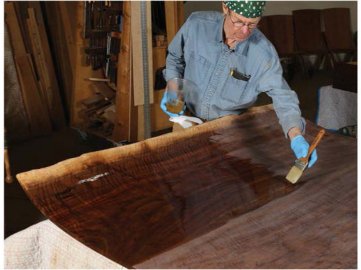
The final coat. The last coat of varnish should go on full strength, but it can also be thinned by 10% again if you feel it's too thick.
