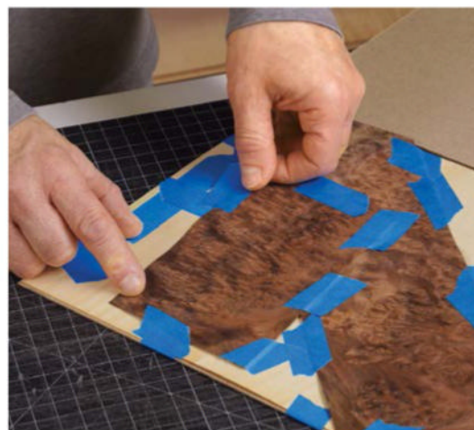
Secure it in place. Tape the piece down onto the background veneer (and any other veneer pieces that are already taped down).
