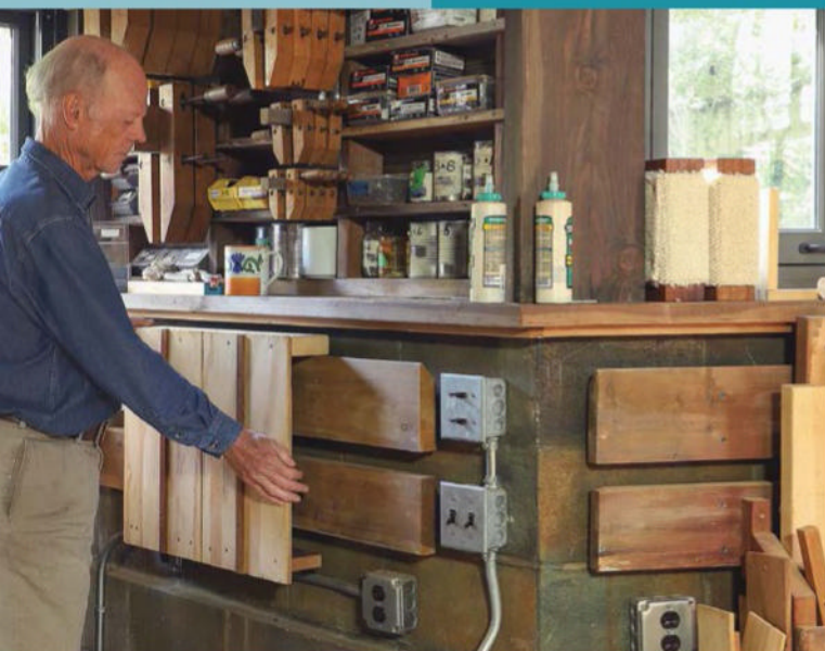
Bumpers, nailers, hangers. The concrete-block walls are lined with 2x8 bump boards. They soften the impact when a workpiece hits the wall and provide a convenient nailing or screwing surface. The upper board's top edge is beveled, making it a French cleat for hanging jigs.
