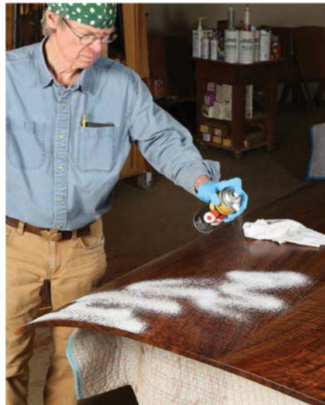
The final coat. The last coat of varnish should go on full strength, but it can also be thinned by 10% again if you feel it's too thick.
