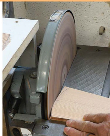
Creating the curve. The arc at the bottom end of the stave takes just a moment to shape at the disk sander.
