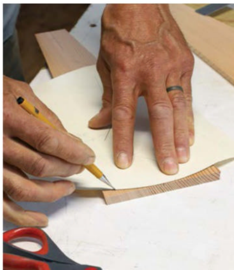
Arcing the ends. For this shade, Rolland adds a decorative curve to the wide end of the staves.
