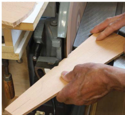
Notch with a disk. Pressing the stave against the edge of the disk makes shallow triangular notches that come together to form the finished piercing design.
