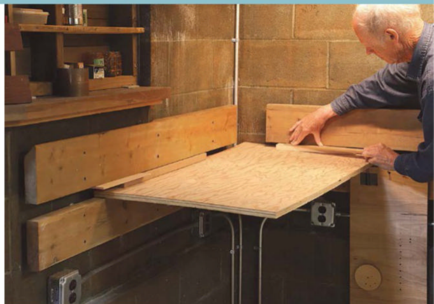
The corner table. When he needs an extra work surface, Sawyer slides a sheet of plywood between the bump boards at an inside corner and secures it with pairs of opposing wedges.
