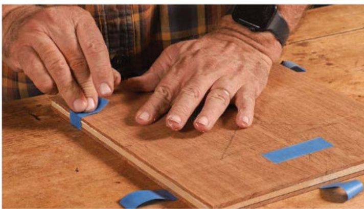
Panel lamination. Spread glue on the substrate—in this case \frac{1}{4} -in. MDF—and tape the veneers in place top and bottom. The tape will keep the veneers from shifting under clamp pressure.
