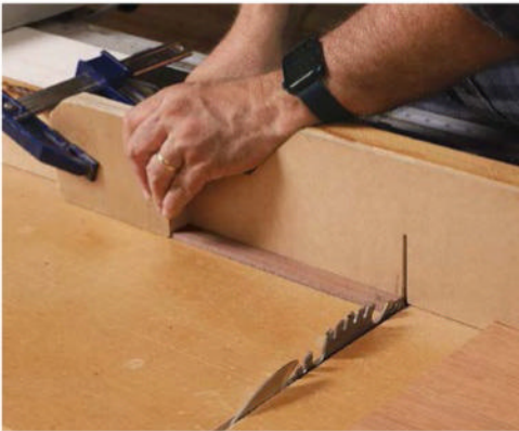
Shooting for a perfect fit. To cut the top panel to exact size, Stevens measures the dry-assembled frame with story sticks. He uses a shooting board to plane the sticks' end grain and dial in the exact length.
