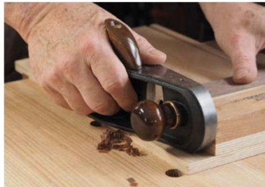
Focused control. The side handle of the Veritas Miter Plane is mounted right over the blade, giving the user exceptional control over the cut.
