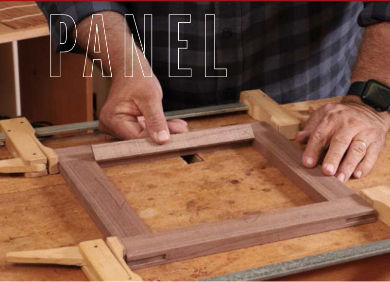
Shooting for a perfect fit. To cut the top panel to exact size, Stevens measures the dry-assembled frame with story sticks. He uses a shooting board to plane the sticks' end grain and dial in the exact length.
