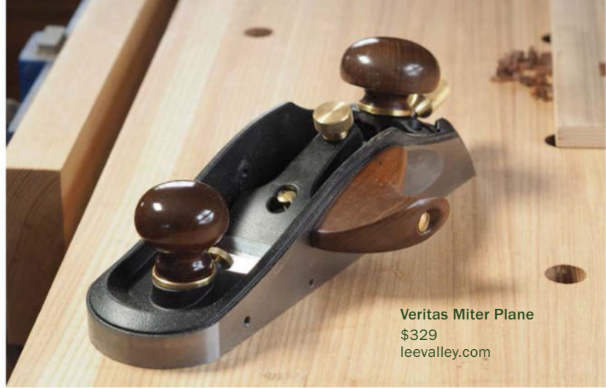
Focused control. The side handle of the Veritas Miter Plane is mounted right over the blade, giving the user exceptional control over the cut.
