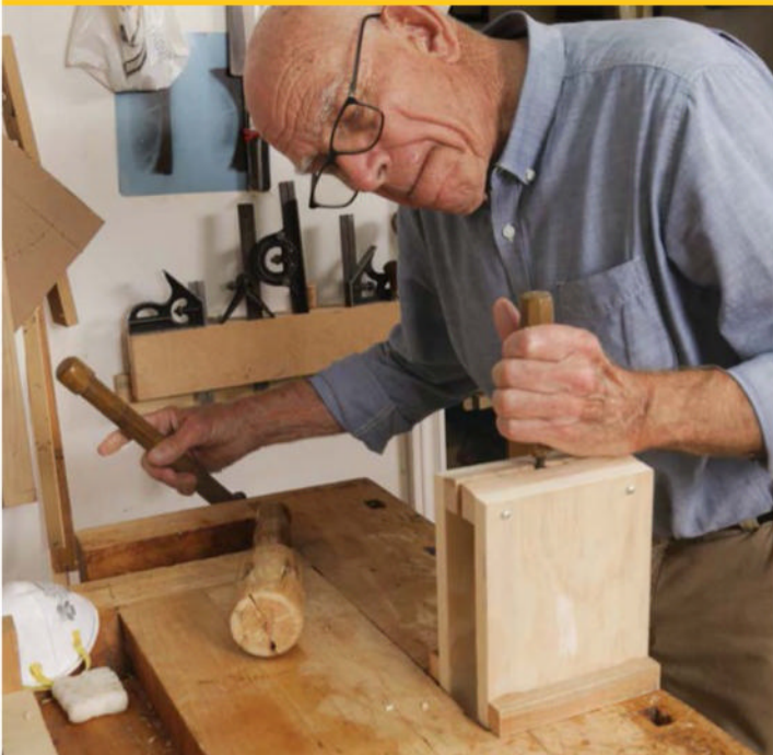
Tool holding. To save the faces of his bench vise from being marred by the metal blade, Howes uses a shopmade wooden tool clamp with sacrificial jaws that can be replaced when they get damaged.
