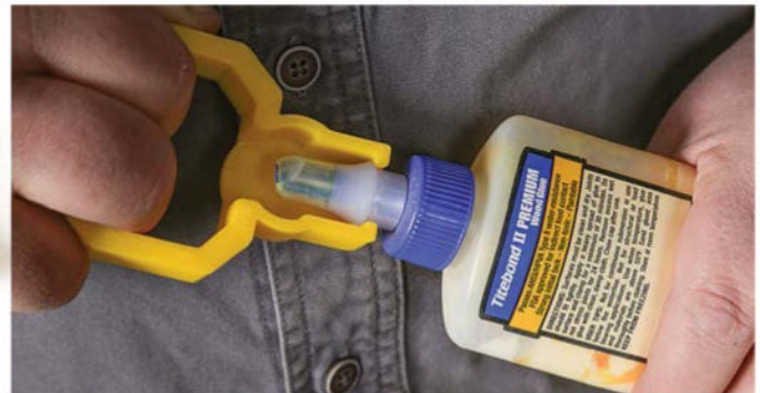
Glue-bottle gripper. This may look like a useless print until you start tussling with a defiant glue bottle. Then you realize it cost just $0.39 to make and you didn't have to lift a finger except to click the Print button.
