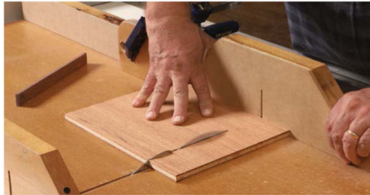
Impeccable crosscut. Stevens uses a second story stick to set a stop block on the crosscut sled and cut the panel to length.
