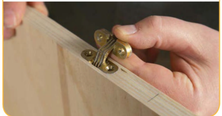
Easy concealed hinges. Concealed hinges add a simple look to any design but are far from simple to mortise for without a proper template. No matter what brand or size you're using, printing your own jig will get you the perfect fit each time.
