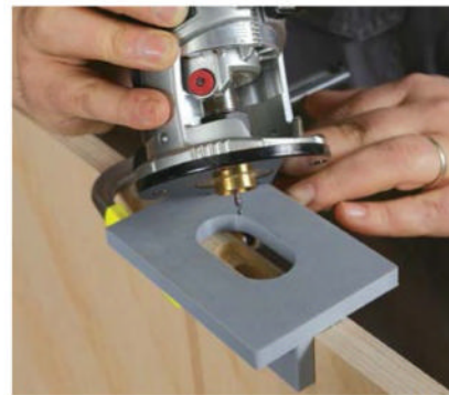
Easy concealed hinges. Concealed hinges add a simple look to any design but are far from simple to mortise for without a proper template. No matter what brand or size you're using, printing your own jig will get you the perfect fit each time.
