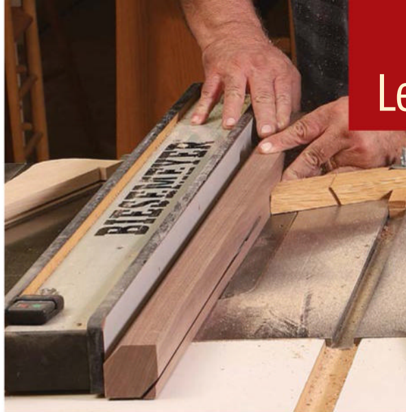
Begin with two bevels. With the table saw's blade set to 45°, make two rip cuts to create a pair of parallel faces.
