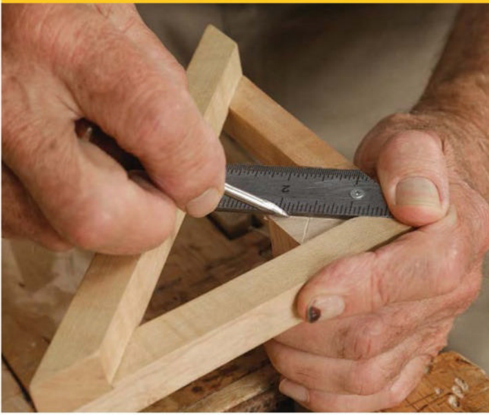
Mark the center. Before shaping the handle, Howes scratches two diagonals with a center square to find the center point for the lathe.
