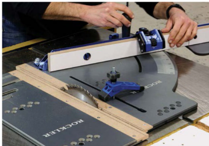
Easy set. With the oversized protractor scale and solid stop block, Godet was able to create a perfect set of miters on the first try.
