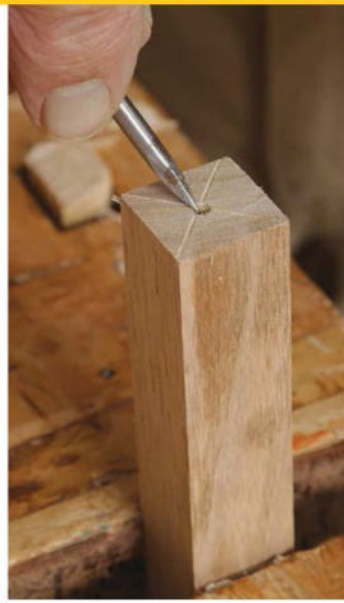
Good practice. For a better hold in the lathe, punch a center mark with an awl and saw kerfs on the diagonals for the drive center to grab.
