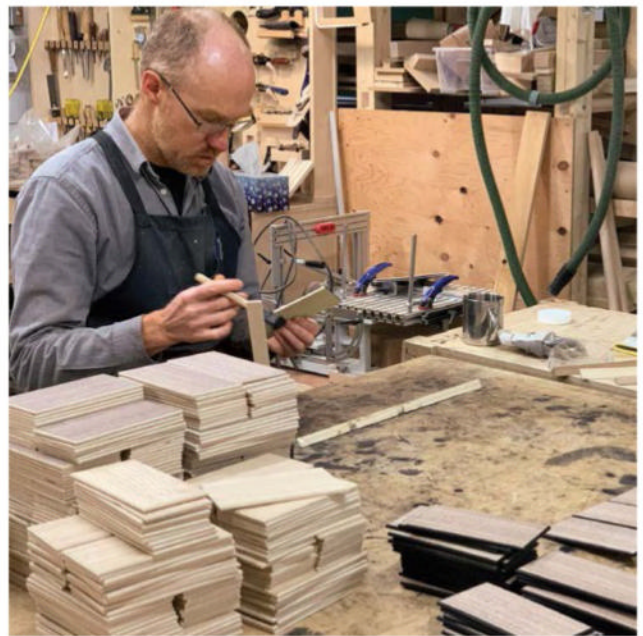
Screen gems. To make the cascading pattern on this standing screen, Solar arranged thin plywood tiles that he veneered variously with white oak, two tones of walnut, and silver leaf.
