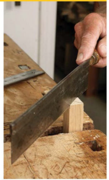
Good practice. For a better hold in the lathe, punch a center mark with an awl and saw kerfs on the diagonals for the drive center to grab.
