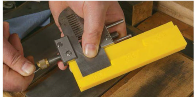
Sharpening setup. An easy-to-print jig to set the bevel angle on a honing guide is handy around the shop. The PLA material is easy to clean and, with its bright yellow color, hard to lose.
