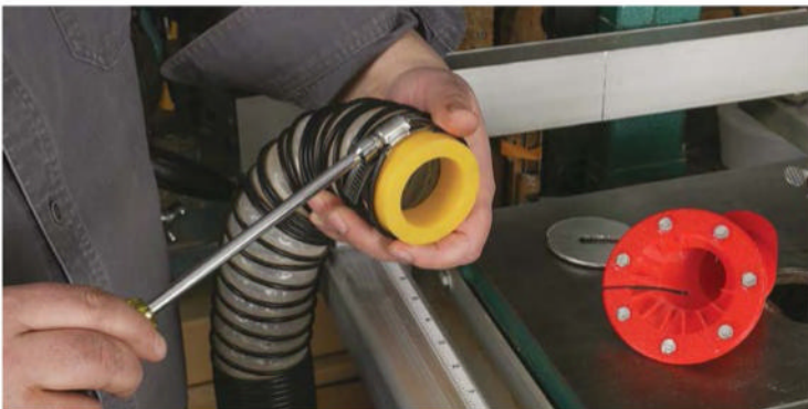
Versatile dust extraction. This effective port allows ideal dust collection at the bandsaw. Magnets embedded in the print hold the port in place but allow easy removal for regular maintenance. Add a coupler to increase your hose diameter when the dust really starts to fly.
