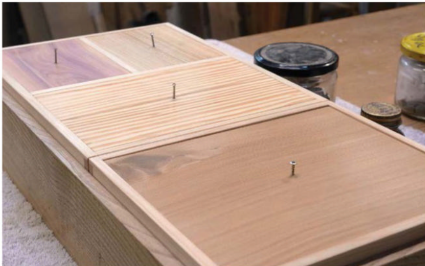
Challenger. The design of Martin's sewing box was determined in part by a challenge he set for himself: to make two inner boxes with a flawless piston fit inside an outer one.
