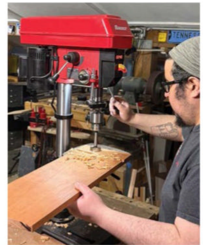
Enough power. The Bauer didn't bog down when aggressively drilling in cherry with a 2-in. Forstner bit.
