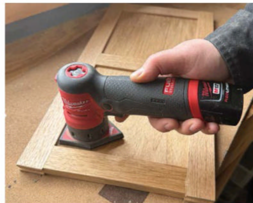
Put baby in a corner. The head of the sander can be rotated in almost any orientation. In Strano's shop, the sander lives with the point going backward, but he can easily spin it around using just an Allen key.
