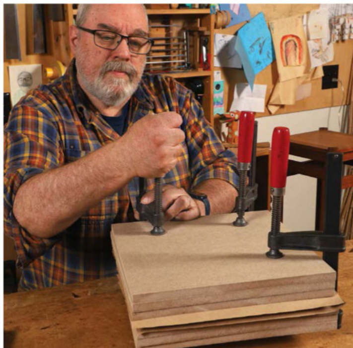
Plenty of pressure. For a panel of this size, cauls and F-clamps provide all the pressure you need to make a flat and flawless veneer lamination. For much larger panels, a vacuum bag simplifies the process.
