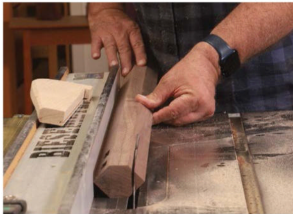
Rip the fifth face. Return the table saw's blade to 90° and make a rip cut to create the outer-facing fifth facet of the leg.
