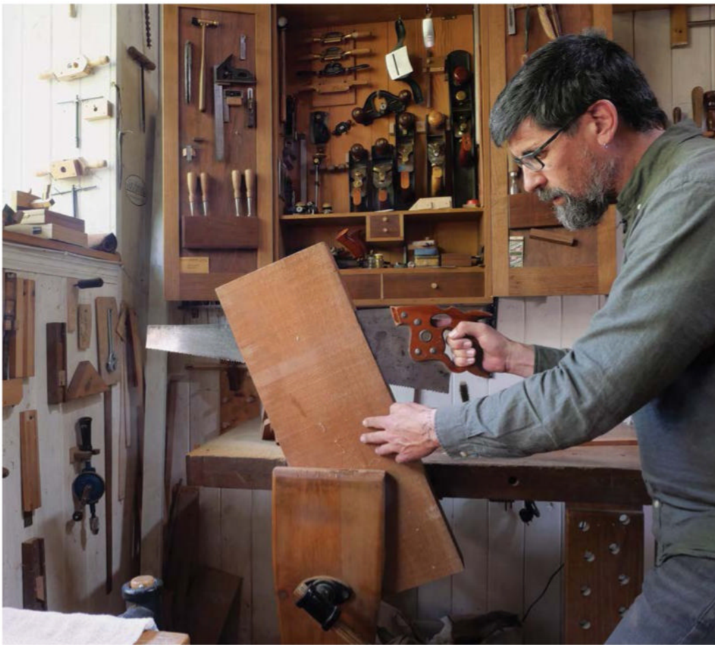
The elbow is the engine. Martin's dedication to handwork begins with dimensioning. Here he resaws red cedar. The Swedish pine sides of the inner boxes were resawn from reclaimed beams.
