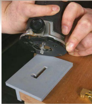
Frustration-free knife hinges. Mortising for knife hinges can be tricky, but Strano designed a template to work simply with a router, leaving minimal chisel cleanup for a perfect pressure fit.
