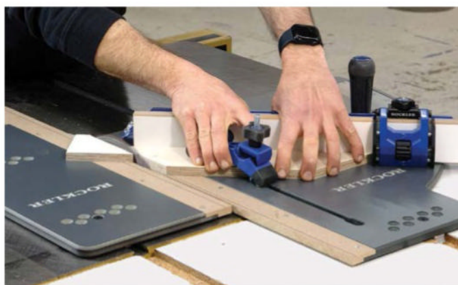
Future proof. The zero-clearance inserts are made out of ¼-in. MDF, but replacements could be replicated out of readily available sizes of MDF you probably already have in your shop.
