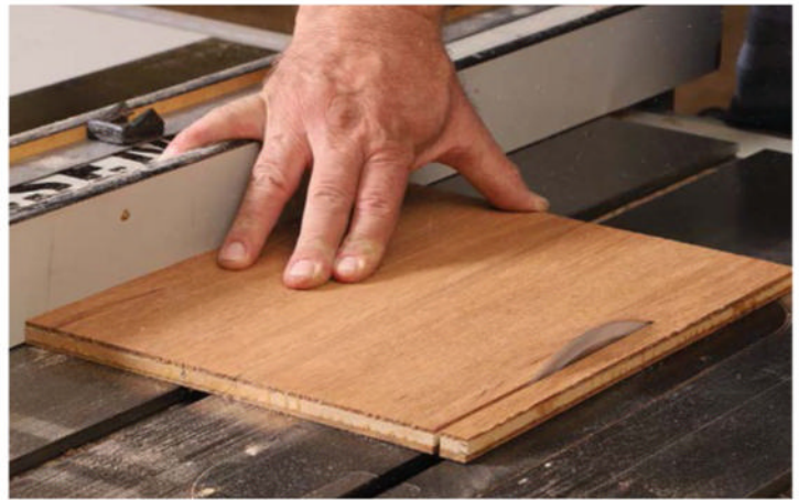
A perfect rip. After using a story stick to set the table saw's fence, Stevens rips the panel to width.
