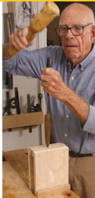
Split the handle. Setting the chisel parallel to the handle's grain makes for a nice clean split.
