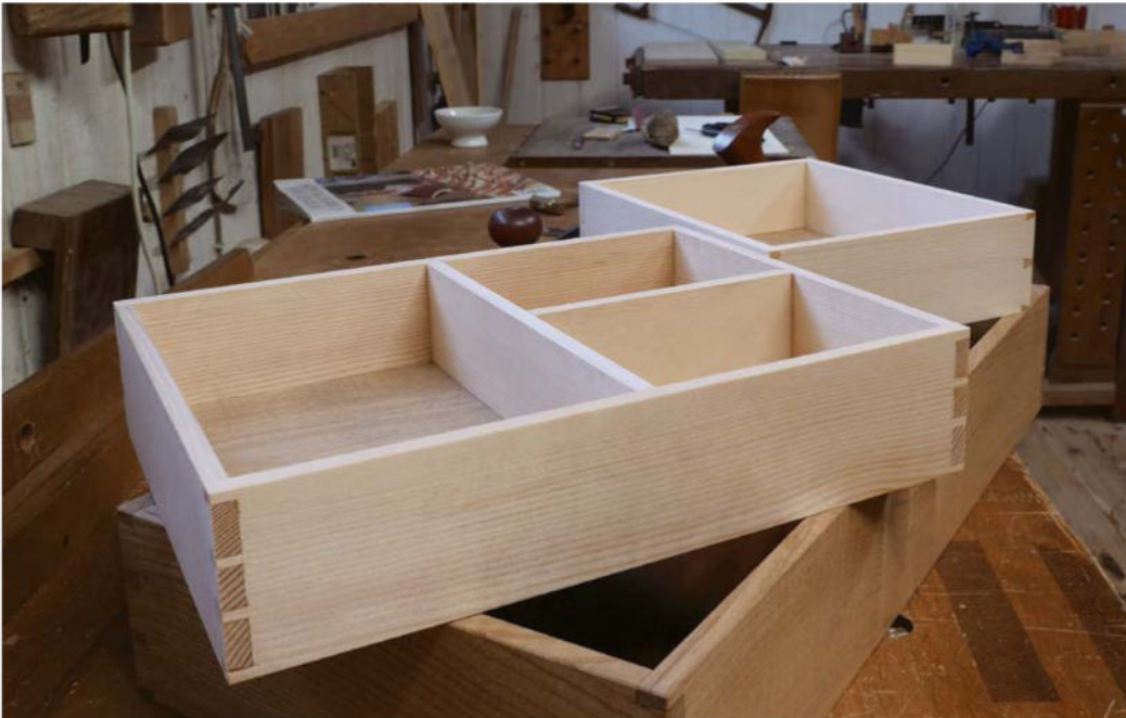
Challenger. The design of Martin's sewing box was determined in part by a challenge he set for himself: to make two inner boxes with a flawless piston fit inside an outer one.
