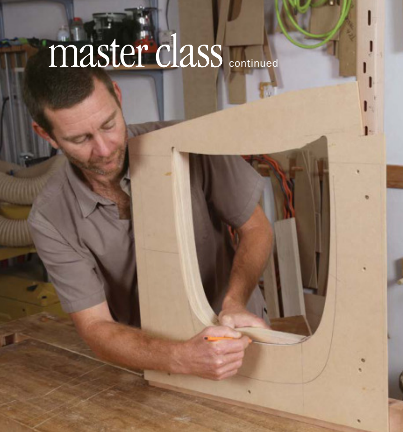
Inner leg shape. This jig tackles the curve of the inside of the leg assembly. Set the piece on the jig into the 90° fence and trace the curve.
