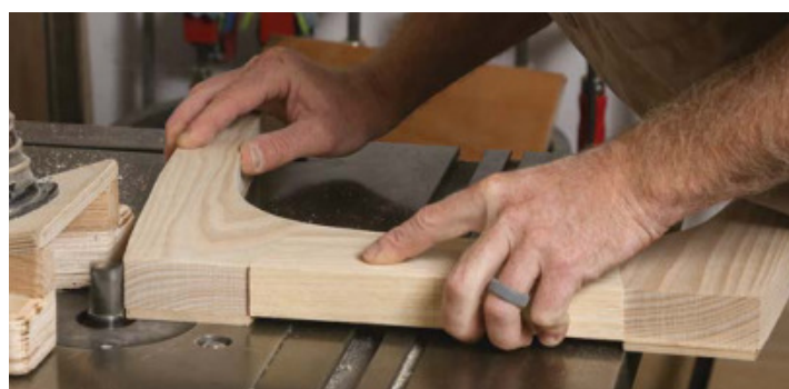
Outer leg shape. Tape the leg templates to the bandsawn outer edges of the legs (left), and template-rout the exterior to final shape (above).
