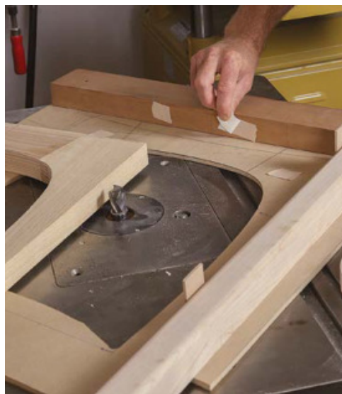
Inner leg shape. This jig tackles the curve of the inside of the leg assembly. Set the piece on the jig into the 90° fence and trace the curve.
