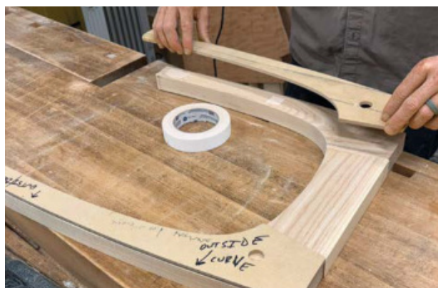
Outer leg shape. Tape the leg templates to the bandsawn outer edges of the legs (left), and template-rout the exterior to final shape (above).
