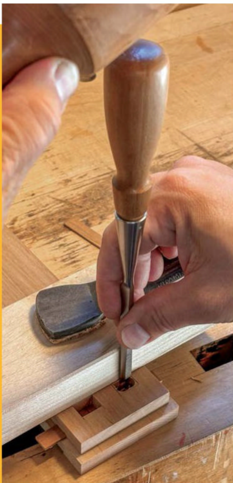
Clean up. Insert a sacrificial strip of wood in the dado to avoid blowout during chopping. Use a chisel to square up and clean out the walls of the mortises.
