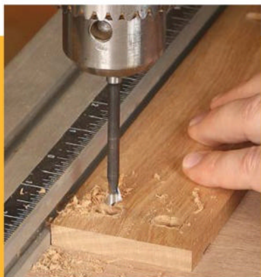
Drill first. Remove the waste with a Forstner bit on the drill press, being careful to stay inside the dado.
