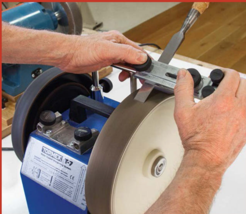
Speed test. Gochnour compared two CBN wheels to the standard Tormek wheel. The 200-grit CBN wheel (above) removed material roughly 20% faster than its 600-grit cousin, but twice as fast as the Tormek wheel (right).
