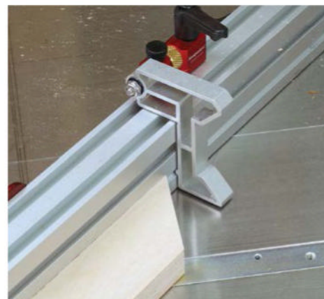
Smart features. The micro-adjustable flip stop includes a small tab that engages with the front of the fence to keep pointy miters from sliding past it.
