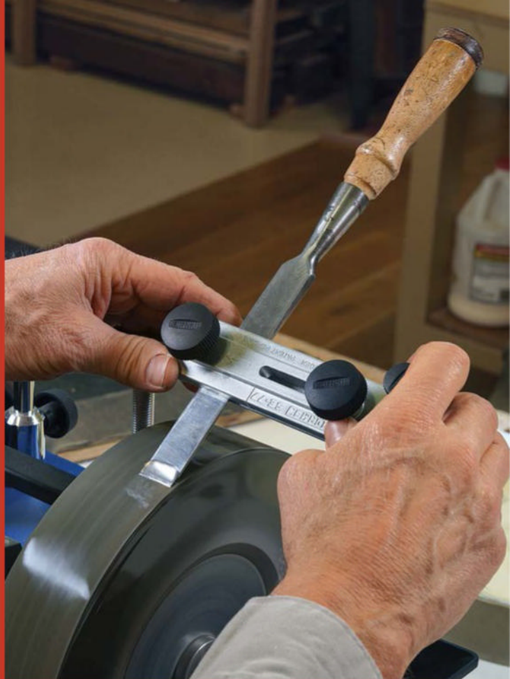
Speed test. Gochnour compared two CBN wheels to the standard Tormek wheel. The 200-grit CBN wheel (above) removed material roughly 20% faster than its 600-grit cousin, but twice as fast as the Tormek wheel (right).
