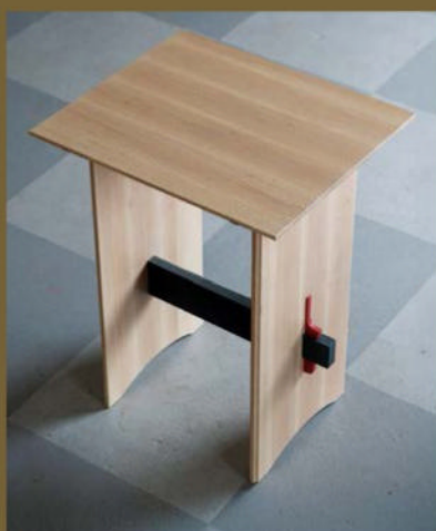
Traveling table and stools. The side table in ash, with milk-painted stretcher and tusk tenons, was made to be flat-packed. Tapered sliding dovetails join its thin legs and top. The jaunty stools with staked legs are a mobile take on a traditional milking stool.
