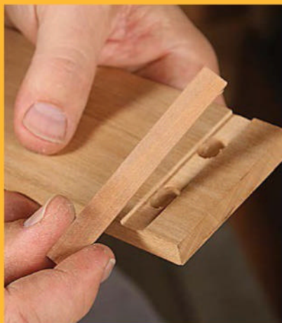
Clean up. Insert a sacrificial strip of wood in the dado to avoid blowout during chopping. Use a chisel to square up and clean out the walls of the mortises.
