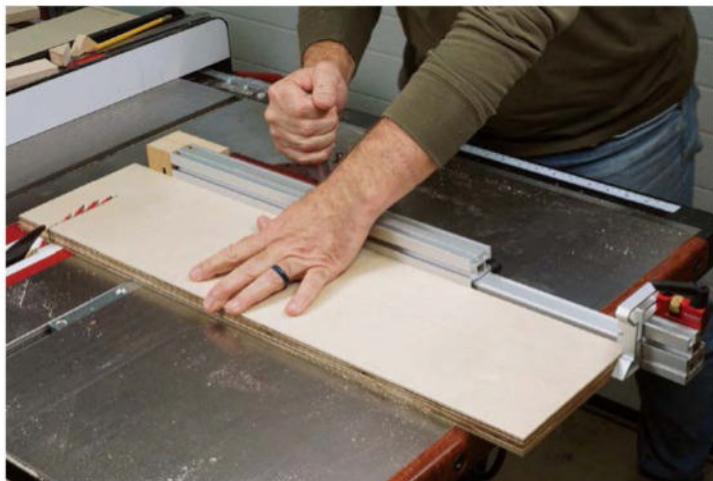
Big, accurate crosscuts. The fence extension and rock-solid flip stop allow repeat crosscuts up to 31 in. long. The spring-loaded indexing pin in the head guarantees that those cuts are square.
