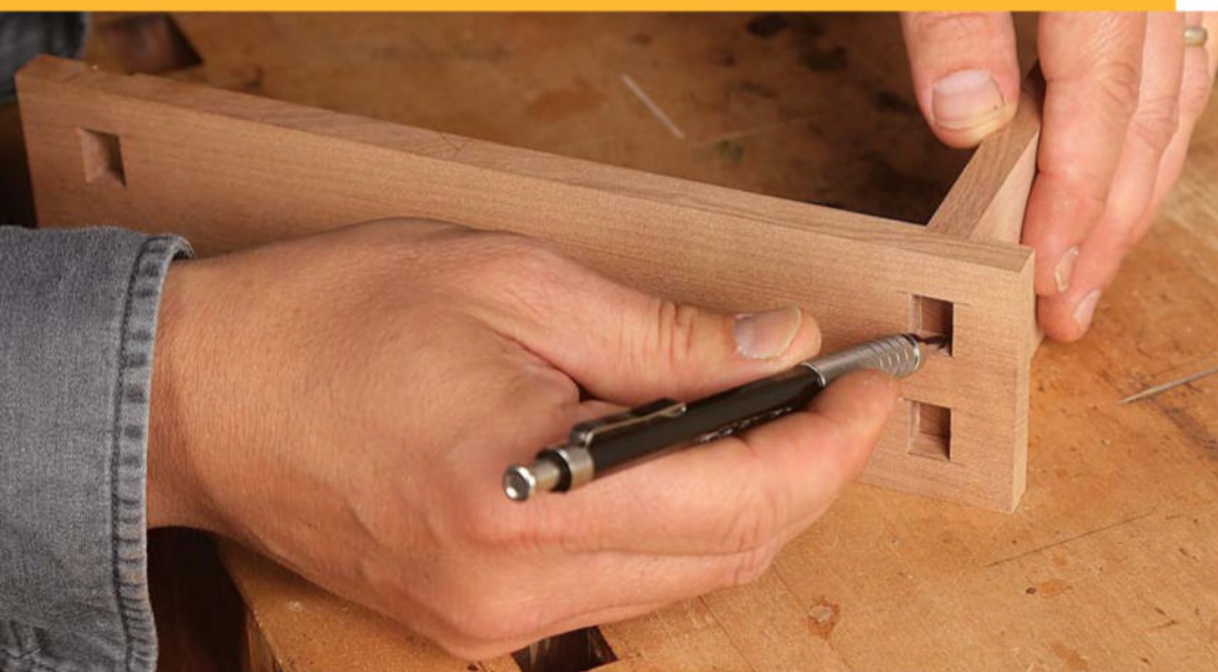
Transference. With the mortises cut and cleaned up, insert a short side into the dado, and use a pencil to transfer the mortise locations to the end of the short side.
