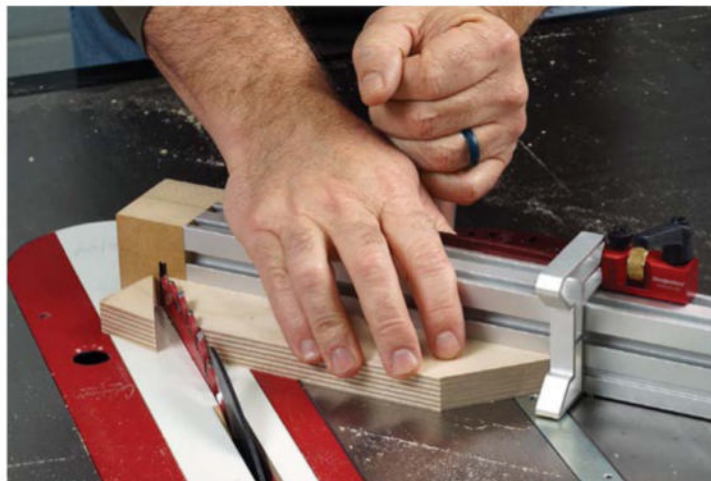
Miters are just as precise. The fence pivots easily from one angle setting to another and locks in each position securely and accurately.
