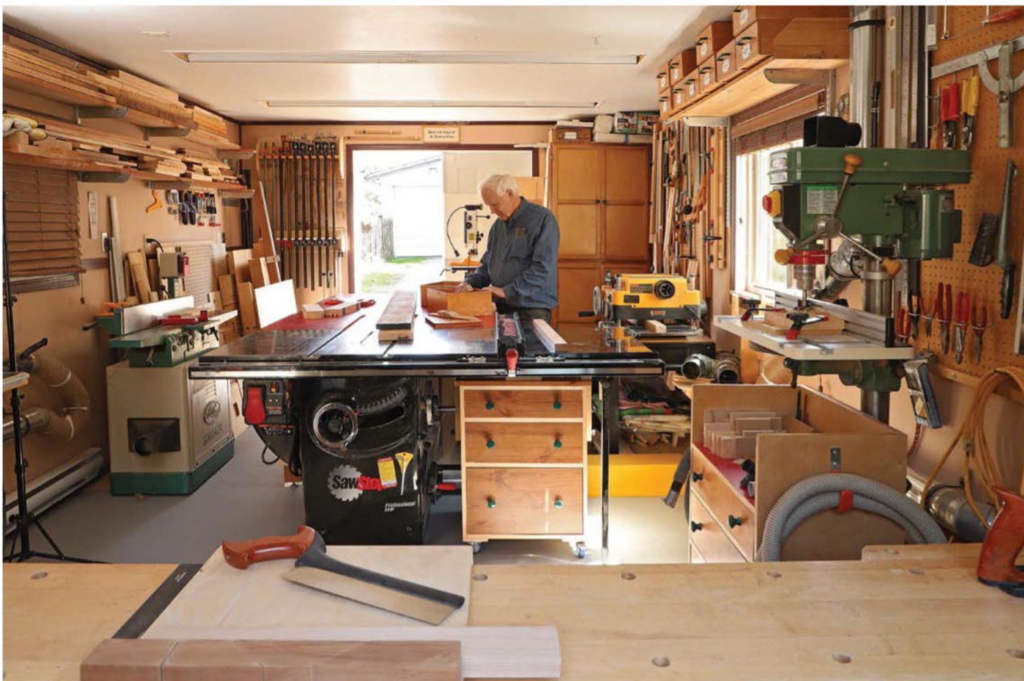
Snug and sensible. The table saw and its outfeed/assembly table anchor the center of McIvor's small shop, and his other machines hug the perimeter. Wall space is utilized for storage right to the ceiling. Fixtures recessed in the ceiling provide ample light without reducing headroom.
