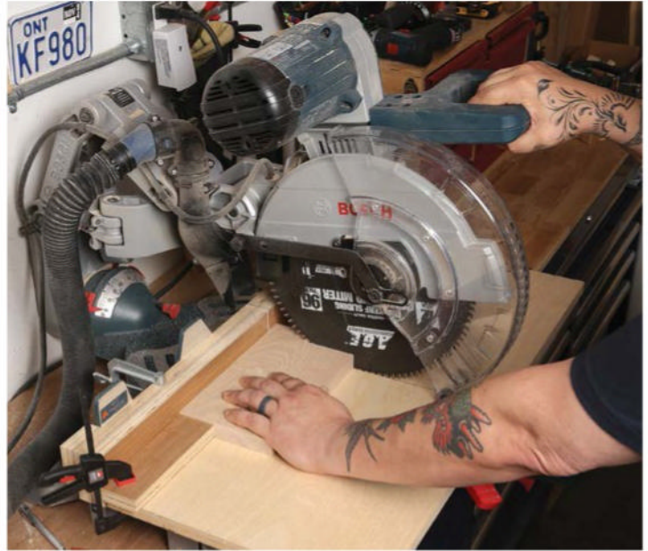
Miter-saw setup. An auxiliary table with a back fence attaches to the miter saw, creating a larger work surface and zero-clearance support for crosscuts. It also allows you to easily add stops for repeatable results.
