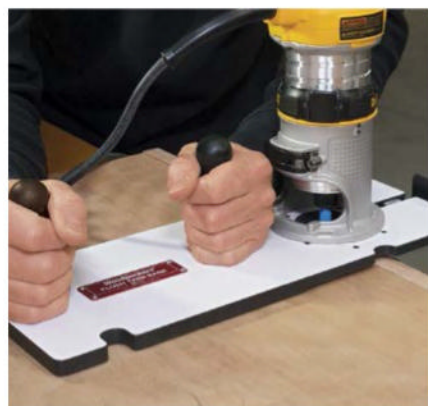
Trim edge-banding quickly and accurately. The stiff plate keeps the router level and slides easily over the surface.
