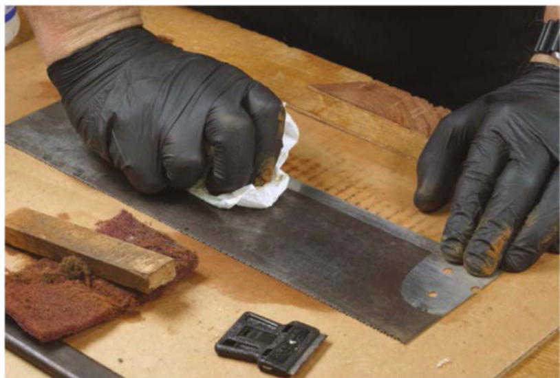
Wipe off the gunk. Use a cotton rag to wipe away the grime you've lifted off the blade plate.
