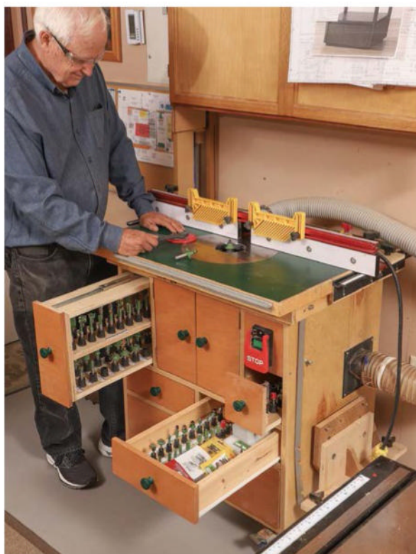
Stacked with storage. McIvor's router table provides easy-access storage for scores of router bits. Handheld routers and accessories fill the lower drawers.
