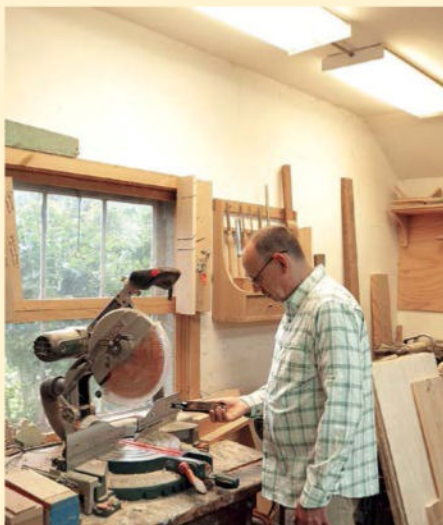
Measure at working height. By taking your readings just over bench or tool height, you will focus on the points that matter most—where the work is being done.
