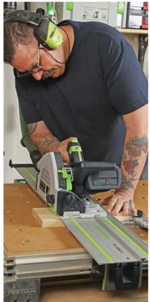
A hinged guide rail and track saw. Working on an MFT (multifunction table) makes it easy to square up and secure workpieces against a fence and stop. With the flag stop set, you can ensure repeatability and accuracy.
