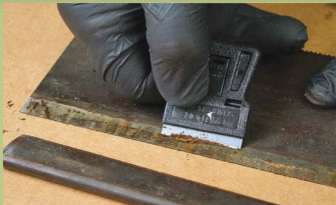
Scrape away the grime line. Use a razor to scrape away the line of grime and debris that builds up where the back meets the blade.
