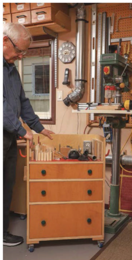
Stacked with storage. McIvor's router table provides easy-access storage for scores of router bits. Handheld routers and accessories fill the lower drawers.
