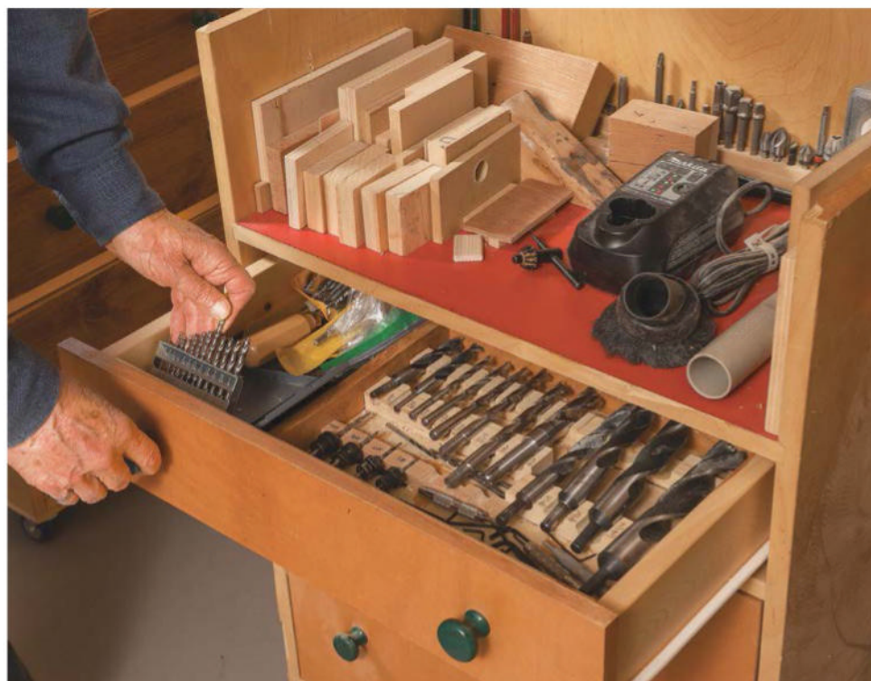
Drawers dedicated to the drill press. The chest that sits below McIvor's floor-model drill press holds a wide array of bits and drilling accessories. Built on casters, it can be rolled away from the drill press when McIvor needs to lower or tilt the table to drill large workpieces.
