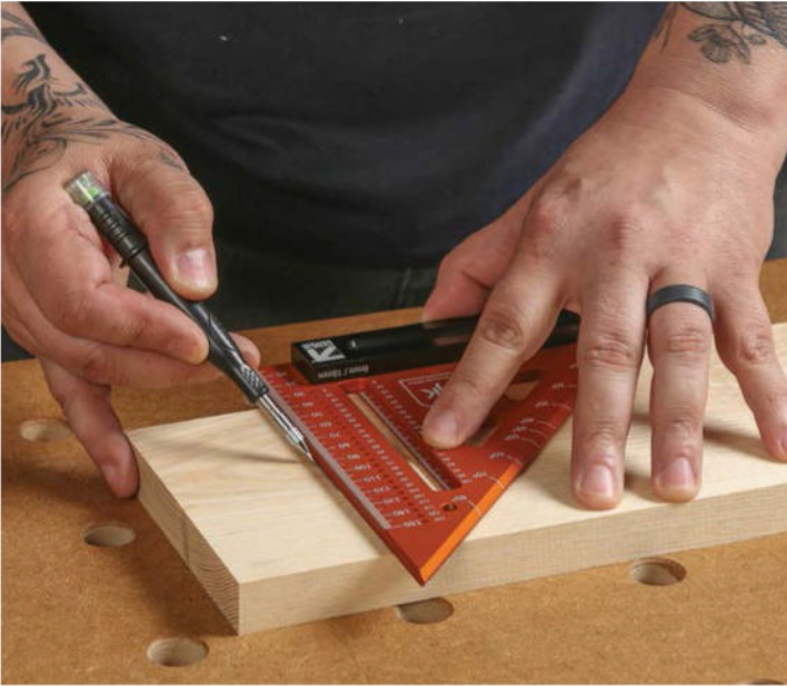
Strike a line. All accurate cuts start with good layout lines. Reliable squares and a good pencil are a must.
