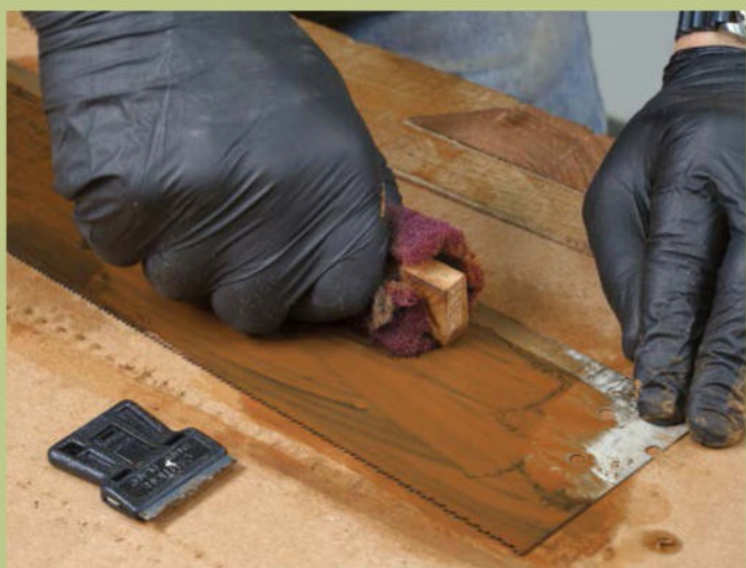
Scrape away the grime line. Use a razor to scrape away the line of grime and debris that builds up where the back meets the blade.
