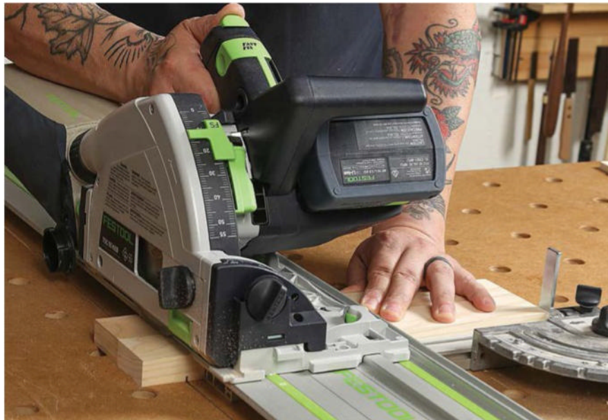
Shoulders via the track saw. The advantage of cutting shoulders on the track saw is that you can lay like pieces side-by-side and cut multiple shoulders at once. Set your blade depth and go.
