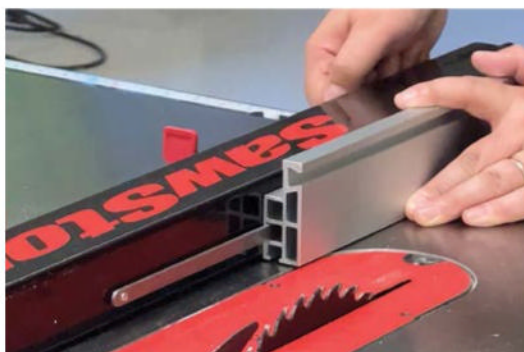
Smart stop block. The face is adjusted with three cam locks on the right side of the fence tube. Loosen the locks and pull the fence back clear of the blade, and you can use it as a stop block when crosscutting with your miter gauge. The rip fence's scale indicator will give you the correct reading for the crosscut.
