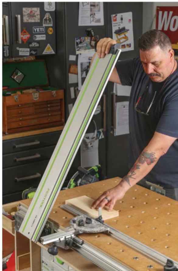
A hinged guide rail and track saw. Working on an MFT (multifunction table) makes it easy to square up and secure workpieces against a fence and stop. With the flag stop set, you can ensure repeatability and accuracy.
