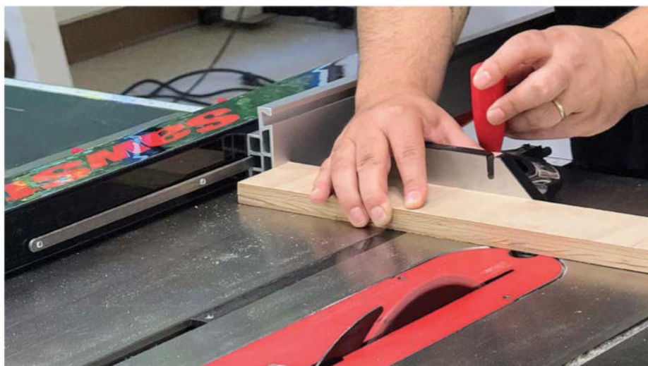
Ups and downs. The fence face is easily switched between its high and low orientations. There are dual scale indicators, one for the high position and one for the low. The face can also be used as an L-fence.
