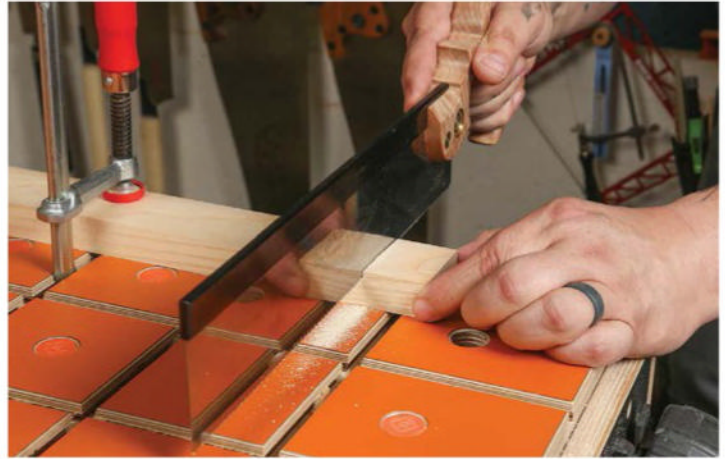
Shoulders by hand. Sometimes ditching the machines and cutting shoulders with a handsaw is most efficient, since there is no setup time.
