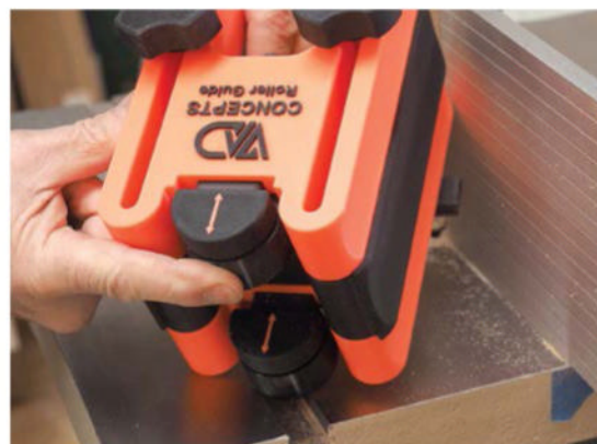
Spring assist. The spring-loaded wheel helps immensely with cuts where a variance in pressure against the fence or the table could make the workpiece unusable.
