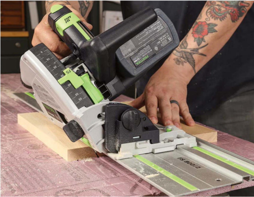
Track-saw beveling is a breeze. Working again on a piece of rigid foam insulation, line up the track with your marks, tilt the blade, and make your cut. The foam keeps your workbench from being scarred with kerf marks.
