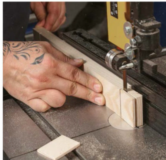
That's cheeky. The bandsaw is well suited for cutting the cheeks of a tenon. With the aid of a fence to keep things straight, the surface right off the saw is usually good enough to go straight to glue-up.
