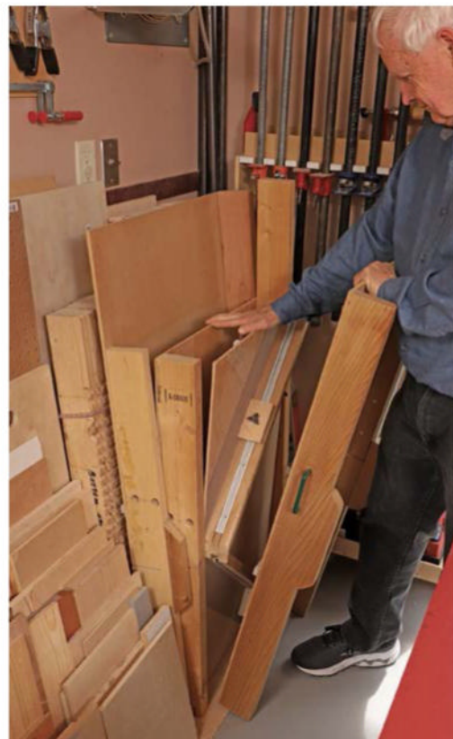
Nesting sleds. Mclvor built his many table-saw crosscut sleds with different front-to-back dimensions so they could nest inside each other for more-efficient storage.
