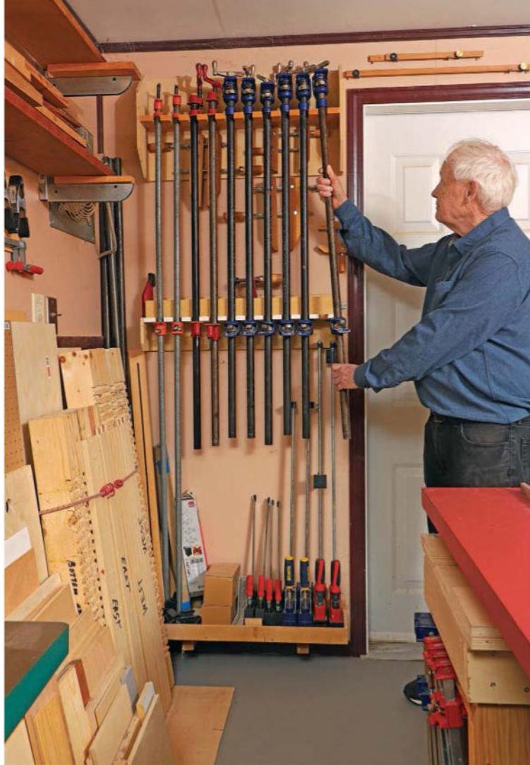
Interlacing long clamps. The wall-mounted rack Mclvor made accommodates pipe clamps hanging above and parallel-jaw clamps between them, supported on a shelf below. Hand-screw clamps laid flat to the wall hang behind the pipe clamps.
