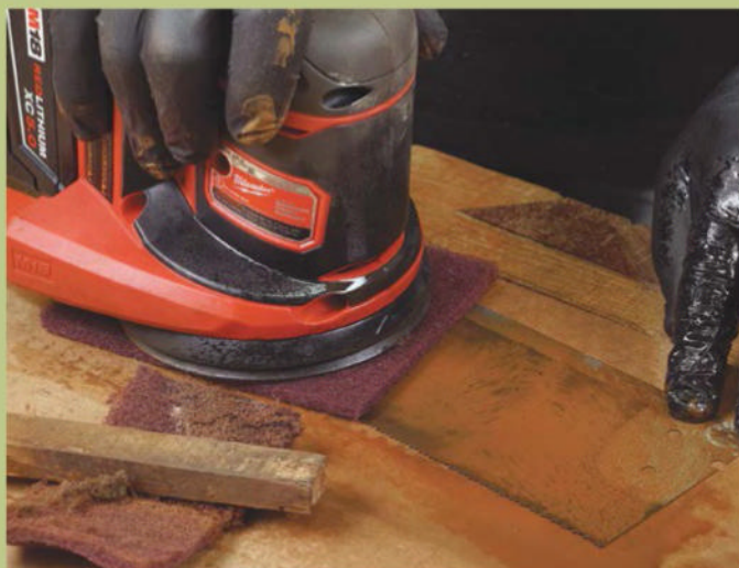
Abrade the blade gently. With alcohol as a lubricant, use abrasive pads to begin removing the grime on the blade. You can do this by hand or with the assistance of a random-orbit sander placed over the pad.
