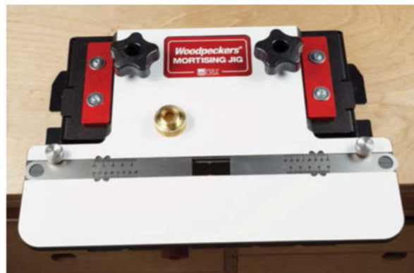
Slick top. The top is covered with low-friction laminate, and it slides fore and aft to position mortises on a workpiece. Sliding rulers control mortise length.
