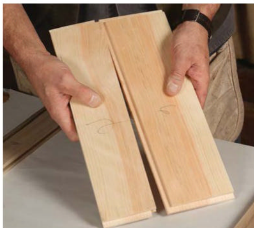
Rails first. Before gluing the rails into the legs, glue them to each other.
