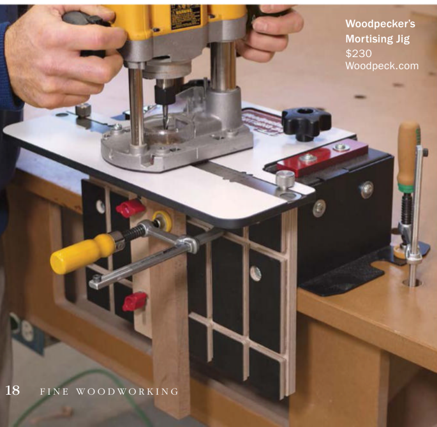
Fast, accurate mortises. The jig works with your plunge router to cut mortises up to ½ in. thick and 3½ in. long. Add clamps and simple fences to hold workpieces in a variety of positions.
