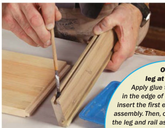
Rails first. Before gluing the rails into the legs, glue them to each other.
