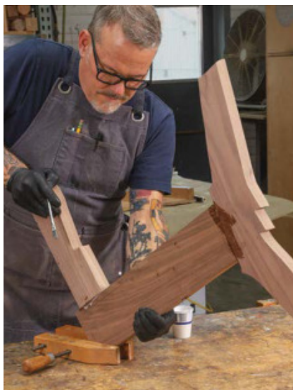
Slow assembly. Epoxy's long open time permits you to assemble the whole side (except for the armrest, which is added later) in one go. A hand-screw clamp keeps the parts upright as you seat the front leg.
