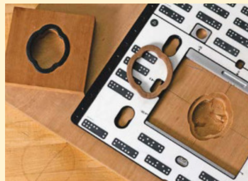
Pierced tsuba detail with ebony inlay. Shaper Plate brings the Origin router to any surface, and Origin does the rest. All that's left is a bit of work to soften the edges of the inlay.
