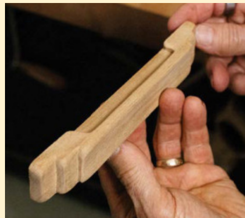
Cloud-lift drawer handles. Origin handles the bulk of the shaping on these drawer pulls, making them more uniform and much faster to manufacture.
