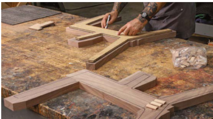
Place and trace. With all the side parts sawn out and their mating surfaces flattened, put them in position and trace the finished template onto them. Also, mark the joints for Dominos.
