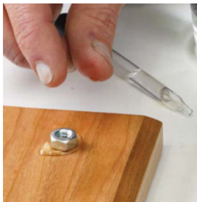
Tough test. To assess the durability and protection of hard-wax oil finishes, the author wet the surface of each test board and placed a steel nut on top, checking the effect in 3-hour intervals.
