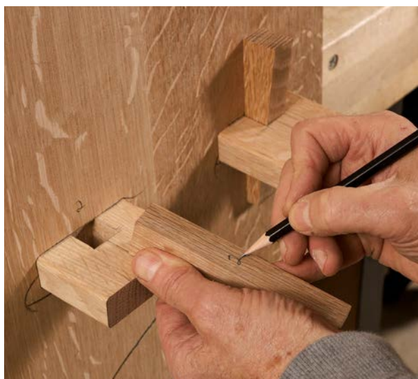
Custom fitting. A clean fit of the tusks is key both functionally and visually. Hartman fits each one individually, tweaking with a handplane where necessary, and labels each to its mortise.
