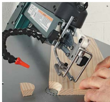
Angled cuts are easier. The head tilts on Grizzly's new scrollsaw, not the table, letting the work stay level. The dust port is very effective.
