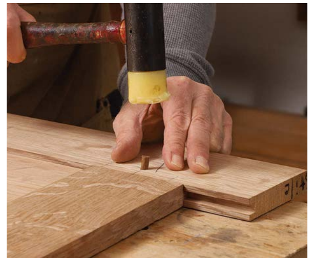
Peg it. Hartman glues the frame and locks it tight with drawbore pegs.
