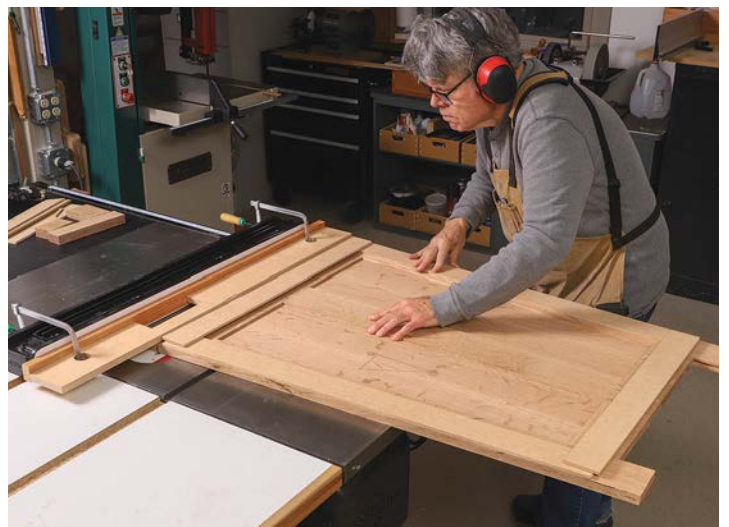
Template in practice. Having built the back slightly oversize, Hartman used double-stick tape to attach the trapezoid template to the assembled frame. Then, with an L-fence clamped to the table saw's rip fence, he ran the template against the L-fence to cut the back to final shape.
