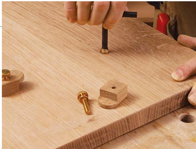
A twist under the top. To attach the top, Hartman made buttons that twist into slots cut into the case sides. Bolts with knurled knobs fit into threaded inserts to secure the buttons and make the case easy to knock down and reassemble.
