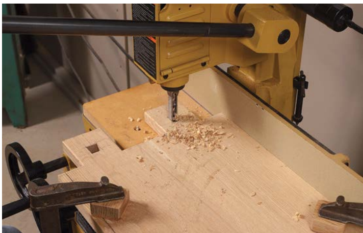
Tusk mortises start by machine. After dry-fitting the through-tenons in the case sides to facilitate layout of the tusk mortises, Hartman cuts them with a hollow-chisel mortiser.
