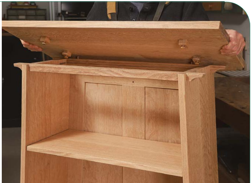
A twist under the top. To attach the top, Hartman made buttons that twist into slots cut into the case sides. Bolts with knurled knobs fit into threaded inserts to secure the buttons and make the case easy to knock down and reassemble.
