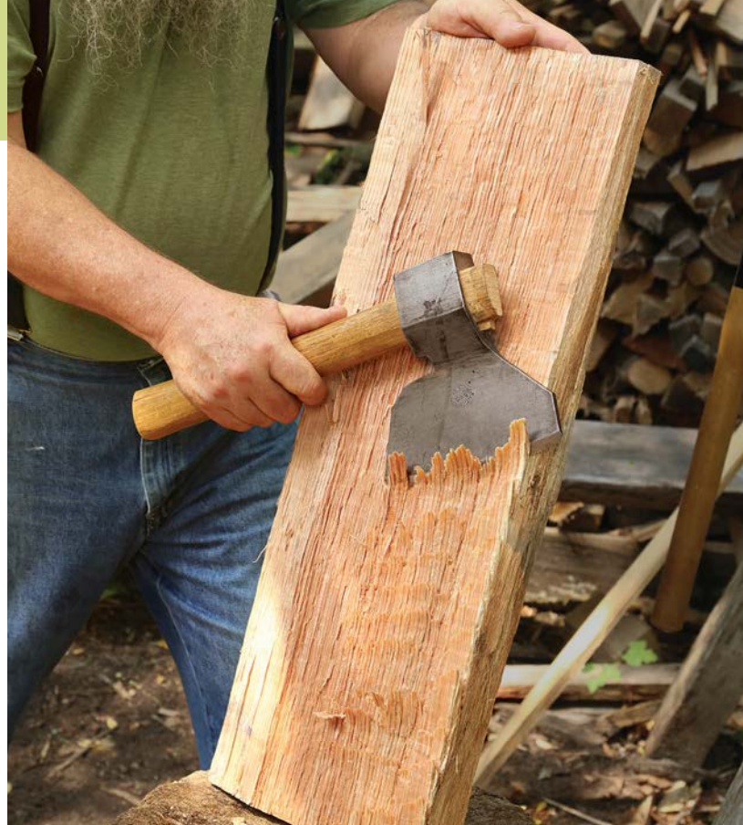
Prep for planing. Keep your leg tucked behind you for stability and safety. Make scoring cuts at an angle, working from the bottom toward the top, but not all the way. Then lightly swing the hatchet from the top down to break off the scored fibers. Repeat until you reach the desired thickness. Flip the stock end-for-end to finish the full length.
