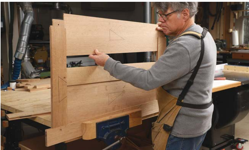
And angled panels. The back panels, their outside edge cut to the familiar 3° angle, get dropped into place dry.
