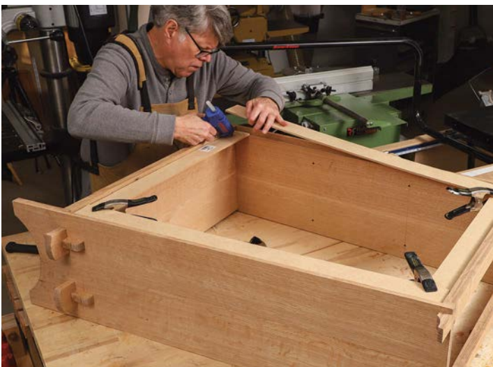
Template for a trapezoid. Instead of trying to measure the opening for the back, Hartman created a template of the shape by inserting four strips of \frac{3}{4} -in. MDF into the rabbets and grooves where the back will be fitted, then hot-gluing the strips to each other at the corners.
