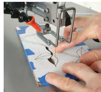
Marquetry champ. Vibration is minimal and the blade is held tightly, making precise marquetry cuts easy to achieve.
