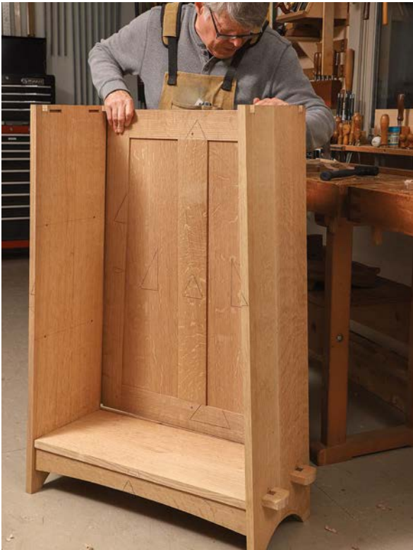
Backing in. With the sides slightly loose, Hartman fits the back into the side rabbets and drops the tongue at the bottom into its groove.
