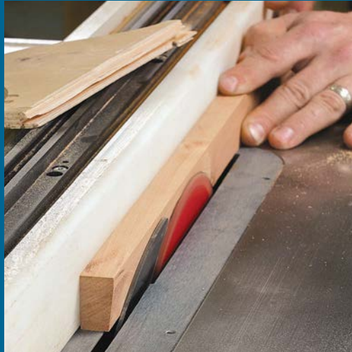
Shape the parts. Bevel the edges of the parts, rabbet them for the grill fabric, and bandsaw curves along their inside edges.
