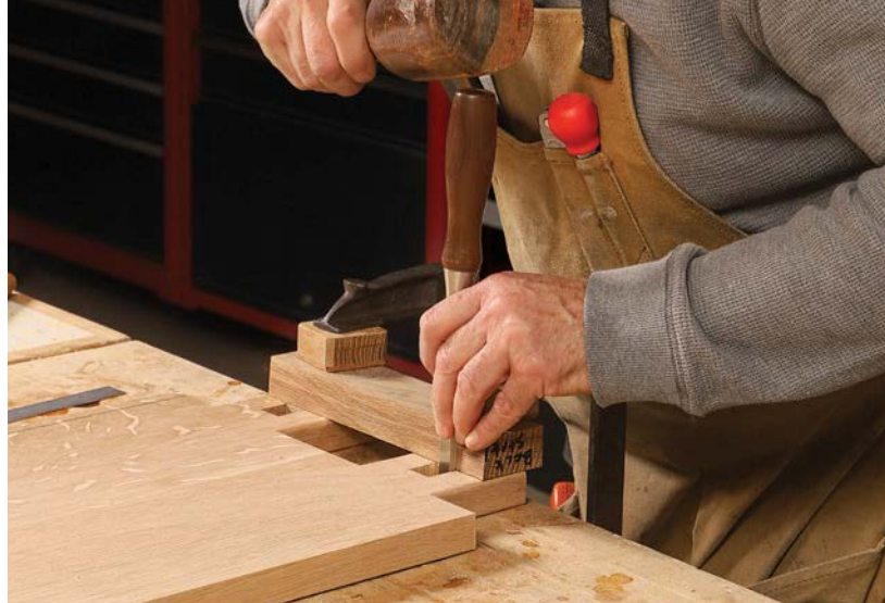
They end at the bench. Hartman clamps an angled guide block to the tenons as he chops the outer wall of the tusk mortise. The tusk is tapered at 7°; since the case side is canted 3°, the guide block is angled at 4°.
