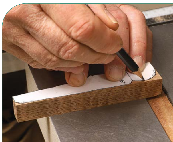
Paper template. Once the tapered tusks are fitted, Hartman traces a paper pattern to define their decorative shape. He'll follow the layout lines with careful bandsaw cuts and clean up with an edge sander and some filing and hand-sanding.
