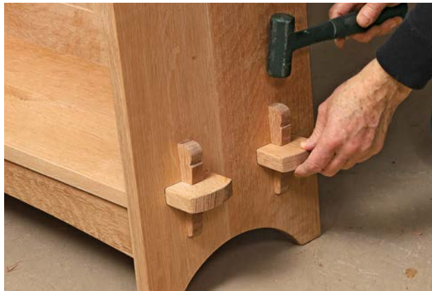
Lockdown. Fit the stretchers into their notches, pressing them down flush with the sides. Then knock home the tusks to lock the sides tight.
