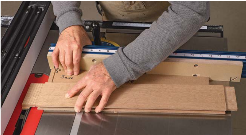
Angled frame tenons. The frame-and-panel back is tapered to match the case. Here, using his 3° wedge against the miter gauge, Hartman cuts the rail tenon at the table saw with a dado blade. The rip fence acts as a stop for the shoulder cut.
