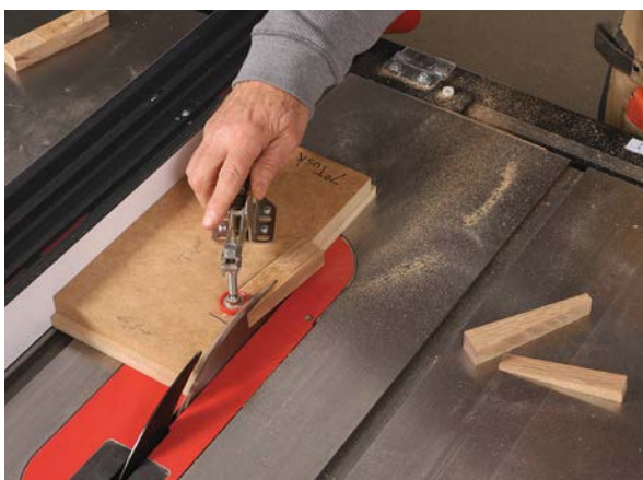
Tapered tusks safely sawn. To cut his 7° tusks safely, Hartman made a jig from two layers of MDF. The top layer has a toggle clamp and a 7° notch to fit the tusk blank; the bottom layer supports the blank, enabling it to be clamped.
