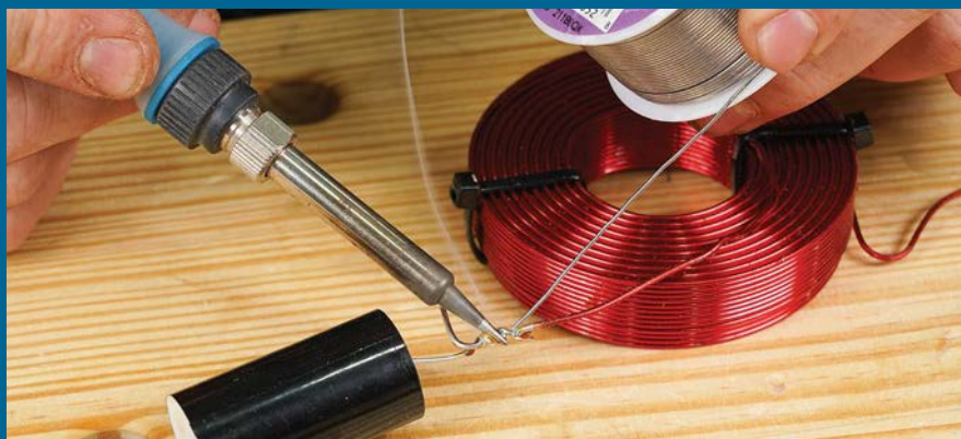
Step 3: Heat the joint and add solder. Apply heat to the joint for a few seconds, and then melt solder into it. Be sure to heat the wires and let them melt the solder, rather than trying to melt solder onto a cold joint.
