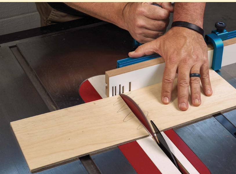
Real-world cuts. Christiana made multiple square cuts, resetting the angle each time, to check for consistency (above), and made a mitered frame with each gauge (right) as well, which compounds any error in the 45° setting.
