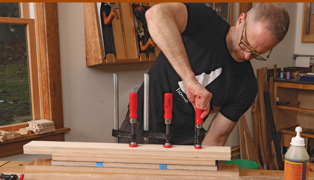
Lamination. With cauls top and bottom to spread the clamping pressure, Korsak glues sheets of shopsawn veneer to both faces of the apron's Baltic-birch substrate. Blue tape keeps the veneer from shifting before the glue tacks.
