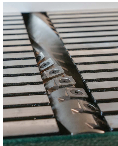
Top-notch cutterhead. The helical cutterhead has two spiraling rows of four-edged carbide teeth, which produce amazing surfaces on the toughest woods.
