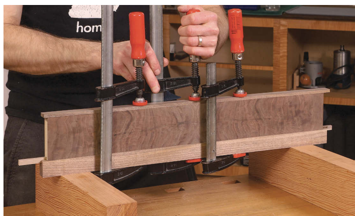
On with the edging. Korsak glues the spline and edging to the apron. The edging is flush to the inside of the apron and proud of the outside.
