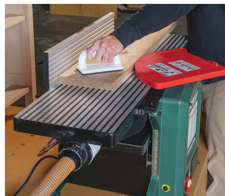
Jointer mode. Switching to jointer mode requires remounting and resquaring the fence, lowering the planer bed, and relocating the dust shroud. Dust collection is very good with a shop vacuum (shown), and even better with a full-size collector.
