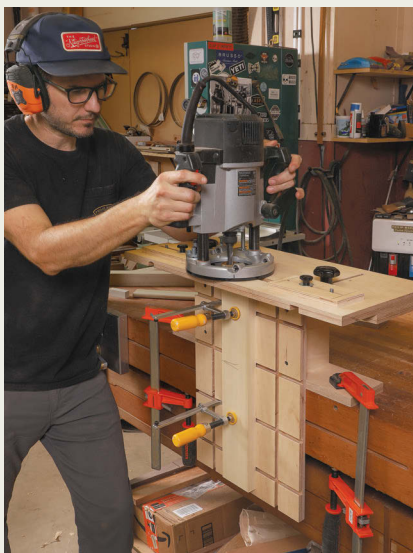
A smart solution for slip-tenon joinery. Philip Morley's routing jig offers an affordable alternative for cutting fast and accurate mortises in parts of any shape.
