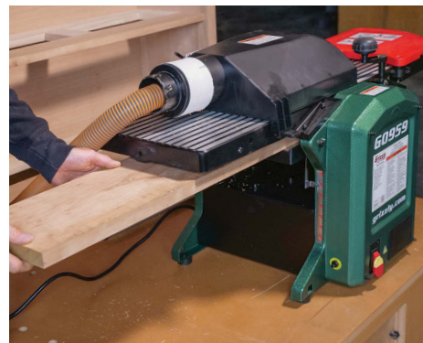
Planer mode. The jointer tables stay in place in planing mode, so you'll have to reach under them to feed and retrieve short workpieces. The planer's effective depth of cut is limited to roughly \frac{1}{32} in. on hardwoods.
