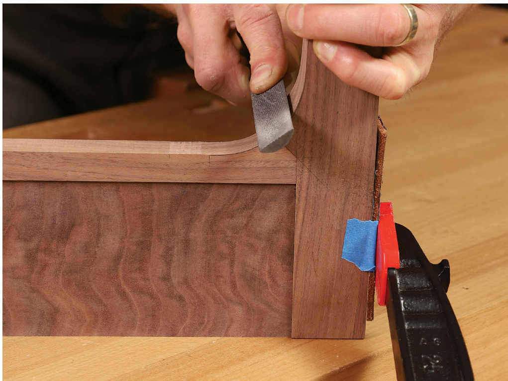
A clean sweep. The curve below the gunstock miter needs to look continuous from the leg to the apron. Korsak fairs it with a curved file and later finesses it with sandpaper.
