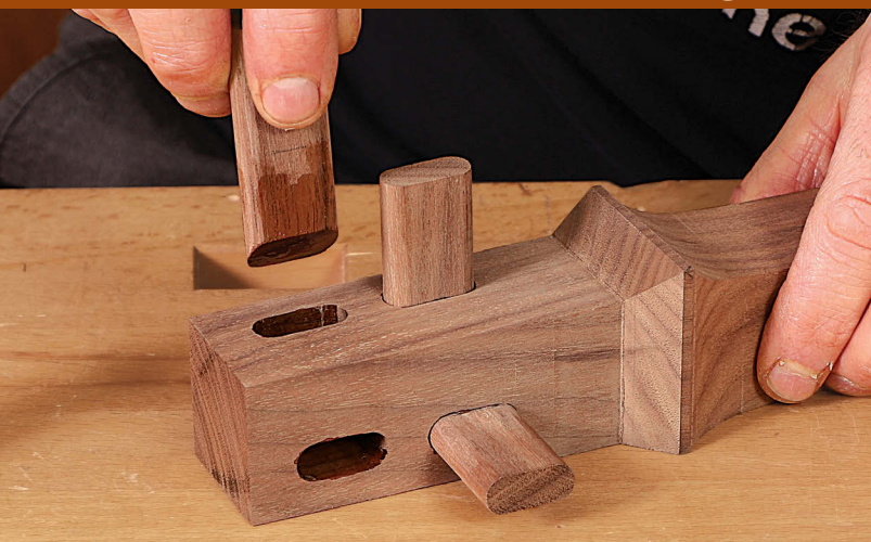
Securing the slip tenons. After spreading glue in the mortises and on the mitered end of the slip tenons, Korsak glues them in place, making sure he gets contact between the miters.
