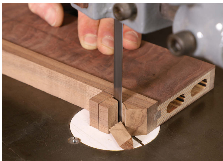
Relieving the edging. Once the miters at both ends of the apron edging are cut, Korsak bandsaws away the waste between them.
