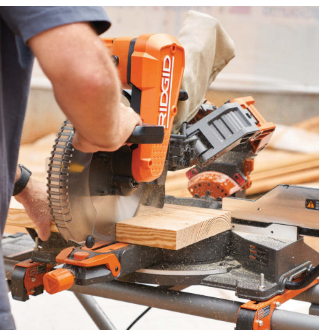
Arms for heavy lifting. The smooth-acting slide mechanism gives the Ridgid R4241 a nearly 16-in. crosscut capacity, and the articulating arm makes it possible to cut 5¼-in.-tall baseboard against the fence.
