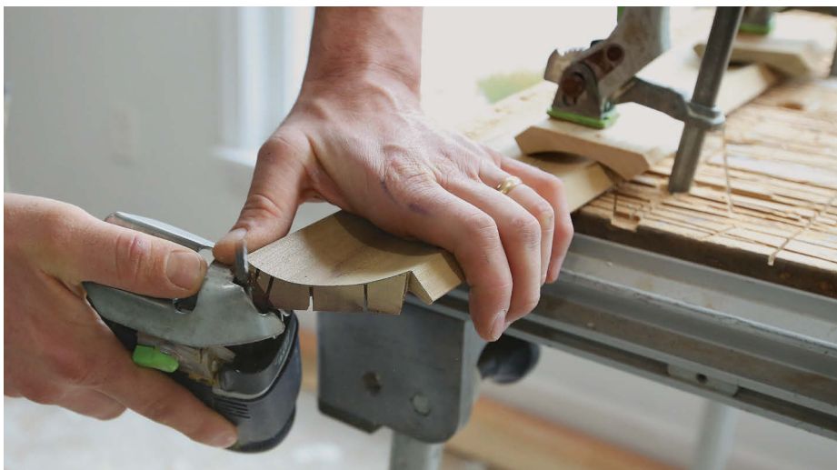
Better jigsaw coping. A well-known secret among trim carpenters, the Collins Universal Coping Foot lets you use nearly any jigsaw to easily cope all kinds of trim and moldings.
