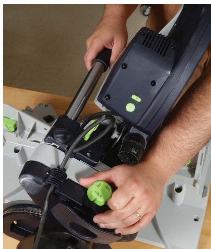
Bevels are a breeze. A rotating knob limits the range of overall travel left and right. A micro-adjust knob on the front allows precise bevel adjustments.
