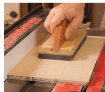
Miter the fence and base. Leave a small flat at the tip of the miter to aid with assembly.
