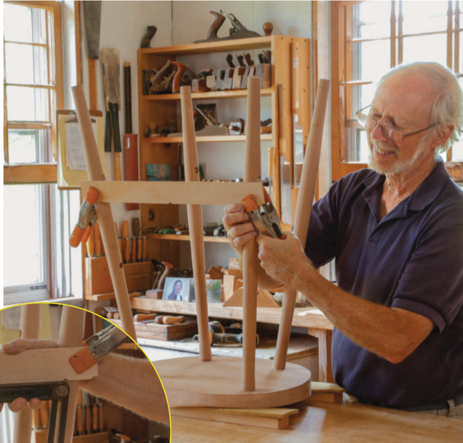
Mock up the stool to get the drilling angles for the front and rear stretchers and foot rest. The holes for the stretchers and foot rest need to be drilled at an angle. Get this by putting the legs into the seat and clamping a straightedge across the stretcher location (above). Then adjust a bevel gauge until it sits in line with the leg. This is the angle for that hole. Repeat the process for each leg.
