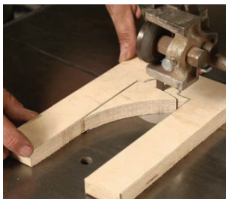
Bandsaw the platform frame. A simple U-shaped frame that's the same overall size as the routing template surrounds the feather platform and holds the template in place.
