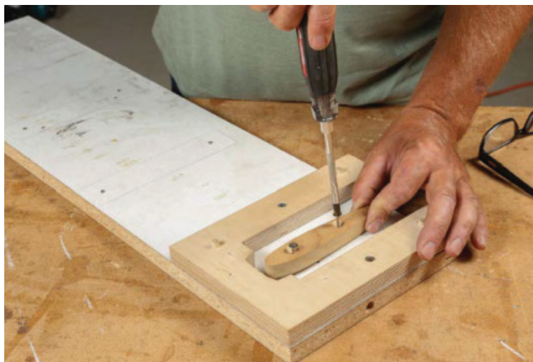
Feather platform. Trace the paper template you started with onto a scrap of wood, and cut the shape on the bandsaw to make the platform that holds the feather blank while routing. Finally, drill and screw it and the frame to a piece of plywood or other sheet good.
