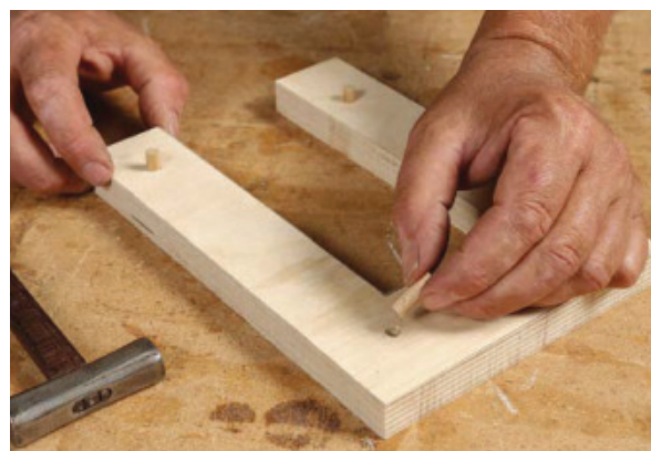
Dowels locate template to frame. Tape the template to the frame, and drill dowel holes in both. Then glue and tap dowels into the frame. The dowels hold the template still during routing, but it's easy to pop the template on and off.
