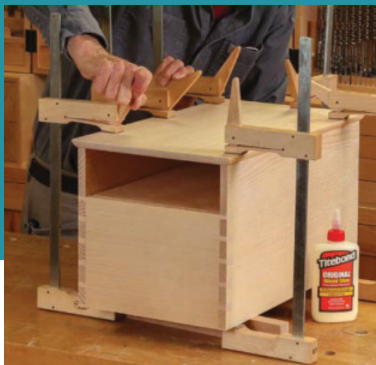
Glue the bottom to the case. Center the case on the quartersawn bottom, and glue and clamp it in place.
