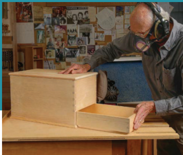
Fit the drawer. Becksvoort uses a belt sander to fine-tune the fit of the drawer.
