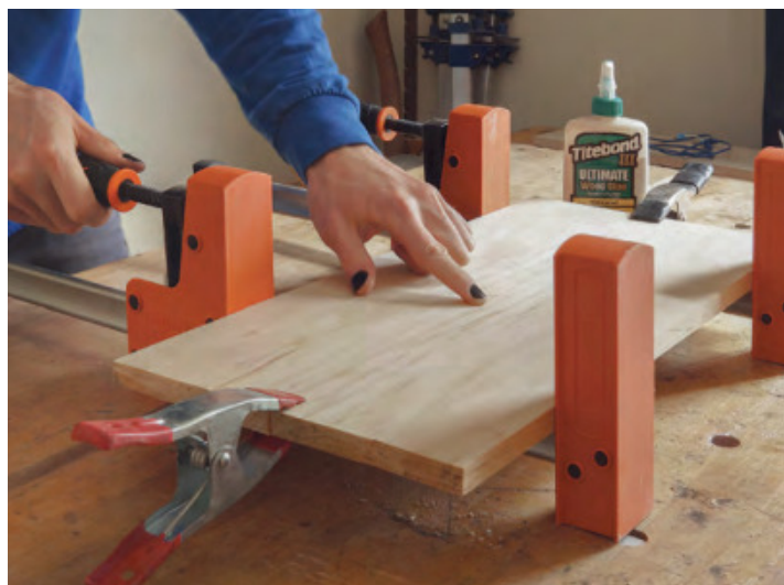
Glueline rip blade lives up to its name. Test boards' edges were glue-ready off the blade, yielding a joint that was tight and free of gaps.
