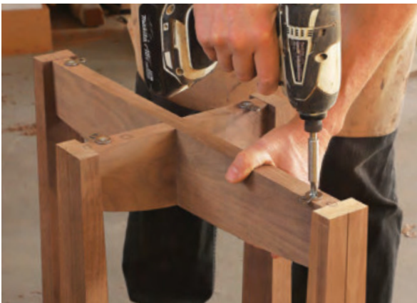
Figuring out the figure 8s. Wanting to recess the figure-8 fasteners into the underside of the top, Throop first screws them directly to the top of the rails.
