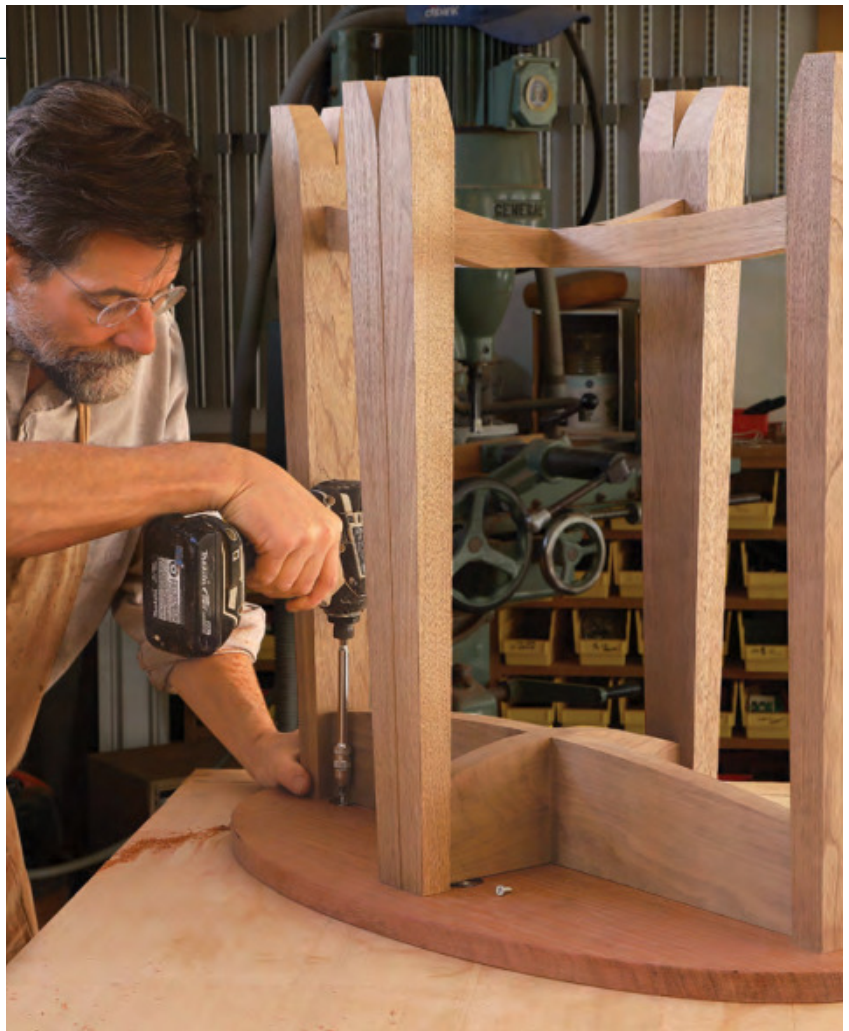
Neat mortises. When set in their mortises and screwed down, the figure 8s sit flush with the underside of the top.
