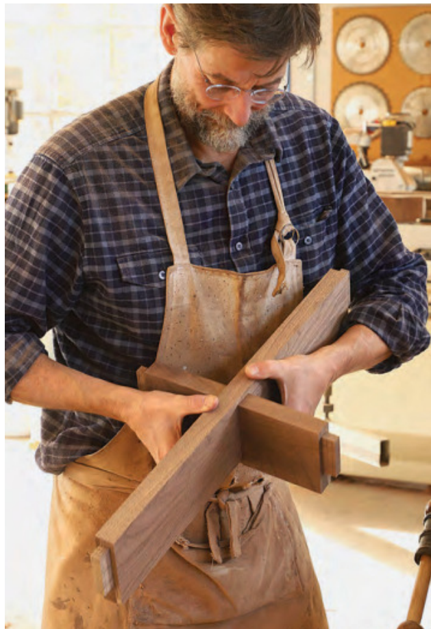
Well-fitted half laps. Having cut the second slot slightly tight, Throop uses a few strokes of a shoulder plane to achieve a perfect fit.
