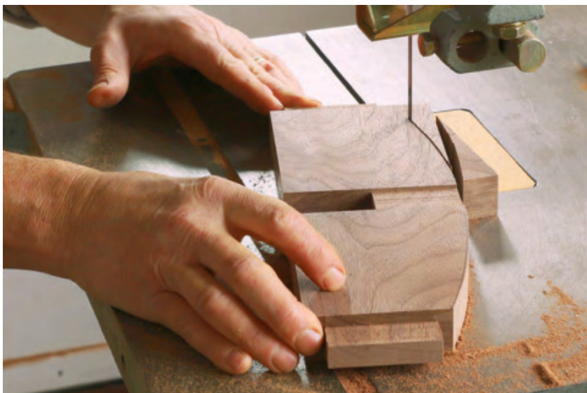
Taking care of the curves. Having cut and fitted the tenons and half-laps, Throop bandsaws the rails' curves and then smooths them at his edge sander.
