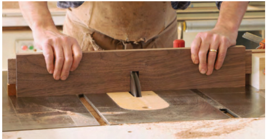
The mating slot. With the first rail's dadoes and slot cut, Throop can measure to find the correct width for the mating slot. He cuts it using the same centering technique.
