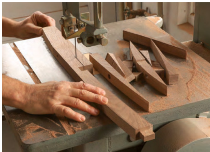
Curving the stretchers. Bandsaw work achieves the curves. Edge sanding smooths the convex curves, but Throop uses a compass plane to fair the concave ones.
