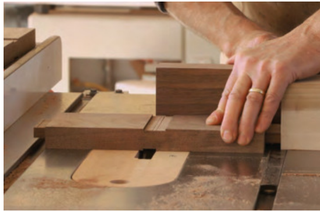
Centering device. The half laps begin with shallow dadoes for the shouldered portion of the joint. Throop cuts in two passes using a stop block on the miter gauge and turning the workpiece end for end between passes, ensuring the dado is perfectly centered.
