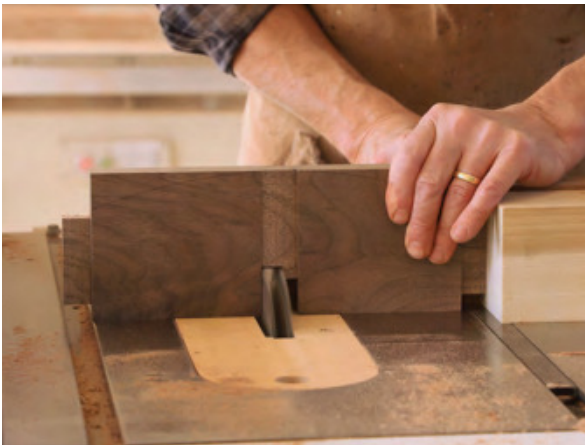
Slot-cutting. With the stop block in the same location, Throop turns the rail on edge and raises the dado blade incrementally to cut the half-lap slot.
