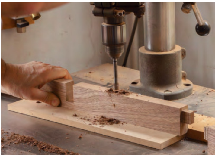
Boring for screws. After completing the stretchers' tenons and half laps, but before cutting their curves, Throop drills clearance holes and counterbores for the screws that will fasten the shelf.
