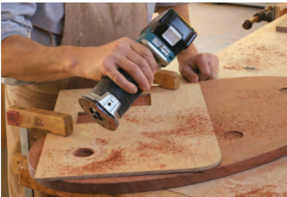
Inset ovals. After inverting the base on the top and marking the locations of the figure 8s, Throop uses a template to rout shallow oval mortises for each of them.
