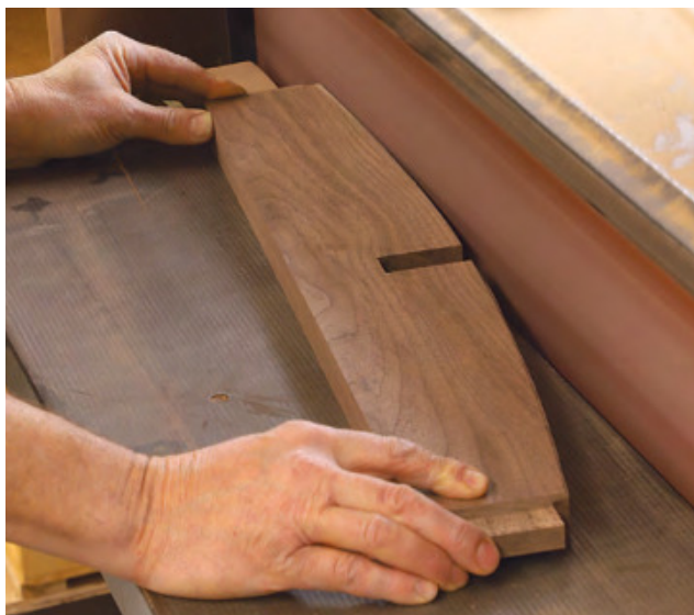
Taking care of the curves. Having cut and fitted the tenons and half-laps, Throop bandsaws the rails' curves and then smooths them at his edge sander.
