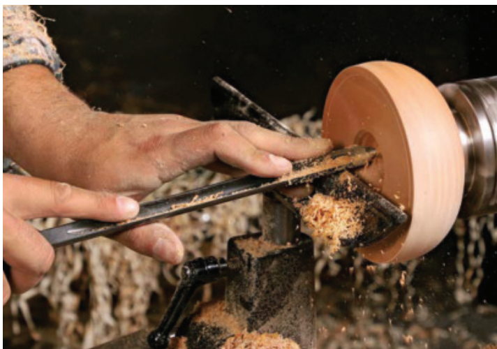
Open up the inside. With a \frac{1}{2} -in. deep-fluted gouge, make a series of progressively wider and deeper hollowing passes toward the center depth hole.
