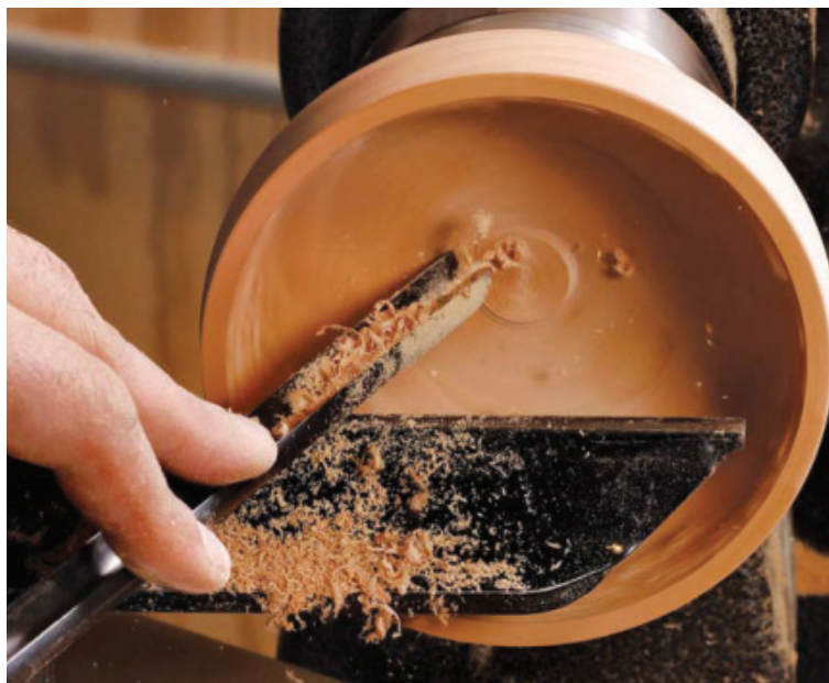
Finessing the flatter parts. A \frac{1}{2} -in. deep-fluted interior gouge, with its snub-nosed grind, lets Monaco finish the bottom of the interior. Before removing the base from the lathe, he applies oil and wax.
