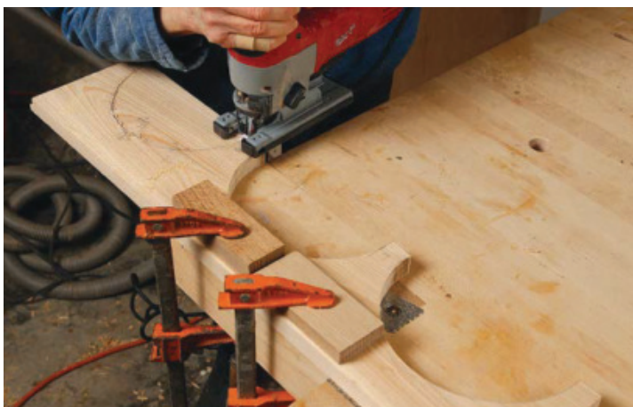
Shape the arches. As with the shape of the sides, rough out close to the line, and template rout the final shape of the arches on the frieze.
