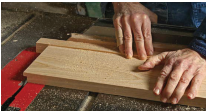
Stub tenon. Cut the stub tenon on each end of the frieze with multiple passes on the tablesaw.
