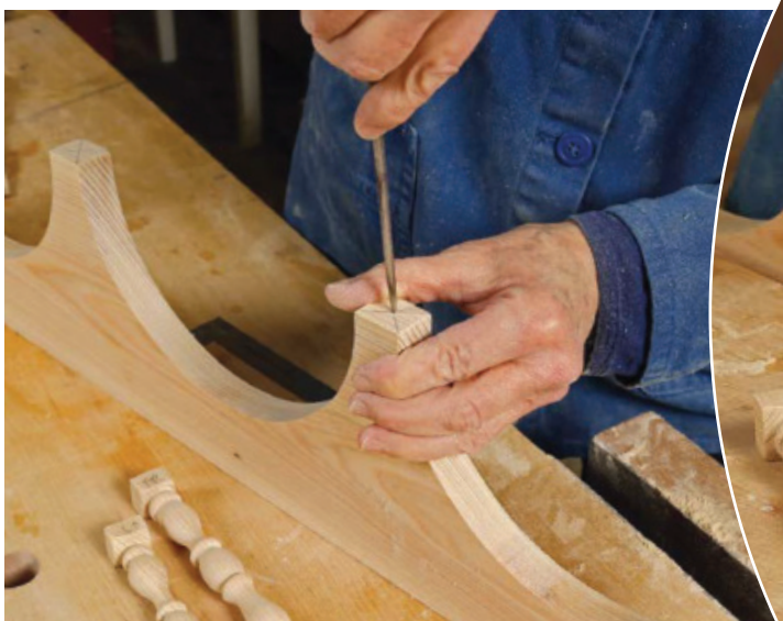
Drill dowel holes for the spindles. Mark the center point on the top of the spindles and on the squares at the bottom of the center arch. Then drill holes for the dowels that will join the spindles to the center arch. Spindles turned by Julie Jackson ( surclewood.com ).
