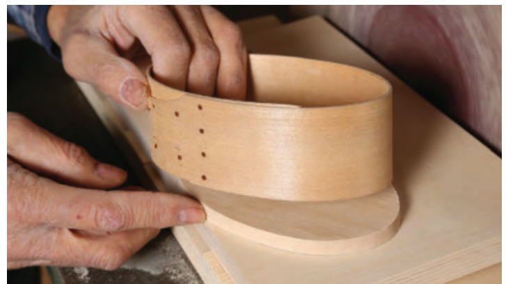
Bottoms up. Miller uses the bevel jig for the tops and bottoms of Shaker boxes. After scribing the inside shape of the box onto the bottom blank and sanding to the line, he fits the bottom into the oval box. The narrow side goes in first and allows the bottom to wedge into place, sealing it perfectly without putting too much pressure on the delicate box.
