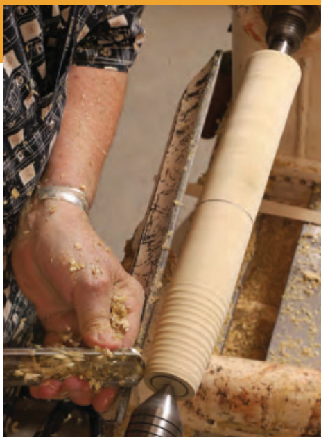
Start at the end. Using the same tool holding, posture, and body movement, begin cutting with shorter passes at the narrow end of the taper, and take progressively longer passes.
