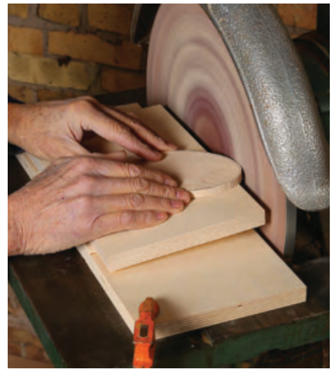
Bevel your curves. This jig allows you to present straight or curved edges to the sanding disc at an angle. Clamp the jig to the sander table, and work to your line.
