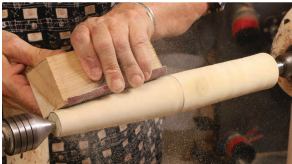
Sandpaper cleanup. A sanding block and some 120-grit paper quickly smooths out any tears in the tapered surface.
