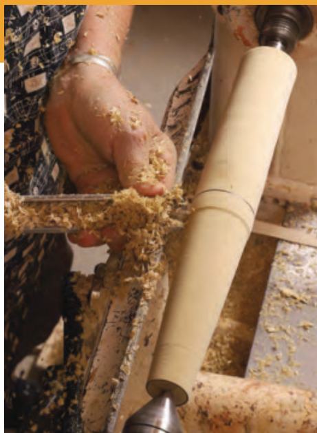
Long passes finish the taper. With the taper almost fully formed, Ireland begins a pass just shy of the workpiece's midpoint.
