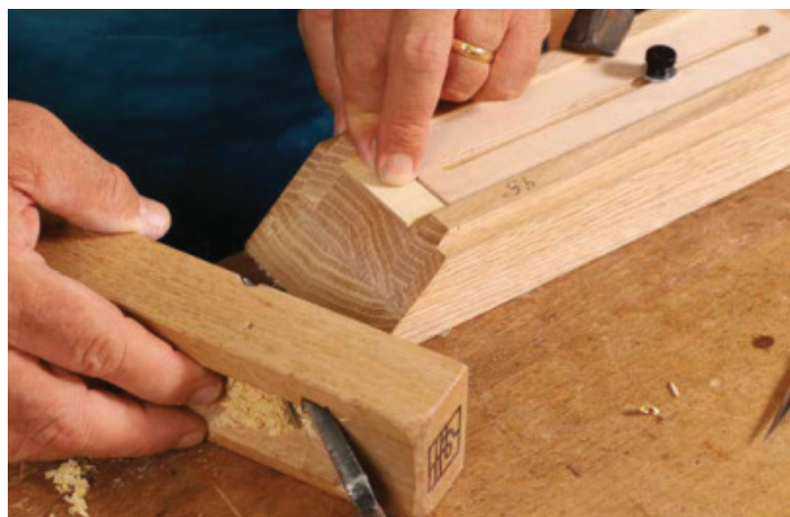
Miter number 2. A few strokes of the plane create a second miter, finishing all four pieces.
