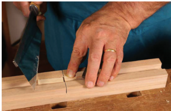
Saw to rough length. The strips are then stacked in a miter box, with their miters against a stop, and cut to rough length.
