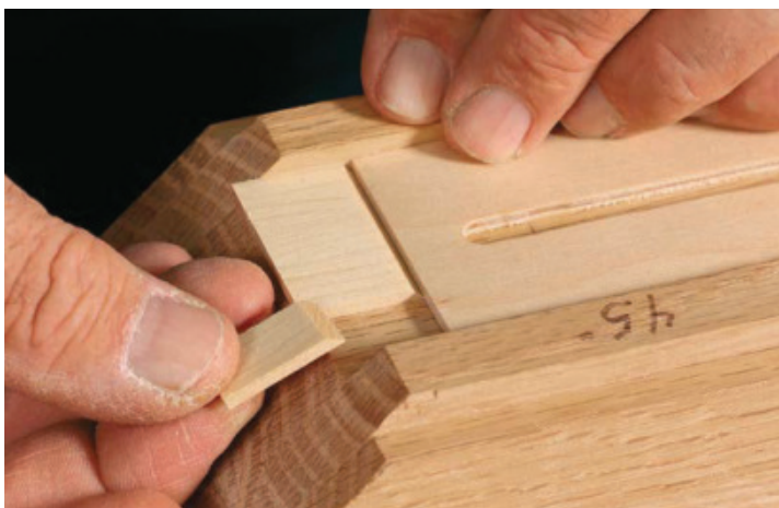
Back into the miter jig. After resetting the jig's stop, Stevens presses the mitered end of the strips against it.
