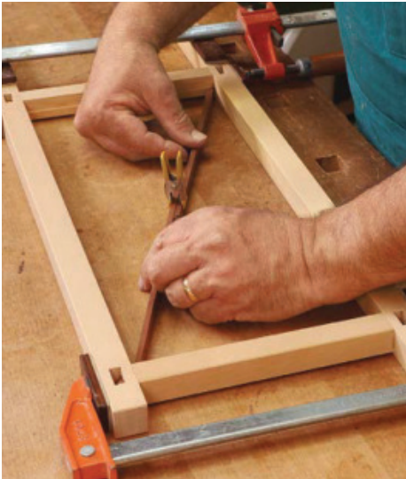
Front and back first. Stevens assembles the Andon in stages, starting with the front and back frames, which he glues up flat on his bench. Here he checks the diagonals of one frame with squaring sticks.
