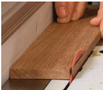
Bevel the edges. The top and bottom edges of the drawer sides are ripped at 4.75° off 90°.
