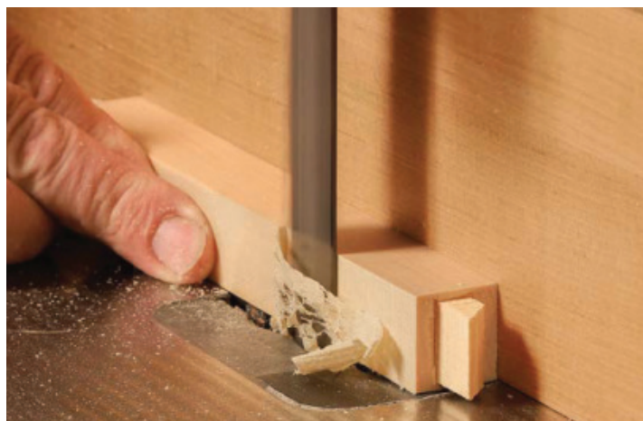
Rails get ripped. To simplify the joinery, the rails, like the legs, are milled \frac{7}{8} in. square. But after the tenons are cut, Stevens trims \frac{1}{16} in. off the outside face of the rails, so they'll be inset from the legs.
