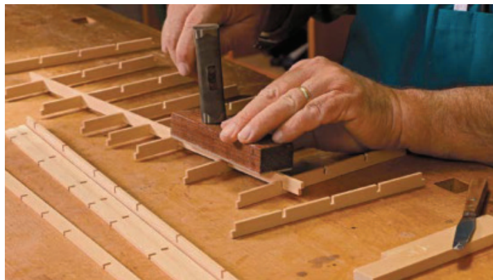
Gentle assembly. A hardwood block faced with mat board helps engage multiple half laps at once.
