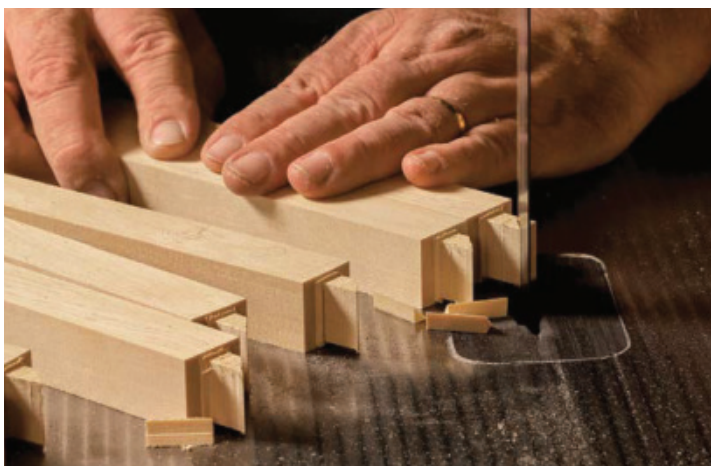
Freehand miters. Mark the miters on the tenon ends and cut them freehand on the bandsaw. The miters aren't a glue surface, and needn't be precise. Stevens holds a pair of rails as he saws for added stability.
