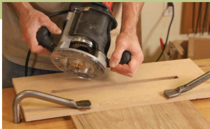
Sliding socket. With a router template aligned to the knife marks on the shelf, Gochnour cuts the through sliding dovetail housing for the stretcher. The template slot is 5/8 in. wide, and the bushing is 5/8 in. dia. The dovetail bit, ½ in dia. and 14°, is set to cut ¼ in. deep.
