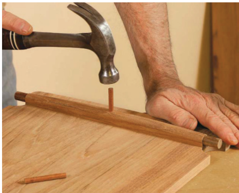
Just pin it. The stretcher's sliding dovetail gets no glue. It is just fixed at the center with a pin that's glued and tapped into place.
