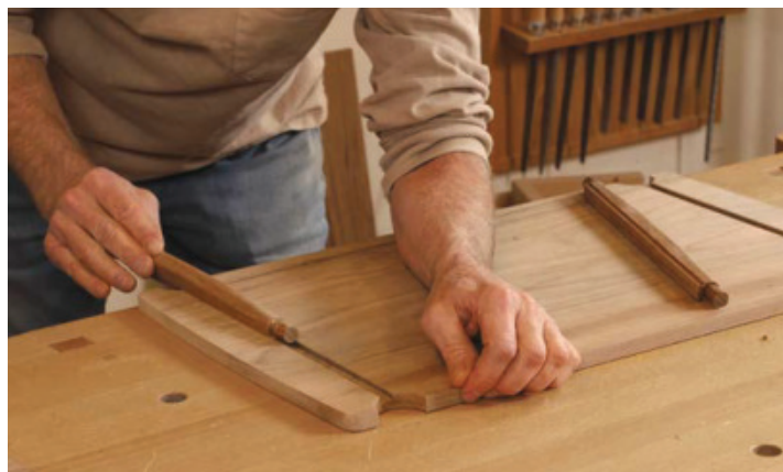
Shaped up and ready to slide. Once its dovetail has been cut and fitted, the stretcher is sawn to a crown along its underside and then shaped to a round profile with a spokeshave.
