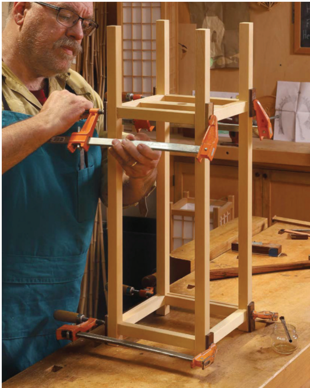
Front and back first. Stevens assembles the Andon in stages, starting with the front and back frames, which he glues up flat on his bench. Here he checks the diagonals of one frame with squaring sticks.
