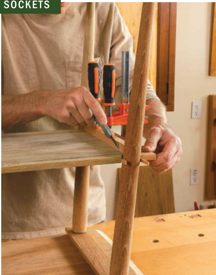
Dummy stretchers. To facilitate layout, Gochnour makes an extra pair of stretchers from scrapwood. They're identical to the real stretchers, but with no dovetail. He inserts them in the legs, clamps the shelf in place, and marks their location with a knife.
