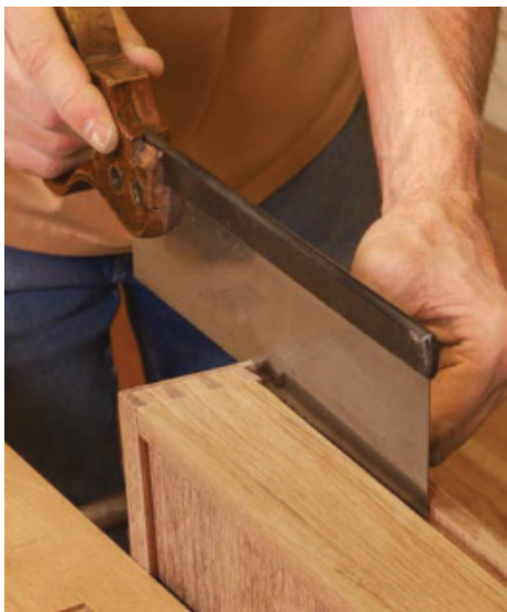
Handwork completes the runner groove. After assembling the drawer, Gochmour gingerly cuts a series of sawkerfs to open the back end of the runner groove. Then he'll square up the stopped end of the groove with a chisel.
