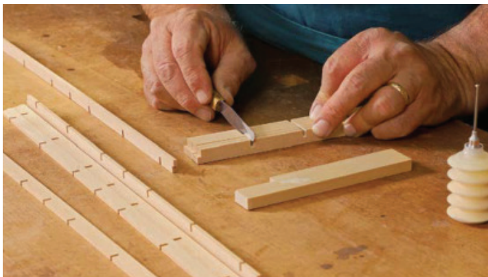
Gang up the strips for gluing. To prepare for assembly, Stevens aligns a batch of horizontal strips and applies glue to their half laps.
