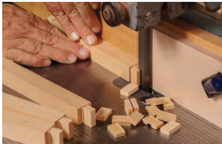
Bandsawn cheeks. With a stop block clamped to the bandsaw fence, cutting the rail cheeks goes quickly. After all the face cheeks are cut, move the fence and cut the edge cheeks.
