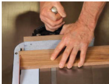
Angle the ends. On the drawer front and back, the ends are crosscut at 4.75° with a miter gauge at the tablesaw.
