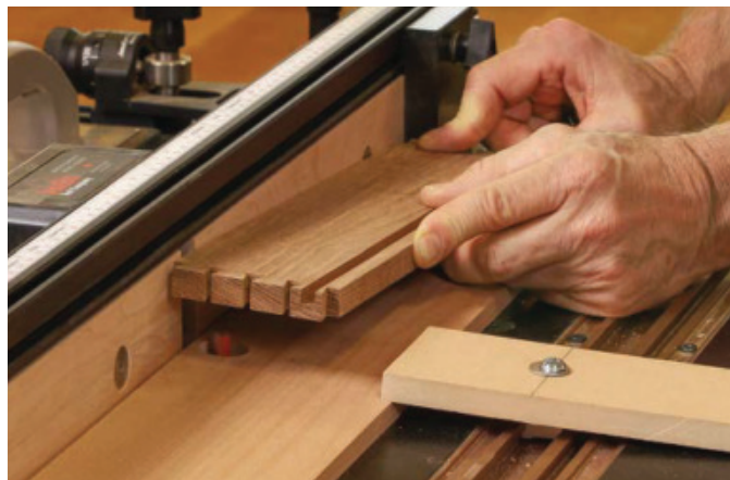
Sides get two grooves. After cutting angled through-grooves for the bottom at the tablesaw, Gochmour routs a stopped groove for the drawer runner. The workpiece rides on a tapered auxiliary table to give the groove a 4.75° angle.
