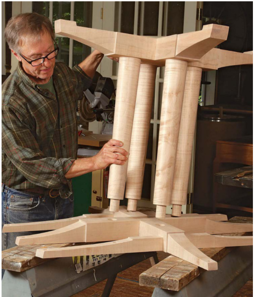
Bring the base together. Lamb assembles the two components upside down, letting him clearly see the mortises in the upper brace. Because the members are large, you may need a clamp on either side of the post to ensure even clamping.
