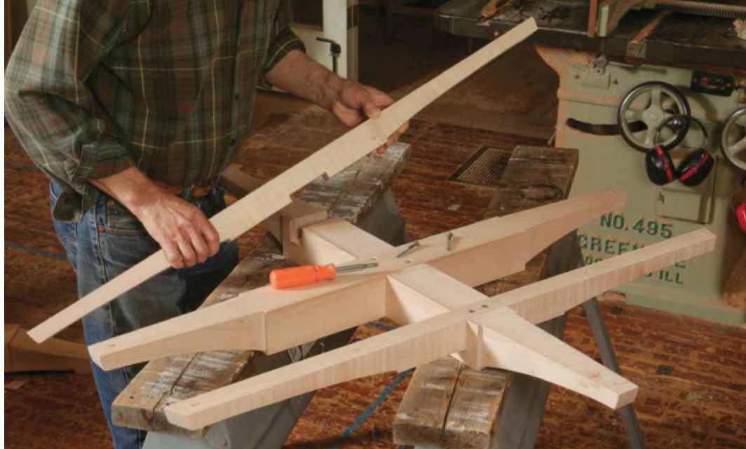
Add the minor braces to the upper lap assembly. These smaller braces help support the top and are half-lapped into place. Screw these in place as well.
