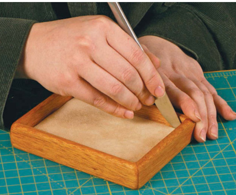
Refine the fit. As a final step, run an ordinary table knife around the lining to smooth the edges in place.
