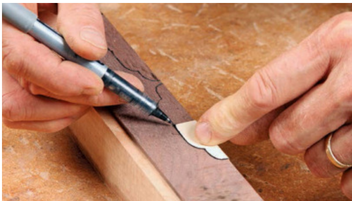
Draw the basic shape. Stowe uses a half-template cut from a manila folder so that the two halves of the pull are symmetrical.
