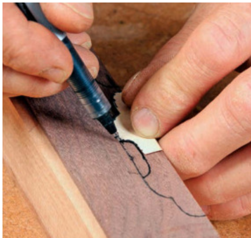
Draw the basic shape. Stowe uses a half-template cut from a manila folder so that the two halves of the pull are symmetrical.
