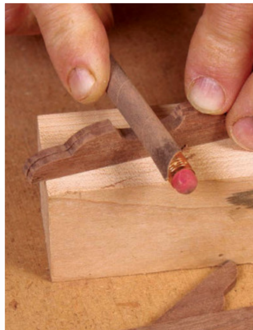
Refine the shape with sandpaper. Stowe groups the pulls to make it easier to keep the edges square to the faces. He uses 1-in.-wide sandpaper glued to a pencil to get into the tight curves.
