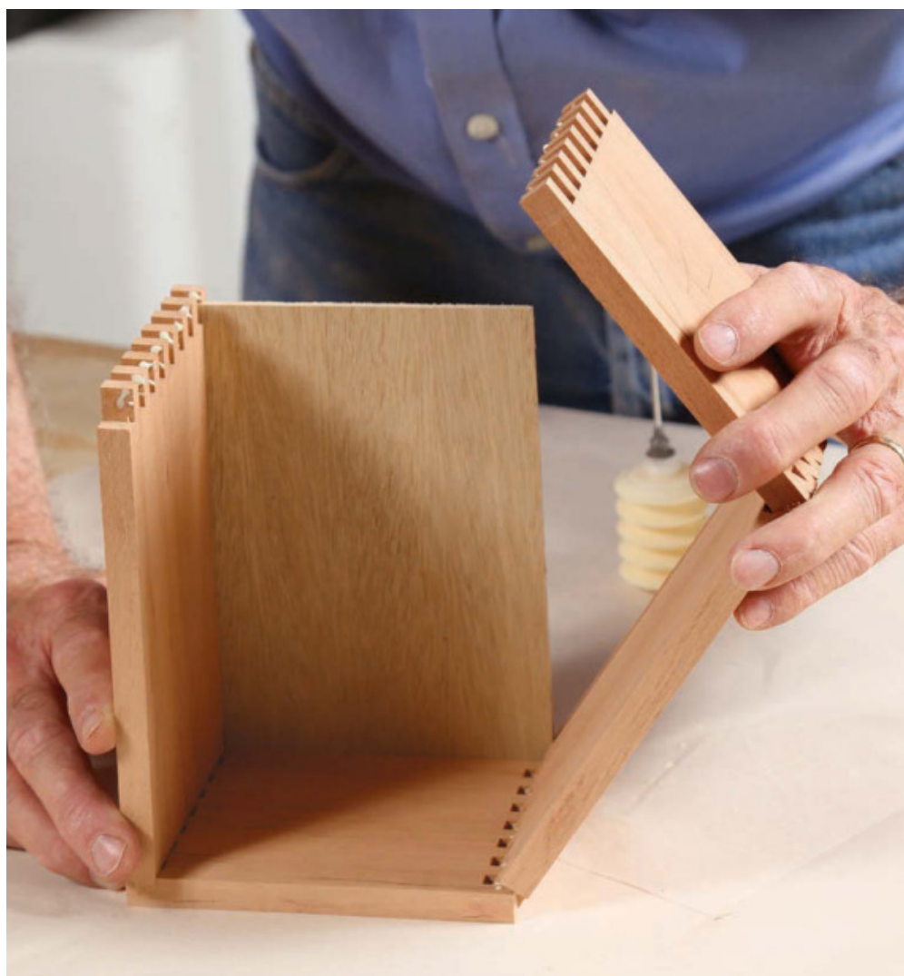
Wrap up. Assemble the sides around the bottom. If the parts are cut well, clamps may not be needed. Friction is often enough to hold the pieces. Check for square before letting the glue set.
