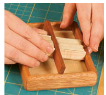
Fit and smooth. Fit the ring holder and divider into the box and smooth the fabric into place.
