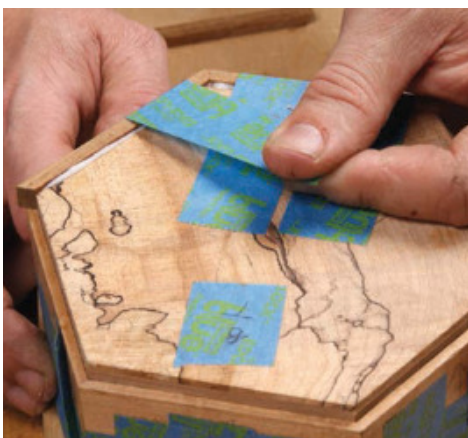
Saw and shoot. Saw the banding to length, and use the 60° bench-hook setup to trim the ends.
