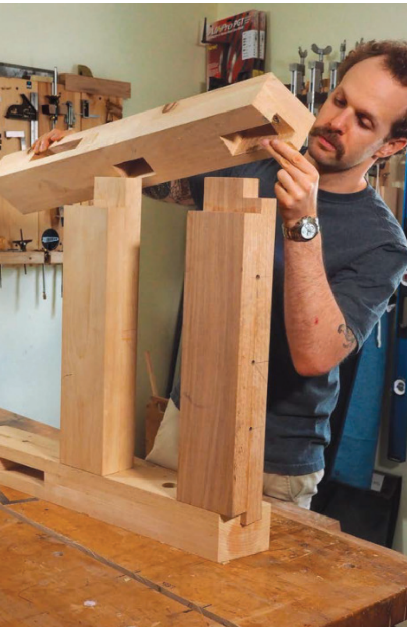
Dry-fit end assembly to mark the angle on the upper short stretcher. This waste is removed so the stretcher's upper edge lies flush with the legs. Bandsaw close to the line and, after gluing up the assembly, refine the cut with a long plane.
