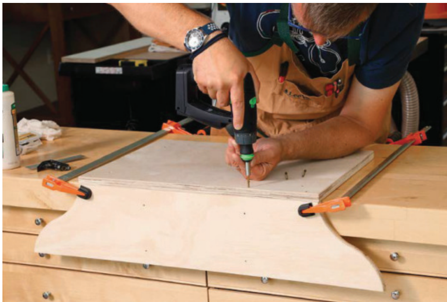
Glued and screwed. Guldenstern built the drill-press table from plywood and assembled it with glue and 2-in. star-drive trim-head screws.
