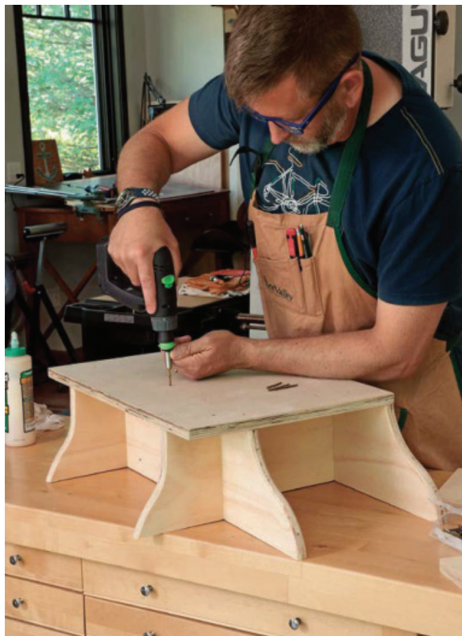
Put the bottom on the top. Once the dust box sides and the front fins are screwed in place, Guldenstern screws through the bottom to firm up the fixture.
