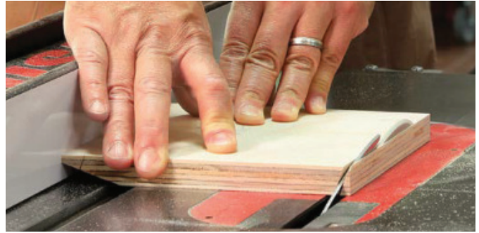
Angled walls funnel the airflow. Using \frac{1}{2} -in. plywood, Guldenstern makes a pair of angled inner walls for the dust box. He miters the top edge at the tablesaw with the workpiece held vertically and clamped to a longer, thicker board for stability. He cuts the bottom edge with the workpiece flat to produce the complementary angle.
