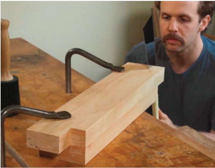
Cut the short stretcher's tenons to width. These stretchers are also laminations. The shorter front board forms the tenons' shoulders, and the longer rear board forms the cheeks.
