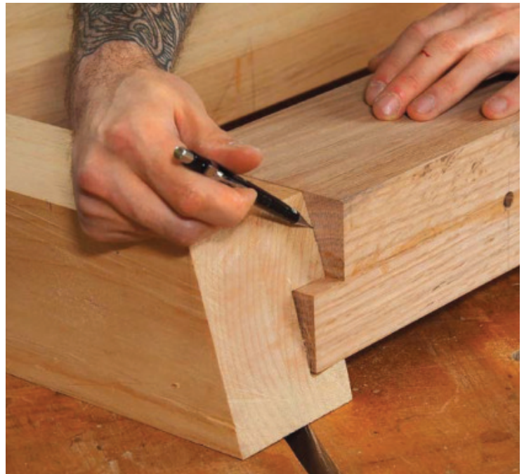
Dry-fit end assembly to mark the angle on the upper short stretcher. This waste is removed so the stretcher's upper edge lies flush with the legs. Bandsaw close to the line and, after gluing up the assembly, refine the cut with a long plane.
