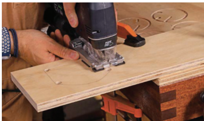
Dust opening. Before cutting the sides of the dust box to length, he creates a window in one of them where the dust-collection port will be attached.
