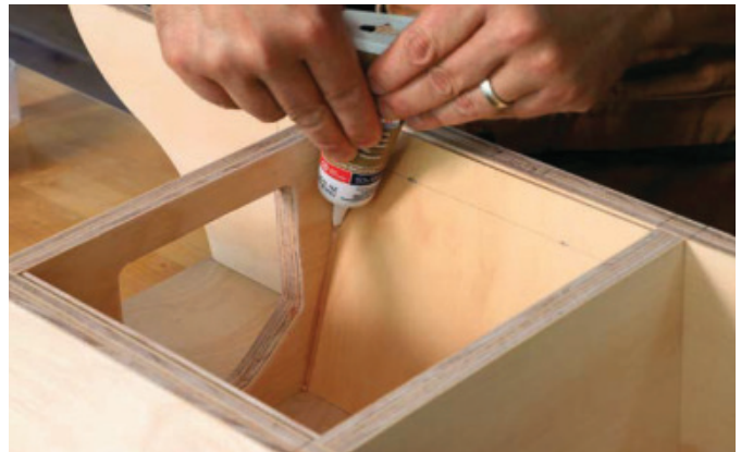
Tack on the inner walls. Glue and staples hold the angled inner walls in place. Caulking the corners minimizes air leakage.
