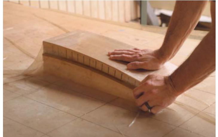
Gaining an atmospheric advantage. Morley puts the wrapped package—core and bending form—into his vacuum bag to apply final, even clamping pressure.
