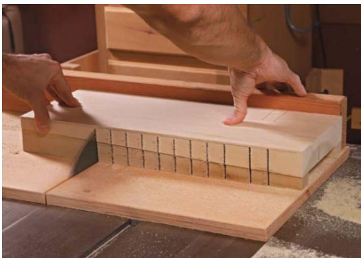
Cut kerfs in the core. With the inside face of the core facedown and the blade raised to within \frac{1}{8} in. of the outside face, Morley uses a dedicated sled to cut the slots that will allow the core to bend (above). After cutting all the kerfs, remove what remains of the wedges (right) and scrape off any residue from the tape.
