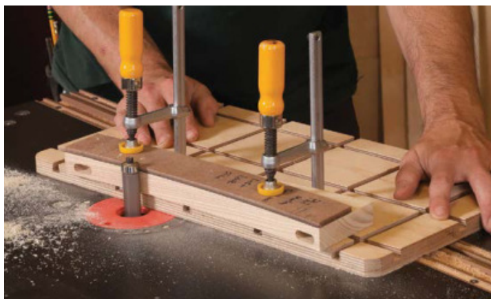
Template-route the stile. After routing mortises for slip tenons and then bandsawing the door stile's curved inner edge, Morley template-routes the curve to finished shape.
