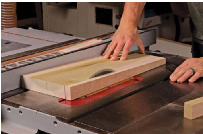
Rip a pair of wedges. To simplify the kerfing process, make your core blank overwide and, after tapering it, rip a wedge-shaped strip off each edge.
