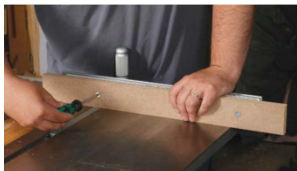
Sacrificial fences don't sacrifice function. The fence can accommodate a user-made sacrificial fence that is secured using T-nuts and screws.
