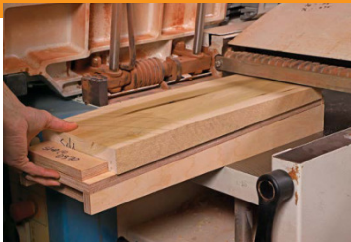
First taper the core. Morley runs his poplar core stock through the planer on a ramped jig. The blank is overwide both in length and width.
