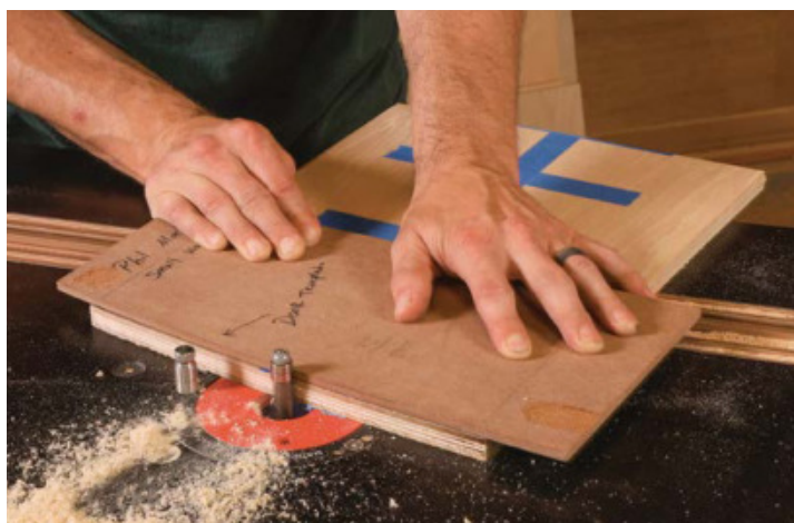
Curve the panel. The door panel, a 1/4-in. Baltic-birch plywood substrate veneered with ash on both faces, gets trimmed to final shape with the large template. The template is adhered to the panel with double-sided tape.
