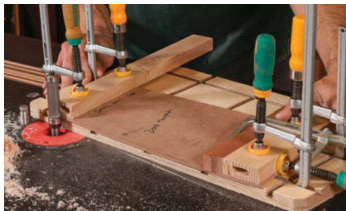
Rails get a trim, too. After cutting the mortises in the rails, Morley routes the ends to a curve, following the wide template. The rails are attached to the template with double-sided tape and firmly clamped to the sled.
