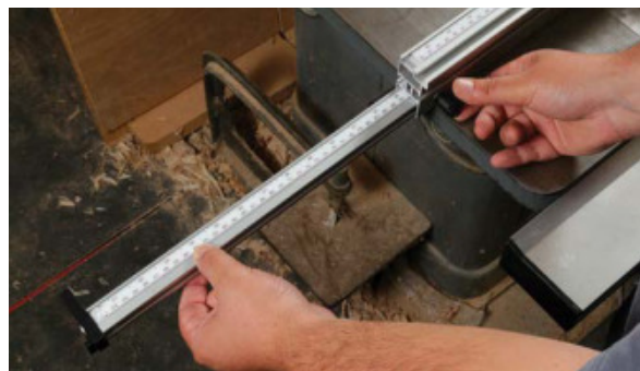
The stretch arm's strong. The fence's main section is 20 in., but its telescoping arm extends it to 36 in. The stops work equally well with the main and telescoping sections.
