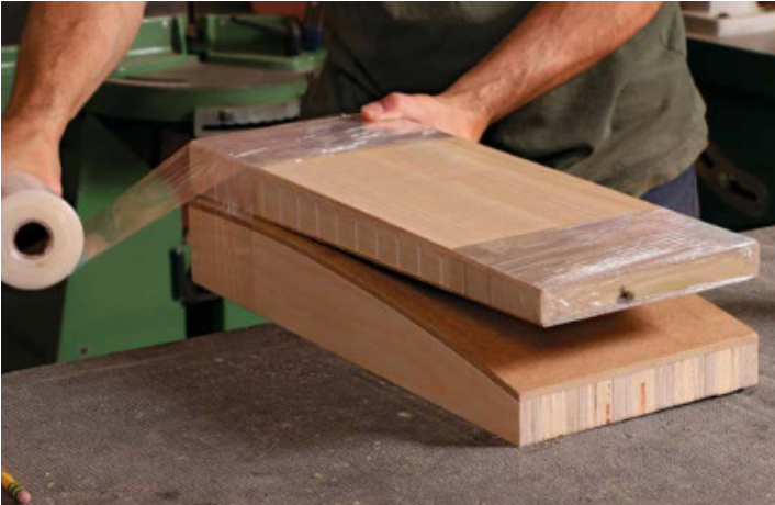
Clear clamps. Bind the veneer tightly to the core with stretch wrap, and then wrap the whole thing to the bending form.
