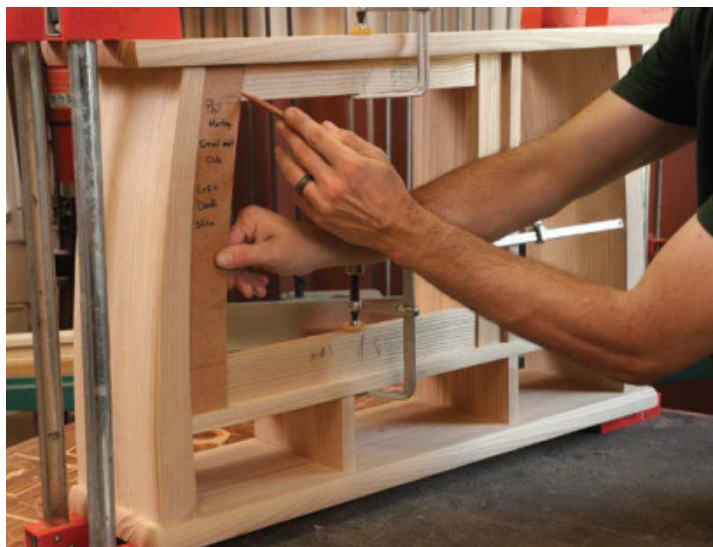
Marking the rails. Using the narrow template, Morley lays out the curved crosscuts on the left end of the rails.
