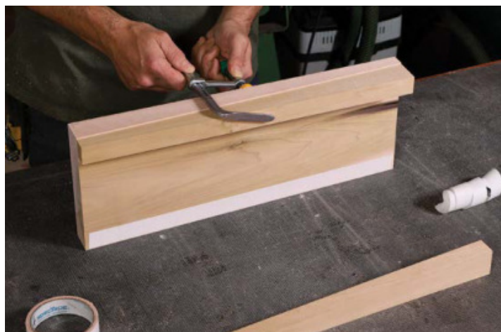
Reverse the wedges and tape them to the blank. Using double-sided tape, attach the tapered strips to the tapered core with their thick end at the core's thin end. Apply clamp pressure briefly along the strip to be sure the tape's grip is firm.
