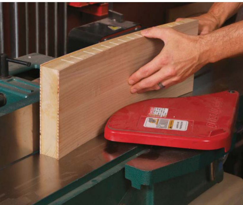
Clean the curved edges. Once the kerfed bend is cured, joint one edge (left). With the convex side down and the jointed edge against the tablesaw fence, rip the side to width (above).
