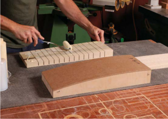
Veneering the core. Morley glues shopsawn ash veneer to both the inside and outside faces of the poplar core. He sliced the veneers from a riftsawn ash board and milled them to \frac{3}{32} in. To get the full width of the side, he edge-glued two veneers.
