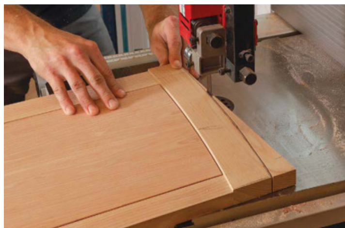
The door's last curve. Having parallel edges is a clamping advantage, so Morley waits until after the door is glued up to bandsaw out the door stile's outer curve. He'll dial in its fit to the cabinet side with a stationary belt sander and hand tools.
