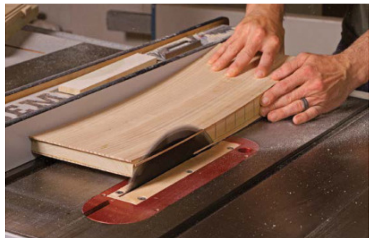
Clean the curved edges. Once the kerfed bend is cured, joint one edge (left). With the convex side down and the jointed edge against the tablesaw fence, rip the side to width (above).
