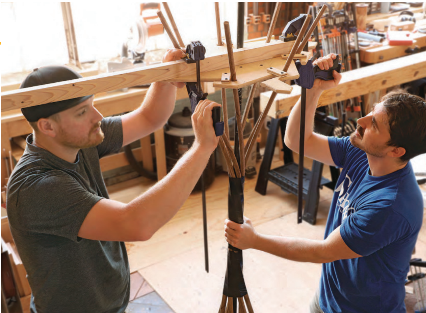
A brake for the upper plate. To keep the helical bend from untwisting, Shaw and Dinneen clamp one end of a long stick across the upper plate and brace its other end against a bracket on the wall.
