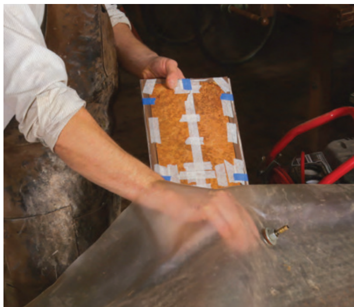
Leave it in the vacuum bag overnight. Michelinie uses a vacuum bag to glue up the panel. He uses blue tape to hold the veneer to the substrate, preventing either from sliding around.
