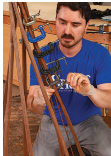
A covert cord. The lamp cord travels down the groove cut in one leg. Shaw here epoxies a spline into the groove to hide the cord.
