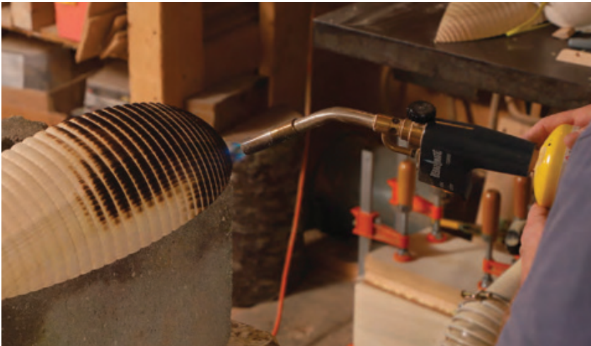
Scorch the surface. Gardner uses a plumber's torch to burn the beaded surface of the shelf. Then he scrubs with a soft wire brush to remove the ash.
