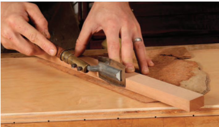
Saw out the burl pieces with a veneer saw and a jointed batten. With four sequentially cut sheets stacked together, saw just outside of your lines. The batten both guides the saw and helps stabilize the veneer.
