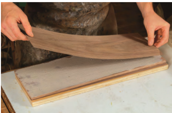
Substrate needs a backer. Because Michelinie wants to even the stresses on both faces of the substrate, he veneers it front and back. The backer veneer is simply a sheet of walnut (left). Be careful to align your front veneer with the edges of the substrate so the book-match remains centered and straight (above).
