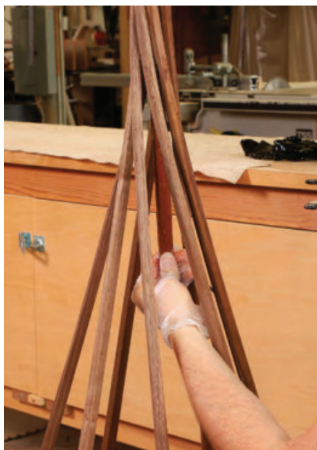
Inserting the center stick. After giving the legs a week to dry, Shaw removes the metal pipe and replaces it with a wooden dowel made from leg scrap. He drills out the dowel, threads the cord through it, and glues it in place with epoxy.
