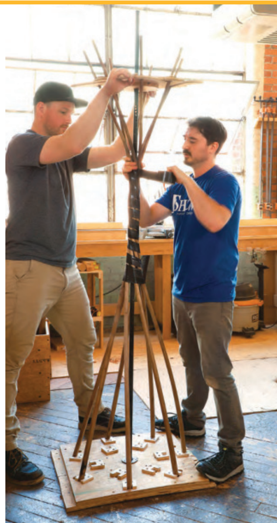
Wrap the twist to keep it tight. With the upper plate rotated as far as he wants it, Shaw wraps the central portion of the twist with packing tape to keep it tight as it dries.
