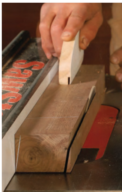
Adding another angle. The legs are canted as well as splayed, and to create that outward angle, Rodríguez rips the top and bottom edges of the rail with the tablesaw blade tilted to 10°.
