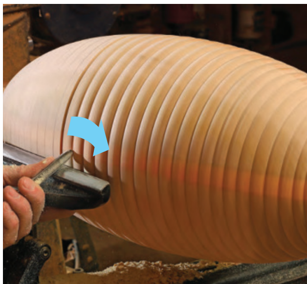
Each bead starts with two grooves. To turn a bead, first make V-cuts centered on the lines on each side of the bead. Gardner uses a ⅜-in. spindle gouge for the larger beads, and a ¼-in. gouge for the smallest ones.
