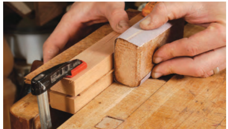
Joint two mating edges with a sanding block. Do this with all four pieces of veneer clamped near their edges and between cauls. Check your work with a straightedge to ensure you have a good glue surface.
