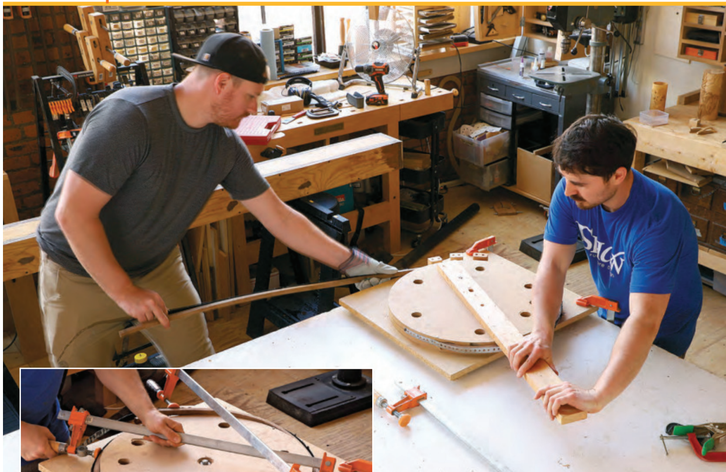
Circular steam-bend. Using a lazy-Susan-like jig, Shaw and Dinneen bend a 6-ft.-long stick into a circle with overlapping ends. A metal bending strap supports the stock as it bends to minimize breakage.
