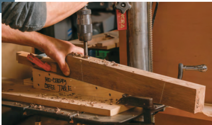
Rail blank on the ramp. To give the legs their outward splay, the mortises for them are drilled at 10° using a shopmade ramp jig on the drill-press table.
