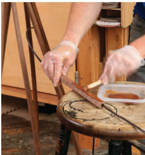
Inserting the center stick. After giving the legs a week to dry, Shaw removes the metal pipe and replaces it with a wooden dowel made from leg scrap. He drills out the dowel, threads the cord through it, and glues it in place with epoxy.
