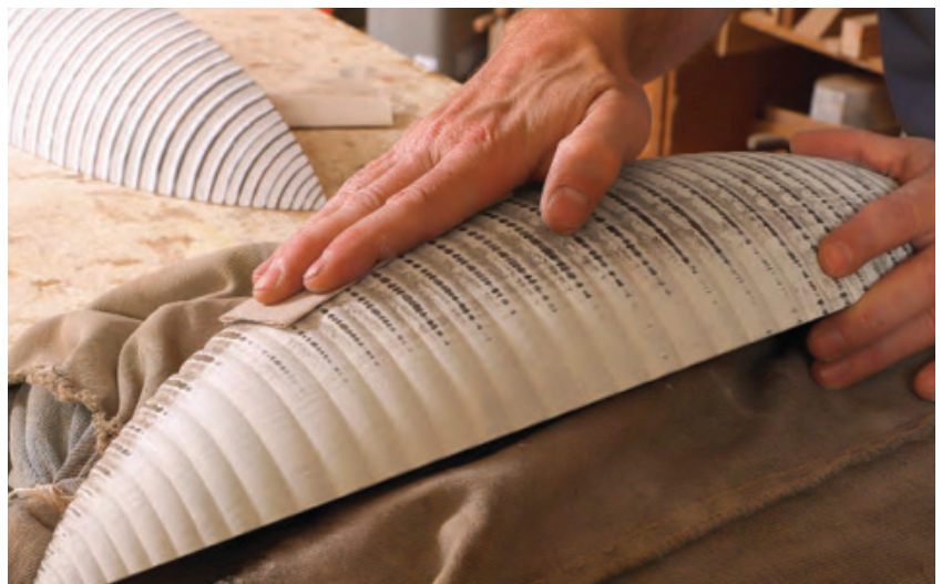
Paint and paper. After cleaning with compressed air, apply three coats of milk paint. When it dries, sand the paint, taking lengthwise strokes and abrading through the paint in the high spots to expose the charring.
