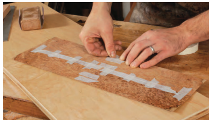
Arrange the panel using veneer tape. To hold the veneer in place during the glue-up later, tape the parts in place. First tape across and along the right and left halves, pulling the tape taut as you go (left). After that, joint their ends using cauls and a sanding block. Finish the panel by joining the two matching ends (above).
