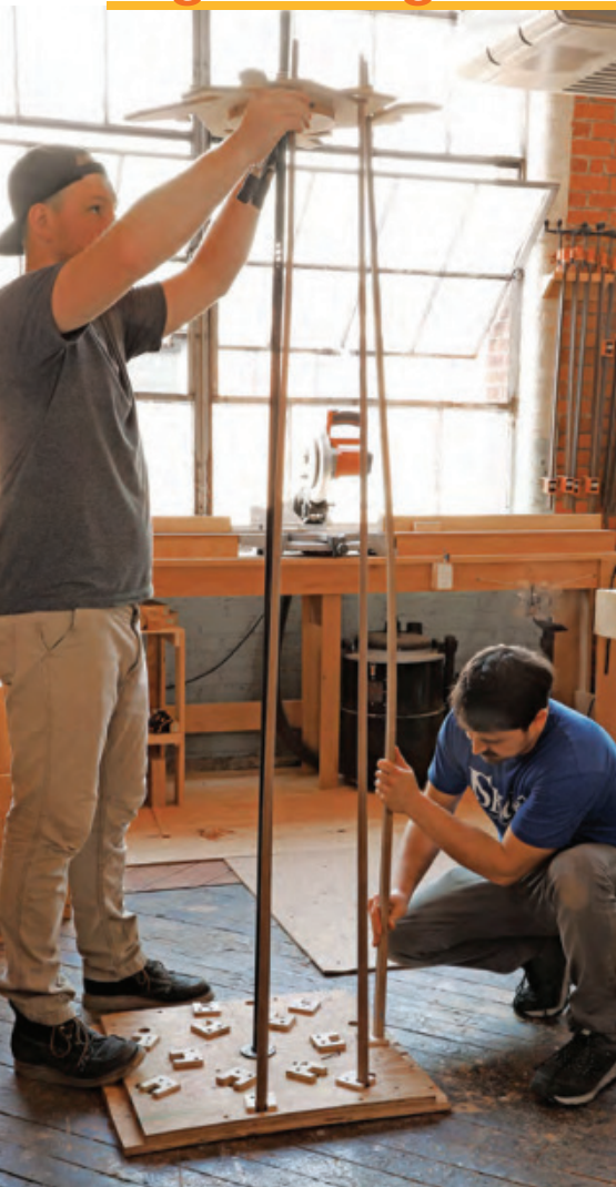
Seven legs, set at speed. Shaw and his assistant, Matthew Dinneen, bring the legs out of the steambox in quick succession. They socket a leg's bottom end into the jig's lower plate and slot its top end into the upper plate.
