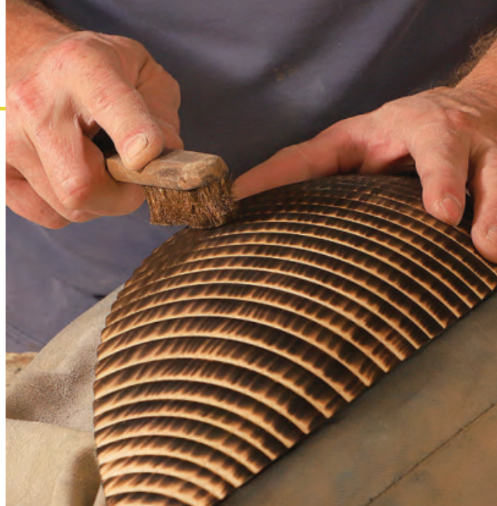
Scorch the surface. Gardner uses a plumber's torch to burn the beaded surface of the shelf. Then he scrubs with a soft wire brush to remove the ash.
