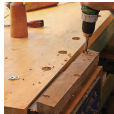
Drill the rail for hardware. The rail will be attached with figure-8 fasteners, which permit the top to move with the seasons. Rodríguez mortises for them by cutting a circle with a Forstner bit in a hand drill and then making a flared opening to the mortise with a chisel.
