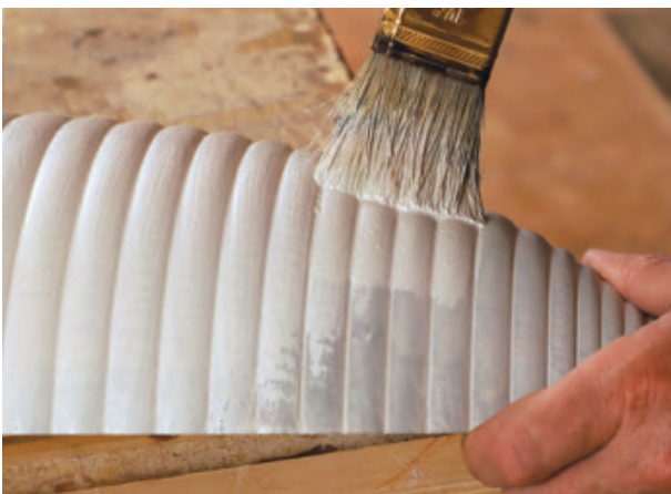
Paint and paper. After cleaning with compressed air, apply three coats of milk paint. When it dries, sand the paint, taking lengthwise strokes and abrading through the paint in the high spots to expose the charring.
