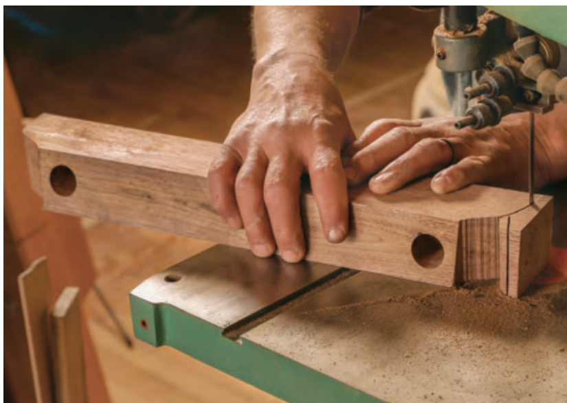
Drill the rail for hardware. The rail will be attached with figure-8 fasteners, which permit the top to move with the seasons. Rodríguez mortises for them by cutting a circle with a Forstner bit in a hand drill and then making a flared opening to the mortise with a chisel.
