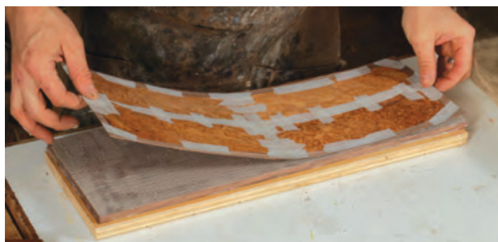
Substrate needs a backer. Because Michelinie wants to even the stresses on both faces of the substrate, he veneers it front and back. The backer veneer is simply a sheet of walnut (left). Be careful to align your front veneer with the edges of the substrate so the book-match remains centered and straight (above).
