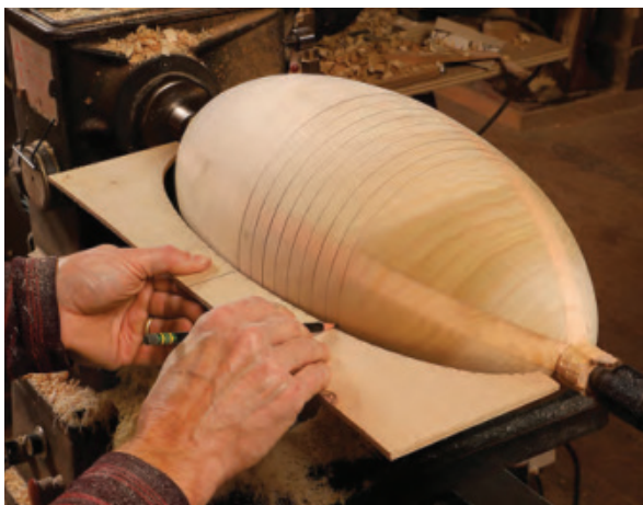
Graduated layout. Following marks on a plywood template, Gardner lays out the bead spacing. The beads graduate in size from the largest at the center to the smallest at the ends.
