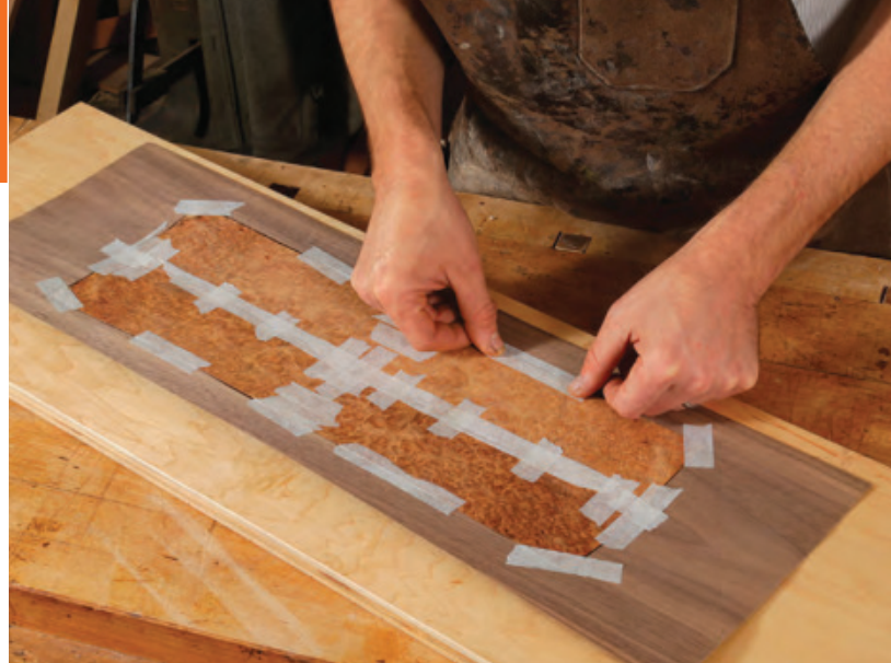
Glue up the burl and window. The joint between the walnut and the burl doesn't need to be neat since the inlaid cross-banding will fill that space. After taping in the burl, cut the walnut to the size of the substrate.
