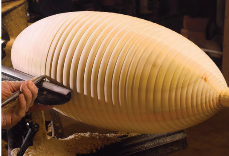
Each bead starts with two grooves. To turn a bead, first make V-cuts centered on the lines on each side of the bead. Gardner uses a ⅜-in. spindle gouge for the larger beads, and a ¼-in. gouge for the smallest ones.
