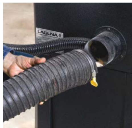
Super dust collection. The port is 4 in. with a 1½-in. T off the side for the blade-guard collection hose. Dust collection is very effective with the blade guard in place, but even without it, dust collection is still good.
