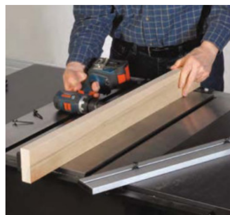
Adaptable rip fence. The rip fence is a single aluminum face on a stout steel frame. The aluminum face can be removed easily for attaching a sacrificial face or custom jigs, a nice touch.
