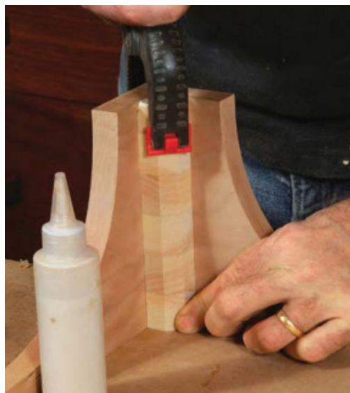
Posts with cross-grain layers strengthen the base's dovetailed corners. These reinforce the feet and act as support posts at each corner of the dresser. McLaughlin crisscrosses each layer's grain to balance strength and stability.
