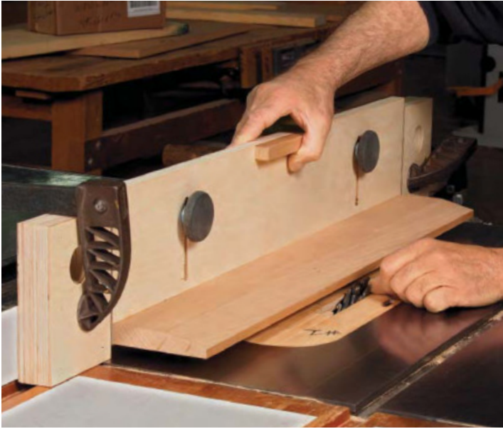
Adjust the height. The tab and threaded knobs make it easy to hold, lift, lower, and lock in the height of the fence.
