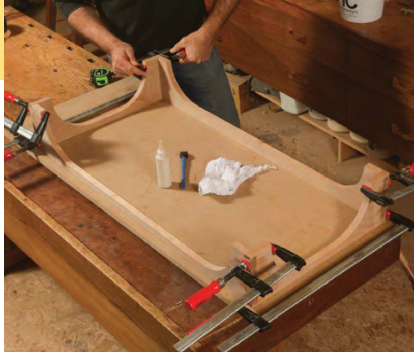
Glue up the base. The tails are wide enough that McLaughlin can apply pressure directly to them rather than using cauls.
