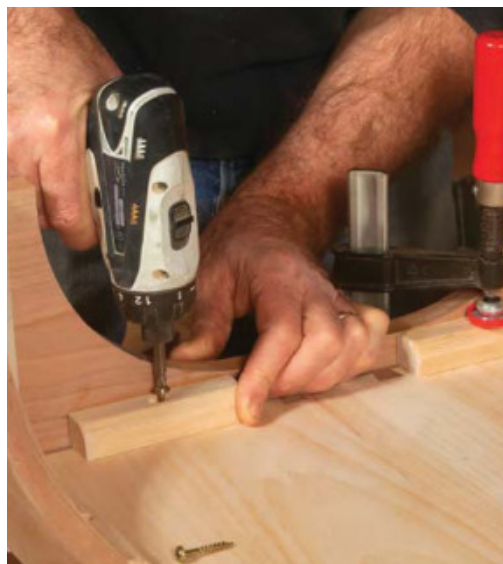
Glue the front attachment blocks to the case; screw on the back ones. These blocks secure the base to the case. Gluing the front ones to the case and using slotted screws on the back ones directs wood movement to the back, keeping the reveal on the front even year-round.
