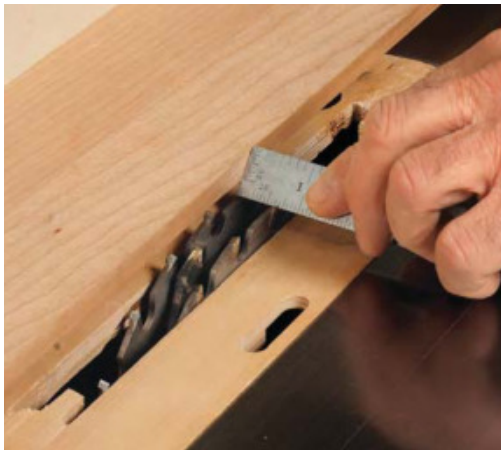
Adjust the height. The tab and threaded knobs make it easy to hold, lift, lower, and lock in the height of the fence.
