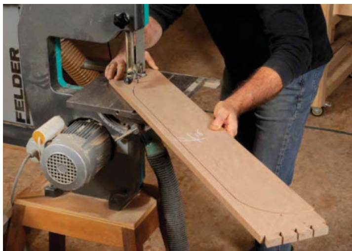
Bandsaw the arch after cutting the dovetails. McLaughlin bandsaws close to the line before refining the cut with a sanding drum and a scraper.
