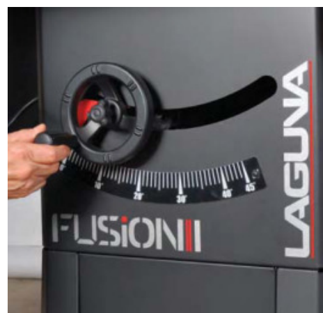
Smooth settings. Blade elevation and angle adjustments are smooth and easy, with little effort required to tilt the blade to its 45° max.
