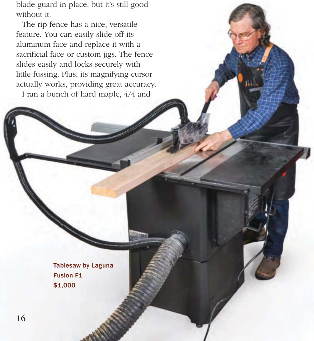
Adaptable rip fence. The rip fence is a single aluminum face on a stout steel frame. The aluminum face can be removed easily for attaching a sacrificial face or custom jigs, a nice touch.
