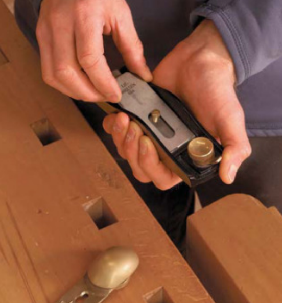
Swap out the iron. Korsak likes a freshly sharpened high-angle iron for end grain.
