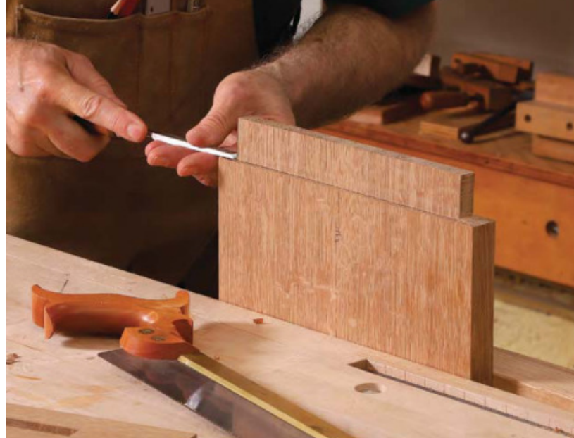
Trim the long tenon to width. With the shelf tenon still full length, establish the end shoulders with handsaw cuts followed by chisel work.
