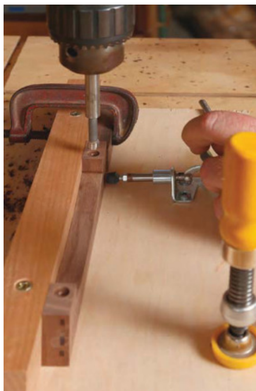
End run around end grain. Because screws into end grain can weaken over time, add threaded inserts to the legs. Bore holes for them on the drill press. Use a fence, a stop block, and a toggle clamp to keep the piece firmly against the fence. But don't glue the inserts in place yet.
