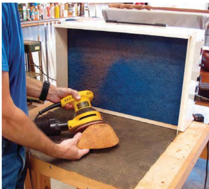
Dust collection at the source. When placed 20 in. from the source, as Oneida recommends, the machine does a great job protecting your work, your shop, and your lungs from fine dust.
