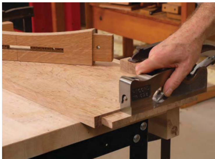
Fit the tenon and mark through the mortise. After cutting the through-mortise and the long groove in the lower rail, Hartman fits the thickness of the shelf tenon with a shoulder plane (left). With the shelf tenon dry-fitted partway into the lower rail, mark the width of the through-tenon using the center mortise as a guide (above).
