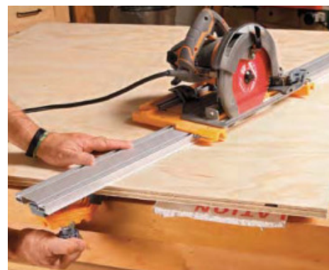
Angled cuts too. Two auxiliary clamps lock the track at angles other than 90°, expanding the capability of this excellent system.
