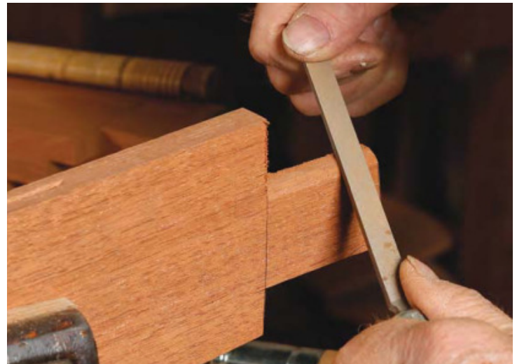
Cut the tenons. Hare cuts the tenons on the bandsaw, but they can easily be cut by hand. Once they're cut, use a rasp and file to round them.
