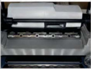
EASY ACCESS TO CUTTERHEAD TO CHANGE INSERT BLADES
