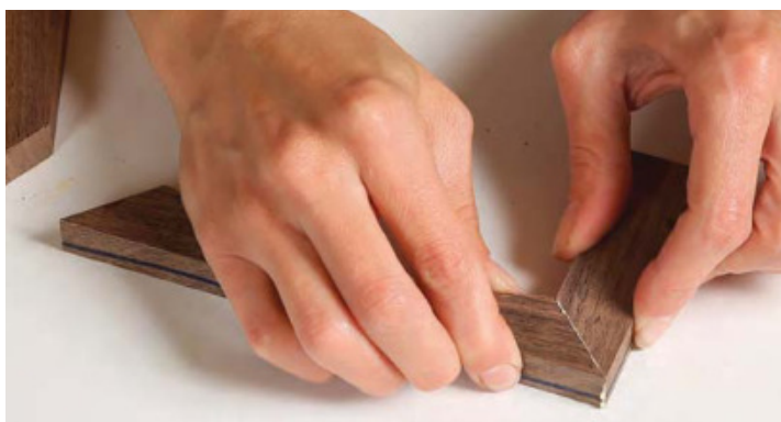
Rub joint gets the job done. Use a dab of glue and rub the joints back and forth against each other until the glue grabs. Hold the joint firmly in place for about 30 seconds and leave the pulls to dry overnight.
