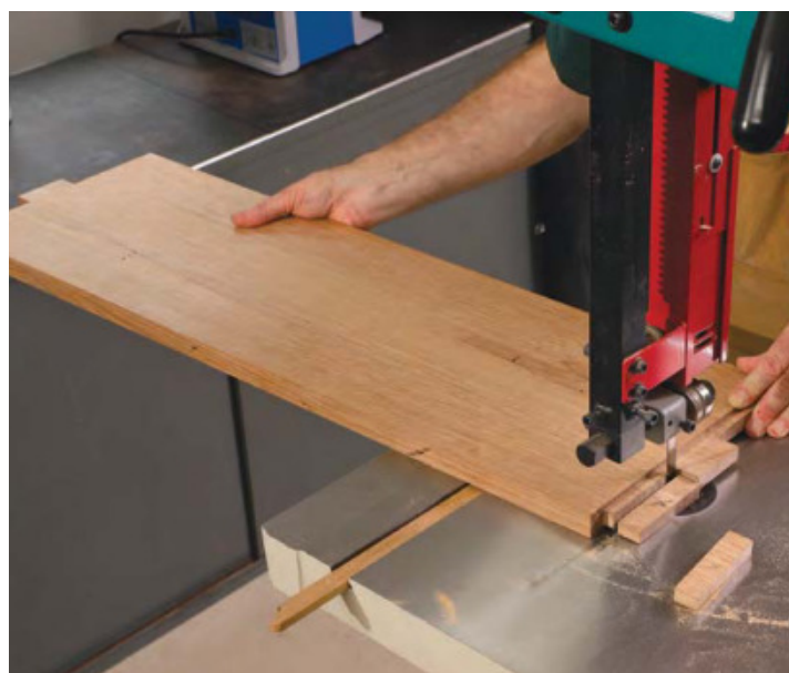
Cut back the tenons. After making careful handsawn kerfs to define the width of the through-tenon, bandsaw the stub tenons to length.
