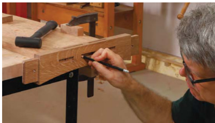
Fit the tenon and mark through the mortise. After cutting the through-mortise and the long groove in the lower rail, Hartman fits the thickness of the shelf tenon with a shoulder plane (left). With the shelf tenon dry-fitted partway into the lower rail, mark the width of the through-tenon using the center mortise as a guide (above).
