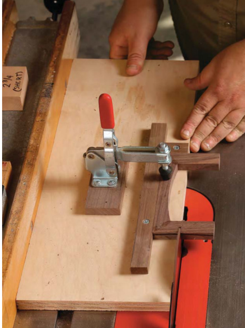
Cut the legs to length. After glue-up, use another simple jig to hold the pull in place while cutting the legs to length on the tablesaw.
