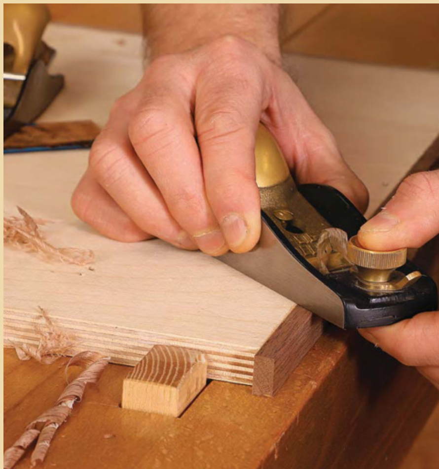
Flushing in two steps. Korsak uses two block planes to flush solid edging to a veneered panel. Here he takes a series of coarse shavings with the first block plane, stopping when the edging is about \frac{1}{64} in. proud of the panel.
