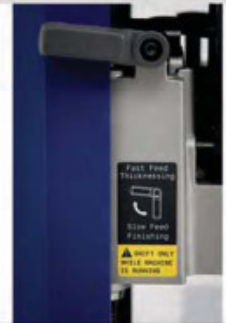
TWO-SPEED FEED RATE SWITCH LOCATED ON FRONT
