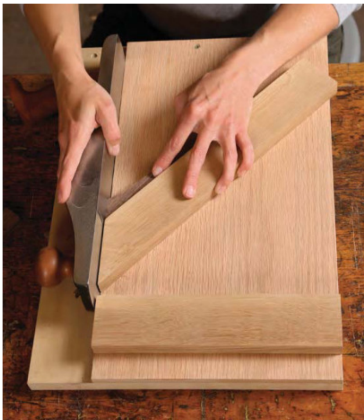
Fine-tune the joint. Prior to glue-up, Huff uses a handplane on a shooting board to clean up the miters.
