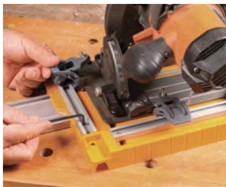
Alignment is easy. Once locked in position to suit your saw, the three toggle clamps let you attach the plate in seconds, returning the saw to the same position each time.
