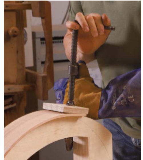
Bending form with a built-in clamp. With a slot at the lower end that pinches the workpiece in place, this form makes for an easy bend without a metal strap. Boggs clamps the upper end of the part to the form to let it set.
