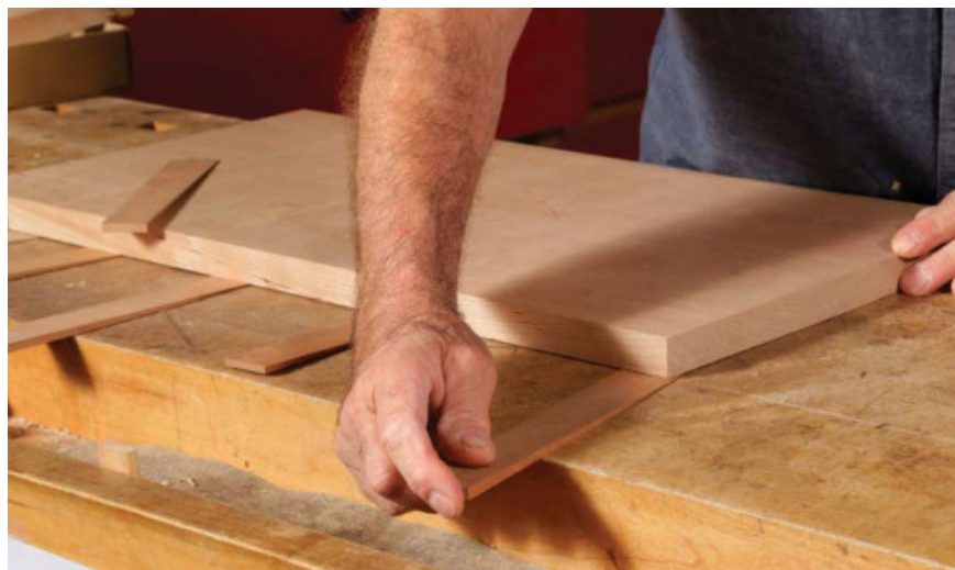
Cup up, wedges down. Van Dyke needs to stabilize the board before he planes it, so he uses wedges and his tail vise.
