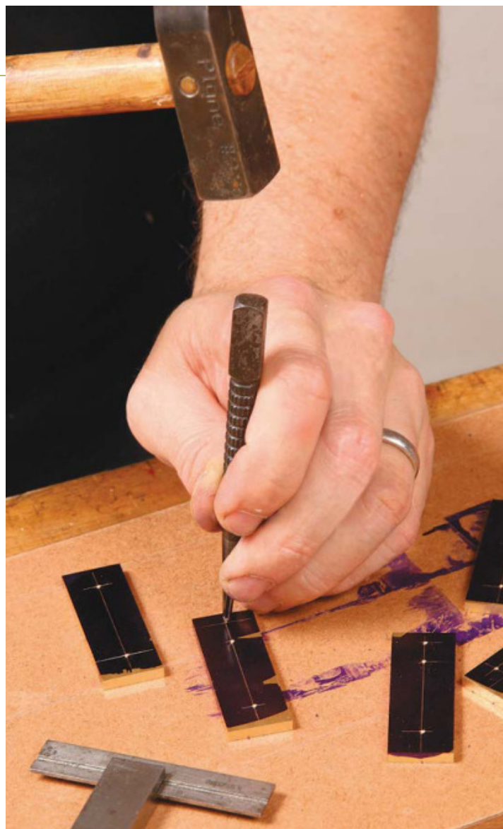
Accurate holes start with a dimple. A center punch leaves a small dent, which keeps the drill bit from wandering.
