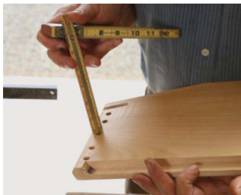
Measure depth and transfer. Measure the depth of the holes in the top and bottom pieces, and transfer that depth minus \frac{1}{16} in. to the dowels in the side pieces.
