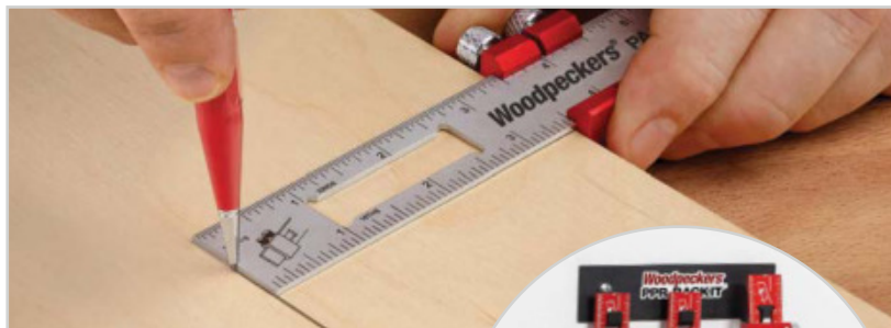
Above: Stop used to hold rule vertical, leaving your hands free for adjusting. Below: Paolini Rule used as a marking gauge. Notch keeps pencil centered.
