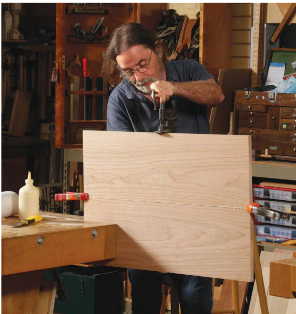
End with a flat panel. Stack the boards and check for flatness with a straightedge. Because of the spring joint, the boards should touch at the ends with a very small gap at the center. When clamped here, the joint will close and pressure will transfer to the ends. As you begin to tighten the clamp, push any bow into alignment if the boards aren't flush along the joint.
