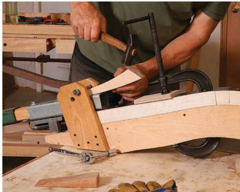
One more wedge. With the second C-clamp tight, Boggs adds a wedge to bring the part all the way home to the form. After 10 minutes on the bending form he'll move the part to a drying rack.
