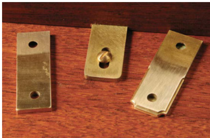
Match the look to the piece. Kellogg uses simple polishing and shaping techniques to adapt the look of the tabs to the style of the furniture he's building. Note how age and oxidation have given the installed tab at center a warm, matte look.
