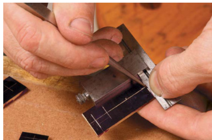
Accurate holes start with a dimple. A center punch leaves a small dent, which keeps the drill bit from wandering.
