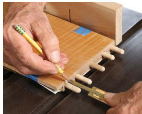
Measure depth and transfer. Measure the depth of the holes in the top and bottom pieces, and transfer that depth minus \frac{1}{16} in. to the dowels in the side pieces.
