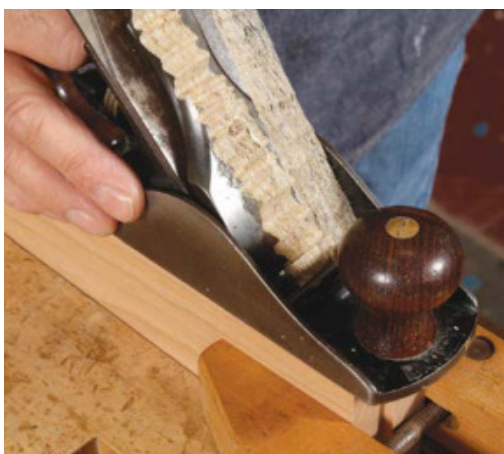
Final pass is full-length. A continuous shaving side to side and end to end ensures a quality surface for the strongest joint.
