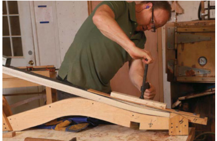
Clamp the first curve. Before pulling the part down onto the form, Boggs clamps the section that gets a concave curve.
