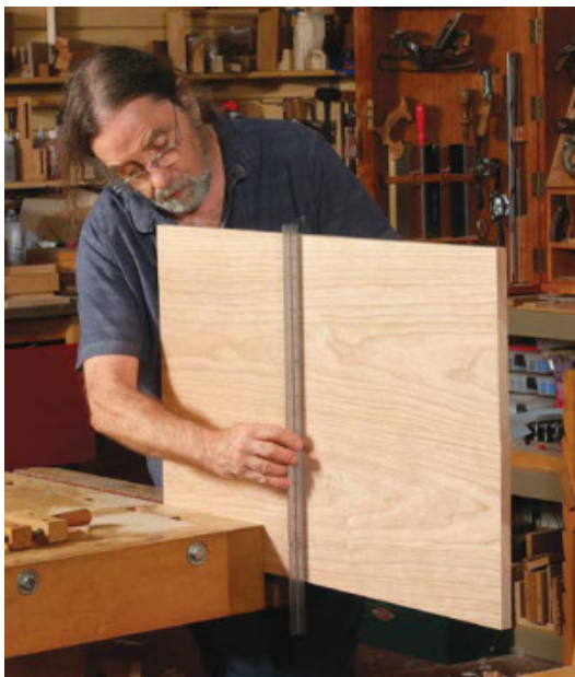
End with a flat panel. Stack the boards and check for flatness with a straightedge. Because of the spring joint, the boards should touch at the ends with a very small gap at the center. When clamped here, the joint will close and pressure will transfer to the ends. As you begin to tighten the clamp, push any bow into alignment if the boards aren't flush along the joint.
