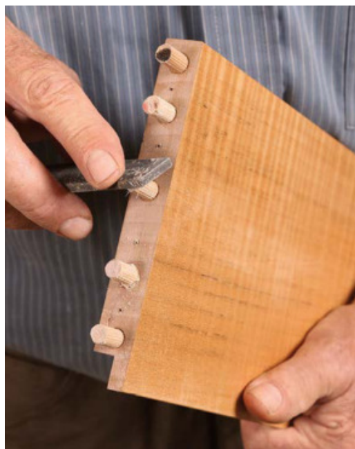
Cut dowels to length. With the dowels glued into the workpiece, crosscut them to length using a miter gauge. Then file a slight chamfer around the tips, making them easier to fit. Confirm that the dowel holes in the face-grain parts are about \frac{1}{16} in. deeper than the exposed dowel length. Welter uses fluted dowels, which will expand when glue is applied, ensuring a tight joint.
