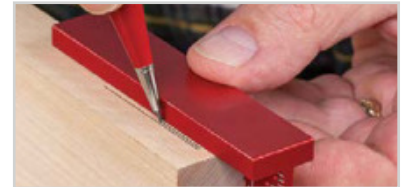
Locate center with the other side.
