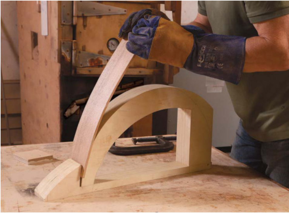
Bending form with a built-in clamp. With a slot at the lower end that pinches the workpiece in place, this form makes for an easy bend without a metal strap. Boggs clamps the upper end of the part to the form to let it set.
