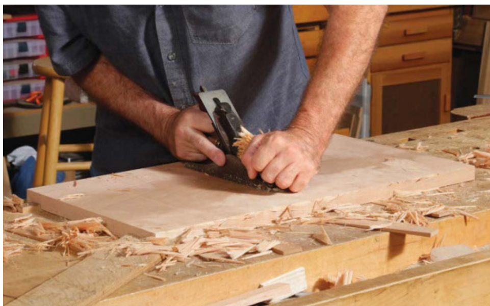
Cup up, wedges down. Van Dyke needs to stabilize the board before he planes it, so he uses wedges and his tail vise.
