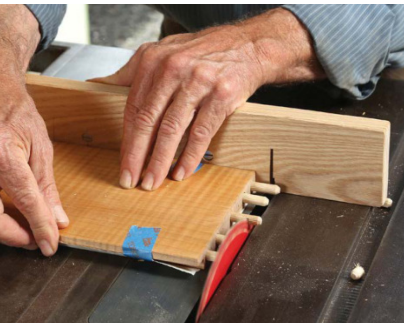
The first step. Glue the dowels into both ends of the side pieces.
