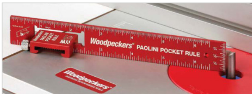
Above: Stop used to hold rule vertical, leaving your hands free for adjusting. Below: Paolini Rule used as a marking gauge. Notch keeps pencil centered.
