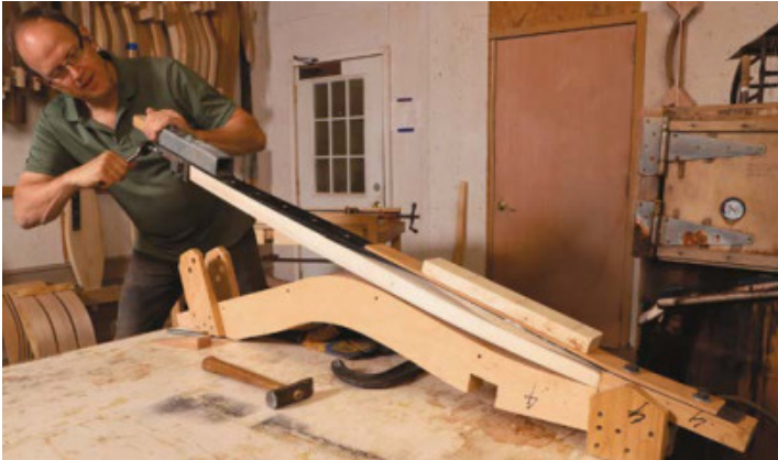
Commercial compression. To bend these chair posts, Boggs uses a compression strap from Lee Valley. After inserting the workpiece he tightens the adjustable foot, snugging it up to the end of the part.
