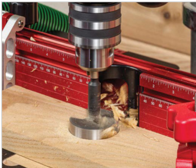
Dust collecting DP-PRO Fence captures dust and chips at the source.
