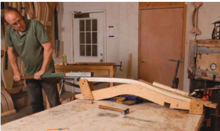
Time for some serious leverage. After re-tightening the adjustable foot and fully tightening the C-clamp, Boggs pulls down with the compression strap, inserting a cheater bar for extra leverage.
