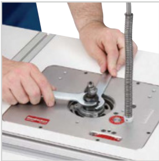
Above-the-table router bit changes with many router models.
