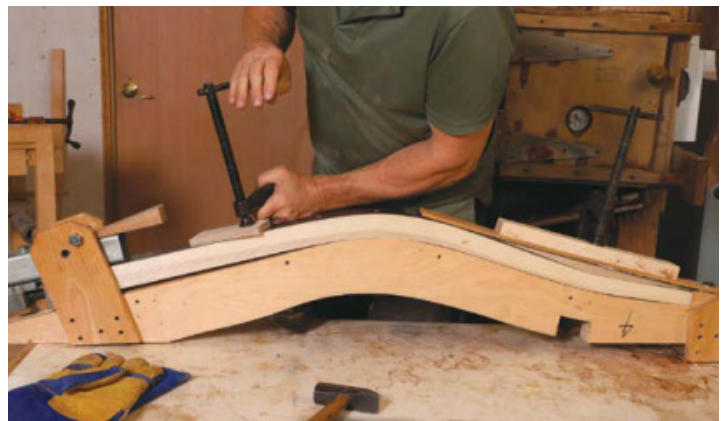
Wedge and clamp. To keep the workpiece close to the form, Boggs uses a pin and wedge system. Then he applies pressure with a second C-clamp to pull the part to the form.
