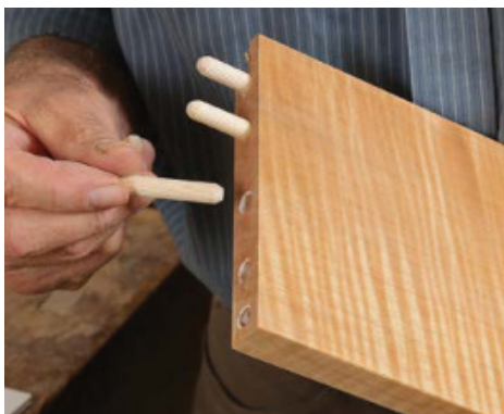
The first step. Glue the dowels into both ends of the side pieces.
