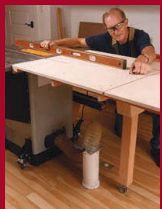
Easy height adjustment. The sturdy support leg can be adjusted from above the table to compensate for uneven floors, as well as for mobile bases that raise and lower the saw.
