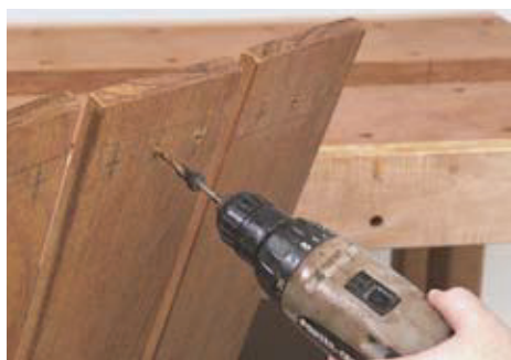
Drill pilot holes for the cleat. But don't create countersinks. Those go on the other side.
