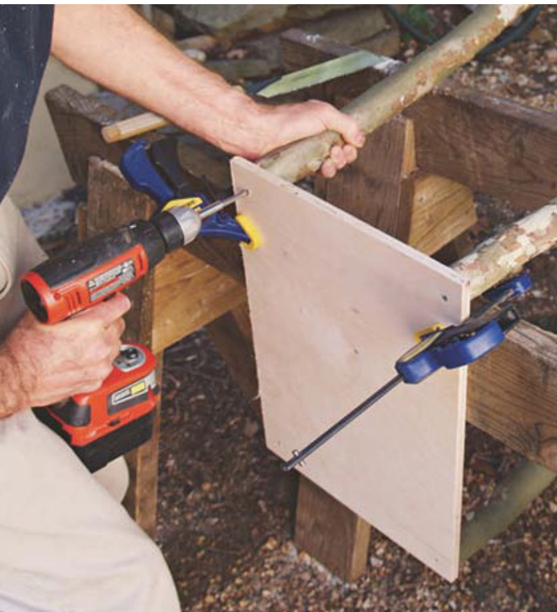
Screw the legs in place. Clamp the top to sawhorses. The sawhorses also support the legs as you screw them in place.
