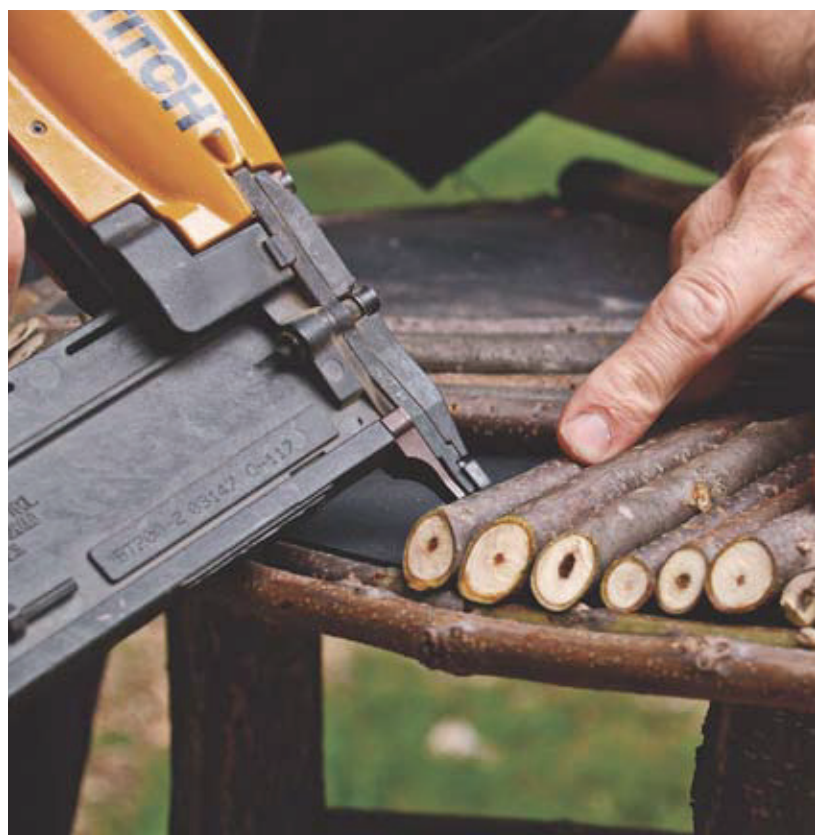
Finish the top. Arrange sticks in a pattern and nail them in place on the top.
