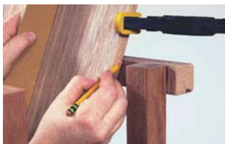
Mark for the back. This shows where to pre-drill the back for a screw. Use a spacer to set the distance between the back planks.
