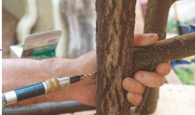
Predrill, countersink, and screw the legs to the cross-stretchers. The \frac{3}{8} -in. countersunk hole is just the right size for a dowel plug.
