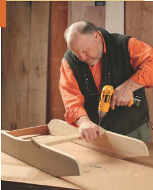
Make a subassembly. Screw the stretcher to the front and follow with the lower cradle.
