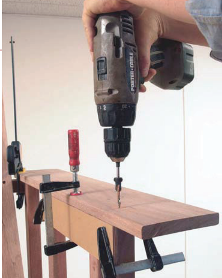
Attach the arm. Drill the countersinks with the arm in place so that the holes are located accurately. Use plywood to set the overhang.
