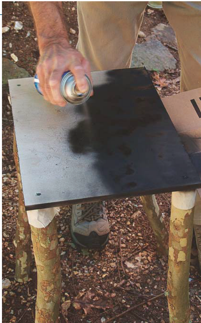
Paint the plywood top. Spray paint works best. Use a piece of cardboard to shield the legs from overspray. Also, put masking tape around the tops of each leg for extra protection.
