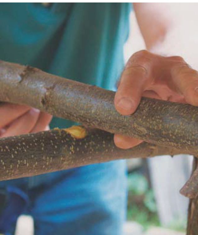
Notch the second stretchers. Use a knife to cut the notch. This small joint increases the base's strength.
