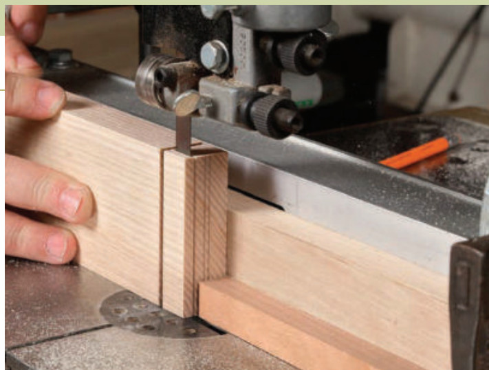
Bandsawn cheeks. Cut the aprons' front and back cheeks using the bandsaw. Set a stop to keep from cutting into the shoulder.
