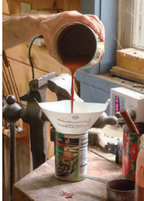
Strain the mixture. After stirring well, pour the paint through a conical paper strainer to keep lumps and foam out of the mixture.
