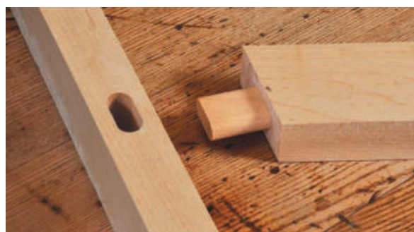
This versatile tool handles both sides of a joint. Riding along the inside and outside of a template will yield each half of a joint. Angled tenons are just as easy as straight ones.
