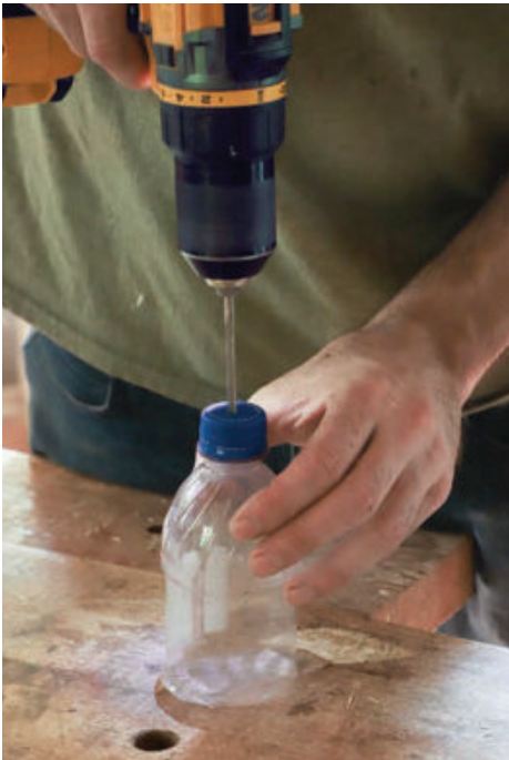
High-tech viscosity gauge. To make a device to measure viscosity, cut a plastic soda bottle in half at the waist, then drill a \frac{5}{32} -in.-dia. hole in the lid.
