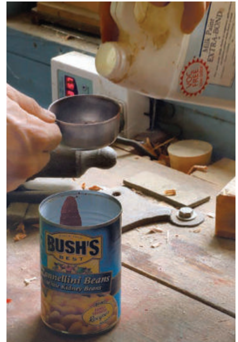
Make the first coat stickier. You can increase milk paint's adhesion to bare wood by using an additive like Extra Bond. Mix in one part additive to two parts milk paint.
