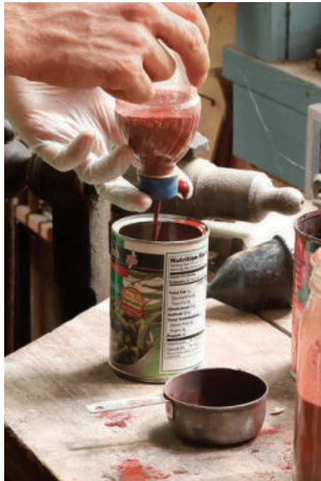
The gauge in use. Cover the hole and pour in \frac{1}{2} cup of paint. Uncover the hole and see how long it takes the paint to flow out. Nine to 11 seconds is about right.
