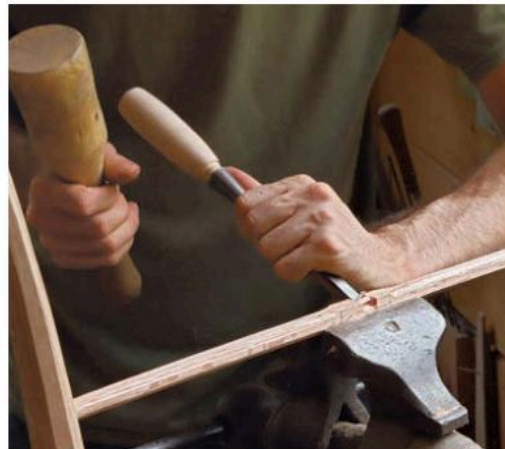
Hand tool half-lap. Cut to your knife lines with a handsaw, then chisel out the waste between the sawkerfs.
