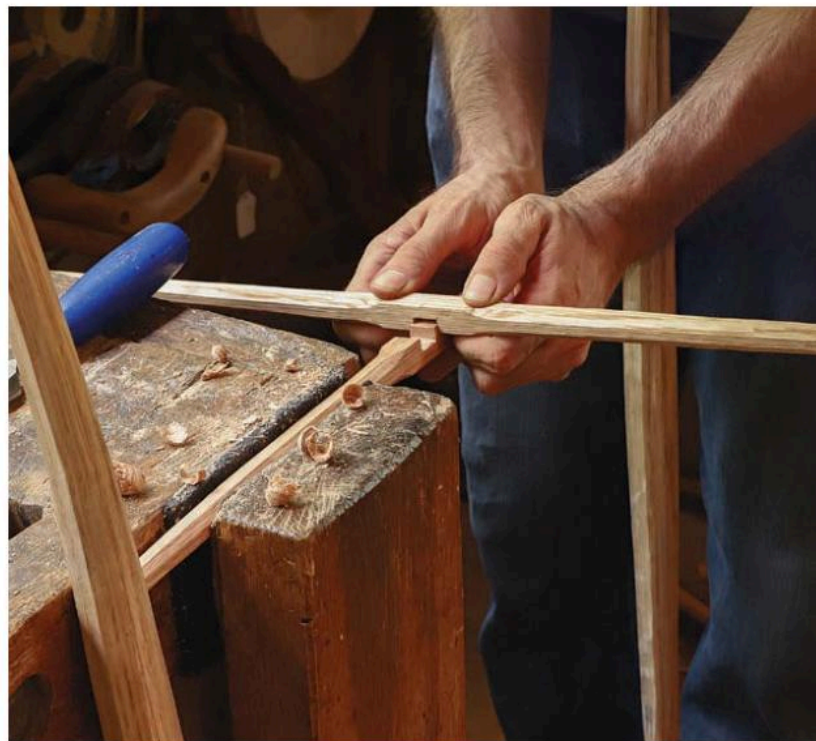
Test time. To dial in the width of the half-lap, test it on the un-notched section of the other stretcher. Adjust the cheeks with a chisel if necessary.
