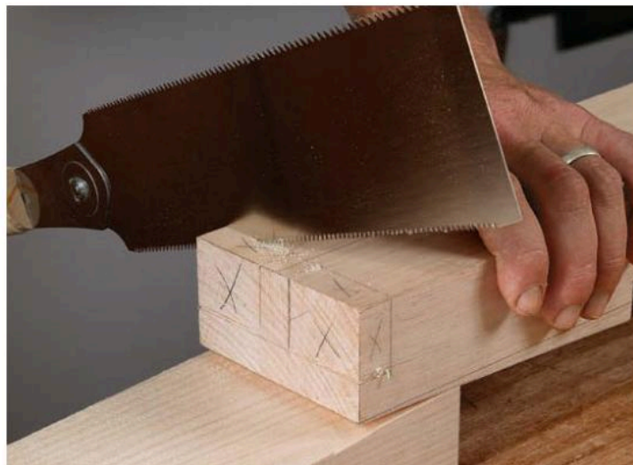
Start sawing the end T-notch. Cut the rips before the crosscuts. Hunter uses an offcut to support the workpiece.
