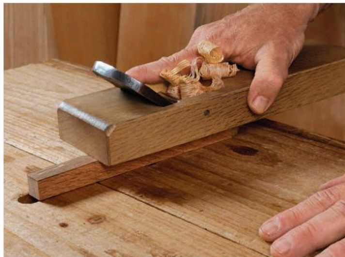
Wedge needs a taper. For the wedge to work, saw a \frac{1}{16} -in. taper on the step of one half of the joint (left). Then make a hardwood pin to fit (above). Make the pin overlong so you can trim it flush later.
