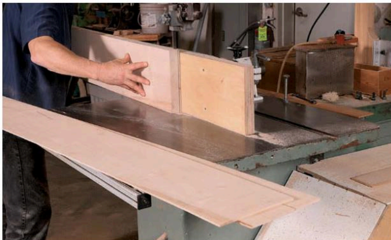
First build a fence. Boggs uses a high fence on the bandsaw when slicing laminates for bending.
