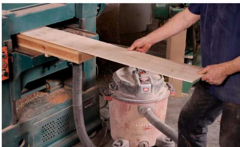
Suction table for the planer ensures smooth results. With a port on the bottom for the shop vacuum and slots on the top to suck down the laminates, Boggs's hollow suction table lets him plane very thin laminates.
