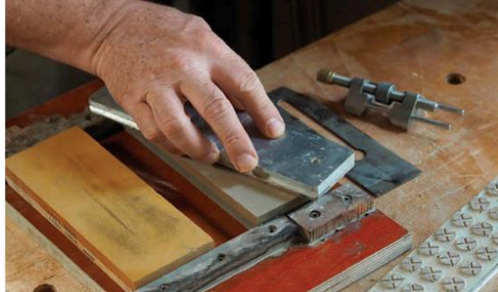
Raised abrasives cut quickly. With more edges in contact with the waterstone, these lapping plates surface the stones faster.
