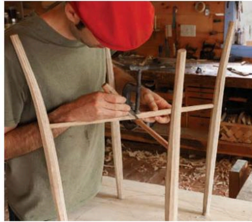
Clamp and scribe. With one subassembly fully dry-fitted into the tabletop and the other lowered in until the stretchers make contact, use a knife to mark where the stretchers cross. Remove the subassemblies and finish the layout with a square and a marking gauge.
