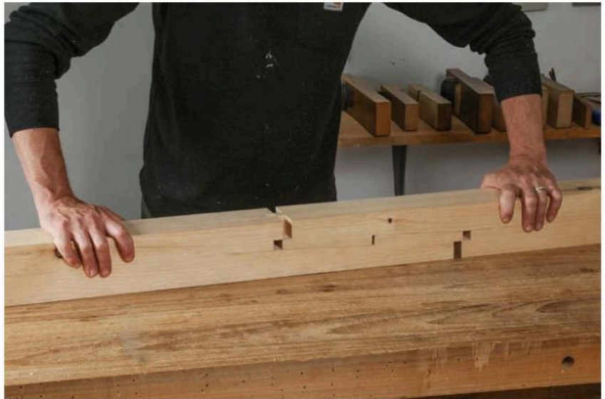
Give it a squeeze. Place one half on top of the other and press the joint together with a few light hammer taps to test the fit.
