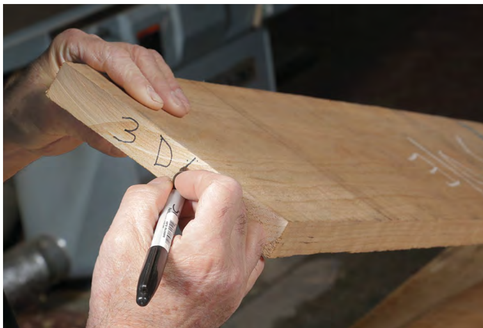
Label the ends. Cleaning the board's surfaces at the jointer and planer will remove your marks there; moving them to the ends lets you keep track of the parts.
