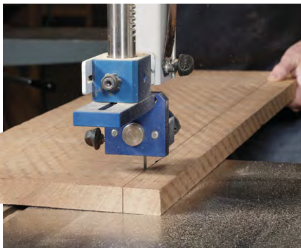
Cut to rough length and width. Rough boards are unsteady, making the chopsaw and bandsaw the safer tools.
