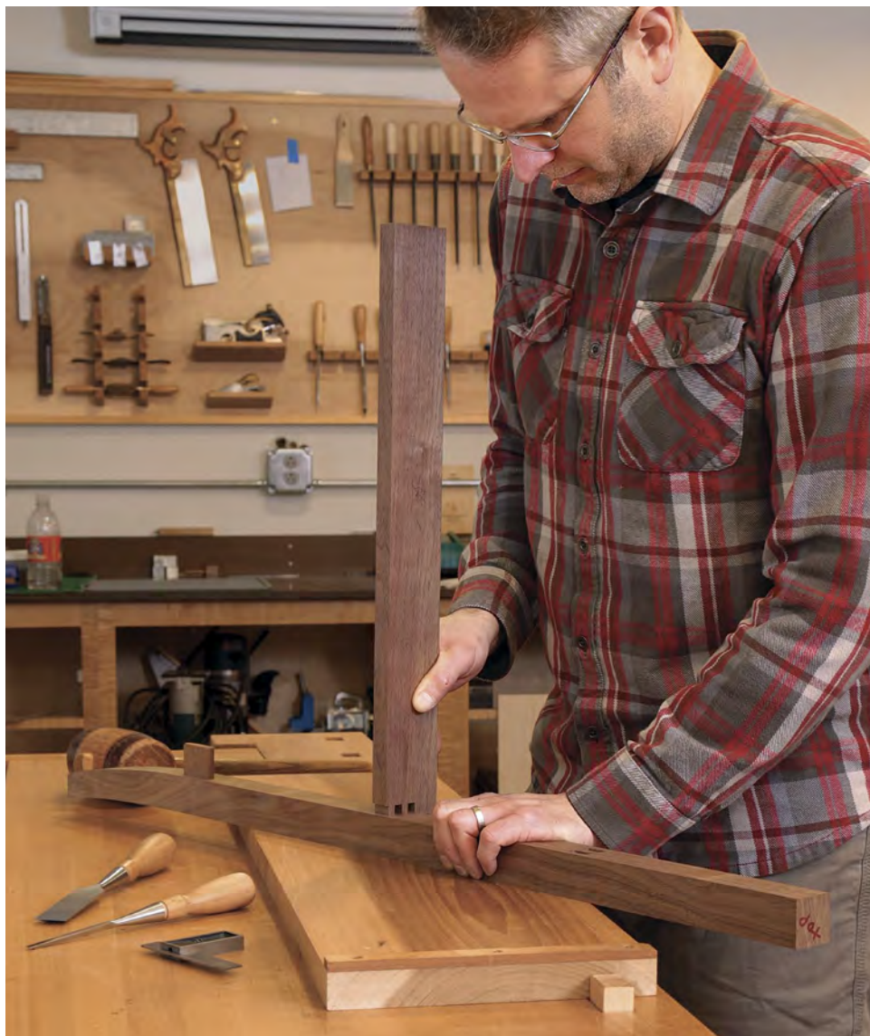
Last task. Square up the rounded corners of the router cuts, removing most of the waste before finishing with a last light paring pass right at the shoulder line.
