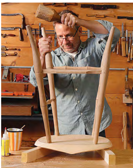
Dry tenons. Fit the legs up through the seat without glue, and make marks for tenon wedges perpendicular to the seat's grain direction.
