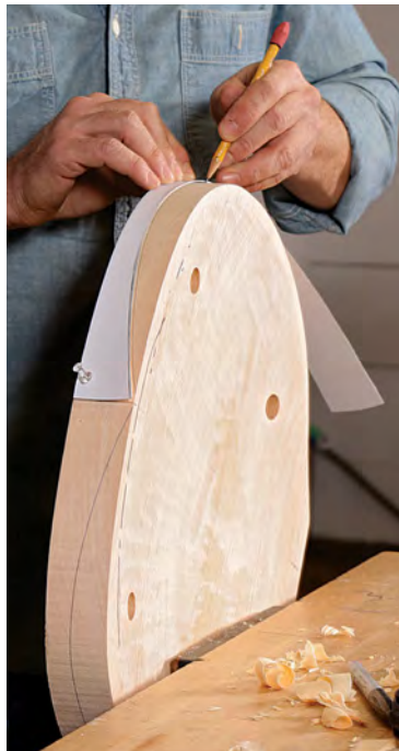
First the dish. Using an inshave (or a large gouge) relieve a wide oval-shaped area toward the back of the seat. Galbert drills two \frac{5}{8} -in.-deep holes to guide the depth of the dish.
