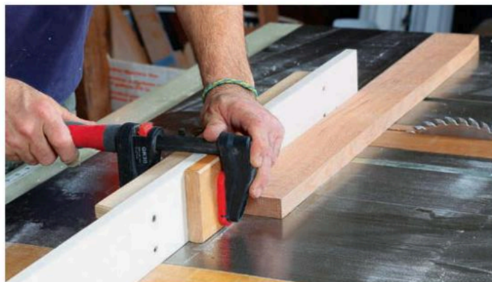
Room to turn. The position of the GearKlamp's handle left Dunton plenty of space to operate it. Here he's securing a stop block to his miter gauge and his fingers don't get trapped between the handle and the saw table.
