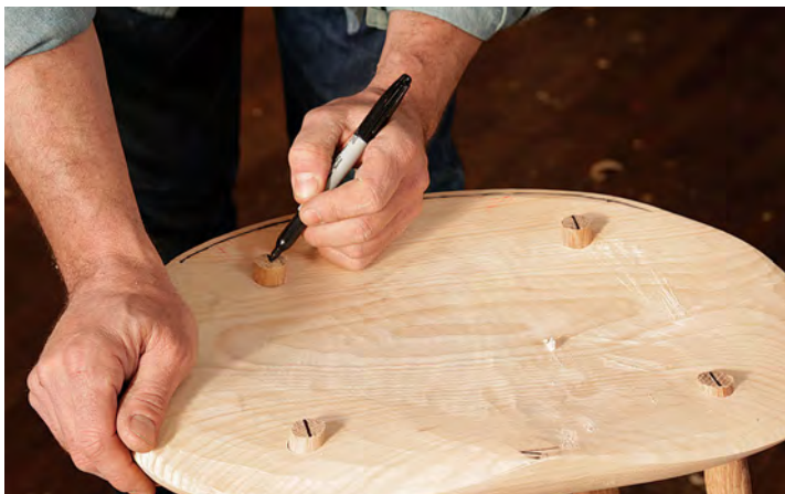
Dry tenons. Fit the legs up through the seat without glue, and make marks for tenon wedges perpendicular to the seat's grain direction.
