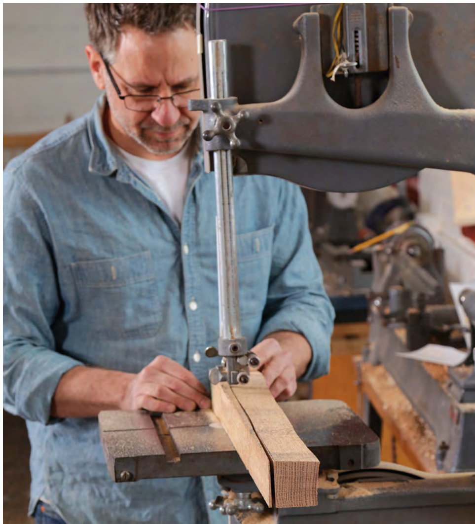
Sawn or split. If you don't have green wood to split from the log, you can saw your leg stock from lumber.
