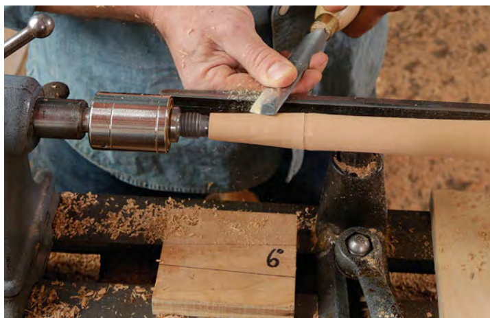
Tapered tenons. While turning the tapered tenons at the top of the legs, Galbert uses a template placed on the lathe bed with a 6° taper drawn on it as a guide.
