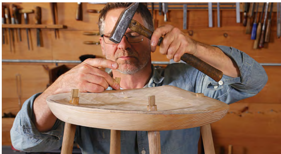
Glue and bang, then drive a wedge. To knock the legs home at final assembly, Galbert elevates the inverted stool on spacers. Then he flips the stool and glues and drives the wedges.
