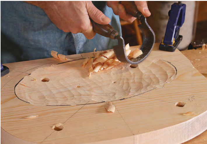
First the dish. Using an inshave (or a large gouge) relieve a wide oval-shaped area toward the back of the seat. Galbert drills two \frac{5}{8} -in.-deep holes to guide the depth of the dish.
