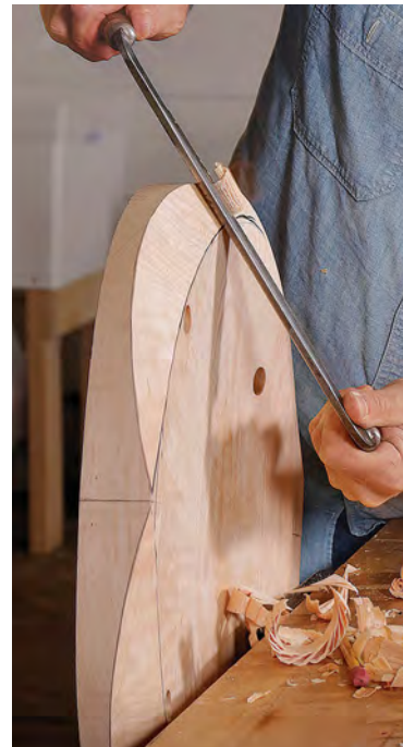
Edgework. Flexible thin plastic makes perfect template material for laying out the shaping at the edge of the seat (far left). To shape the edge, Galbert uses a drawknife to create a series of chamfers, first broad, then narrower.
