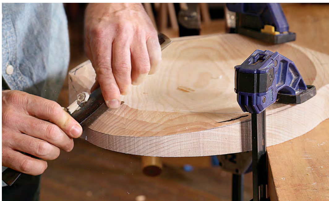
Spokeshave blends the facets. After shaping the edge with drawknifed chamfers, blend them to a fair curve with a spokeshave.
