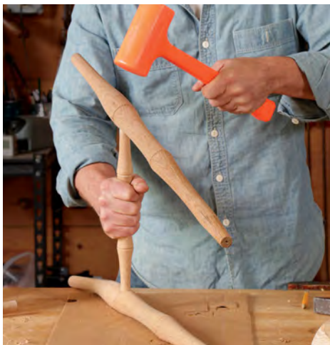
Front and rear first. Using Old Brown Glue, which has a leisurely open time, Galbert begins assembly by gluing in the rear stretcher and the footrest.
