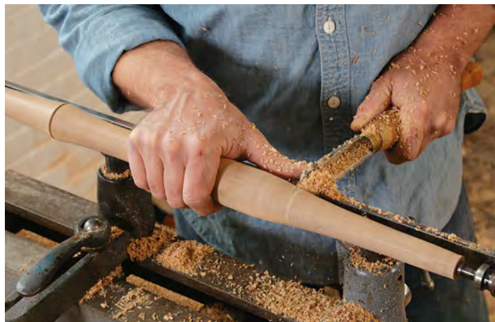
Double curve. To turn the S-curved bottom section of the leg, where the bend will be, first make a long shallow concavity, then complete the shape by cutting downhill to create the adjoining convex section.
