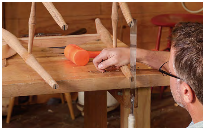
Kerfs for wedges. After removing the legs from the seat, follow your layout lines to cut kerfs for the tenon wedges.
