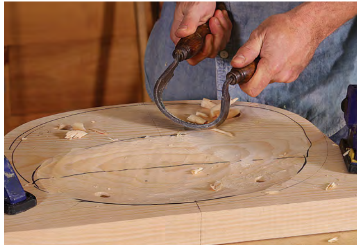
Then the ramp. Use an inshave to carve an angled plane from the deepest part of the dish up to the front rim of the seat.
