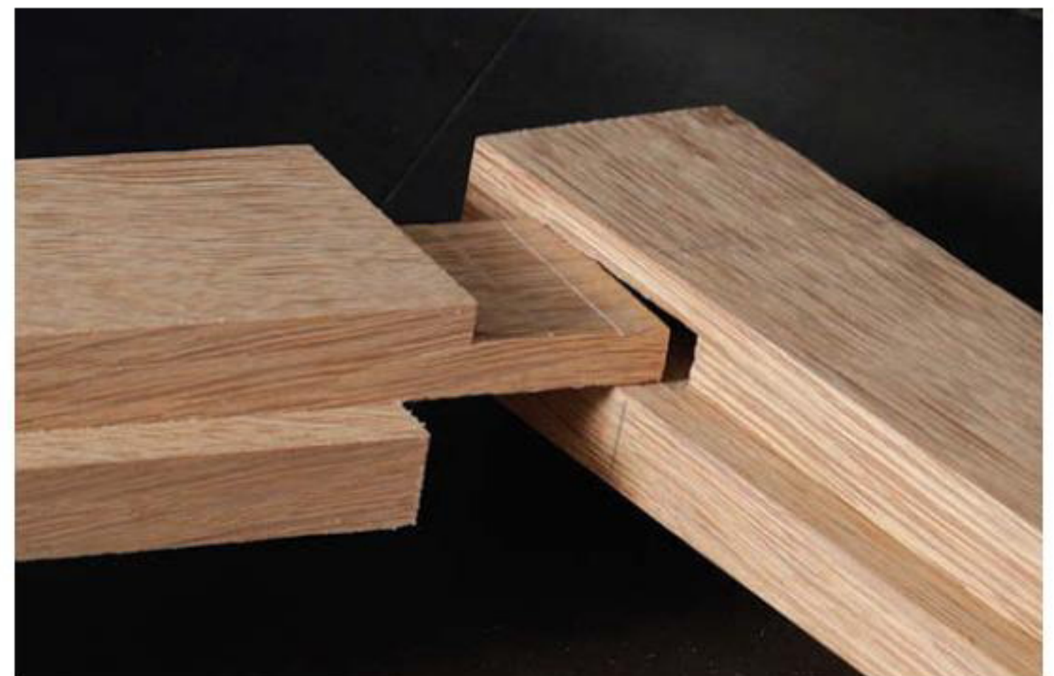
Cut the front tenon cheek. Adjust the fence to the final width of the tenon and use a miter gauge to cut the cheek in two passes.
