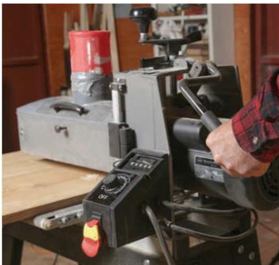
Fast-acting lever. Bickford appreciated the lever for quick large-scale adjustments to the drum height. The sander has a micro-adjustment wheel as well.
