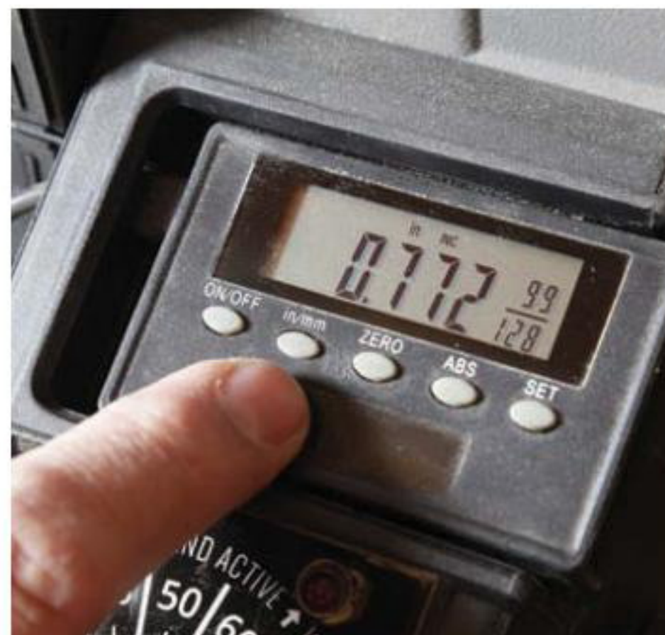
Digital readout. The scale, which displays the space between the drum and the bed, can be set to imperial or metric.
