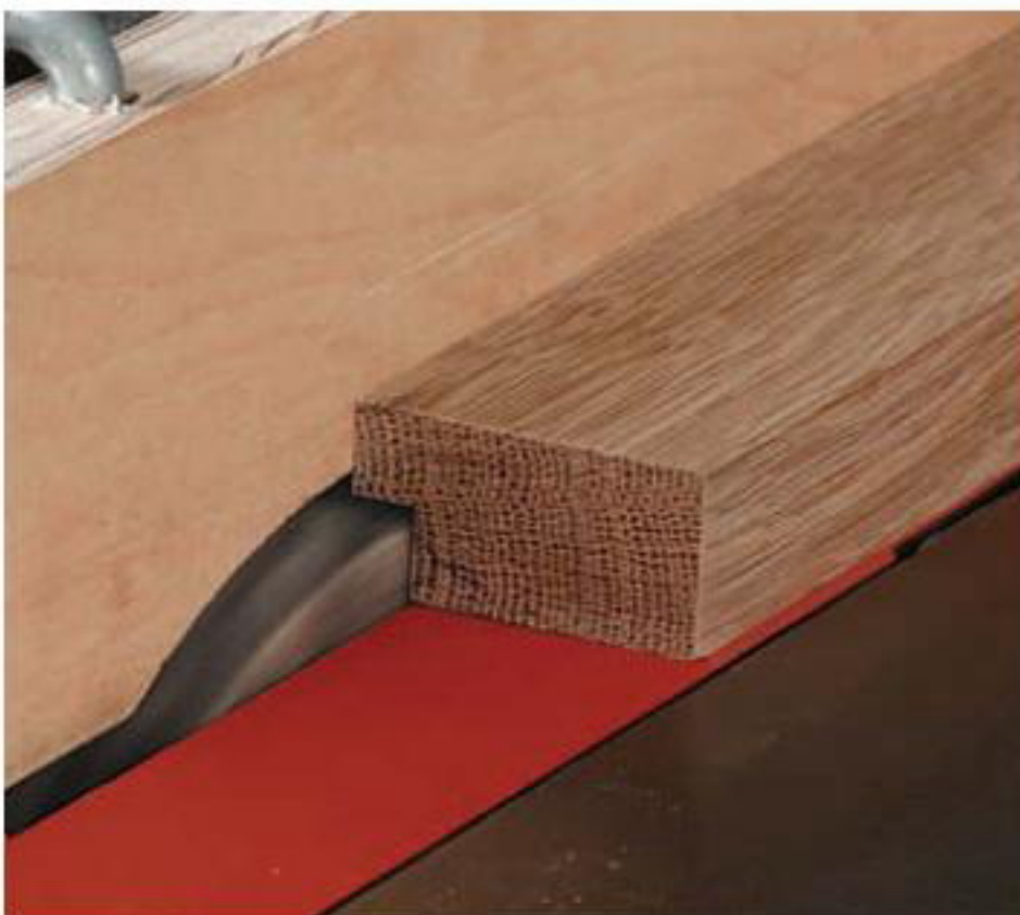
Start with the rabbet. Use a dado blade partially buried in a sacrificial fence to make the cut.
