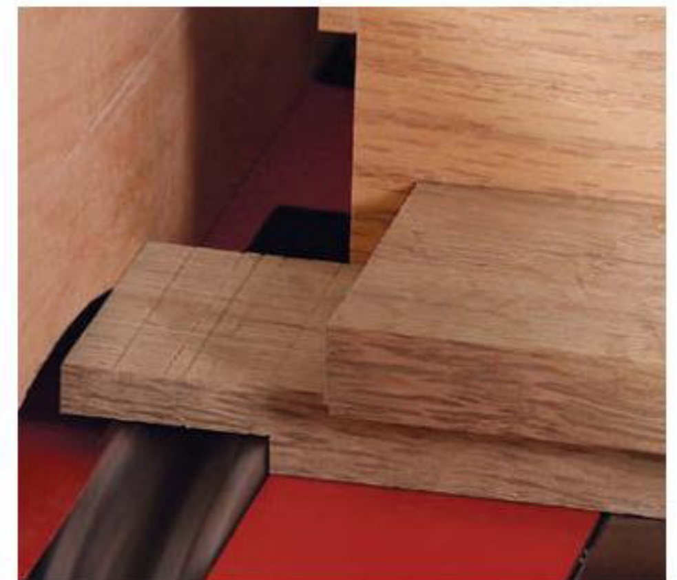
Cut the rear cheek. Adjust the fence to account for the width of the rabbet when cutting the second cheek.
