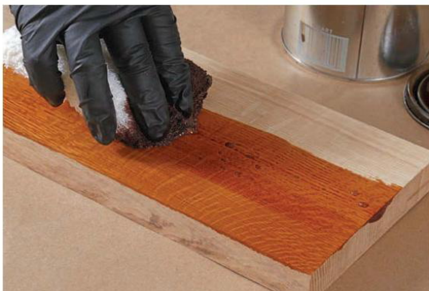
Dye and seal. Sandry adds an overall tone to the wood by wiping on TransTint golden brown dye (above). Then he seals the finish with SealCoat, a blond dewaxed shellac (right).
