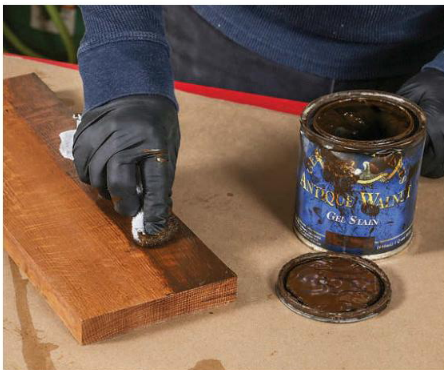
Add a glaze. Sandry uses General Finishes walnut gel stain as a glaze to darken the pores and highlight the medullary rays of the oak. He works the stain into the wood, then wipes it off to achieve the desired color. Sandry sealed it with a sprayed lacquer, but any satin finish would be appropriate.
