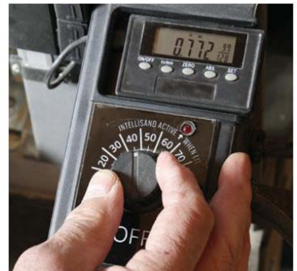
Speed control. A dial rheostat controls the conveyor speed up to a maximum of 10 ft. per minute.
