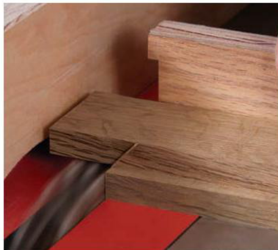
Cut the front tenon cheek. Adjust the fence to the final width of the tenon and use a miter gauge to cut the cheek in two passes.
