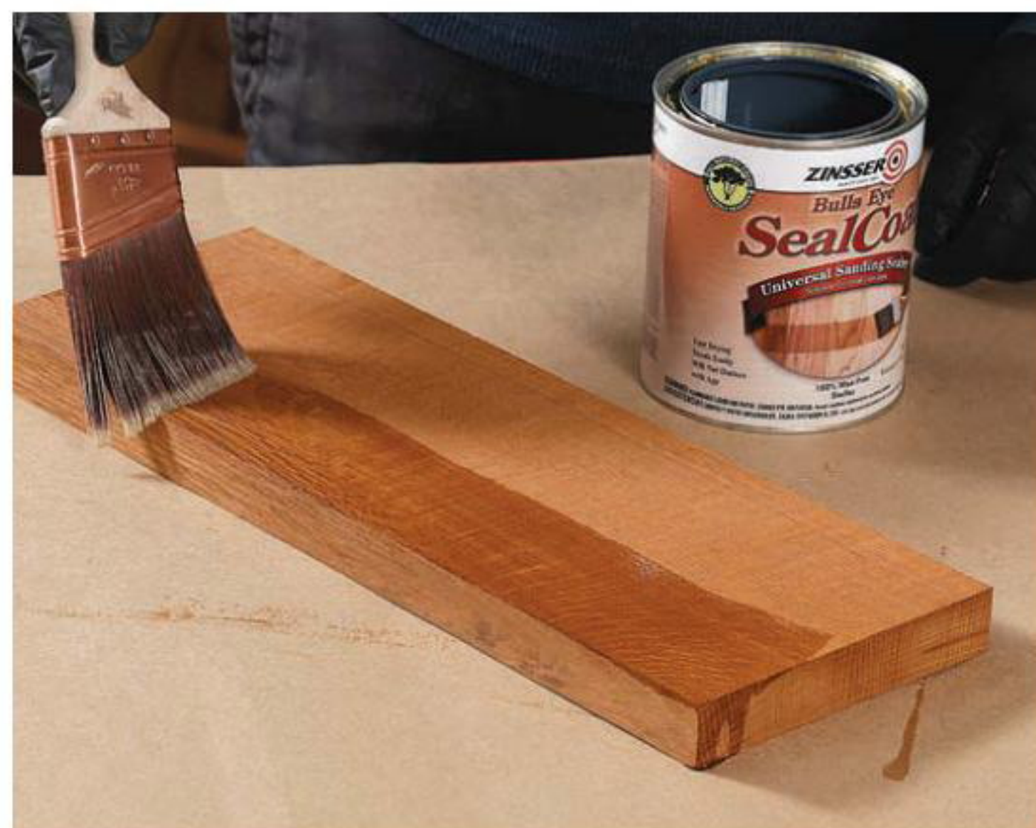
Dye and seal. Sandry adds an overall tone to the wood by wiping on TransTint golden brown dye (above). Then he seals the finish with SealCoat, a blond dewaxed shellac (right).
