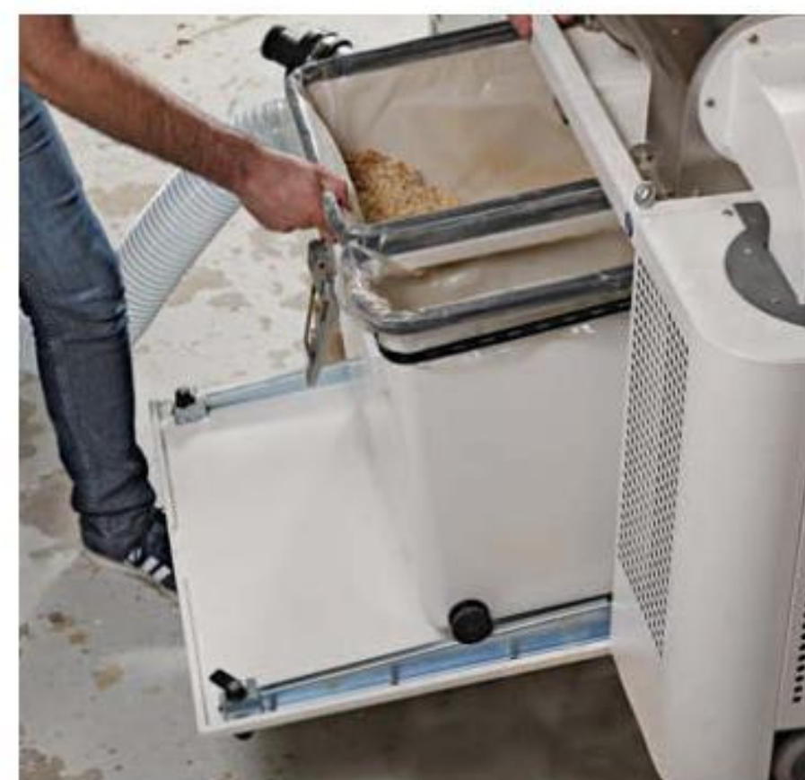
Take out the trash. Emptying the machine is simple, as the internally mounted bins slide out easily. The larger bin collects larger chips, while dust goes into the smaller container.
