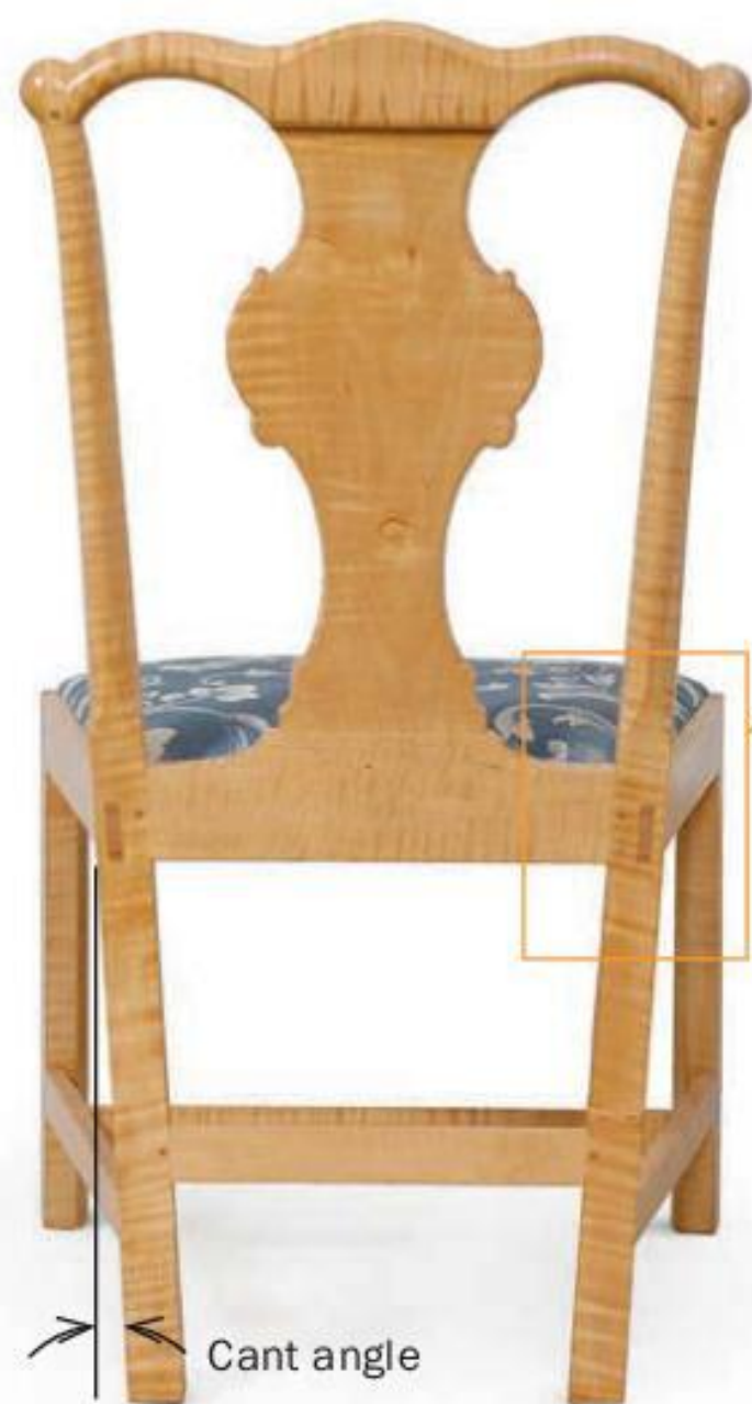
Seen from the back, the legs on a Chippendale chair tilt in at the bottom. This is the cant angle.
