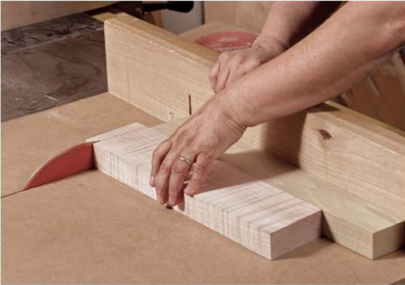
Cut the rail blank to length, angling the ends. Brown uses a wedge against the fence of his crosscut sled to hold the stock at the cant angle.
