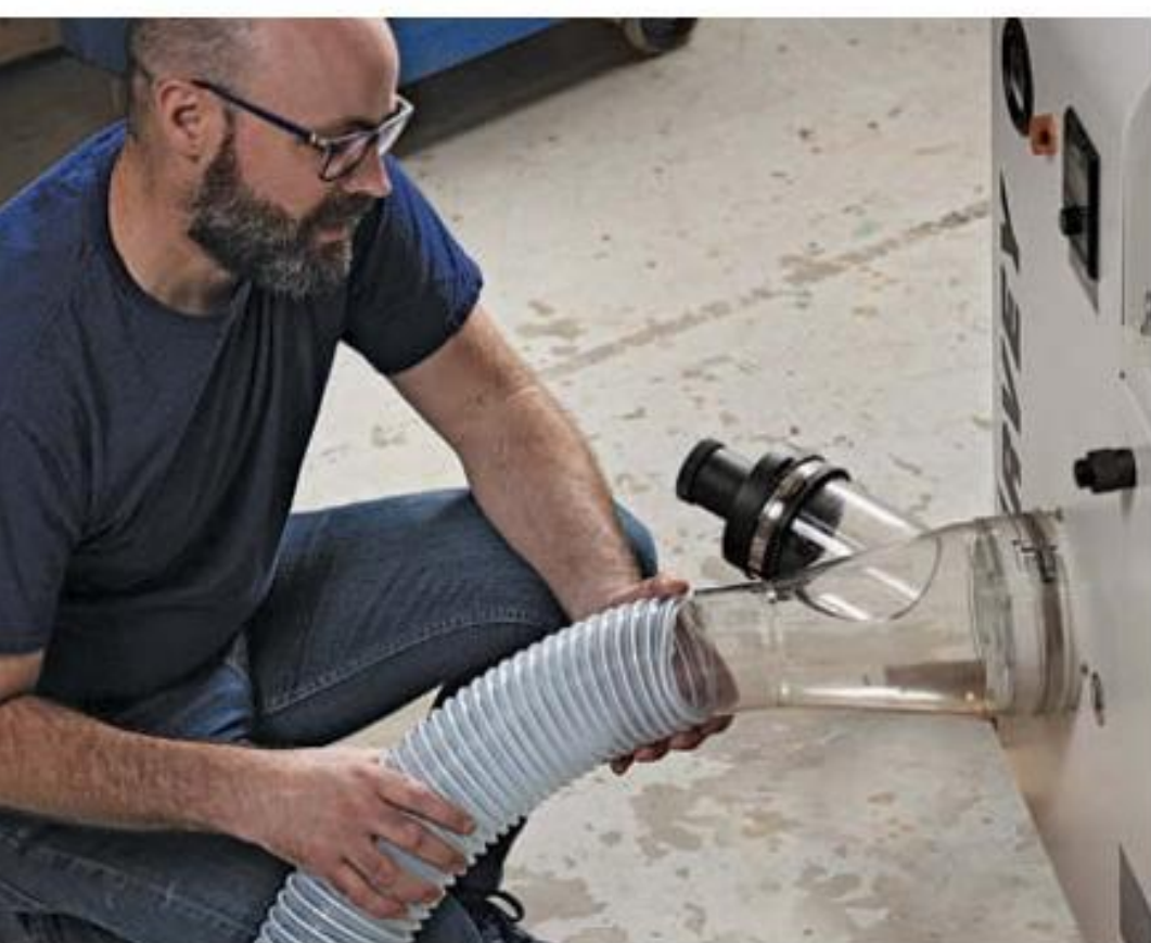
Ready to reduce. Provided with the unit is a split connector with a 4-in. port and a 2-in. port. It fits over the 6-in. inlet port.
