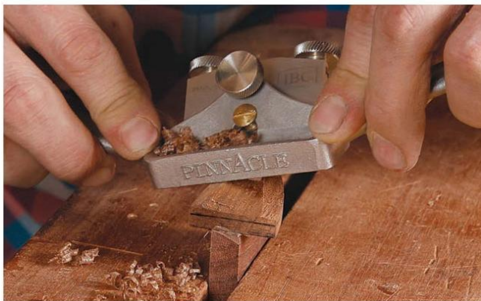
Round the front. After removing the temporary handle from the front of the pendant, hot-glue a handle to the hollow back. Clamp it in a vise, and round the front of the pendant with a spokeshave or a small block plane.
