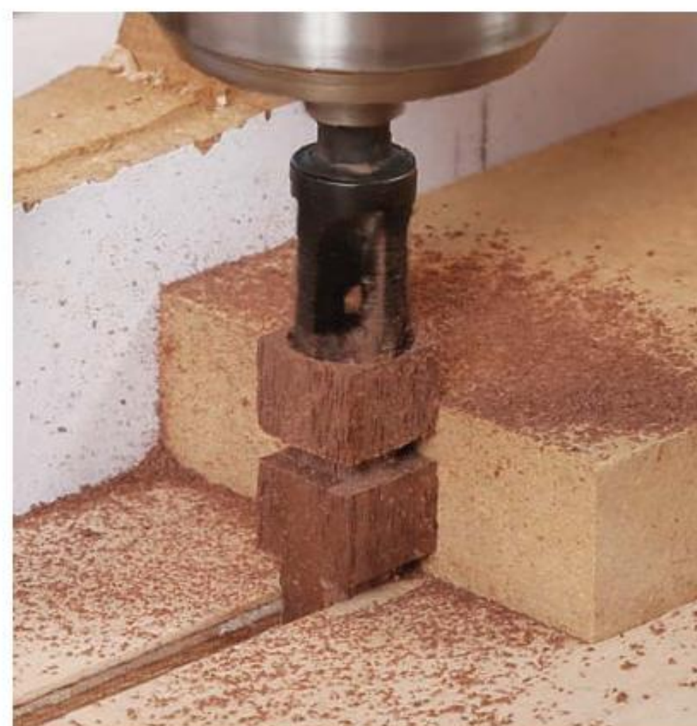
Cut the round tenon. A plug-cutter is the perfect tool for the job. Morley sets the stop so that the blank is centered under the cutter.
