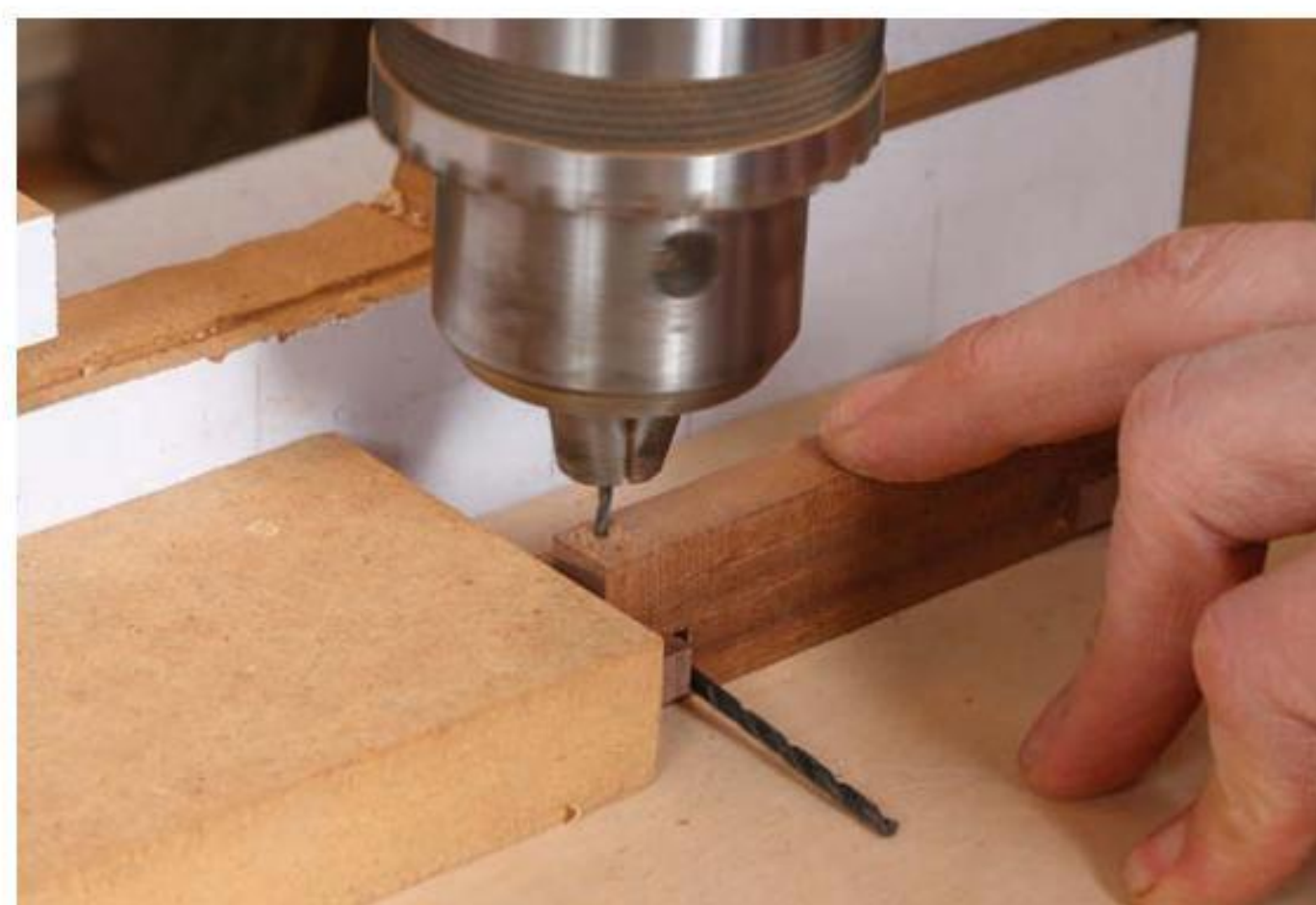
Drill for the pin. Fit the post and pendant blank together using a \frac{1}{16} -in.-dia. drill bit as a spacer. Push the pendant blank into the groove and against the stop (left). Then drill a \frac{1}{16} -in. hole through the pendant and post (above).
