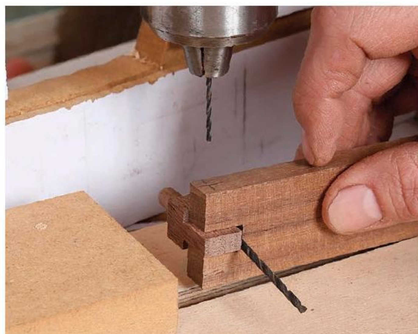
Drill for the pin. Fit the post and pendant blank together using a \frac{1}{16} -in.-dia. drill bit as a spacer. Push the pendant blank into the groove and against the stop (left). Then drill a \frac{1}{16} -in. hole through the pendant and post (above).
