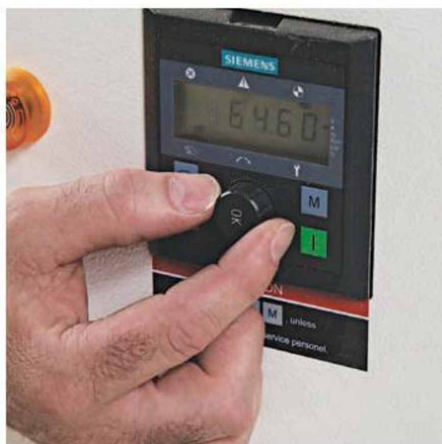
Variable speed. In addition to a soft start, the machine has a dial that lets you vary its speed to adjust the suction to the task at hand.
