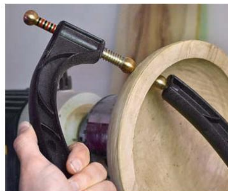
Sliding scale. A spring-loaded pin keeps two measuring points tight against the inner and outer surfaces, and the color-coded stripes on the top of the pin indicate the bowl's thickness.
