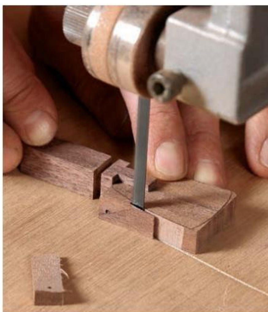
Rough out the pendant. After tracing a template onto the blank, bandsaw to the line. A spare post blank serves as a push stick.
