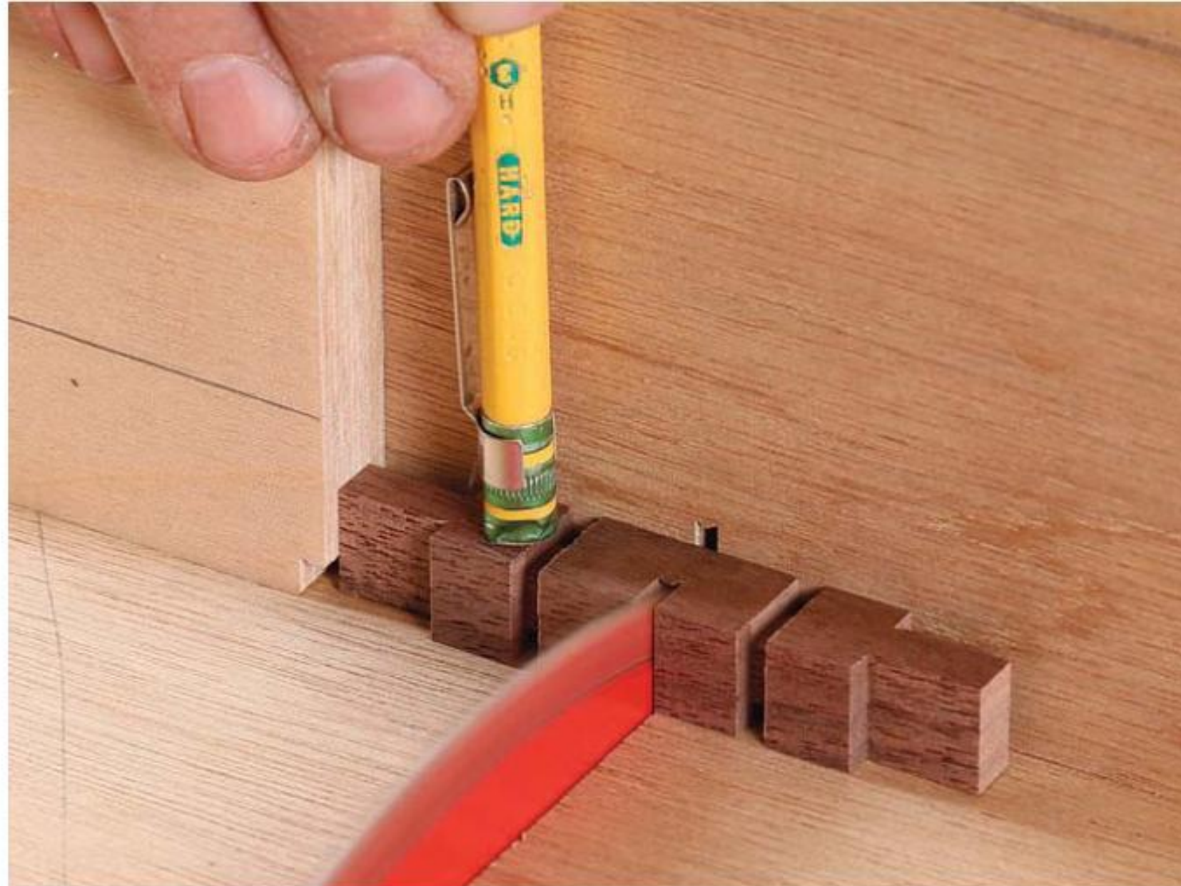
Two posts from one blank. Cut both posts to length using a stop.
