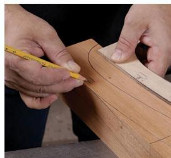
Leg layout. After tracing the side pattern onto the blank, mark the ankle for a chamfer. Mark the leg's center by eye, then mark a little less than halfway to the back edge.
