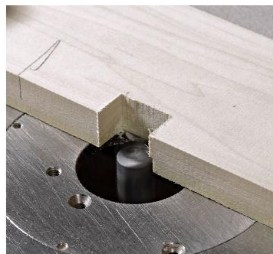
Zero-clearance fence stops tearout. With the right end clamped down, pivot the fence onto the bit so that it cuts the right side of the precut notch. Keep the opening small to prevent stock from tipping into the space.
