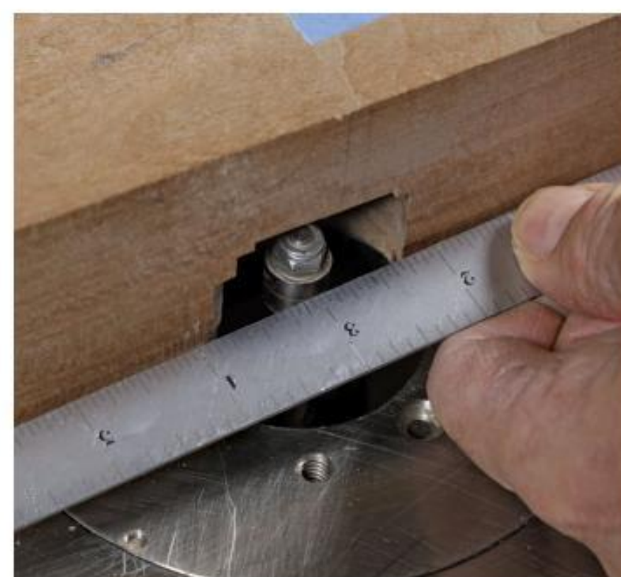
Fence and bearing should be flush. This makes cuts safer and more accurate.
