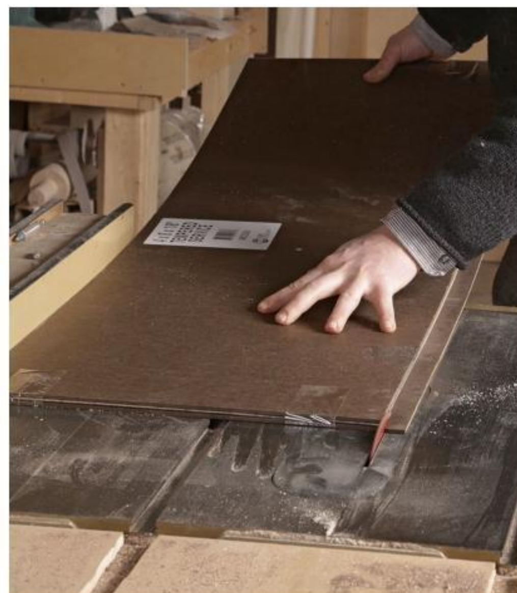
Cut the blotter to depth. With the leather glued to the Masonite backer, sandwich the leather with another piece of loose Masonite, and rip to final width.
