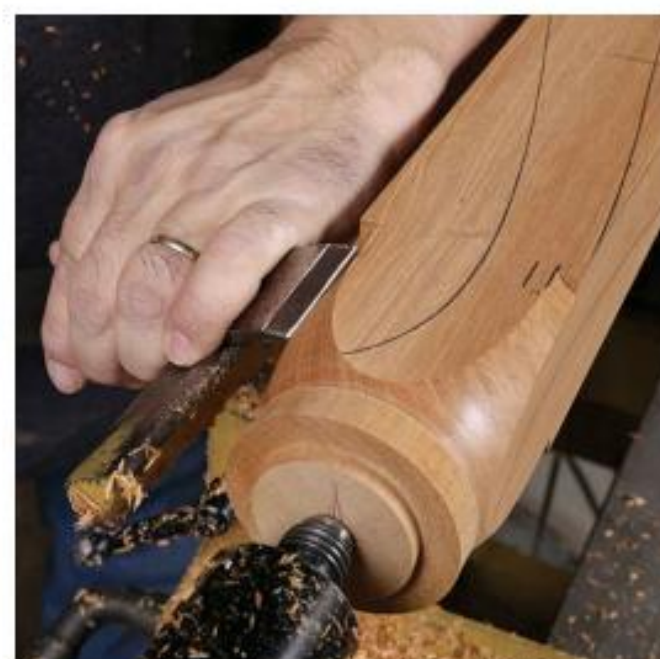
Turn the heel. The inward sweep at the back of the ankle is created by turning a fair curve with a skew chisel. It begins at the chamfer mark and sweeps right down to the scribe line at the top of the foot.
