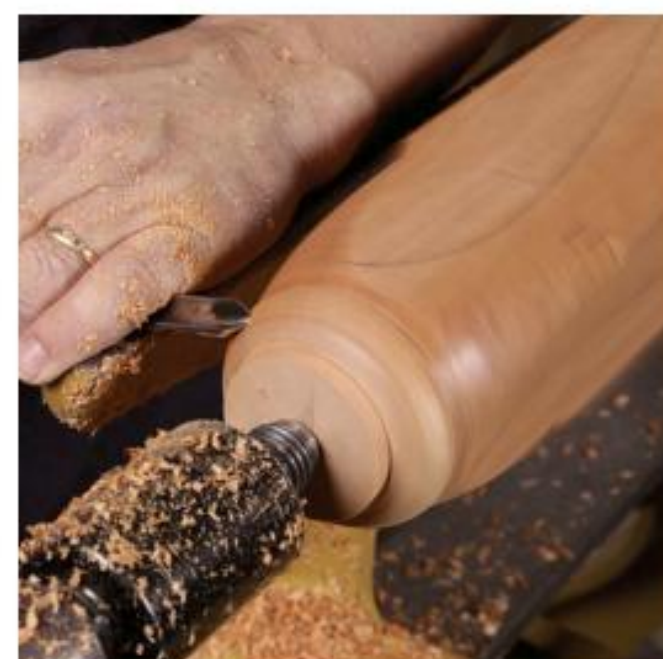
The foot curves under. With the heel curve shaped, you now have access to turn the underside of the foot to its curved profile. You can make this cut with a skew, a spindle gouge, or a scraper.
