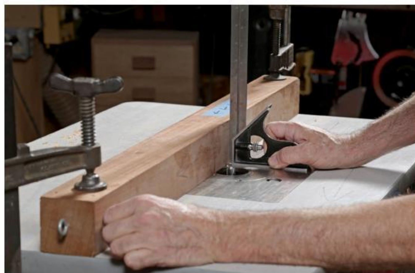
Clamp and check for square. Van Dyke finds that the simplest and most reliable fence is just a thick piece of stock milled straight and square.
