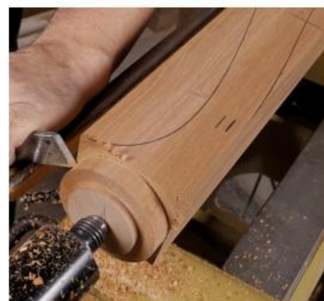
Scribe with a skew. After turning the foot to a cylinder, use a skew to make a deep scribe line at the top of the foot. This will help as you carve the top of the foot.
