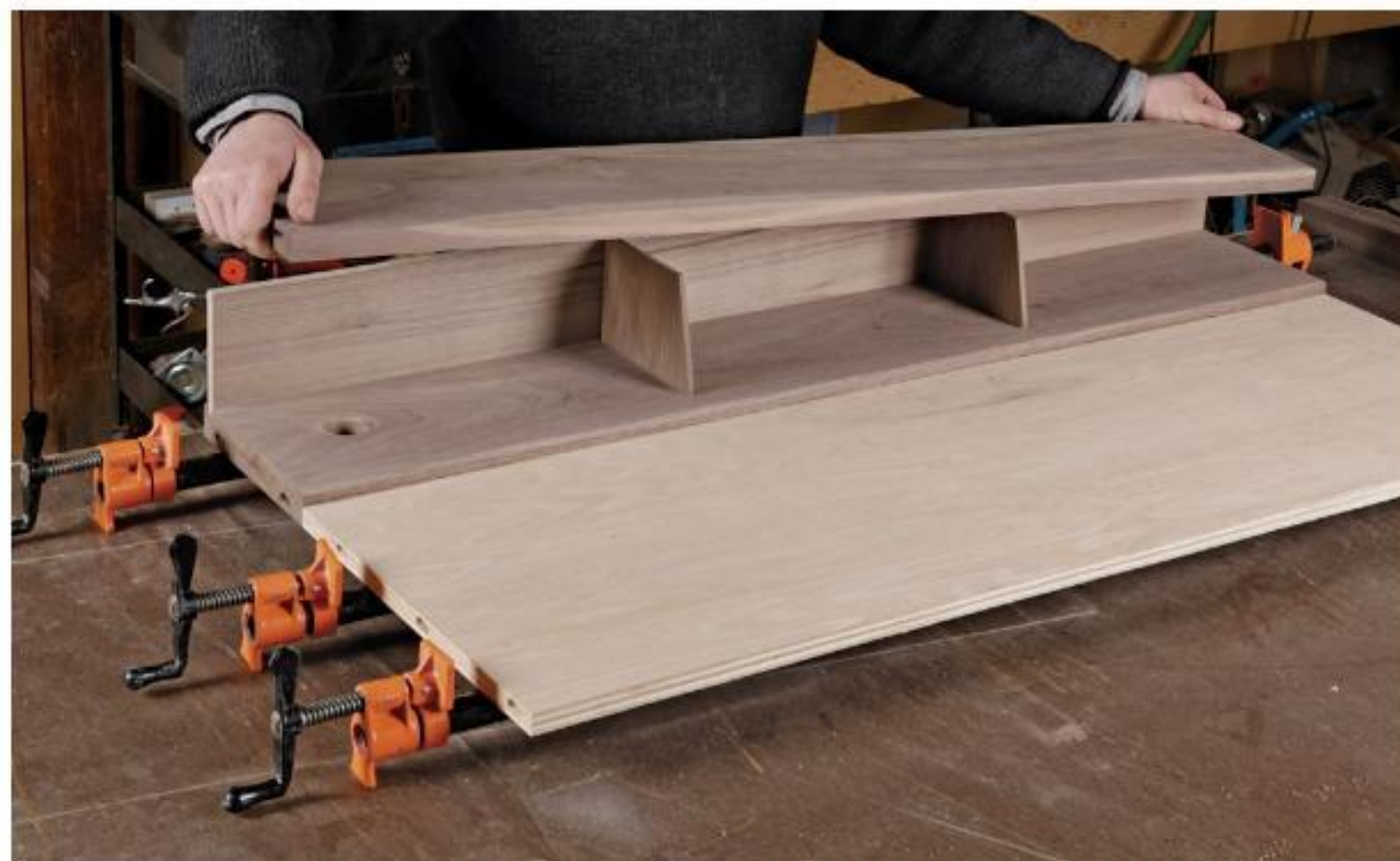
Final assembly. After setting the gallery back and drawer dividers in place, fit the gallery top (left). Then add the end caps (below).
