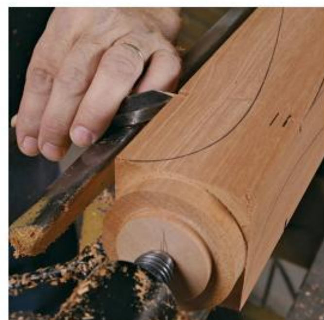
Define the chamfer. Use a parting tool to cut to the depth of the chamfer mark, then carry that chamfer down the rest of the leg.
