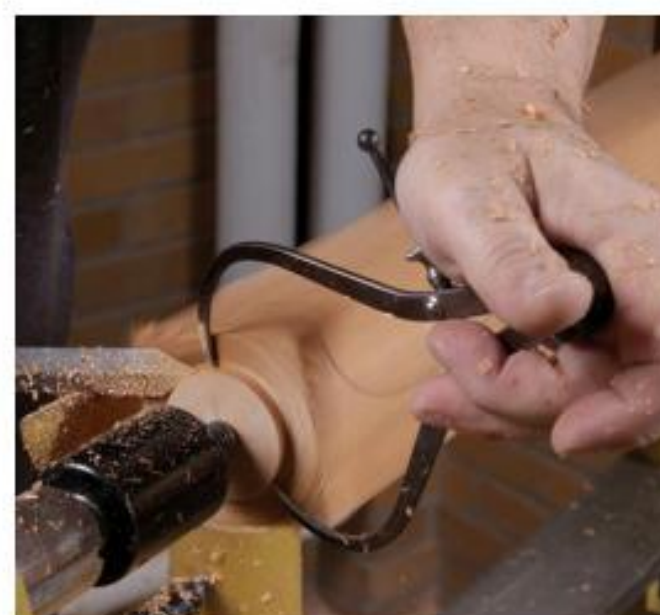
Turn the pad first. With a parting tool and calipers, turn the pad to a cylinder the same diameter as the inner line on the bottom pattern.
