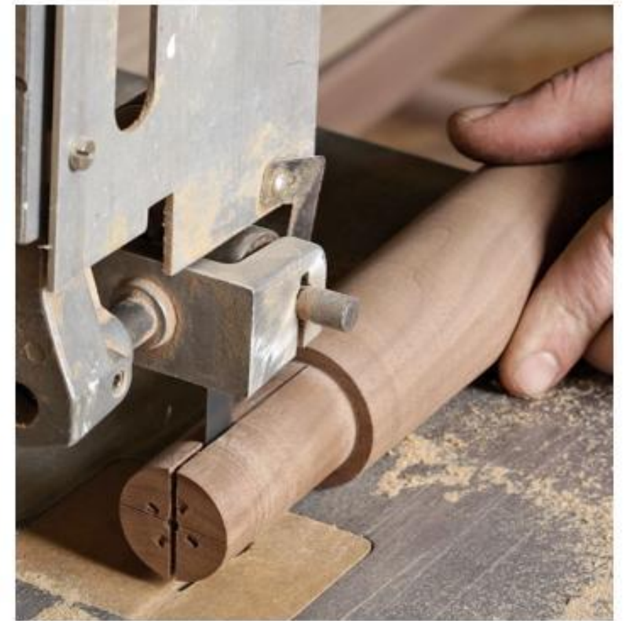
Turn and kerf. After turning the legs and stretchers, prepare the leg tenons for wedging by kerfing them on the bandsaw.
