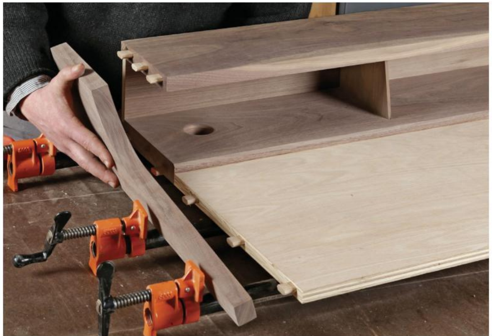
Final assembly. After setting the gallery back and drawer dividers in place, fit the gallery top (left). Then add the end caps (below).
