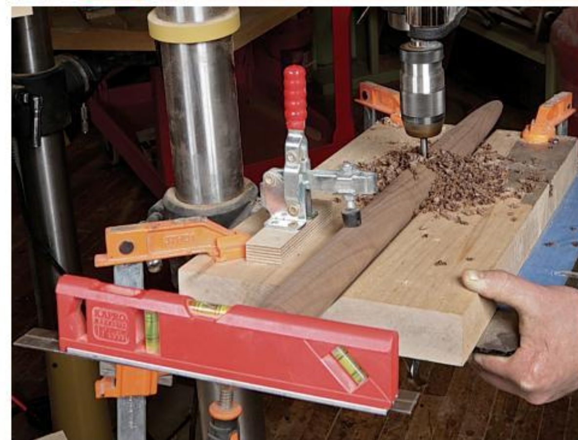
Mortising tips. To be sure the mortises in the rear leg for the side and rear stretchers are perpendicular to each other, Robbins slips a rule into the wedge kerf in the leg tenon and attaches a magnetic level to it. He then drills one mortise when the rule is vertical, the other when it's horizontal. While making the holes, the drill-press table is angled 3° to account for the rake and splay of the leg.
