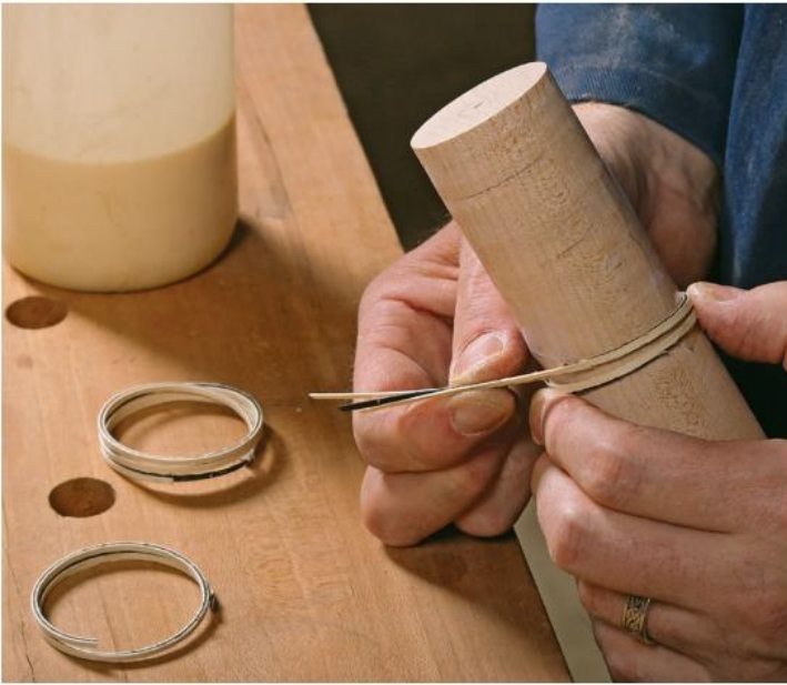
Wrap and tape. After adding glue to the strips, Latta wraps them around a cylinder. He again turns to clear tape to keep the thin stringing secure while the glue sets.
