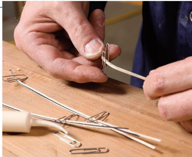
Prebend and glue just the end. Latta rolls the ends of the strips around a burn-in knife to start the radius for the cyma curve. Apply glue to one end of the pieces and clamp them using a paper clip. This will make the end stout enough to miter but leave the rest of the stringing, which is unglued, free to bend into the curves.
