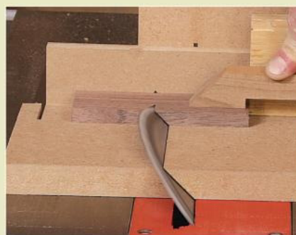
To maximize the length and strength of the slip tenons, Korsak glues them into intersecting mortises, being sure the miters meet. Once the glue cures, he proceeds with the full assembly.
