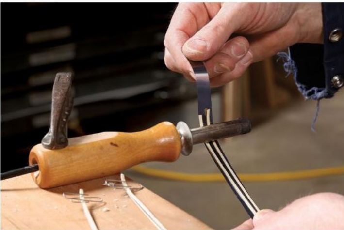
Prebend and glue just the end. Latta rolls the ends of the strips around a burn-in knife to start the radius for the cyma curve. Apply glue to one end of the pieces and clamp them using a paper clip. This will make the end stout enough to miter but leave the rest of the stringing, which is unglued, free to bend into the curves.
