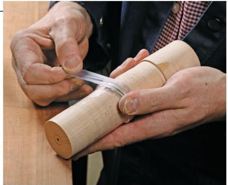
Wrap and tape. After adding glue to the strips, Latta wraps them around a cylinder. He again turns to clear tape to keep the thin stringing secure while the glue sets.
