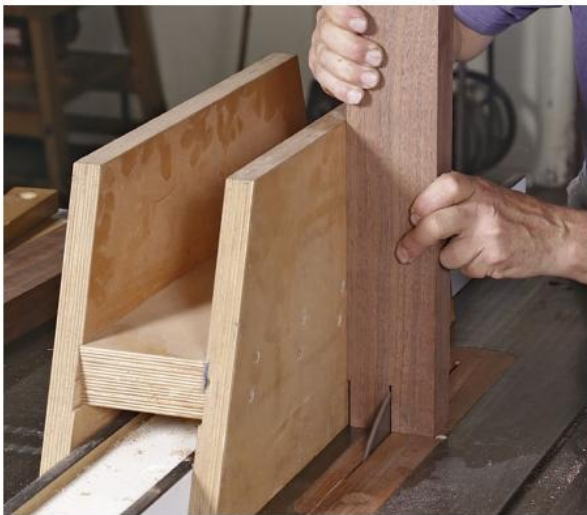
Tenons on top. Cullen cuts the cheeks of the through-tenon first, using a shopmade tenoning jig.
