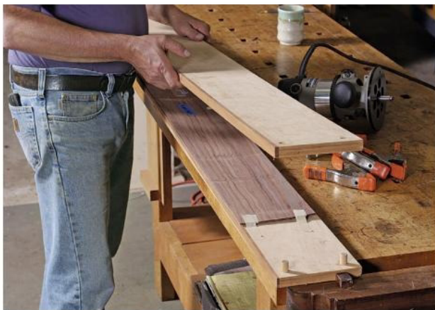
Shopsawn sheets. Sawing his own veneer enabled Cullen to match the solid wood in the bed exactly. He used a bandsaw to cut the claro walnut veneers \frac{1}{16} in. thick, then had them thickness sanded to \frac{3}{64} in. thick.
