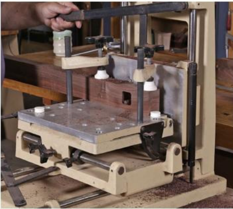
Multi-Router mortises. Cullen likes the Multi-Router for mortising because of its speed, accuracy, and easy setup.
