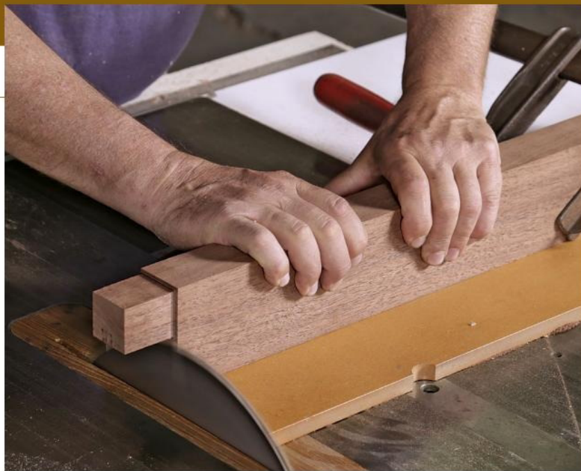
Shape the shoulders. With a crosscut jig on the tablesaw, Cullen cuts the tenon's shoulders: small ones first, wide one last.
