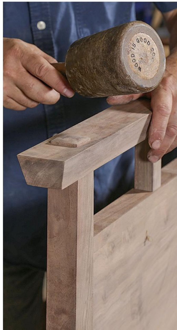
On with the posts. Using the tapered cutoffs as cauls, glue the posts to the rails and panels.
