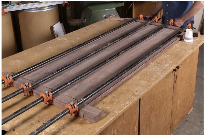
On with the posts. Using the tapered cutoffs as cauls, glue the posts to the rails and panels.
