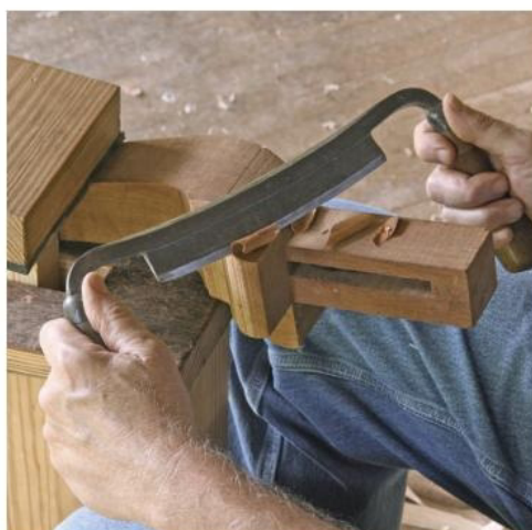
Smoothing tool too. Working bevel-up, Buchanan uses the drawknife to smooth the bandsawn curves of a cabriole leg.
