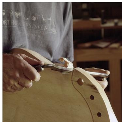
Deep scoop. The bevel-down knife allows Buchanan to make a deep incut on the side of a chair seat.
