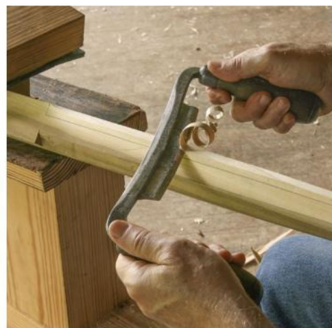
Stopped facets. Working on the leg of a table, Buchanan creates tapered facets that are stopped at the top end.
