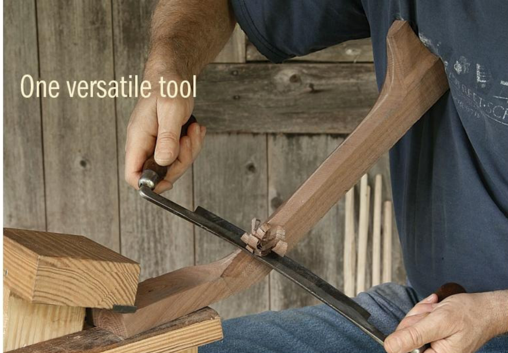
A natural at complex shaping. Used bevel down, the drawknife can create complex shapes with speed and precision. Here Buchanan carves a guitar neck.
