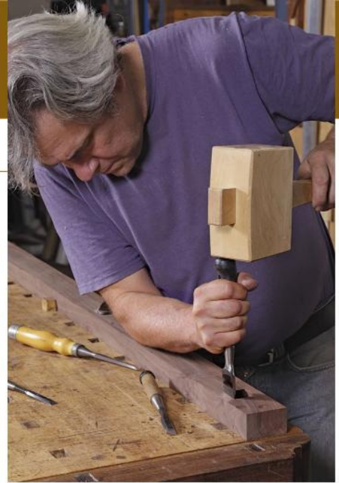
Chisel carefully. The through-tenon in the top rail is the bed's signature detail, and Cullen chisels to layout lines on both faces of the rail to make an impeccable mortise.
