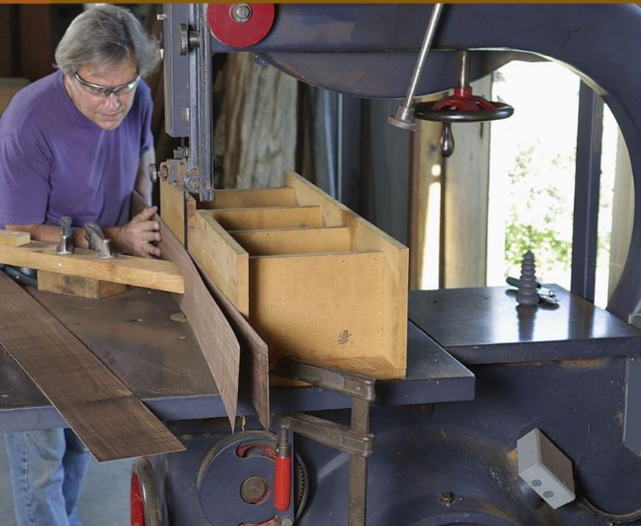
Shopsawn sheets. Sawing his own veneer enabled Cullen to match the solid wood in the bed exactly. He used a bandsaw to cut the claro walnut veneers \frac{1}{16} in. thick, then had them thickness sanded to \frac{3}{64} in. thick.
