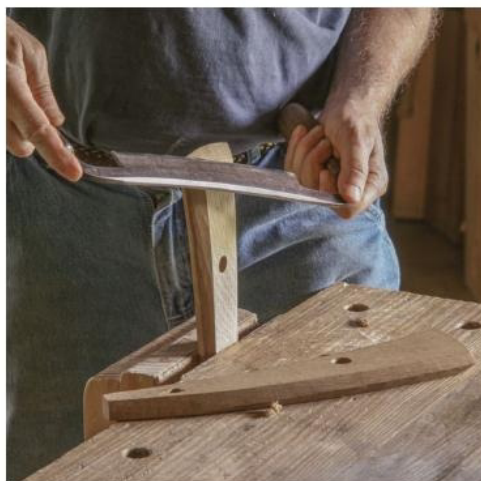
Give me an arm. With the workpiece in his bench vise, Buchanan shapes the end grain on the arm of a Windsor chair.
