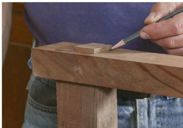
Build the pyramids. After marking around the tenon where it emerges from the upper gallery rail, Cullen uses a block plane, rasp, file, and sandpaper to shape the top to a softened pyramid.
