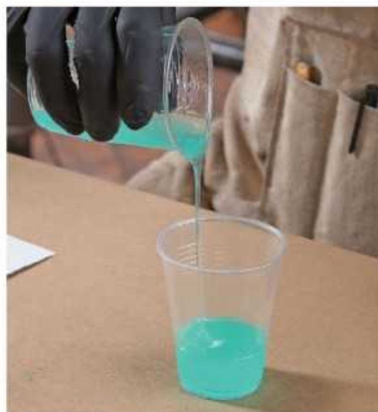
Mix the two parts. Moore uses a digital scale, because mixing by weight is more accurate than mixing by volume.
