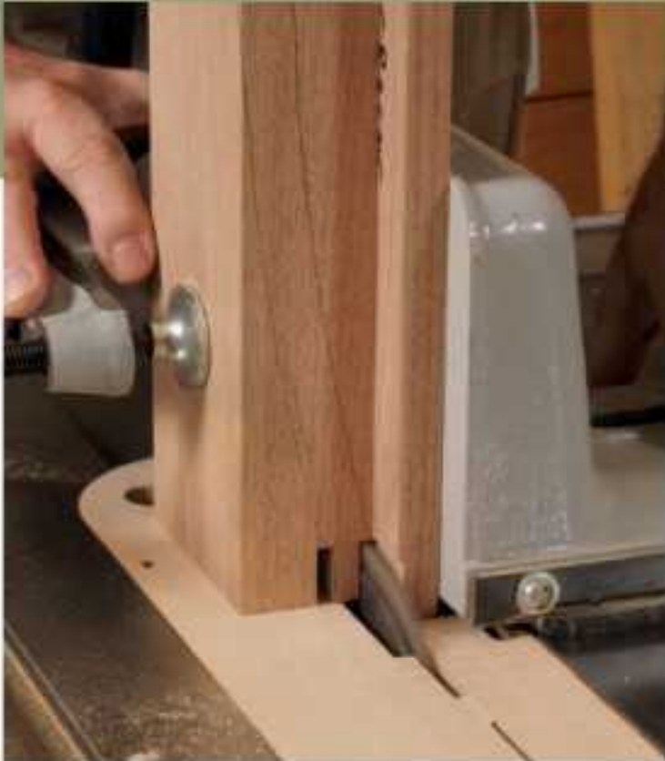
Cut the tenons before the curves. The same blade and spacer used for the seat rail tenons are used for the back rails as well.
