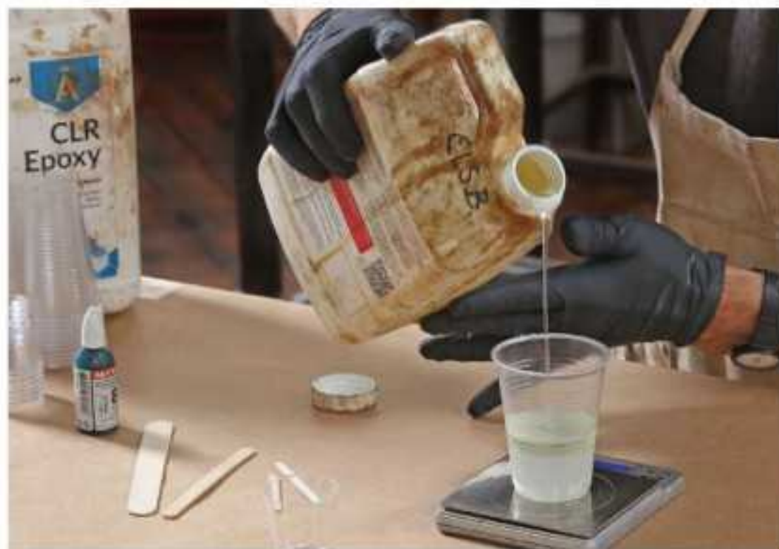
Mix the two parts. Moore uses a digital scale, because mixing by weight is more accurate than mixing by volume.
