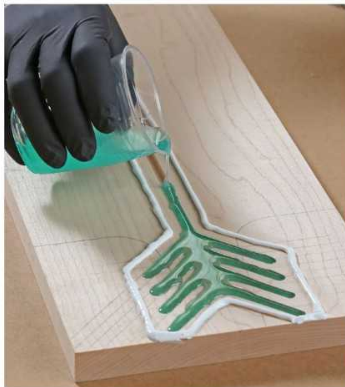
Overfill the grooves. Level the board first. Let the epoxy run through the grooves and rise above the surface (below). Most air bubbles will be found up in this excess, rather than down in the groove.
