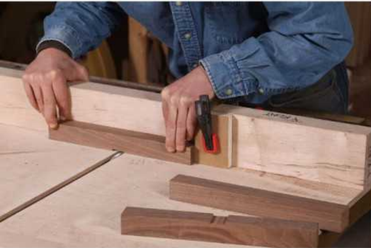
A notch for the brass. Using a dado blade and a stop, Robbins cuts the centered dado for the brass bar in two passes.
