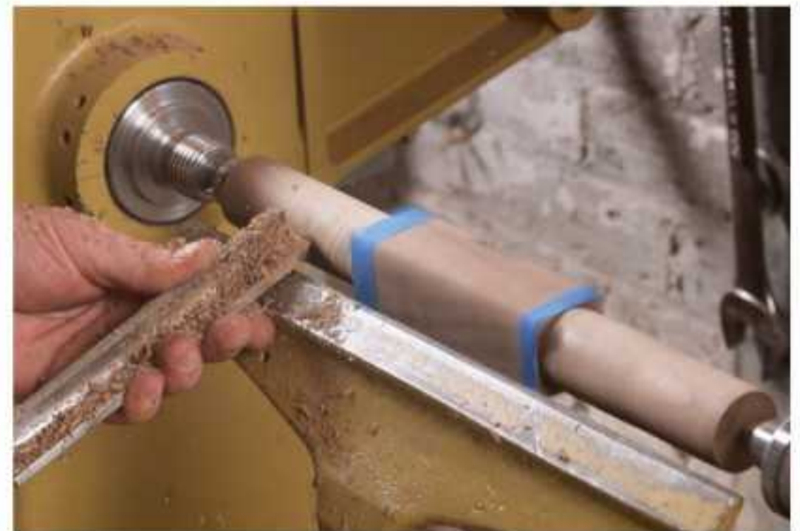
Tape trick. Robbins wraps the blanks with blue tape to ensure he'll get a clean transition between the square and cylindrical sections of the stretcher when he turns them on the lathe.
