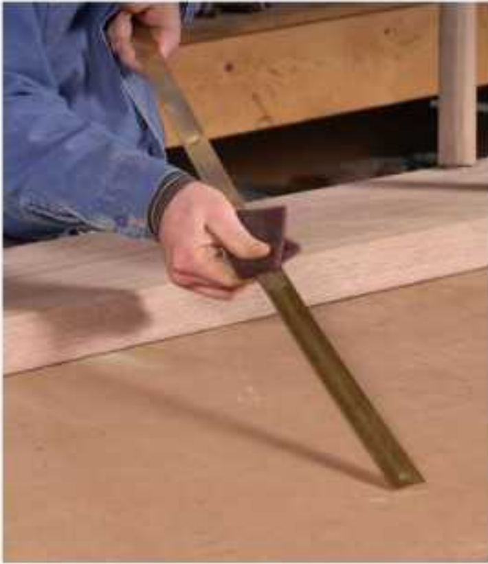
Quick cleaning. Rubbing with a Scotch Brite metal finishing pad makes the brass gleam.
