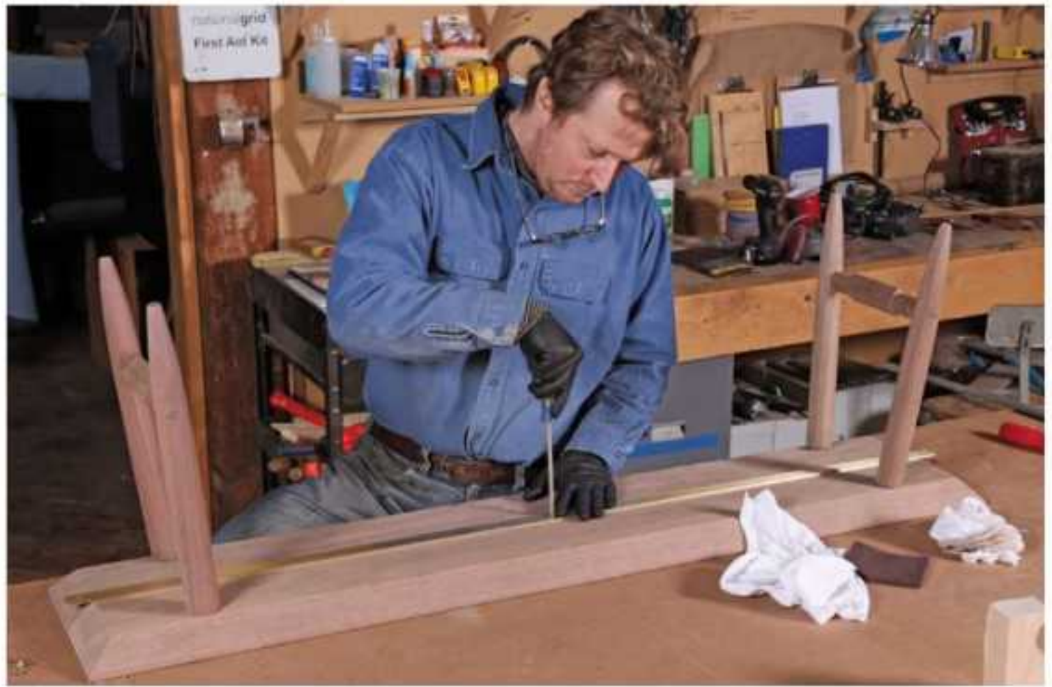
Tighten the screws. After driving the center screw (above), Robbins installs the knock-down fittings through the stretchers (below). Rubber gloves keep him from smudging the brass.
