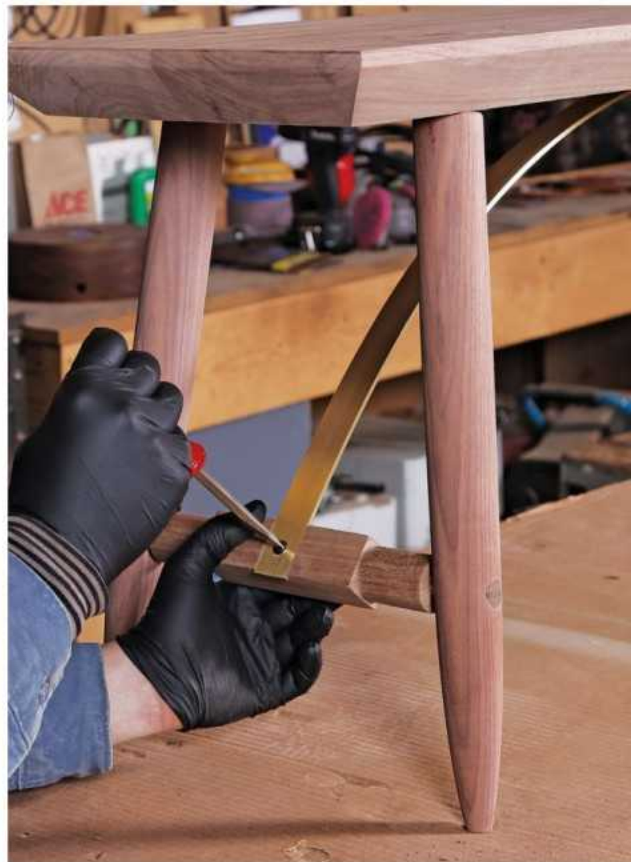
Tighten the screws. After driving the center screw (above), Robbins installs the knock-down fittings through the stretchers (below). Rubber gloves keep him from smudging the brass.
