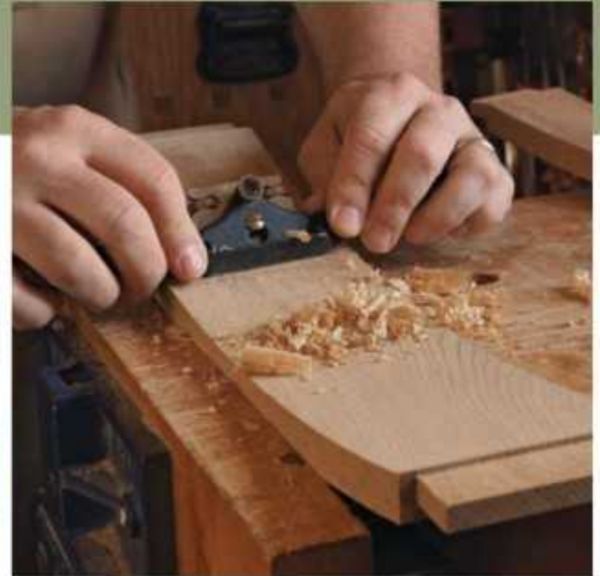
Saw and smooth the curves. A steady hand and sharp blade at the bandsaw should leave just a little waste to clean up. Pekovich uses a spokeshave followed by a card scraper to quickly smooth away the bandsaw marks.
