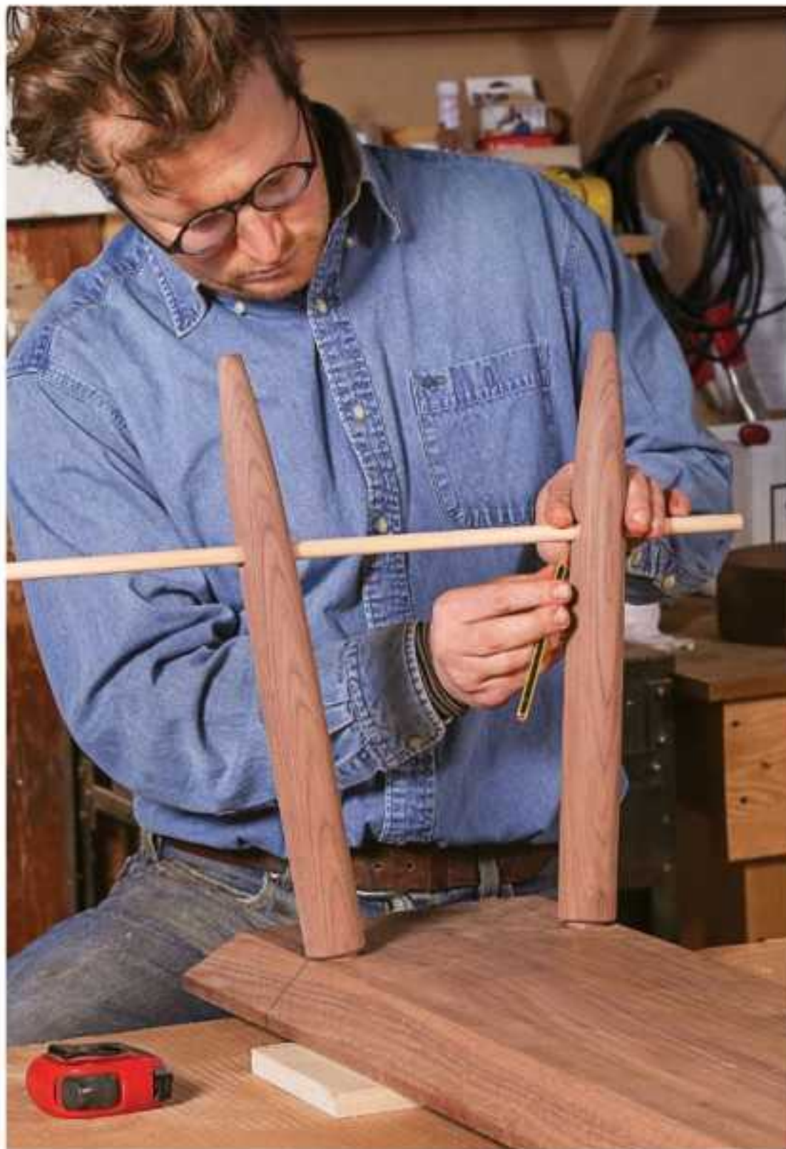
Dimensioning by dowel. To get a precise shoulder-to-shoulder measurement for the stretcher blank, Robbins dry-fits the legs and marks a dowel rod threaded through the stretcher mortises.
